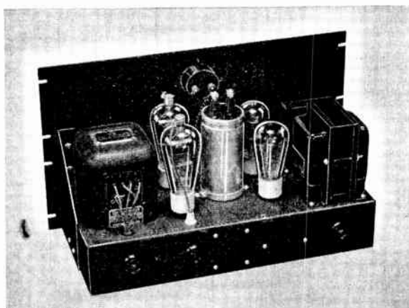
MODULATOR AND POWER SUPPLY Chassis: 17" x 10" x 3"; Panel: 10 1/2"
