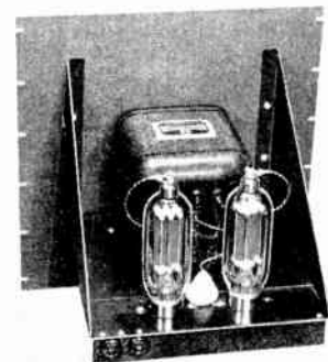
CLASS B MODULATOR Chassis: 13" w. x 13 1/2" d.; Panel: 19 1/4"
