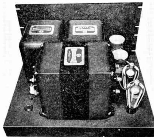
HIGH VOLTAGE POWER SUPPLY Chassis: 20 1/4" x 15 3/4" x 2 1/2"; Panel: 10 1/2"
