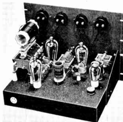
R. F. UNIT Chassis: 17" x 12" x 3"; Panel: 14"
