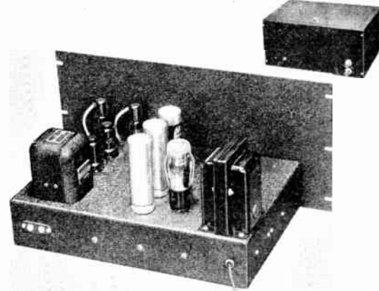
PRE-AMPLIFIER CHASSIS AND ASSEMBLY Chassis: 17" x 10" x 3"; Case: 19" x 13" x 8 3/4"
