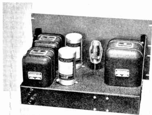
EXCITER POWER SUPPLY Chassis: 17" x 10" x 3"; Panel: 10 1/2"
