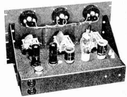
EXCITER UNIT Chassis: 17" x 10" x 3"; Panel: 10 1/2"
