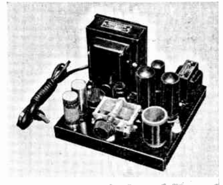
CHASSIS VIEW Chassis: 8" x 3" x 1"
