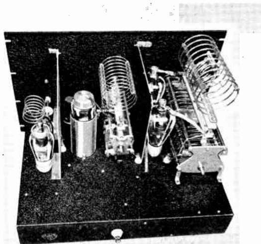
R. F. UNIT Chassis: 17" x 13" x 3"; Panel: 12 1/4"
