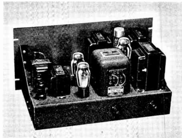
SPEECH AMPLIFIER AND POWER SUPPLY Chassis: 17" x 10" x 3"; Panel: 8¾"
