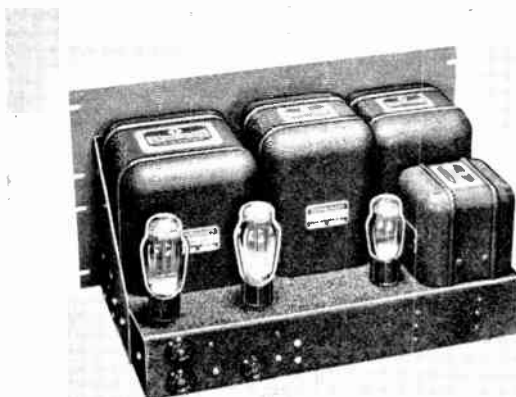
SPEECH AMPLIFIER AND MODULATOR POWER SUPPLIES Chcassis: 17" x 10" x 3"; Panel: 10 1/2"
