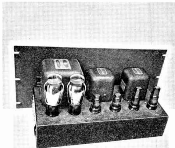
SPEECH AMPLIFIER AND DRIVER Chassis: 15" x 7 1/2" x 3"; Panel: 8 3/4"
