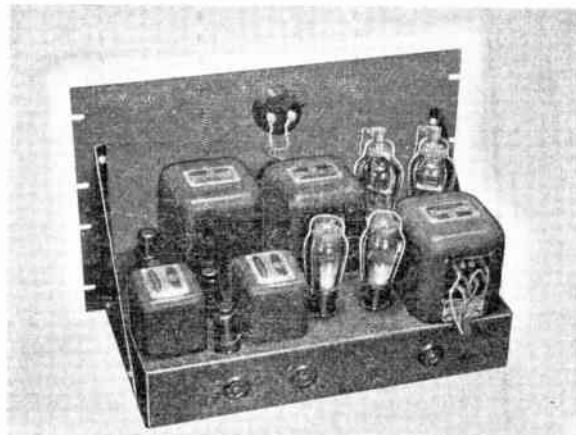
SPEECH AMPLIFIER AND MODULATOR Chassis: 17" x 10" x 3"; Panel: 12 1/4"
