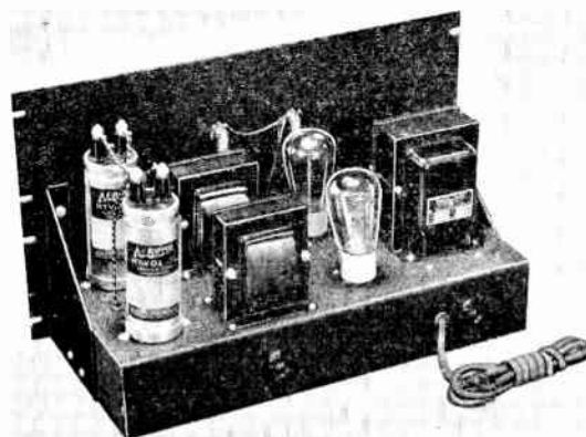
R. F. POWER SUPPLY Chassis: 17" x 10" x 3"; Panel: 10 1/2"
