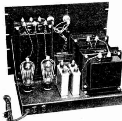
HIGH VOLTAGE POWER SUPPLY Chassis: 17" x 14" x 2"; Panel: 14"
