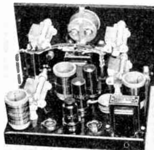
CHASSIS VIEW Chassis: 9 1/2" x 7 1/2" x 1"
