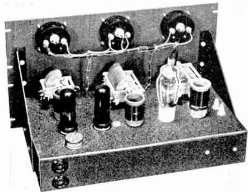
EXCITER UNIT Chassis: 17" x 10" x 3"; Panel: 10 1/2"
