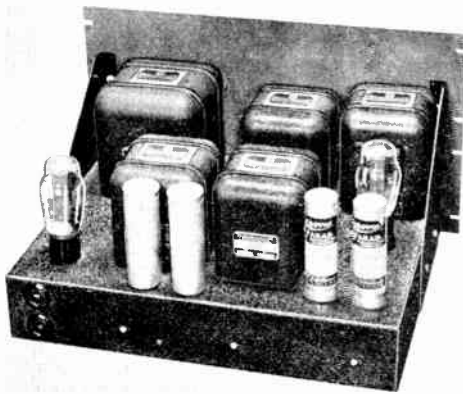
BIAS AND EXCITER POWER SUPPLIES Chassis: 17" x 13" x 3"; Panel: 10 1/2"
