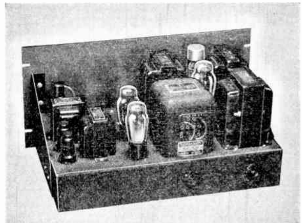
SPEECH AMPLIFIER AND POWER SUPPLY Chassis: 17" x 10" x 3"; Panel: 8 3 / 4 "
