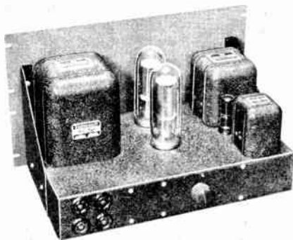
DRIVER AND SPEECH Chassis: 17" x 10" x 3"; Panel: 10 1/2"
