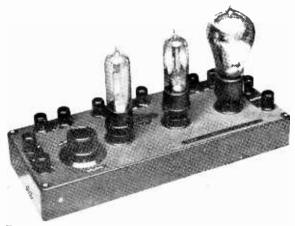
FIG. 34. IGRANIC 3-VALVE RESISTANCE CAPACITY AMPLIFIER
