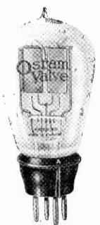
FIG. 20. THE OSRAM U.5 RECTIFYING VALVE
