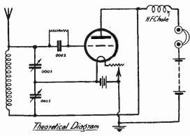
FIG. 5. COLPITTS ONE-VALVE CIRCUIT
