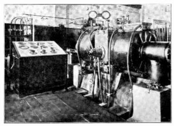
FIG. 4. AN ARC TRANSMITTER AT THE OXFORD STATION
