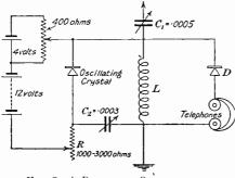
FIG. 7. A PRACTICAL OSCILLATING CRYSTAL CIRCUIT
