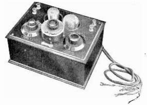
FIG. 33. THE B.T.-H. TWO-VALVE L.F. SET
