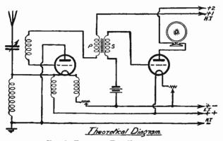
FIG. 3. FILADYNE TWO-VALVE CIRCUIT
