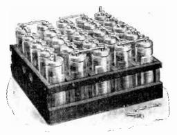
FIG. 10. C.A.V. 60 VOLT, 2 AMP. HIGH-TENSION ACCUMULATOR
