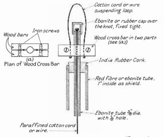
FIG. 1. SECTION OF AN AERIAL INSULATOR. (FLEMING)
