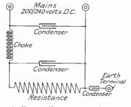
FIG. 4. RADIAC HIGH-TENSION MAINS UNIT DIAGRAM OF CONNECTIONS
