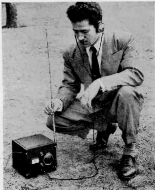
This portable set, designed for defense organizations, picks up near-by broadcasts without the use of a ground
