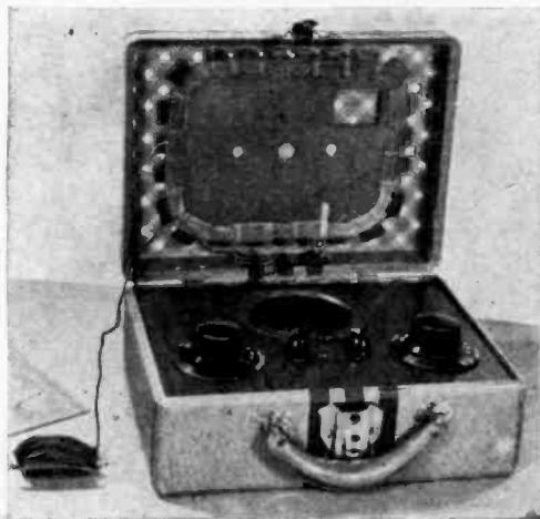
The 9\frac{1}{2} " by 7\frac{1}{2} " loop antenna goes inside the lid of the case and can be concealed by paper if desired
