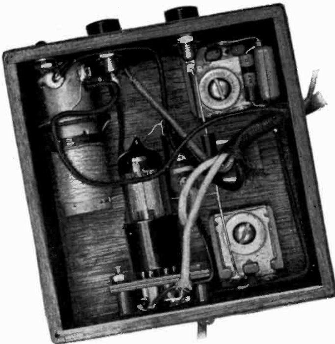
Padding condensers replace the usual-type tuning condensers. Note cabinet details at right
