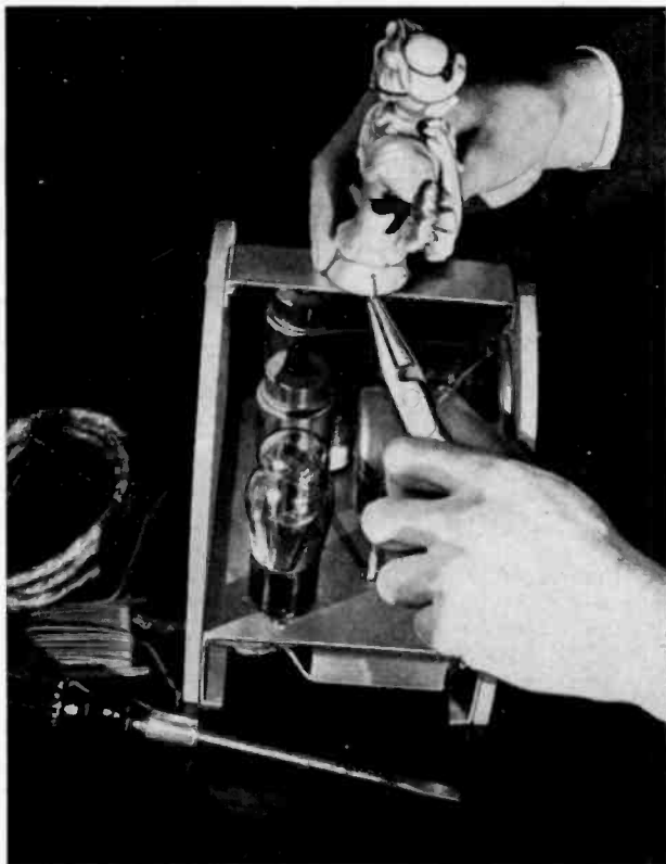
Wire and glue can be used to mount the porcelain figurine on the aluminum brace at the top of the cabinet. Suitable dolls, once popular as telephone covers, can be obtained for a dollar or less
