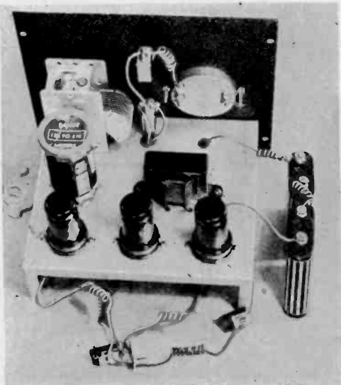
Tubes shown here are the new all-metal, 6.3-volt 6SJ7 type, but battery 1SA6GT tubes will serve
