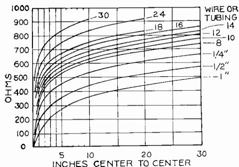
Handy quick-reference chart for determining surge impedance from spacing and wire size of line.
