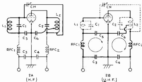
period that the exciting voltage is positive, and then when the grid goes negative, for the oscillation to cease. It will then start up on the next positive cycle, etc. If the ultra-high frequency oscillation is very strong, it would be conceivable for the amplifier to oscillate all the time, instead of only on the positive halves of the excitation voltage.
