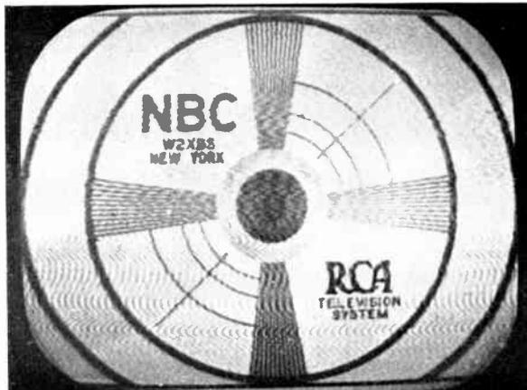
Figure 45—Excessive Diathermy Interference
