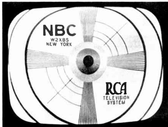
**Figure 41—Vertical Linearity Control Incorrectly Set**
