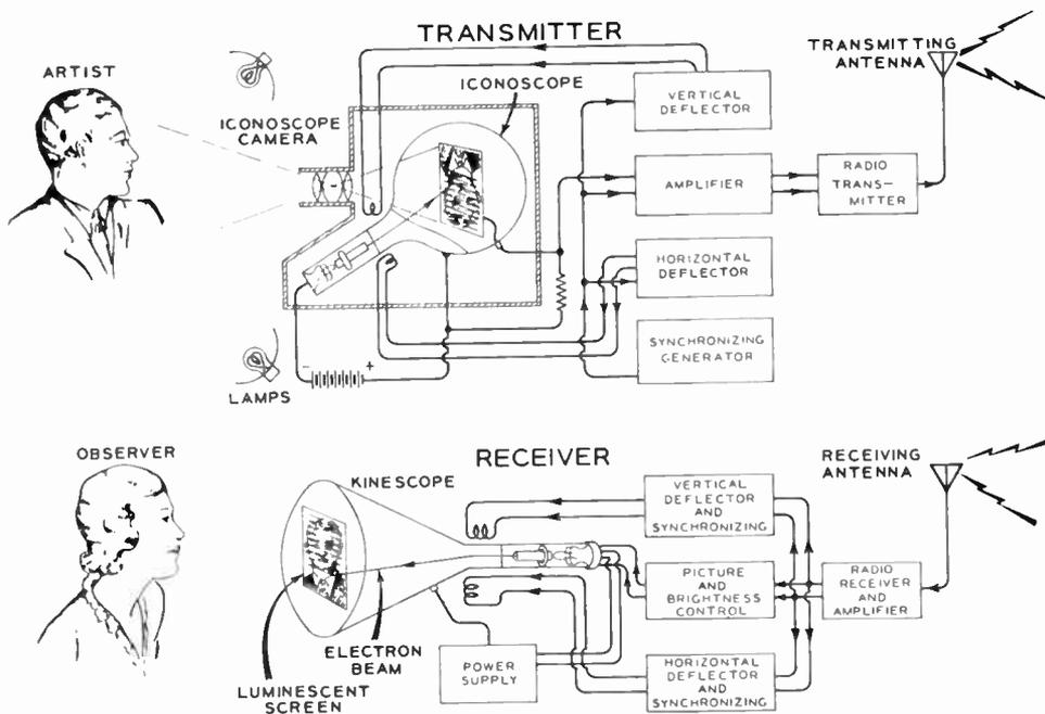
**Figure 1—Schematic of RCA Television System
