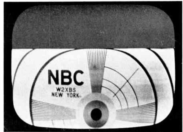
**Figure 38—Vertical Centering Control Incorrectly Set**
