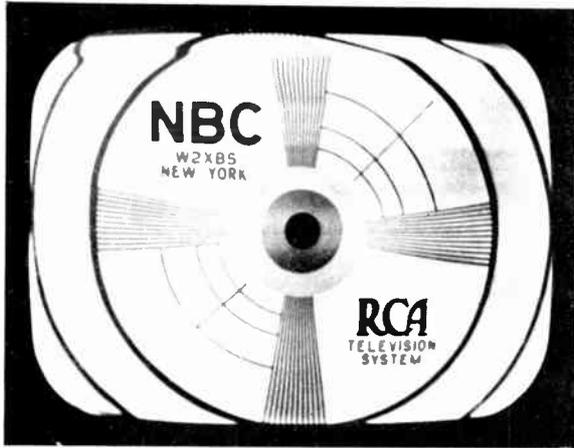
**Figure 52—Unstable—“Tear-Out”—Horizontal Synchronization**
