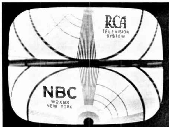
Figure 28—Vertical Hold Control Incorrectly Set
