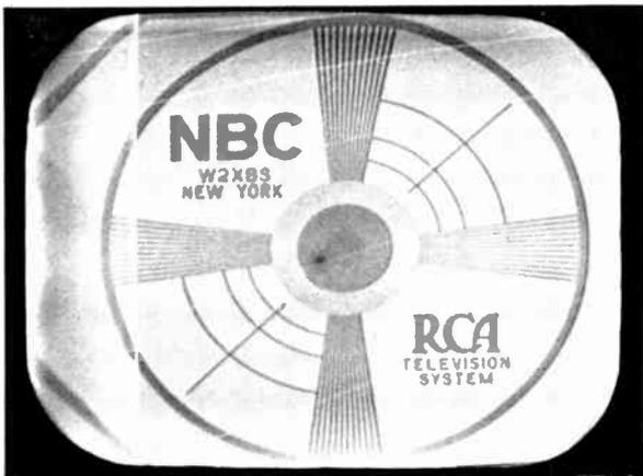
Figure 60—Effect of Damping Tube Failure
