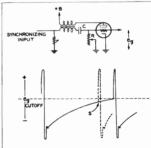
Figure 15—Blocking Oscillator and Wave-form
