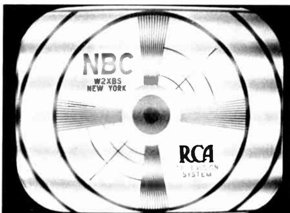
**Figure 33—Sound Modulation in Picture**
