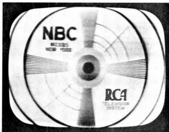
Figure 58—Loss of High Video Frequencies
