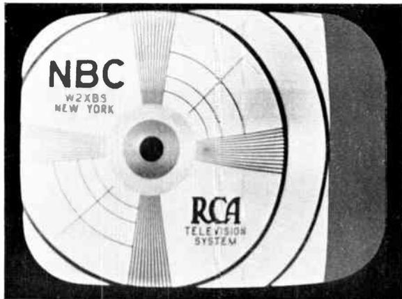
**Figure 36—Horizontal Centering Control Incorrectly Set**
