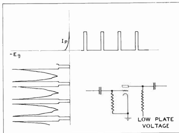
Figure 11—Operation of Synchronizing Separator
