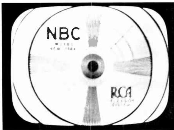
Figure 29—Focus Control Incorrectly Set
