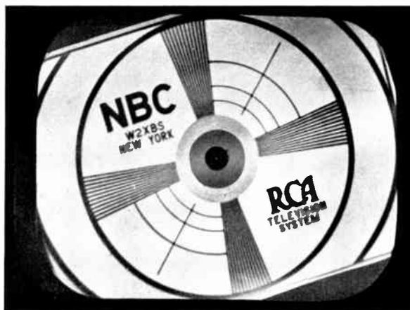
**Figure 34—Picture Incorrectly Oriented**
