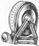
A beautiful new vernier dial made of tarnish-proof etched brass. Smooth, positive action and very efficient. Mounts on sub-panel. Large diameter, deep knurled knob makes tuning grip positive and effortless. Strap drive. Two take up drums on drive shaft. Straps anchored to hull on 180 degree rotation, scale 0-100. Tension spring insures tight straps at all times. Dial is ivory celluloid, lighted. Shipping weight, 2 pounds.
