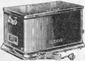
The Reliable "B" is a quiet, economical "B" battery eliminator. It has two variable controls—detector and amplifier, with an extra power tube tap, supplying 135 to 180 volts, and blading posts for negative "B," detector, amplifier and power.
