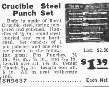
Body is made of finest Crucible steel, spring tempered and polished. Handles of 3/4 in. round steel, knurled and case hardened. Set consists of 4 pin punches and one center punch in the following sizes: Pin Punches, 1/8 in., 3/16 in., 1/4 in., and 5/16 in. Length over all, 7 3/4 in. Center Punch, 3/16 in. Length over all, 6 in. All in neat leatherette roll.
