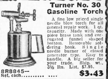
A fine low priced single needle blow torch for all general repair work. 1 qt. capacity. Made with one piece brass tank and corrugated funnel shaped bottom. Removable soldering hook. Single needle burner of closed generator type. Easy to handle. A big seller for your trade. Ship. wt., 3 1/2 lbs. List, \$7.95.
