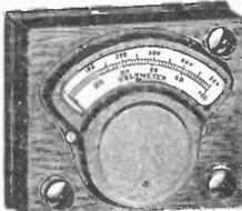
A high resistance Voltmeter for use with "B" eliminators. Much more satisfactory than ordinary voltmeters as it uses very little current, 1 M.A. for the whole scale deflection. Resistance is 1,000 ohms per volt. A very sensitive and high grade instrument. Quantity production makes possible the extremely low price we are able to offer, on scales—0-100; 0-500. Shipping weight, 4 lbs. **3R1800**—List, \$28.00. **Net \$20.58**
