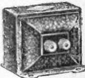
The 30 Henry filter choke has an inductance of 30 henries at approximately 40 mls. This drops somewhat below 30 henries on a 20 mil. load. The DC resistance is 375 ohms. Most efficient with the current from 0 to 60 mls; will not overheat with a load of 85 mls. Used in a filter circuit for B Eliminators, also across output terminals of set in conjunction with a 2 Mfd. condenser to keep high DC current from loud speaker. Completely shielded.
