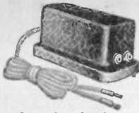
A device consisting of a series of resistances in one case which, placed between any loud speaker and set, will greatly improve reception. It eliminates the direct plate current from speaker winding, thereby increasing volume, yet preventing distortion. It increases frequency range of speaker, especially bringing out full roundness of lower frequencies. Attached in half minute. Case is 4 1/2" x 2 1/2" x 2 1/2" inches brown crystal finish.
