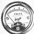
Equipped With D'Arsonval Movement, resistance, 70 ohms per volt. Cases 2 inches in diameter; 2 1/4 inches across front flange. Zero adjuster provided. All cases flush mounting. Black finish. Ship. wt., 3 lbs.
