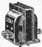
Those Audio Transformers are sealed in black enameled cases to prevent moisture from getting into coils. Built of the highest grade materials to the strictest specifications. Special laminated core insures even distribution to flux through entire circuit. Nickel plated binding posts mounted on Bakelite insulation. 2 3/4 inches high by 2 1/4 inches wide and 2 5/8 inches deep. Ship. wt., 1 lb.
