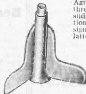
This is a close-up view of the Agitator itself. You can see the three large paddles that give the suds a swift, turbulent, rolling action, and the three specially designed intermediate webs. These latter increase the force of the action, and at the same time protect the clothes from being damaged by winding around post. The Agitator washes the grimest garments as easily as the sheepest silks, without damage or injury to material.
