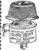
A variable high resistance that provides a positive, gradual, durable, reliable and fool proof adjustment over a range of from practically zero to five megohms or five million ohms. Will carry a capacity of 20 watts and is absolutely noiseless. It is being used in most factory built "B" Battery eliminators for regulating the plate voltage. Requires one 7/16-inch hole for mounting.
