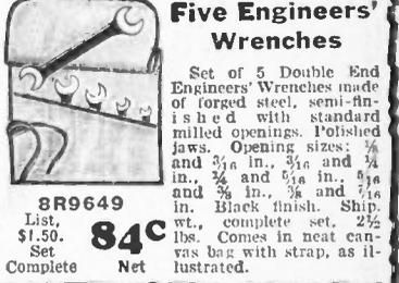
Set of 5 Double End Engineers' Wrenches made of forged steel, semi-finished with standard milled openings. Polished jaws. Opening sizes: 1/8 and 3/16 in., 3/16 and 1/4 in., 1/4 and 5/16 in., 5/16 and 3/8 in., 3/8 and 7/16 in. Black finish. Ship. wt., complete set, 2 1/2 lbs. Comes in neat canvas bag with strap, as illustrated.
