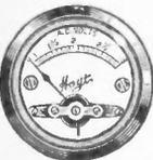
A panel voltmeter for use with AC operated receivers, or for small test panels. The resistance even in the lowest range is over 20 ohms per volt. The case is two inches in diameter for flush mounting with a narrow black rim. Ship. wt., 3 lbs.
