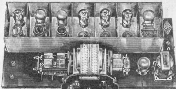
cluding panel, subpanel and incidental parts; two 110 Universal drum dials; 632 2 in. line condensers, 639 twin rotor condenser, Frost 500,000 ohm volume control, Frost 200,000 ohm sensitivity control, Frost 10 ohm gen. short at and switch, Frost cable plug, cable plug socket and Remler 920 audio transformer. Shipping weight, 18 lbs.
