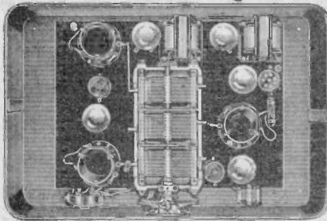
A newly developed five-tube receiver using "Chronophase" radio frequency amplifier. There are three models—Shield Grid model, using two 222, two 201A, one 171 tubes—AC model, using four 227 and one 171 tubes—DC model, using four 201A and one 171 tubes. Very convenient tuning with single knob, two additional controls for volume and trimming.
