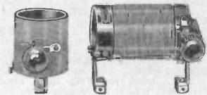
Small size, only 2 inches in diameter. Embody the slot wound primary for extremely high efficiency. Wound on bakelite tubes with trimmers and tickler coils mounted inside. Control shafts protrude through the walls of the tubes and may be regulated from the front of the panel. Convenient knobs provided for this purpose. Complete with mounting feet and soldering lugs on all connections.
