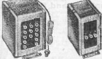
A power transformer suitable for use with a pair of 210 tubes in push-pull, a single 250 or any others of similar characteristics. A high voltage winding of 1,000 volts provided, giving 500 on either side of the center tap. Filament windings of 7 1/2 volts for 210 and 250 tubes. Another of same value for the two 281 rectifying tubes. Low voltage windings for AC tubes. Ship. wt., 7 lbs. 3R1319—List, \$19.00. Net... **\$9.75**
