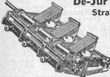
Compact, light in weight and rigid in construction. Equally efficient on high and low wavelengths and being of "straight line frequency" type will spread the stations evenly over the dial. All insulation used is of genuine molded bakelite and is placed outside of electrostatic field reducing dielectric loss to a minimum. Hand capacity is eliminated by grounding end plates to rotor.
