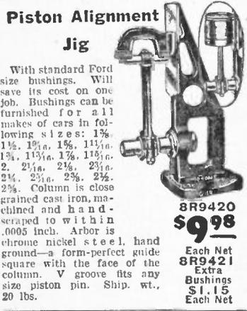
With standard Ford size bushings. Will save its cost on one job. Bushings can be furnished for all makes of cars in following sizes: 1 1/2, 1 3/4, 1 7/8, 1 13/16, 1 15/16, 1 7/8, 1 13/16, 2, 2 1/16, 2 1/8, 2 1/4, 2 1/2, 2 3/8, 2 1/2, 2 5/8, 2 3/4, 2 7/8. Column is close grained cast iron, machined and hand scraped to within .0005 inch. Arbor is chrome nickel steel, hand ground—a form-perfect guide square with the face of the column. V groove fits any size piston pin. Ship. wt., 20 lbs.
