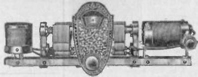
The Tuning Unit used in the new National Browning-Drake Tuner illustrated to the left. A great improvement on devices which have gone before. Actuated by a single dial control. Consists of two National Tuning condensers and coils. Antenna trimmer on left hand one, tickler regeneration control on right. Both regulated by knobs which are on face of panel. Entire unit mounted on a single base. Installed as a unit. Only four holes to drill in panel. Shipping weight, 12 pounds.
