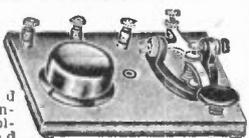
Key and buzzer mounted on a polished wood base. Connect a dry battery to the binding posts on the set, press the key and a buzzing sound will be produced. In a very short time your ear will become accustomed to the various combinations of dots and dashes representing different letters and numerals. Chart included with each set. Base size, 7 inches long by 4 1/2 inches wide.
