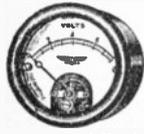
The smallest of the d'Arsonval or moving coil meters. A compact instrument with 2-inch case diameter and 2 1/4-inch rim diameter. Finest coil type movement fully jeweled. Resistance of voltmeters 80 ohms per volt. Black scale on silver background. Ship. wt., 2 lbs.
