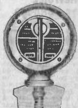
Genuine Boyce Meters are now standard equipment on practically all of the leading makes of cars. The most dependable heat indicator on the market today is placed on the radiator cap; it acts as a faithful guard over the motor. It will save many dollars in repair costs by warning the driver when his motor is too hot. Easily attached by drilling small hole in radiator cap.
