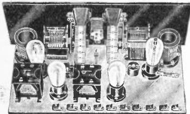
THE famous S-M Universal All Wave Tuners are now more popular than ever. They provide a low price yet ultra efficient tuner for every purpose. The well known four tube circuit so widely popularized—one R.F. stage and regenerative detector followed by two audio stages is used with S-M correctly engineered parts to give truly amazing results. The selectivity is ample for any congested broadcast district, and the reproduction is superb.
