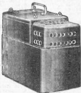
A new and improved device that converts a set using ordinary tubes into an electric set. Instead of using stepped-down raw alternating current to light the filaments of radio tubes, the "ABOX" removes the ripples and delivers smooth direct current so that the ordinary 201A tube can be operated from the AC.
