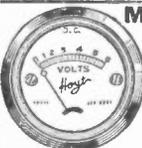
Well-made, dependable meters at a low cost. Both AC and DC types are accurate enough for ordinary readings, but this type meter is not recommended for precision laboratory work. DC meters are magnetic type; AC meters are repulsion type, 2 inch cases with 1/2 inch flange. Shipping weight, 1 lb. 1/2 inch flange. Shipping weight, 1 pound. **DIRECT CURRENT TYPE**
