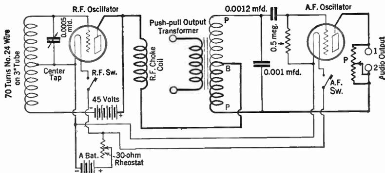
All the constants of the apparatus used in the instrument are given on the diagram. Some information on the use of this instrument will be found on Laboratory Sheet No. 163. The frequency of the audio-frequency oscillations can be varied by using various values of capacity across the push-pull transformer.
