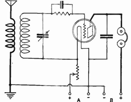
strength will be decreased. For the ordinary 201-A type tube, a grid leak of about four megohms resistance will give the best results. If a soft detector tube is used, a somewhat lower resistance leak is generally required; about one half to two megohms being about right.
