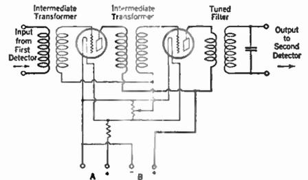
Regeneration in the intermediate-frequency amplifier will considerably improve the selectivity and sensitivity by sharpening the resonance curves of the transformers.
