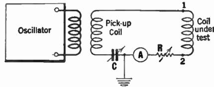
frequency at which the measurements are to be made. It should have plenty of power. In the Laboratory a 210 tube with at least 300 volts on the plate is generally used, but it is doubtlessly possible to use a 201-A as an oscillator with about 100 volts on the plate. The important point is that adjustments in the test circuit should produce no change in the energy delivered by the oscillator.
