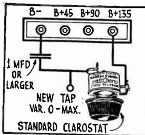
at the right. Since most B-eliminators today have excessive maximum voltage for the -71 or the -12 type power tube, the voltage drop introduced by this method will, if anything, prove desirable in protecting the power tube.
