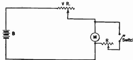
meter. We might have a 10-milliampere meter and desire to read a current of, say, 50 milliamperes; with the aid of a shunt, this can easily be done. The method of calibrating a shunt is indicated in the diagram.
