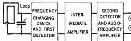
of several r. f. stages (known as the intermediate-frequency amplifier), a detector (the second detector), and the usual audio amplifier.
