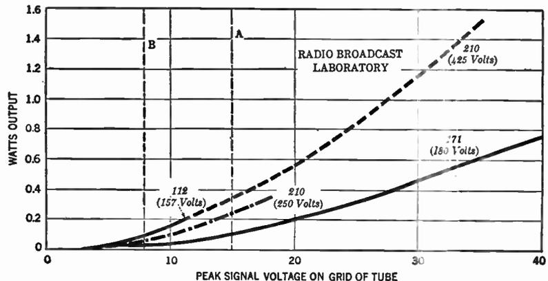
These curves indicate how the power output of the 112, 171, and 210 type tubes varies with different values of signal voltage on the grid of the tube. The significance of these curves is explained in detail on Laboratory Sheet No. 161.
