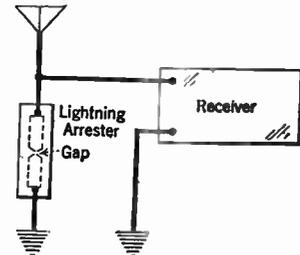
approaching, there is a considerable amount of static electricity present in the atmosphere which tends to accumulate on the antenna system until such time as the voltage is high enough to jump across the small gap in the arrester. This discharge voltage is generally about 500 volts.
