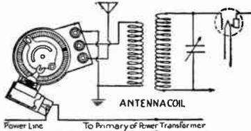
Fig. 2—Tonatrol Type R Circuit
