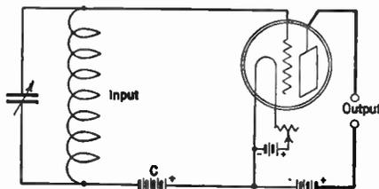
When no signals are being received, the plate current is constant and depends on the adjustment of the C battery. For best operation of a detector of this type, about four volts of C battery should be used on the 201-A when 45 volts are used on the plate. When a signal is received, the plate current varies and is then made up of two compon-
