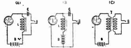
Laboratory, a resistance of 37 ohms in the B power unit, using circuit "A," produced continuous oscillations, whereas a resistance of 600 ohms was necessary in circuit "B" before oscillations were produced.
