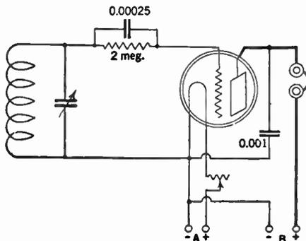
cal adjustment and will operate on from 40 volts up to the maximum that can safely be placed on the tube.
