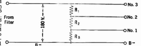
Resistance units for B power units are usually rated in watts and it is essential that the resistances used be capable of carrying the necessary load without overheating. The load in watts being handled by a resistance can be determined by multiplying the resistance in ohms by the square of the current in amperes. In this particular example:
