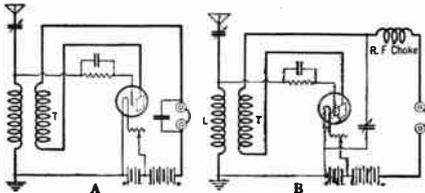
There are several methods of controlling feedback, either by a variable tickler as in A or by a variable resistance shunted across a fixed tickler coil. Another method is by the use of a variable condenser, as illustrated in B.
