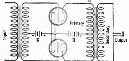
tant, and unless the same care is taken in designing as with an ordinary transformer, the actual results obtained will not make the push-pull arrangement worth while. It is essential that a push-pull transformer have a very high impedance primary and that the frequency characteristic of the transformer be reasonably flat.
