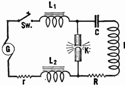
When the discharge is complete, the cycle of charge and discharge repeats itself with a frequency determined by the constants of the inductance L and the capacity C. By carefully choosing these values, large amounts of high-frequency energy can be obtained.
