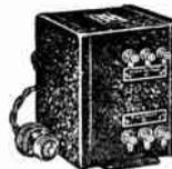
A power supply transformer designed to supply A, B, and C current to two UX-210 power tubes and plate current for the receiver. Rectifies through two UX-281 tubes. T-2098, list price \$20.00.
