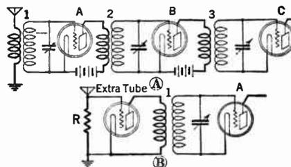
permits exact tuning of each circuit to resonance. In some cases this device consists of a small midget condenser connected in parallel with one of the main tuning elements; sometimes the stationary plates of one of the condensers are mounted on a pivot so as to permit more accurate tuning. But no receiver that has such an adjustable feature can accurately be called a single-control set.
