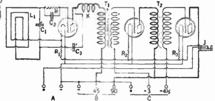
At all times during the operation of the receiver, care should be taken so as to keep the detector tube below the oscillating point since, if this tube does oscillate, a certain amount of radiation will take place which will produce interference with other receivers. Since a loop is being used, this radiation will not be very great, however.
