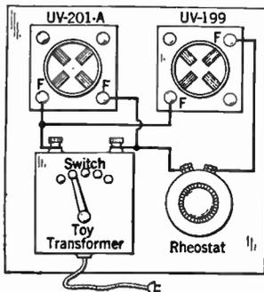
The procedure to be followed in treating a 199 tube is practically the same. At first the tube is "flashed" at eight volts for half a minute. The switch is then placed at the lowest voltage, which is usually about six volts, and then the rheostat is used in order to reduce the voltage to 4½ volts. With this applied voltage the tube is cooked for half an hour, when the treatment is complete.
