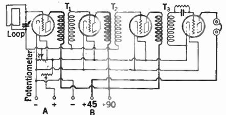
$T_1$ ,  $T_2$ , and  $T_3$ . Receiving sets of this type are not very selective as there is only one tuned circuit to do the "selecting," but they are easy to operate as the tuning condenser and the potentiometer are the only controls. Unless an arrangement for plugging in different transformers is provided, the range over which best amplification is obtained is usually only about two hundred meters.
