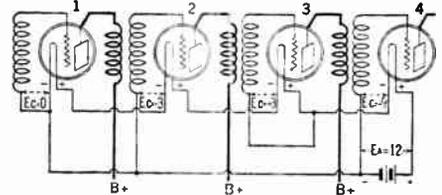
negative bias of 9 since between its negative filament lead and the point where its grid return is connected is the voltage drop caused by three preceding tubes. In the diagram,  $E_c$  represents grid volts. In the article entitled "An A. B. C. Line Supply Device" in the October, 1923, RADIO BROADCAST, diagrams are given of receivers with filaments in series.
