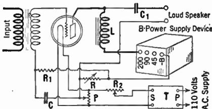
The variable resistance, R, controlling the grid bias, should not be lowered to a value less than 1000 ohms. It should be adjusted to that value (something above 1000 ohms) which gives the best quality of reproduction.
