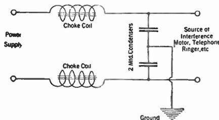
must operate. There will be little difficulty in obtaining satisfactory condensers for use on direct-current circuits since there are many on the market rated at as high as 1000 volts d.c. Frequently these same condensers are not satisfactory for use on a. c. circuits, however, and consequently, if the device to be shunted is operated from a.c., make sure that the condensers used have a satisfactory a.c. rating.
