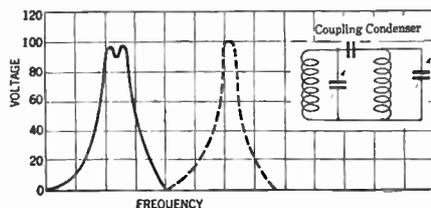
the combination has the form shown by the solid curve. The resonance curve of either separate circuit alone would have the form indicated by the dotted
