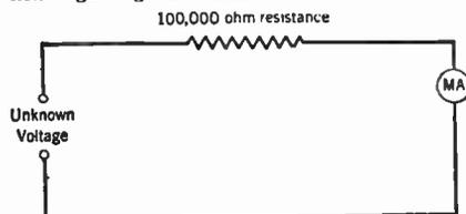
voltmeter, and if the calibration is done carefully, it should be possible to obtain readings which will be accurate within a few per cent. For rough measurements, no calibration is necessary since, if good fixed resistances capable of passing several milliamperes are purchased, their marked resistance value can be depended upon within about ten per cent., and usually the per centage error will be even less than this.
