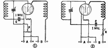
selectivity of the receiver. This is not true of the first method because, when the grid becomes positive, a load is placed on the tuned circuit, and the resistance of the circuit is thereby increased. The result is that it tunes broadly, or, in other words, the selectivity of the receiver is lowered.
