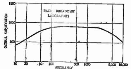
fication is increased. Large bypass condensers across the output of the power unit will frequently be necessary in order to prevent the occurrence of "motor-boating." The frequency characteristic of the complete amplifier is shown by the accompanying curve.
