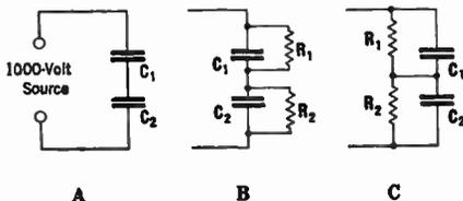
of the condensers. If we have two 500-volt condensers connected to a 1000-volt source, we might equalize the voltage across them by connecting two 100,000-ohm resistances in series across the source, as indicated at C. There would be 500 volts drop across each resistance and, therefore, 500 volts across each condenser, and the latter would then be satisfactory in operation and have normal life.
