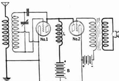
stations it is high frequency current flowing in the antenna that radiates energy in the form of electromagnetic waves (in this case, radio waves). Tube No. 1 is an oscillator in the diagram shown.
