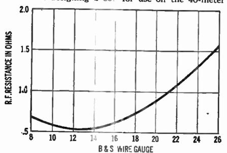
(7500-kc.) short-wave band (all these tests were made at this frequency), it is well to (1.) use about No. 12 to 14 wire; (2.) use a coil form if desired; (3.) use any good dope as a binder; (4.) use any reasonable amount of shielding where advantageous; (5.) keep the form factor (diameter divided by length) around 1 to 2.5.
