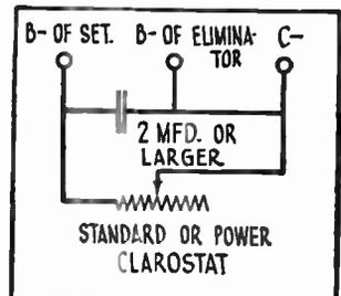
The tone quality of any set operating on a B-eliminator may generally be improved by adding capacity across the plus maximum and minus binding posts. Anywhere from 4 to 8 mfd. of additional capacity may be connected externally.
