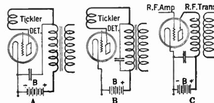
With the former method of connection, the radio frequency currents are returned, by the condenser, directly to the filament and do not need to pass through the B battery. The condenser used at this point should not be larger than is necessary to give good results. Usually a 0.00025-mfd. condenser is large enough, and a 0.001 one should not be used unless it is found necessary.
