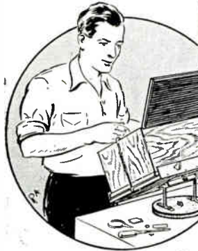
Adjustable radio set cradle shown above makes trouble-hunting easier, for set can be tilted or turned to any convenient position. Pad thumb-screws and metal side plate to prevent scratches on cabinet.
