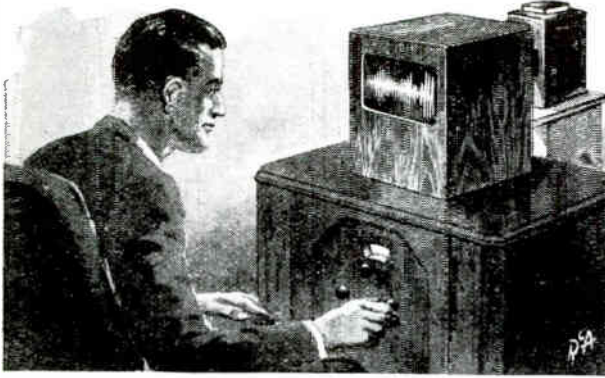
Music and voice from radio is produced in sound patterns on the screen of the "vibrometer," as shown in drawing above.
