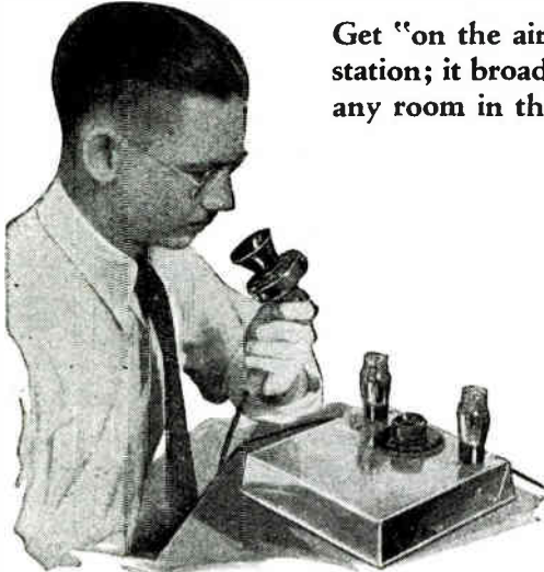
View of completed radio transmitter built into cake pan. Holes are cut in top of pan for tube sockets. Filament switch is in front of left tube. Use large condenser dial. Keep mouth ten in. from transmitter when broadcasting.
