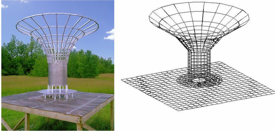
**Figure 10** The MF CFA in operational use at Tanta, Egypt (left); and a scale model fabricated for experimental measurements (right) along with the wire grid model created for numerical analysis.
