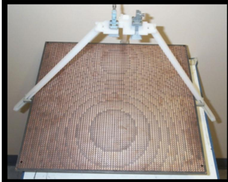
**Figure 7.** Dual-polarization bifocal reflectarray (20/30 GHz).
