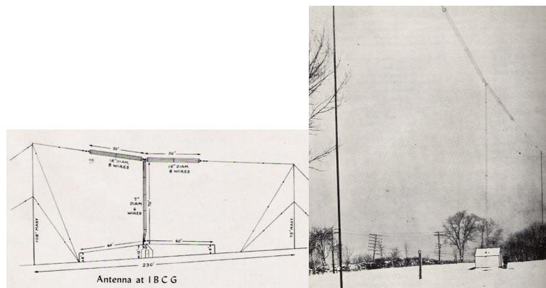
**Figure 4** Antenna system for amateur radio station IBCG, on the left
