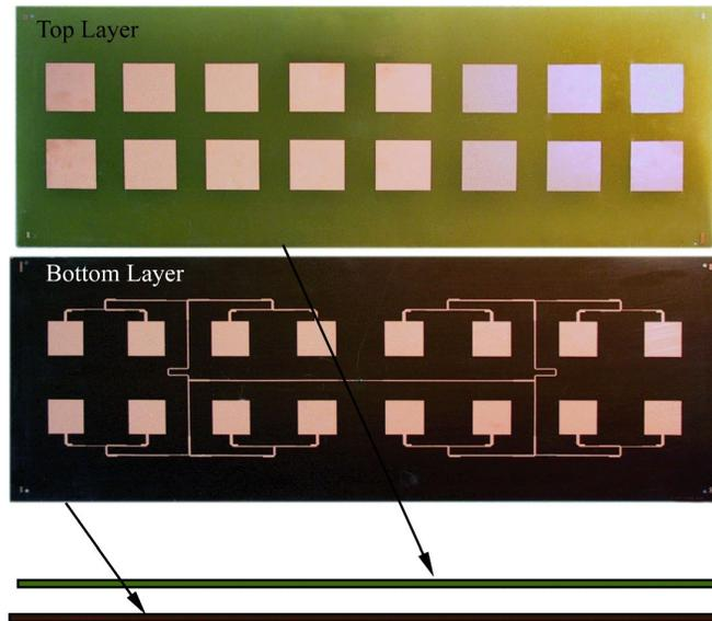
**Figure 4.** Stacked patch array for wideband terrestrial wireless applications (4.85-5.85 GHz).
