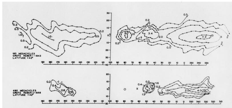
**Figure 16** Grote Reber surveyed the radio radiation from the sky and presented the data as contour maps showing the brightest areas in the Milky Way. The brightest part is toward the center of the Milky Way galaxy in the south. Other bright radio sources, such as Cygnus and Cassiopeia, were recognized for the first time (published in 1949).
