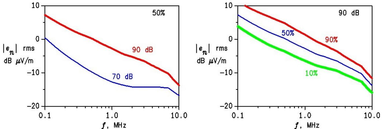
**Figure 6.** Variation of atmospheric-noise levels with frequency
