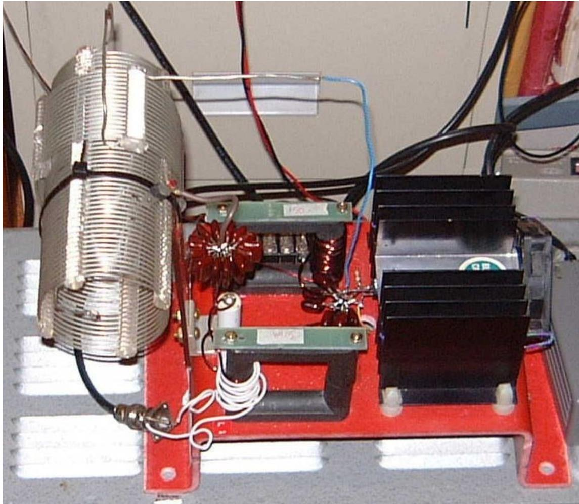
Figure 2 RF deck of the 137 kHz 125 watt transmitter
