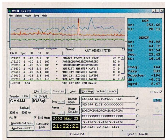
**Figure 11** Main screen of WSJT in JT44 mode displays K1JT's EME contact with GM4JJJ. The large box shows WSJT's attempts to decode GM4JJJ' signal in successive 30-second periods.
