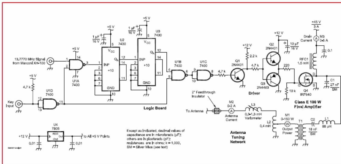
*Figure 3* 137 kHz transmitter schematic. From July 2005 QST, reprinted with permission. Copyright ARRL.
