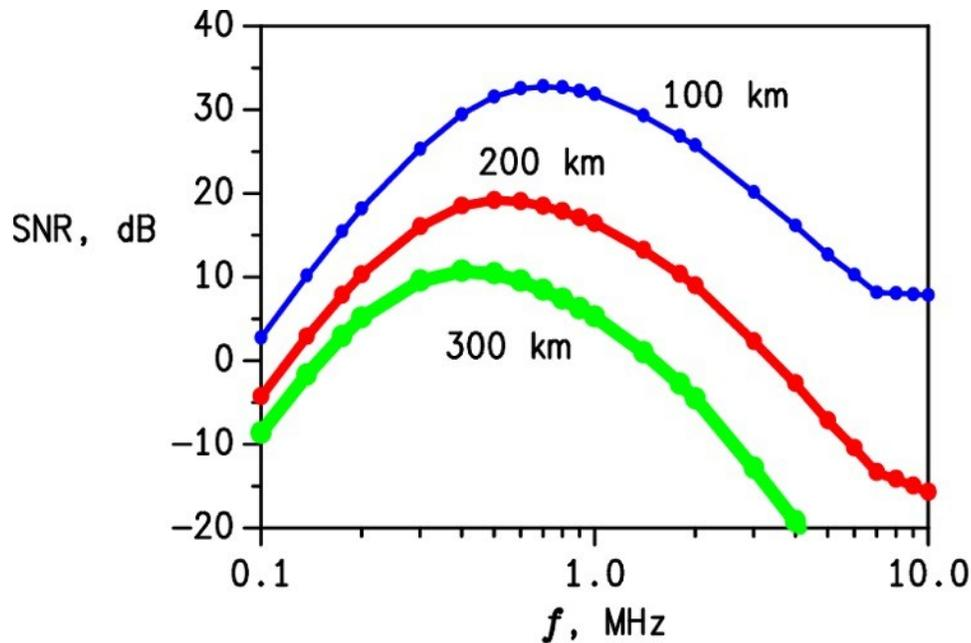
**Figure 8.** Ground-wave signal-to-noise ratio.
