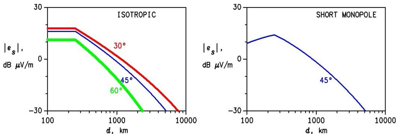
**Figure 9.** Median MF sky-wave signal strength.
