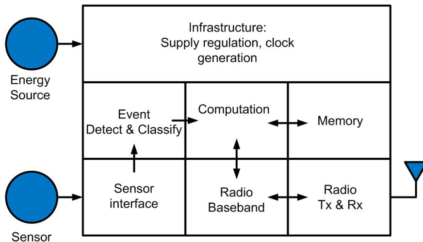
Figure 1. Block diagram of a basic sensor node architecture. The node is completely self-contained and modular, allowing a variety of sensor and energy source configurations.
