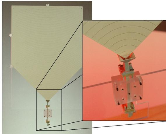
**Figure 9.** Horn-fed holographic-designed antenna.
