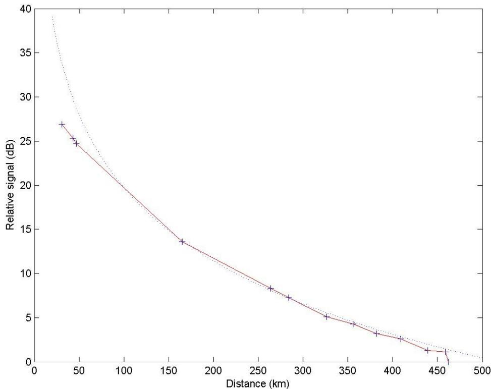
*Figure 8* Plot of signal strength vs. distance. The solid line is a plot of observed levels. The broken line is from Eqn. 10.
