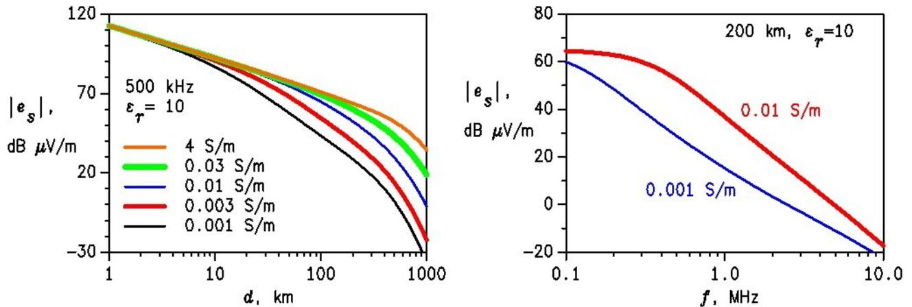
**Figure 7.** Amplitude of the ground-wave signal.
