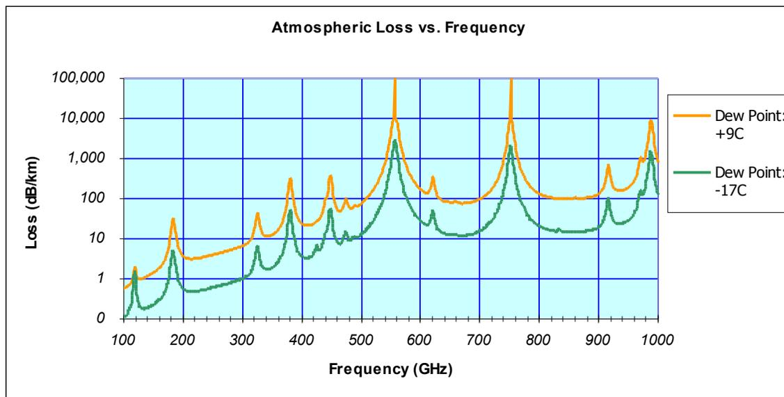
This graph shows the total atmospheric losses from both water vapor and oxygen as a function of operating frequency. When one locates the amateur millimeter wave bands on the graph (122, 134 & 241 GHz) it can be seen that there distinct advantages to operating at those frequencies due in-part to their distance from fixed molecular line resonances such as 119 and 183 GHz. This becomes even more of an issue when one considers operation in
