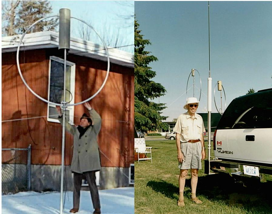
**Figure 5** Author Belrose experimenting with an AMA 1.7 m diameter loop, on the left, and, on the right, two compact loop antennas and a vehicular mounted HF whip antenna, a tunable all bands antenna (TABA), in use during a simulated emergency communications exercise.
