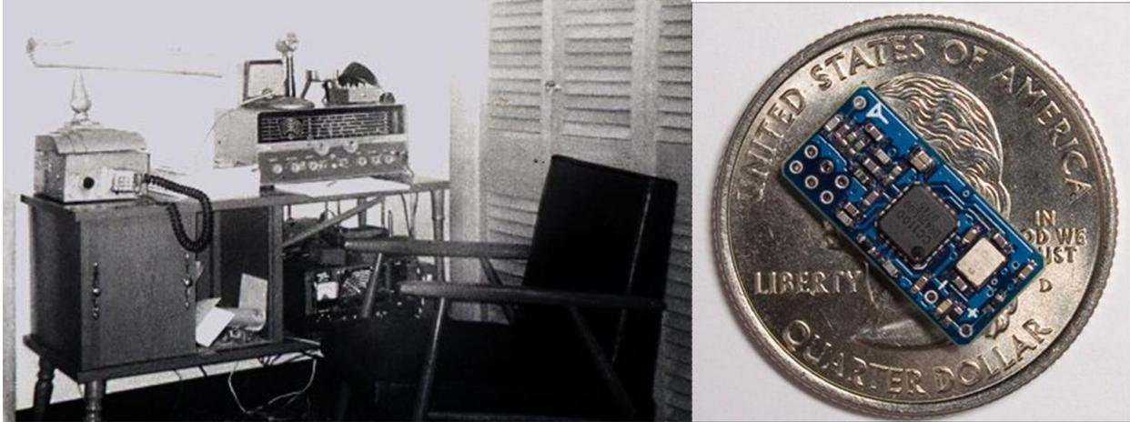
Figure 2. Left: vintage Ham radio transmitter/receiver setup. Right: a wireless sensing node comprising a 900MHz transceiver, low power microcontroller, and non-volatile memory.
