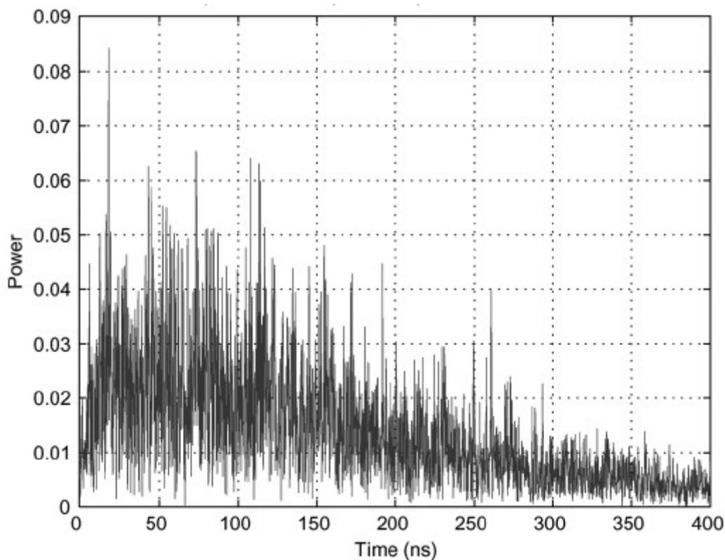
**Figure 1.** A channel impulse-response realization in the industrial NLOS environment [23].
