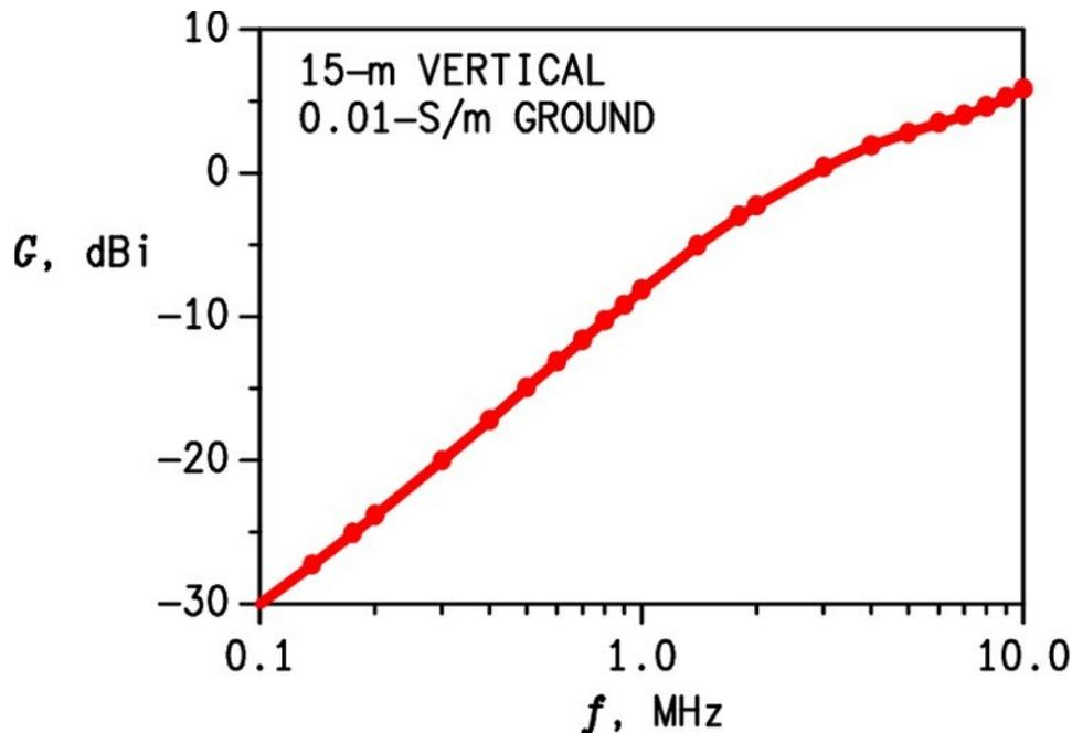
Figure 5. Low-angle/ground-wave gain of 15-m vertical antenna.
