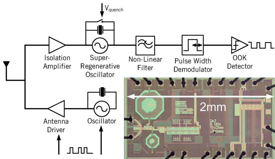
Figure 4. Integrated circuit implementation of a super-regenerative transceiver.
