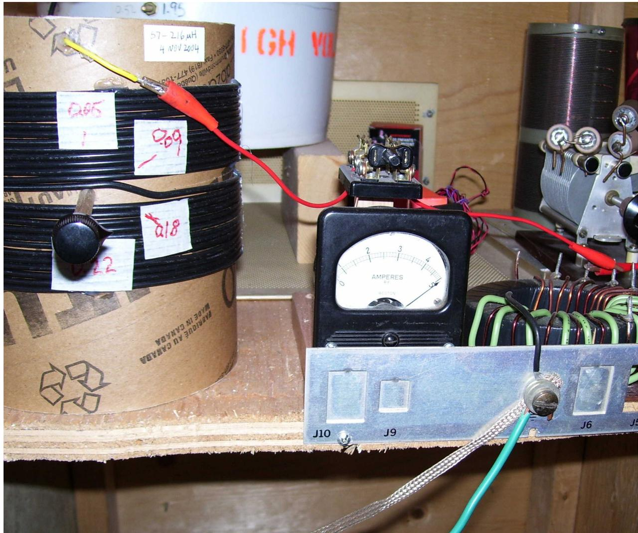
Figure 6 Aerial ammeter: just over 5 amperes to a 100 metre wire
