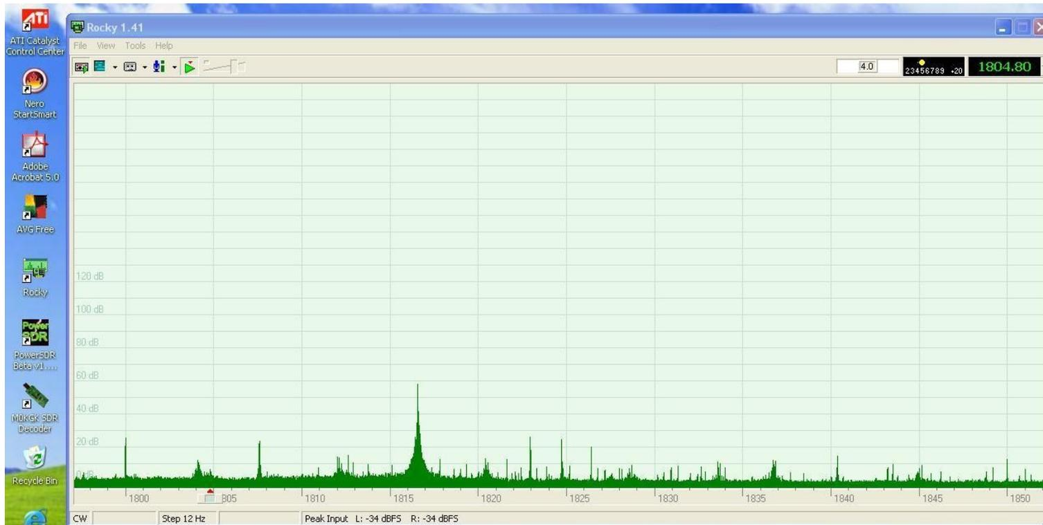
**Figure 1** An SDR-view of the 1.8MHz CW band, using the band scope in VE3NEA's *Rocky* application software and a SoftRock v6 receiver, viewed on the screen of VK6VZ's Pentium IV personal computer. The signals you can see were recorded around local sunrise during the CQ 160 CW contest on 21 January 2006. The x axis of the band scope shows the frequency in kHz, whilst the y axis shows the amplitude of the signal in dB.
