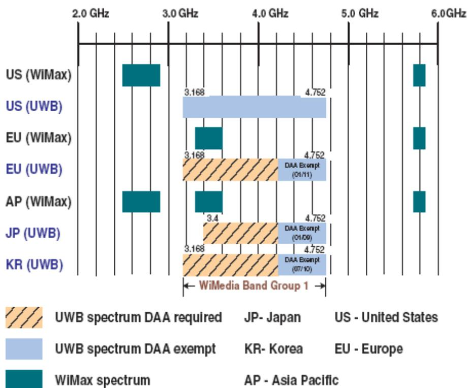
**Figure 2.** Overlapped frequency allocations of UWB and WiMax in various countries [54].
