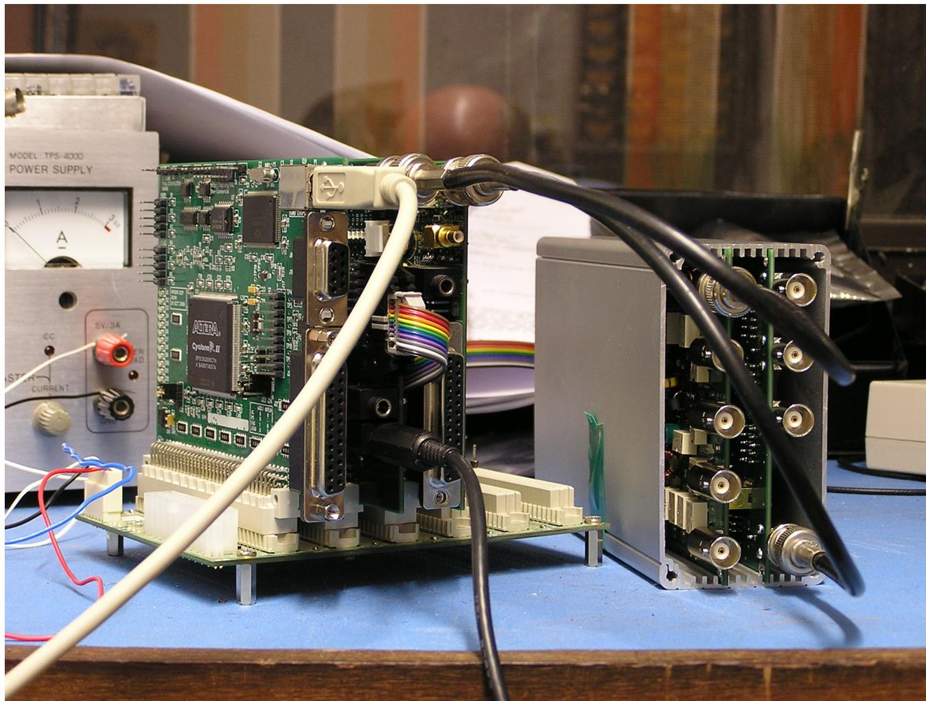
**Figure 5** Photo of VK6APH's prototype transceiver. On the left (from left to right) you can see the Ozy, Mercury and Pentelope boards. On the right are prototype ALEX receiver bandpass filter and transmitter low pass filter, boards mounted in case.
