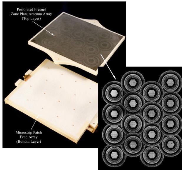
**Figure 12.** Array of perforated Fresnel zone plate antennas at 30 GHz.
