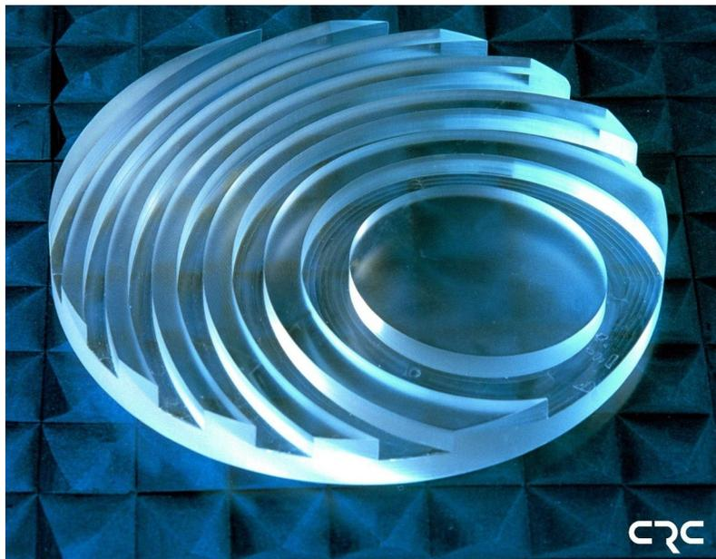
**Figure 11.** Phase correcting Fresnel zone plate antenna with offset beam, designed at 30 GHz.
