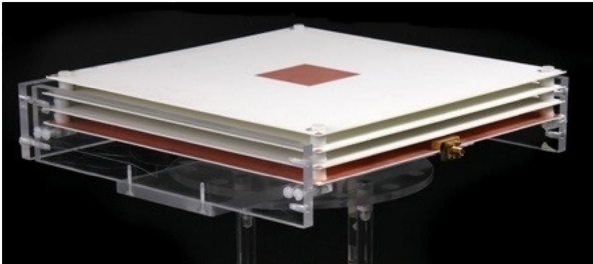
**Figure 5.** Stacked patch for wideband L-Band mobile satellite communications.
