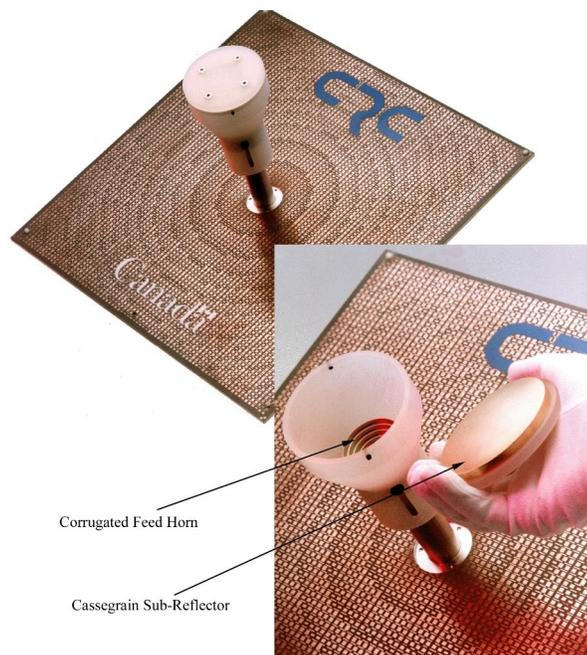
**Figure 6.** Dual-band (20/30 GHz) reflectarray with Cassegrain sub-reflector.
