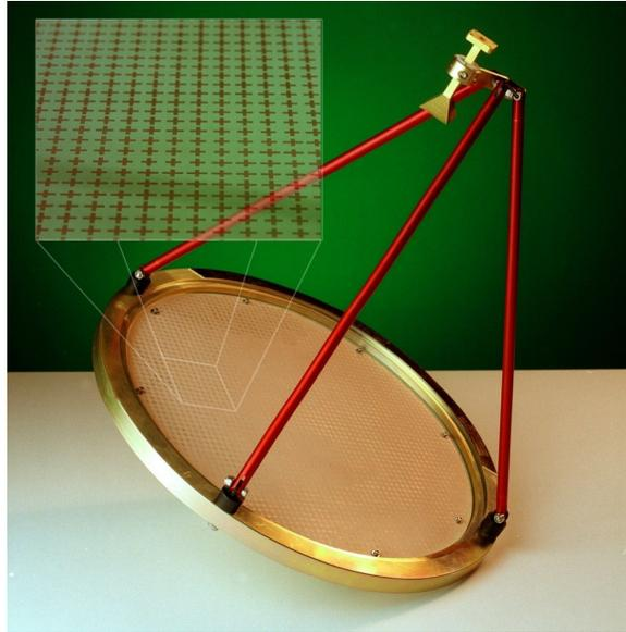
**Figure 8.** Circularly polarization reflectarray (20 GHz).
