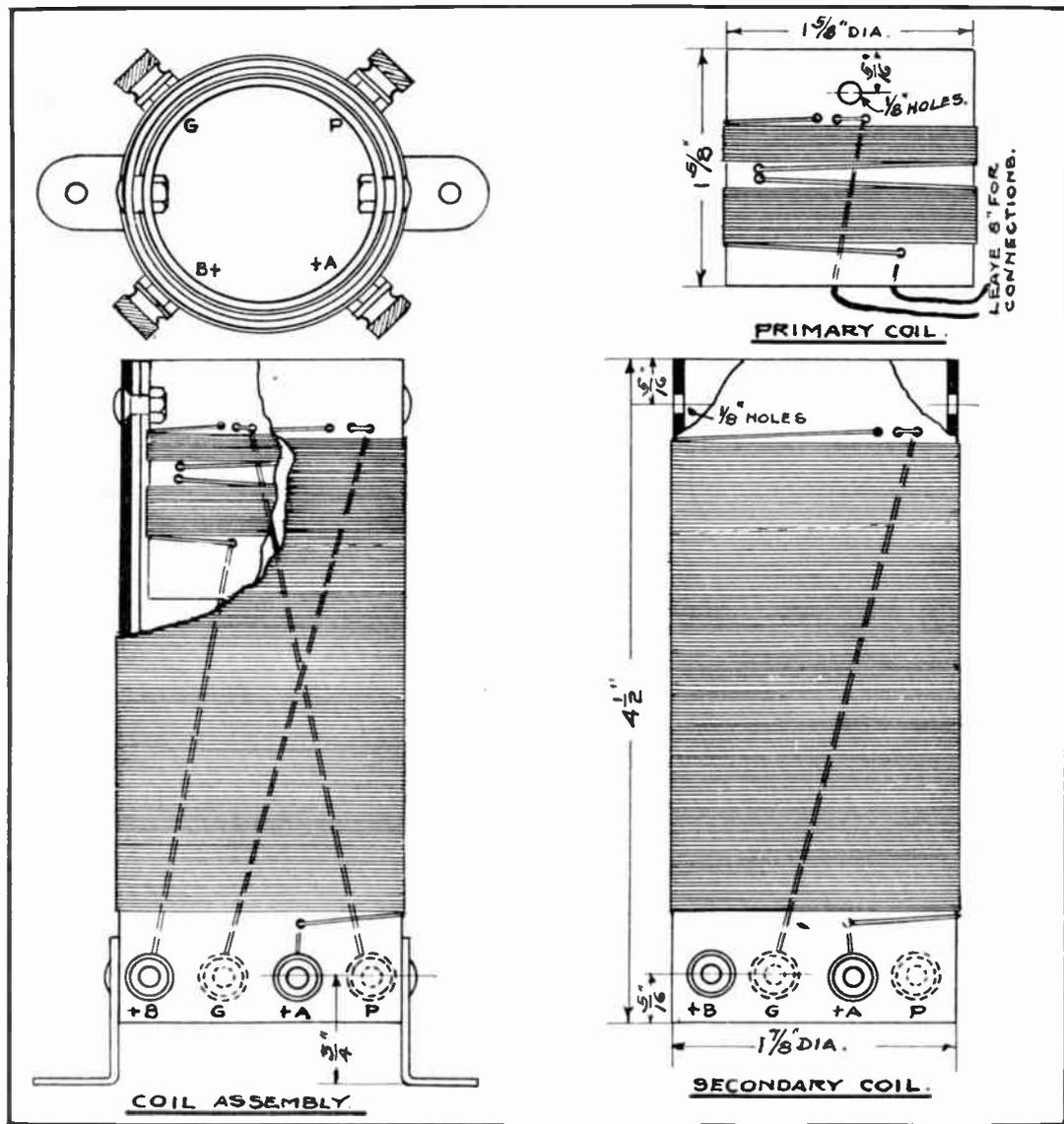
Fig. No. 27—Detailed Drawing Showing How to Construct Coil No. 2 for Duston Special
