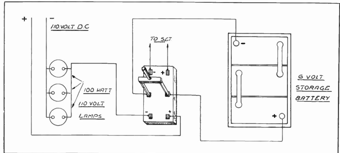
Fig. No. 7—Charging "A" Battery from Direct Current Line
