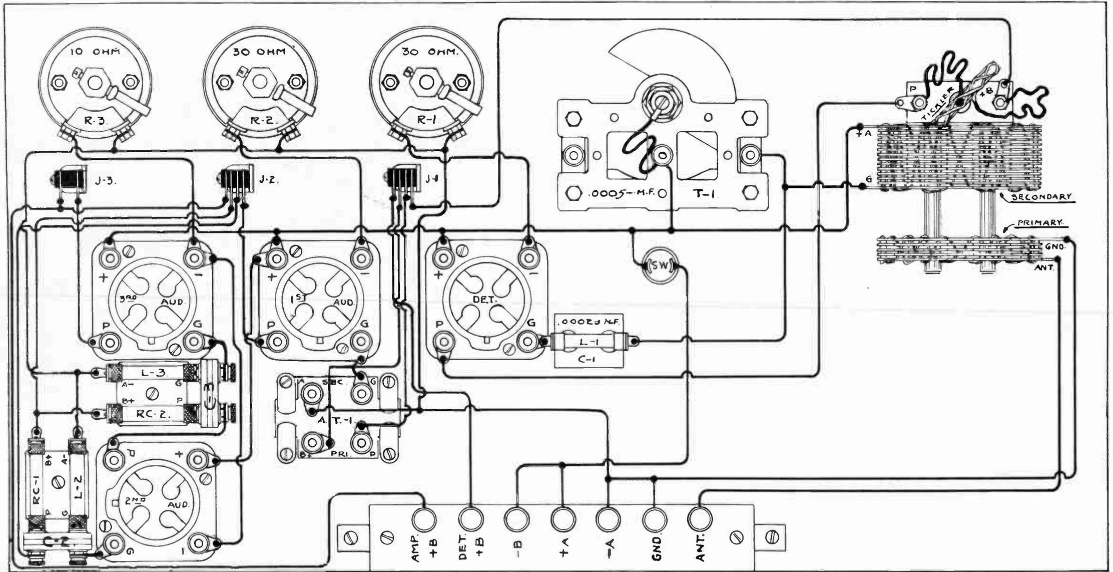
Fig. No. 18—Drawing of Four Bulb Three Circuit Set Using One Stage Transformer Coupled and Two Stages Resistance Coupled Amplification
