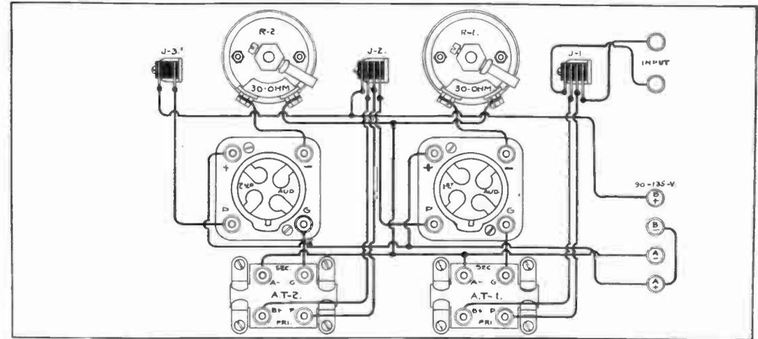
Fig. No. 16—Drawing of Two Stage Audio-Frequency Amplifying Unit
