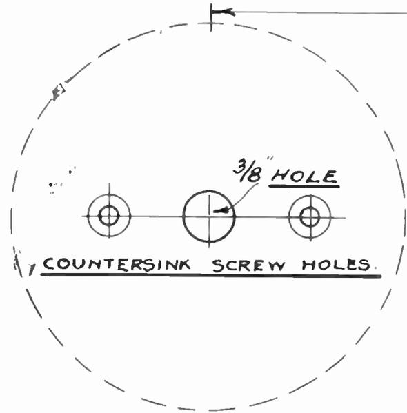
CHECK THESE HOLES WITH YOUR CONDENSER TEMPLATE BEFORE DRILLING. COUNTERSINK SCREW HOLES.
