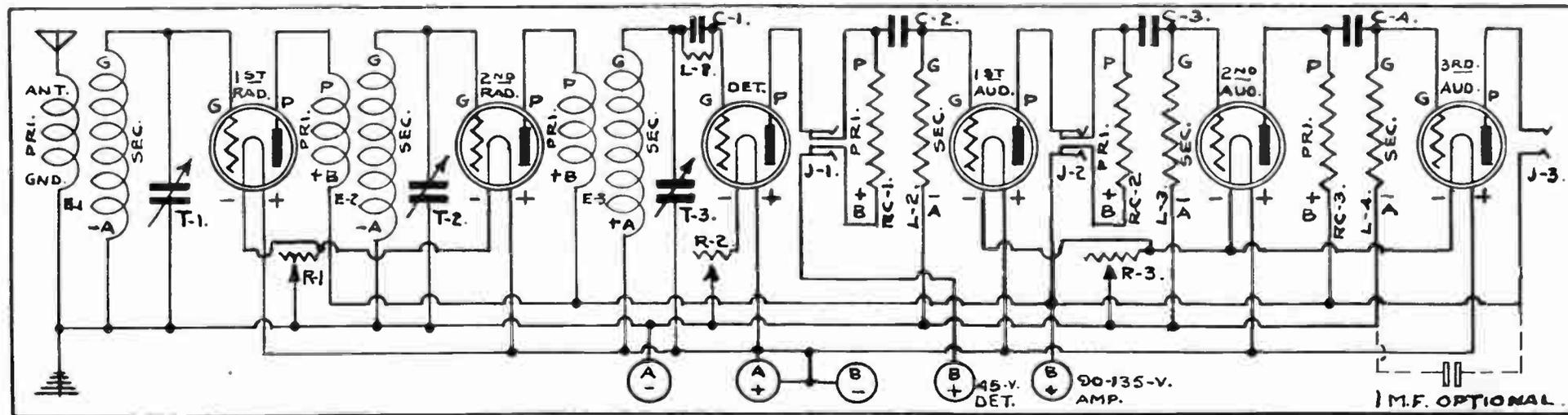
Fig. No. 22—Hook-up Showing Low Loss Set with Three Stages of Resistance Coupled Amplification
