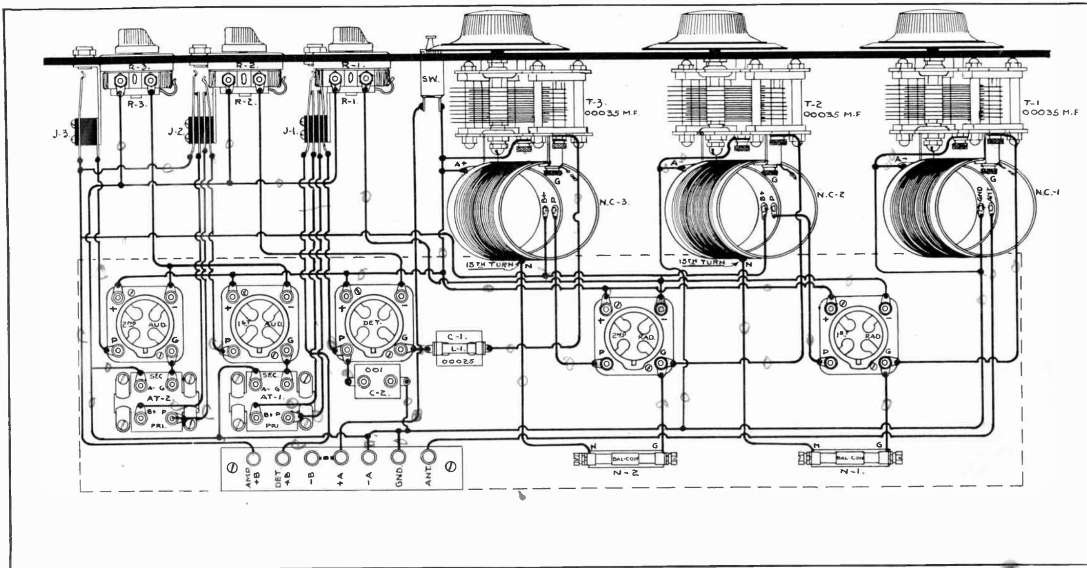
Fig. No. 23—Neutrodyne Type Using Two Audio-Frequency Transformers
