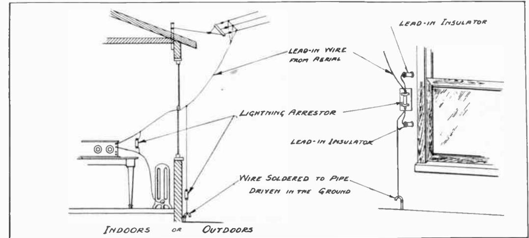
Fig. No. 1—Installation of Lightning Arrester
