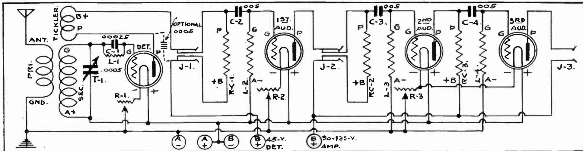
Fig. No. 19—Hook-up Three Circuit Set Using Three Stages Resistance Coupled Amplification
