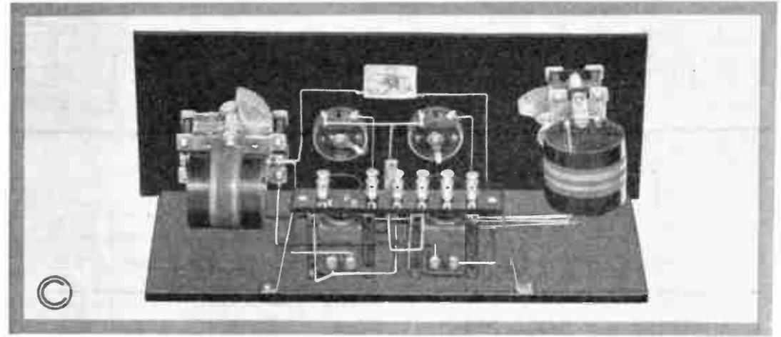
Plate No. 17—Rear View of Two Bulb Reflex
