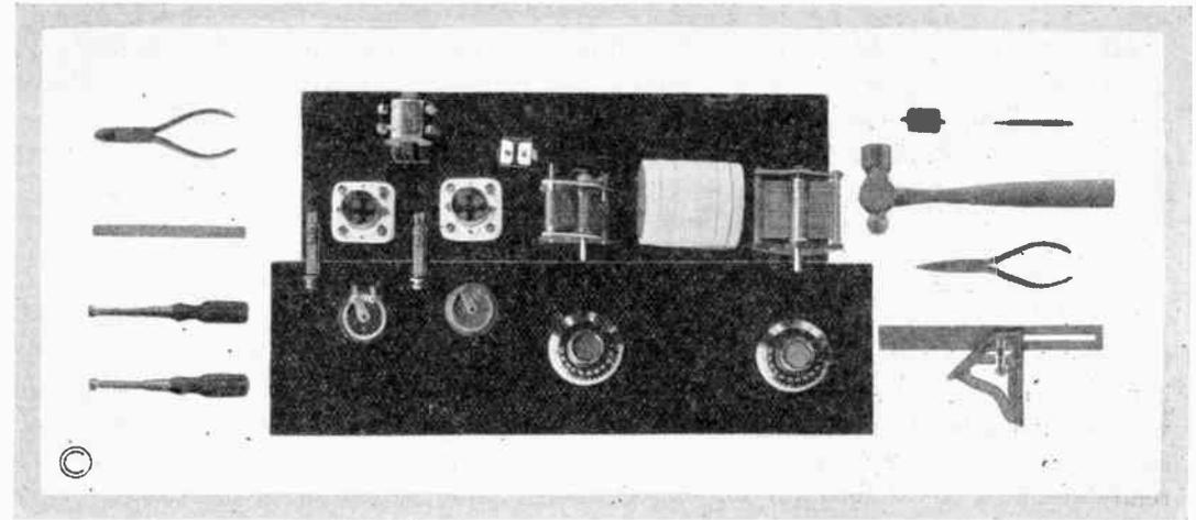
Plate No. 1—Laying Out Panel When Template Cannot Be Had
