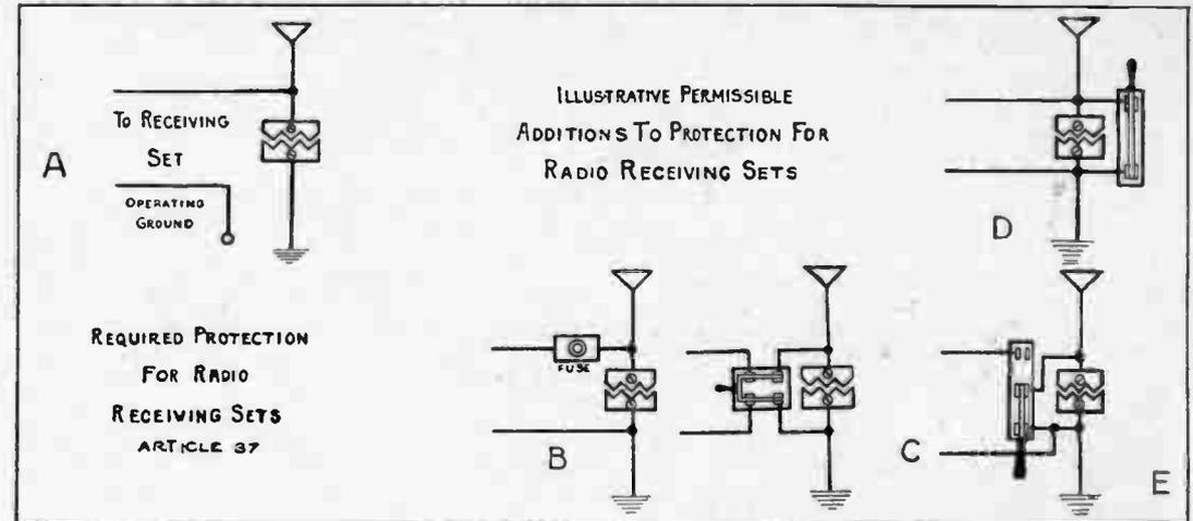
Fig. No. 5—Proper Ways to Install Lightning Arrestor
