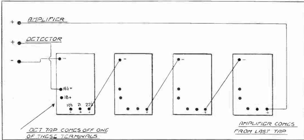
Fig. No. 11—Proper Way to Connect "B" Battery Blocks in Series
