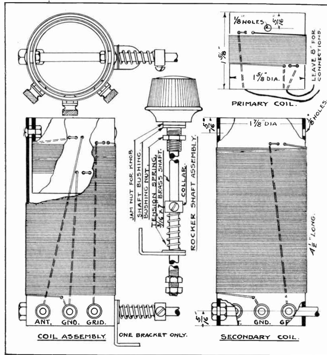
Fig. No. 28—Detailed Drawing of Coil No. 1 for Duston Special
