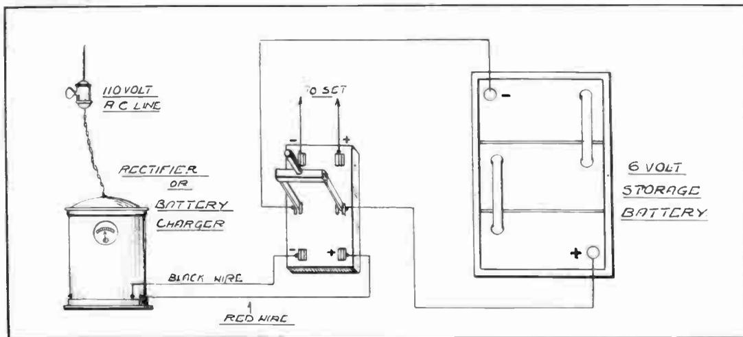
Fig. No. 8—Charging "A" Battery from Alternating Current Line
