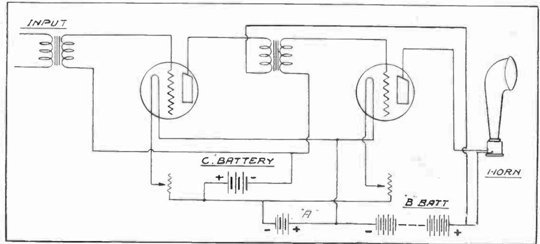
Fig. No. 12—Proper Way to Connect "C" Battery in Amplifier Circuit
