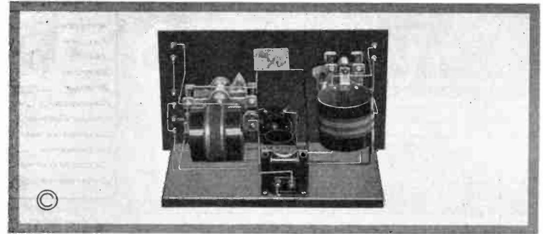
Plate No. 20—Rear View of One Bulb Reflex Set
