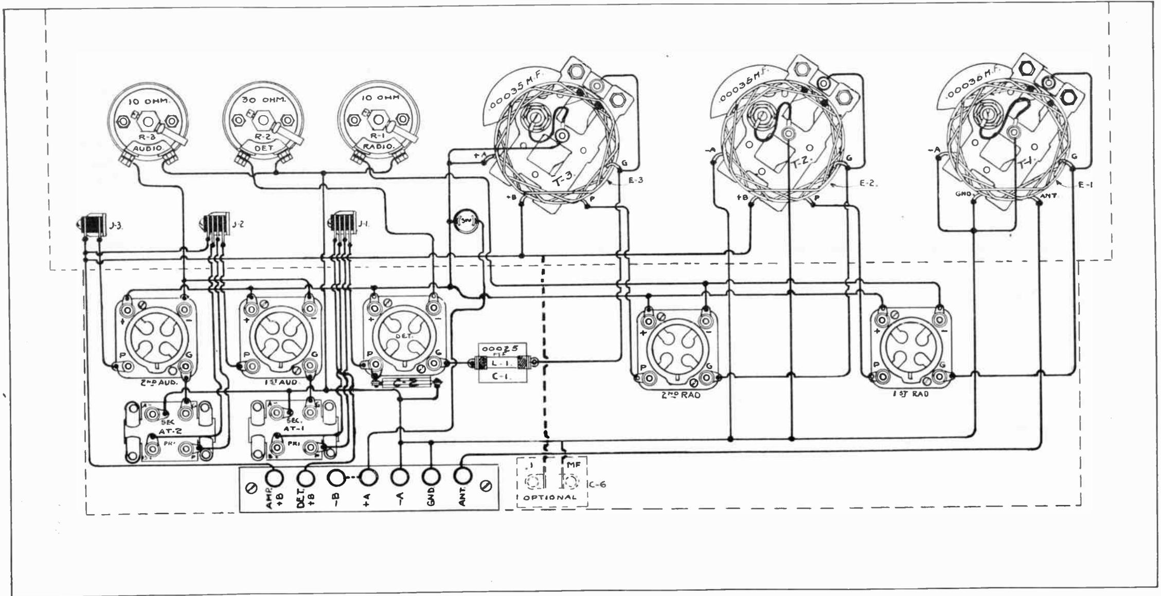
Fig. No. 20—Drawing of Low Loss Radio Frequency Set Using Transformer Coupled Amplification
