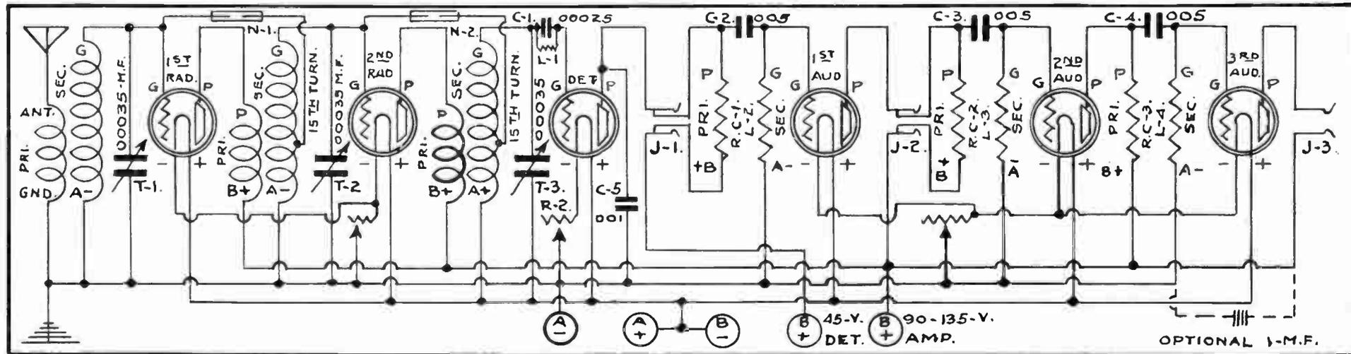
Fig. No. 25—Hook-up Showing Three Stages Resistance Coupled
