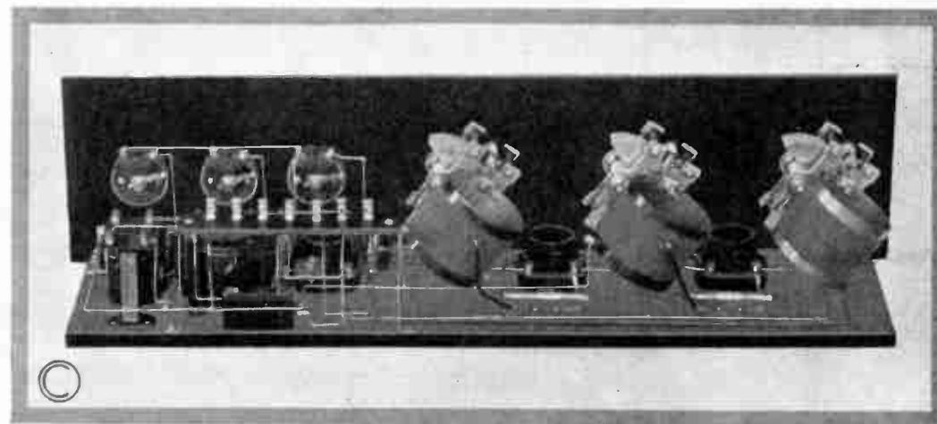
Plate No. 14—Rear View of Neutrodyne Type Receiver—Front View Is the Same as Shown in Plate No. 12
