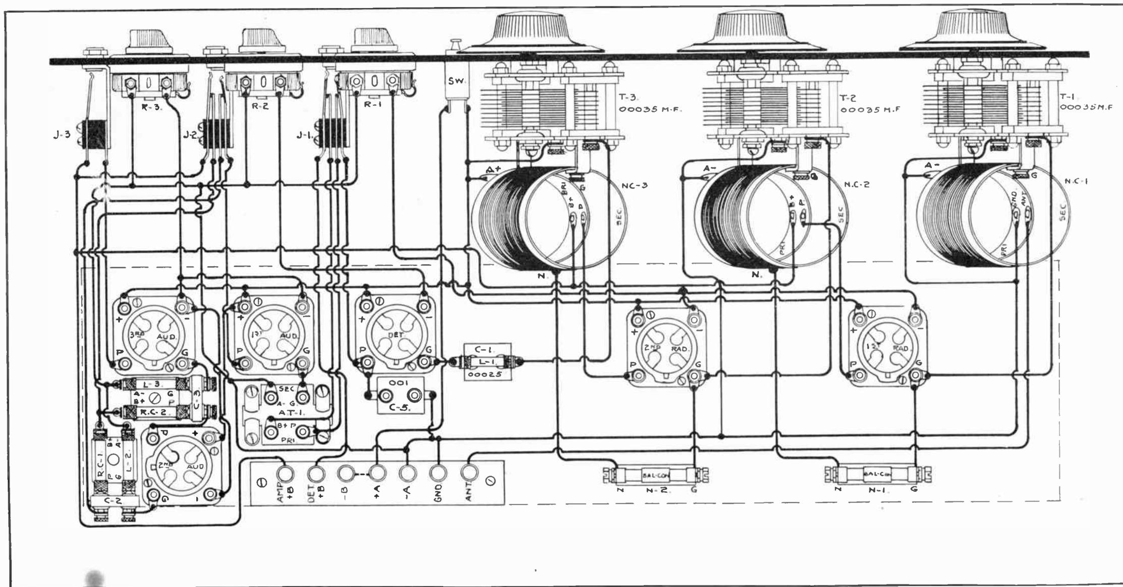
Fig. No. 24—Neutrodyne Type Receiver Using One Stage Transformer Coupled and Two Stages Resistance Coupled A. F. Amplification
