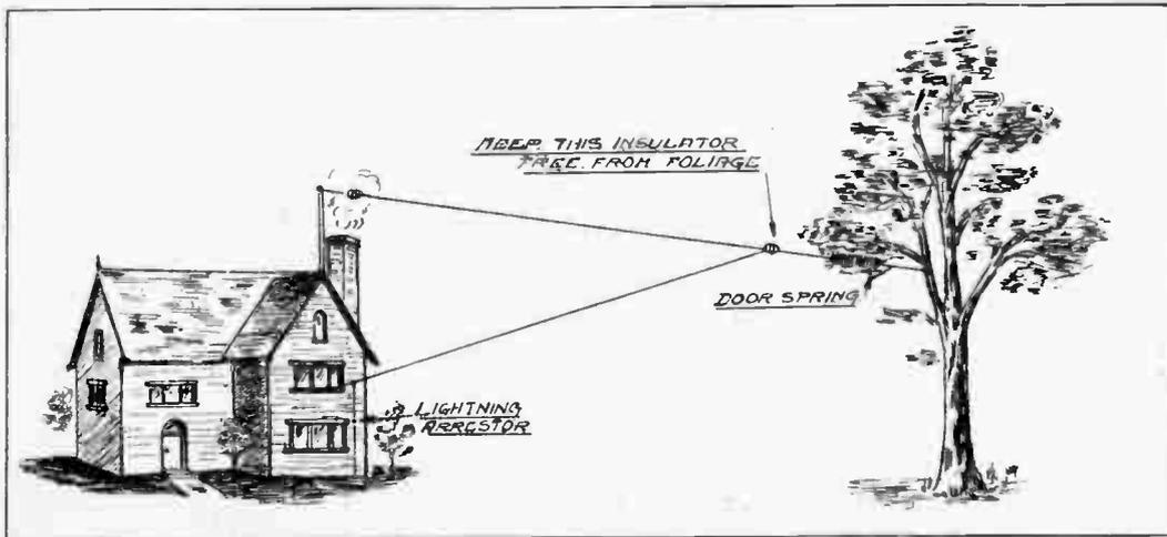
Fig. No. 4—Single Wire "V" Type Antenna
