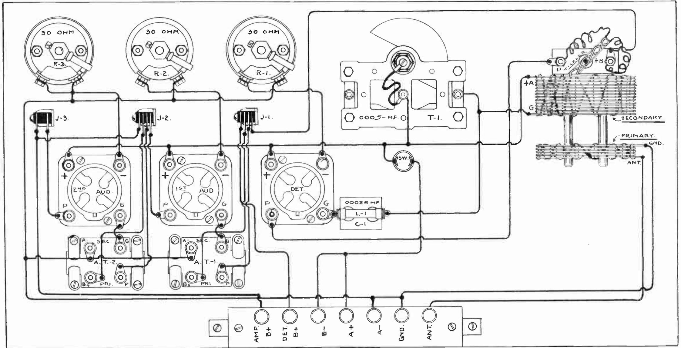
No. 17—Drawing of Three Bulb, Three Circuit Set—Transformer Coupled
