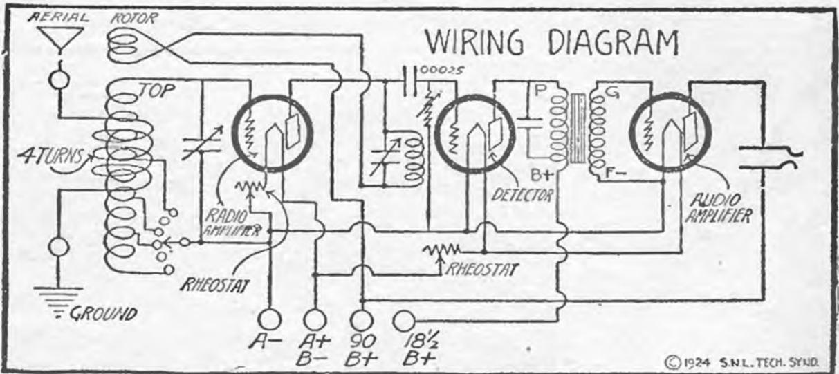
The Superdyne receiver shown above is an entirely new and efficient circuit using a stage of radio, detector, and a stage of audio frequency. It may be constructed with two stages of audio frequency if you desire.
