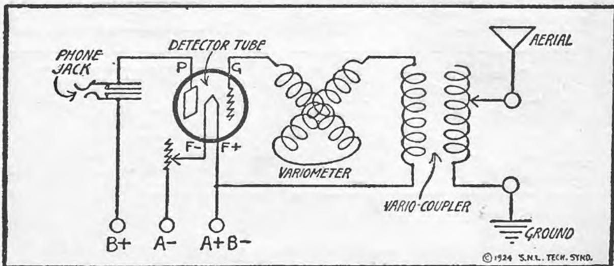
This is a circuit showing how the same apparatus can be used to change your crystal set into a vacuum tube receiver. This is possible without changing any of the apparatus on the front panel, or moving any of the instruments.
