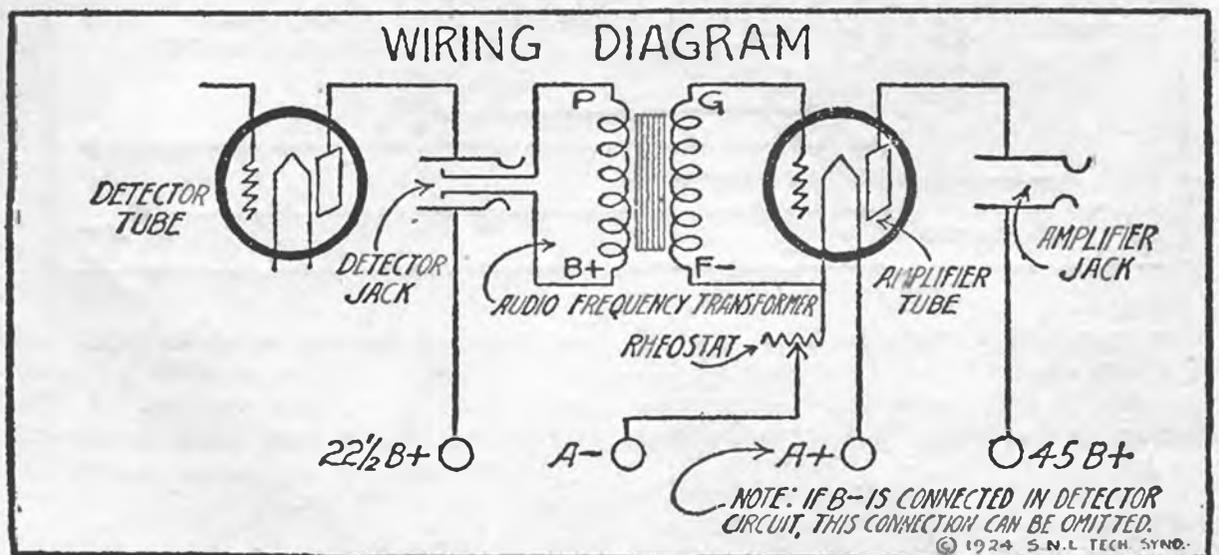
After you have constructed any of the one tube circuits shown on preceding pages, and you wish to add apparatus that will increase the volume of your receiver, the logical step to take is to add a stage of audio frequency amplification.
