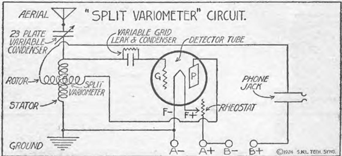
This is a very compact and easily constructed receiver made with a variometer. The circuit derives its name from the fact that the variometer is divided into two windings, similar to the winding of a variocoupler.
