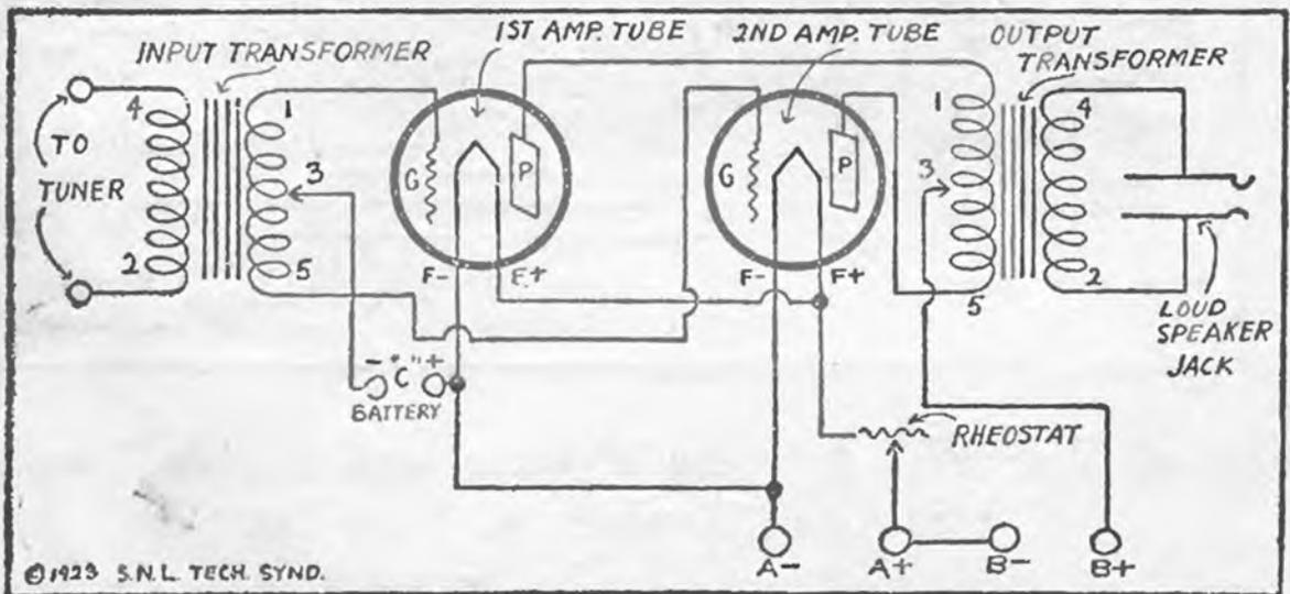
This is an amplifier for use in conjunction with any type of receiving set. It can be attached to a regular detector and two-stage receiver for the purpose of amplifying the signals for loud speaker reception without adding distortion to the output.
