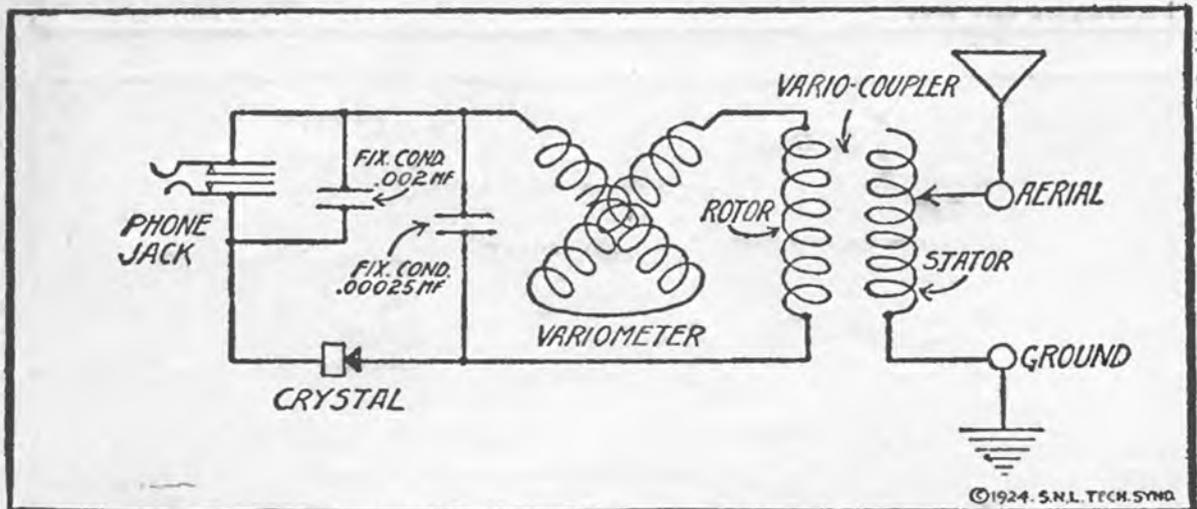
This is a crystal receiver constructed with a variometer and a variocoupler. This receiver is more selective than the crystal circuit shown on the preceding page, due to the fact that a two circuit method of tuning is used.
