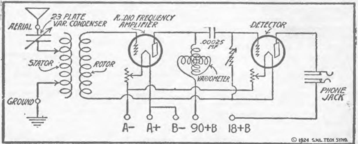
This is a circuit somewhat similar to the Tuned Impedance receiver shown on the opposite page. In place of the honeycomb coil and condenser a variometer is used to tune the circuit between the radio frequency tube and the detector.
