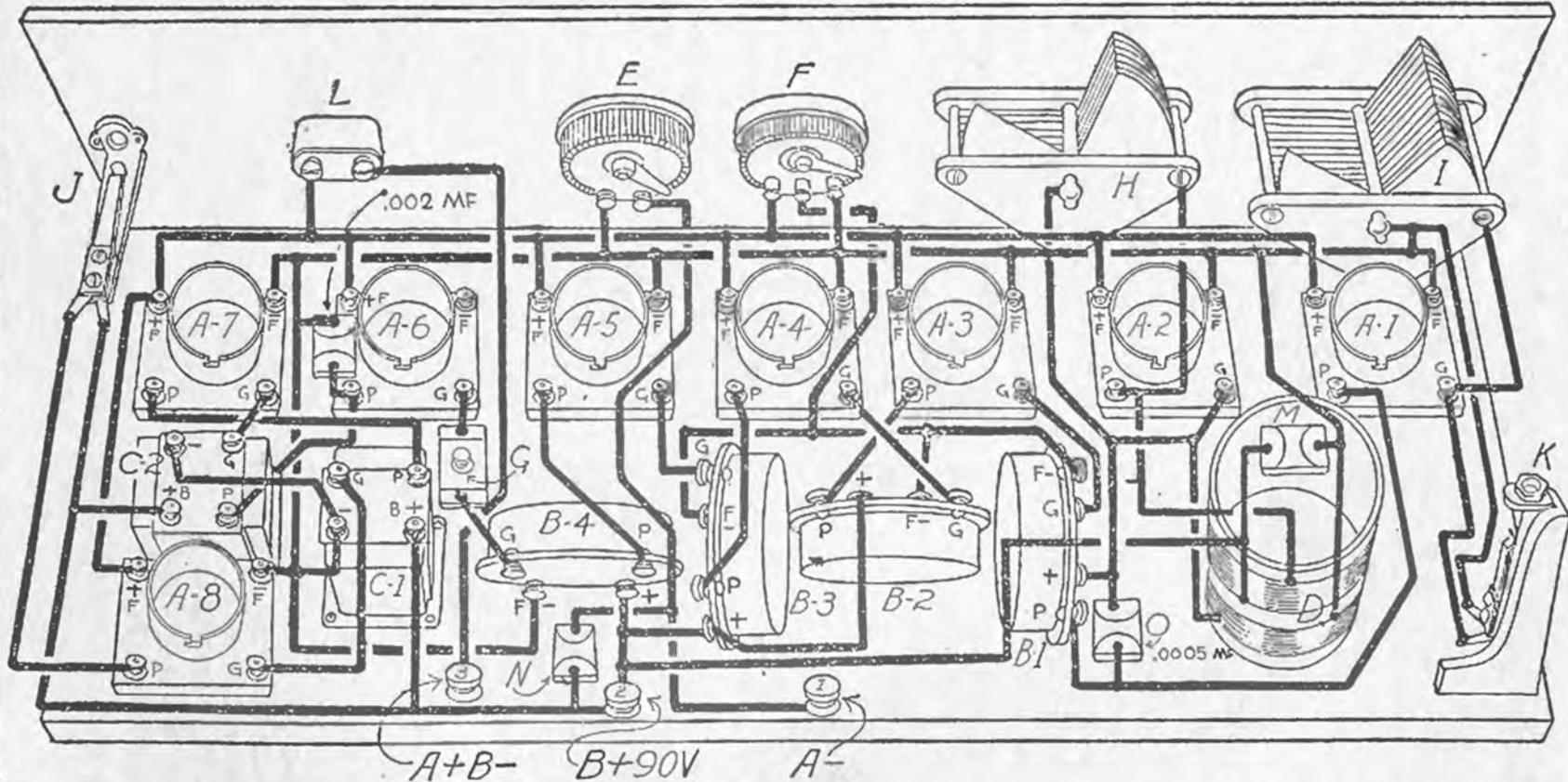
A-1-2-3-4-5-6-7-8 TUBE SOCKETS — E-6 OHM RHEOSTAT — H-VAR. CONDENSER.0005 MF. — L-FILAMENT SWITCH
