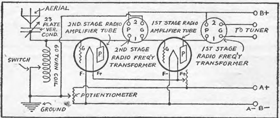
tube can be changed. The wiring diagram shows the connections direct on the transformers for those who prefer to use transformers of other design.
