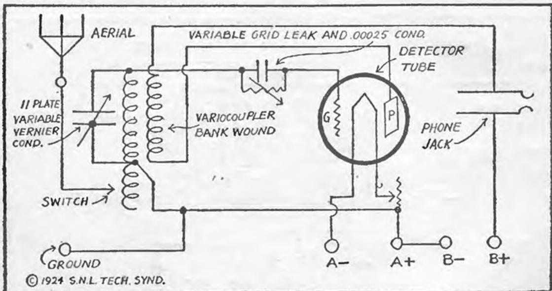
The Haynes receiver is an easily constructed set with a number of likable qualities. One of them being that it is very easy to tune and at the same time being one of the most selective of single circuit broadcasting receivers.
