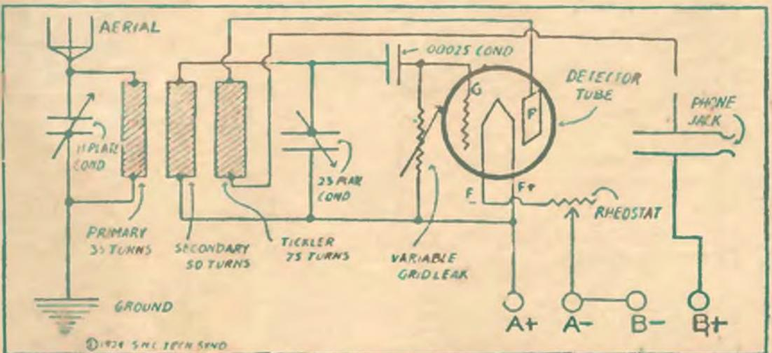
This shows a method of constructing the three circuit regenerative hookup by means of honeycomb coils.
