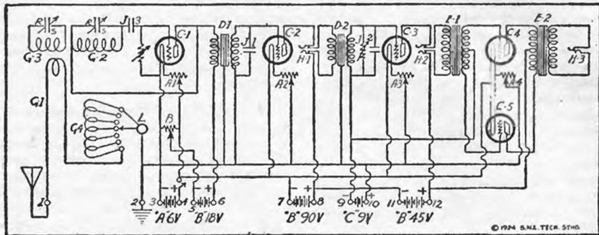
The single tube four circuit tuner can be converted into the five tube set shown on the opposite page by the addition of two stages of audio frequency and a push pull amplifier. The tuning unit remains the same.
