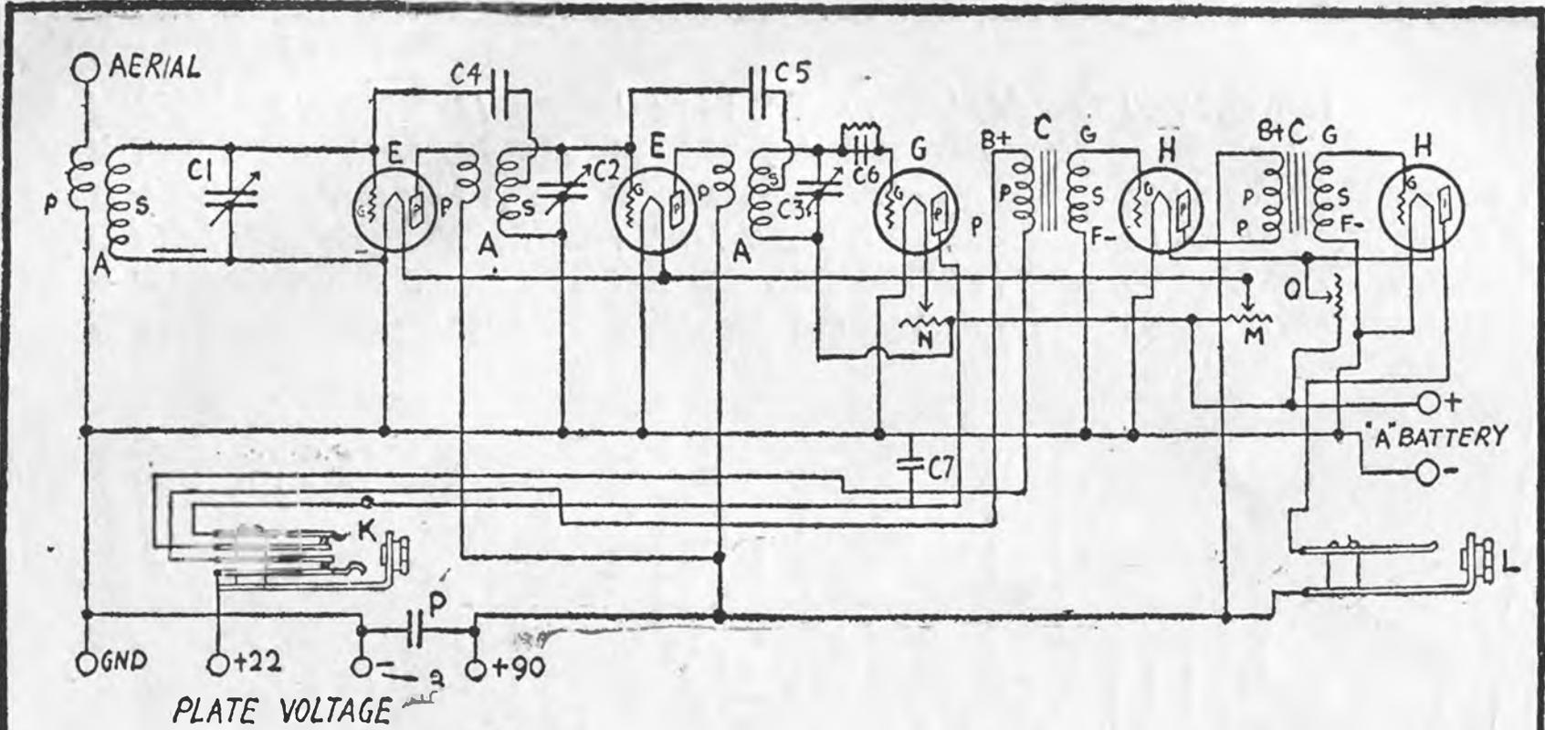
**5 TUBE NEUTRODYNE WITH CONSTANTS CONNECTIONS**
