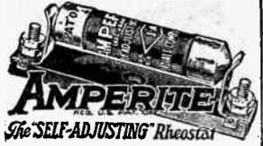
Amperite operates on the thermo-electric principle. This filament has the unique property of changing in resistance automatically as the "A" battery voltage changes. Furnished only complete with mounting.
