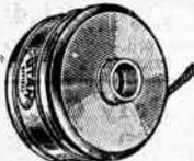
The new Utah Units have the diaphragm connected to the armature through a tripod arrangement. This allows more freedom for the movement of the diaphragm, and decreases necessary movement of the armature for any given vibration. The advantage of this exclusive patented design enables them to stand extreme power without blasting.
