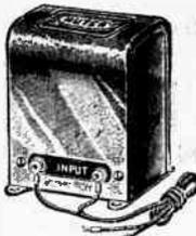
A specially designed dual choke coil and large capacity filter condenser. Enclosed in highly finished enameled metal container. Easily attached. Improves tone, quality and volume by protecting speaker coils from high E voltage and preventing paralysis of speaker unit. Size, 4 in. high, 3 1/4 in. long, 2 1/4 in. wide.
