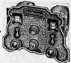
Handsomely engraved escutcheon finished in bronze. 2 control holes in addition to dial controls. Off position shown alongside one hole so filament switch may be mounted behind rheostat, giving equivalent of 3 auxiliary controls. Escutcheon mounts on steel or wood panel. New drum type dials with smooth running drive. Light behind black figures shows through white celluloid.
