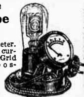
Contains Milliammeter. Tests quickly plate current of all tubes. Grid switch connects to positive and negative filament. Difference in readings shows condition of tube on simple reference table on bottom of tester. Dependable and accurate.
