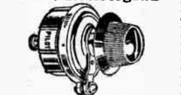
Continuously variable resistance from practically zero to 30 megohms. Resistance material is hermetically sealed in a case molded of special high temperature bakelite material. Widely used as a regeneration control, voltage regulator, volume control and variable grid leak.
