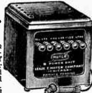
Fixed controls with six taps for all voltage requirements of sets with ten regular tubes or seven and power tube. Model 3000 rates at 40 mills. at 150 volts. Model 3050 delivers 50 mills. at 150 volts and gives 180 volts for power tube. Size, 6 1/2 in. wide, 7 in. high, 8 1/2 in. long. Highly finished enameled metal case with Bakelite front panel. Shipping weight, 15 lbs.
