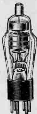
Type 58 Triple Grid Superphonic tube. Heater 2.5 volts at 1 ampere either A.C. or D.C.
