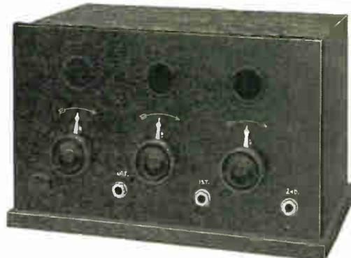
**Detector and Two-Stage Amplifier Unit.**
