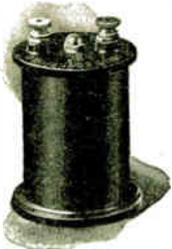
Can be used with great success in the receiving circuit. A high grade fixed condenser. The base and top are made of hard rubber composition and are mounted on a nickel plated tube. Capacity is .003 M.F.D. Shipping weight, 10 ounces.
