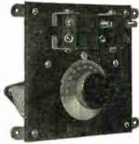
**Three-Coil Mounting and Variable Condenser Unit.**
