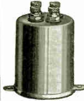
This transformer is designed for use in radio frequency circuits. The transformer is mounted in a highly nickel plated brass case, so constructed that it may be mounted in any standard tube socket. This transformer has given satisfactory results using as high as four stages of amplification. Efficient on wave lengths from 150 to 550 meters. Shipping weight, 1 pound.
