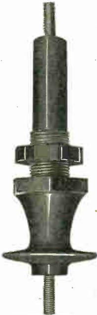
Rain test, 25,000 volts; dry test, 55,000 volts. Length of insulator, 10 inches; length over all, 13 inches; length below shoulder, 6 inches; diameter of top, 4 inches; diameter of shoulder, 3 inches;  $\frac{5}{8}$ -inch locking ring. Diameter threaded section,  $1\frac{3}{4}$  inches, slight taper to bottom;  $\frac{1}{2}$ -inch solid brass rod. Shipping weight, 5 pounds.
