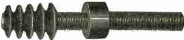
Polished black finish. Rain test, 20,000 volts; dry test, 40,000 volts. Length over all,  $9\frac{1}{16}$  inches; length threaded section,  $6\frac{1}{2}$  inches; 1-inch locknut; diameter threaded section, 1 inch; diameter of shoulder, 2 inches; tapering hole through insulator,  $\frac{1}{4}$  inch outside end,  $\frac{5}{16}$  inch inside end. Shipping weight, 4 pounds.
