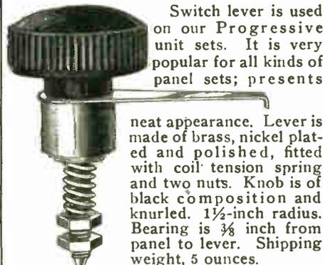
Switch lever is used on our Progressive unit sets. It is very popular for all kinds of panel sets; presents neat appearance. Lever is made of brass, nickel plated and polished, fitted with coil tension spring and two nuts. Knob is of black composition and knurled. 1½-inch radius. Bearing is 3/8 inch from panel to lever. Shipping weight, 5 ounces.
