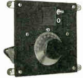
**Single Coil Mounting and Variable Condenser Unit.**
