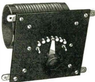
This unit is of special interest to jewelers and all stations especially interested in receiving time signals, weather reports, etc. Unit consists of a tapped coil, wound with high frequency cable or Litzendraht on formica tube. Inductance is varied by means of seven-point switch on front of panel. This unit, together with Crystal Detector or Vacuum Tube Unit and Variable Condenser Unit, makes an excellent receiving set. Shipping weight, 4 pounds.
