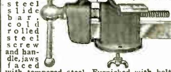
Has solid steel slide bar, cold rolled steel screw and handle, jaws faced with tempered steel. Furnished with bolts for fastening to bench. Width Jaws, In. Opens, In. Shpg. Wt., Lbs. 99A5195 2 1/2 2 1/2 13 \$2.90 99A5196 3 3 1/2 15 3.60 99A5197 3 3/4 4 17 4.30 99A5198 4 6 29 5.20
