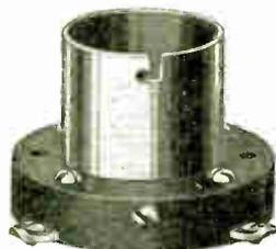
A very high grade tube socket fitted with positive contact springs and is unusually substantial and attractive. Base is of molded Bakelite, and the tube and terminal screws are of brass with polished nickel finish. This socket is adapted to any of the standard four-prong tubes. Transmitting tubes can be used by simply changing two screws. Shipping weight, 8 ounces.
