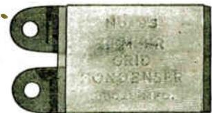
The conductors are stamped from copper sheet and insulated with paraffin paper. The entire unit is encased and impregnated and the terminals are spaced so as to mount on the back of the panel directly on the **6A9659** Grid Leak. Capacity is .00025 M.F.D., the correct value for the type C-300 Gas Content Detector. Shipping weight, 1 ounce.
