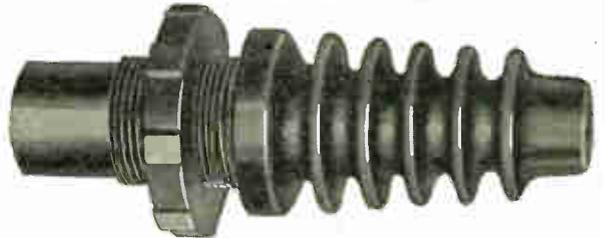
Rain test, 35,000 volts; dry test, 60,000 volts. Length over all,  $9\frac{3}{8}$  inches; length outside end,  $5\frac{1}{2}$  inches; inside end,  $3\frac{7}{8}$  in.;  $\frac{5}{8}$ -inch locknut; diameter at shoulder,  $3\frac{1}{16}$  inches; diameter threaded section,  $2\frac{1}{2}$  inches; tapering hole,  $\frac{3}{4}$  inch inside end,  $1\frac{1}{16}$  inch outside end. Shipping weight, 5 pounds.
