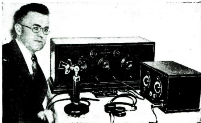
The author with his transmitter constructed from an old neutrodyne receiver.
