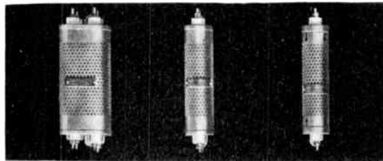
Fig. 106. Small Resistors for Mounting on Back of Switchboard Panel
