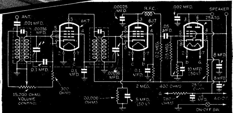
**D**ESIGNED specially for use in a kitchen or kitchenette, this compact three-tube broadcast receiver is built to match the conventional canisters used by housewives to store flour, sugar, and other dry groceries. Operating on either alternating or direct current, the set can be plugged into any house-wiring outlet and requires only a short antenna and no ground.
