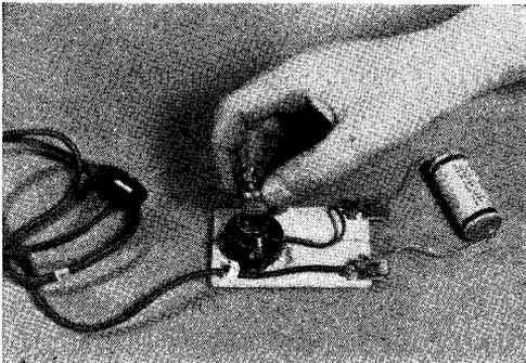
INTERMITTENT AND FADING RECEPTION on some AC-DC receivers and phone combinations is caused by faulty construction of new single-ended tubes, without grid caps. To test for this trouble, tap all tubes with a wooden screwdriver handle, as shown below, and the defective one will induce static. It should be replaced.
