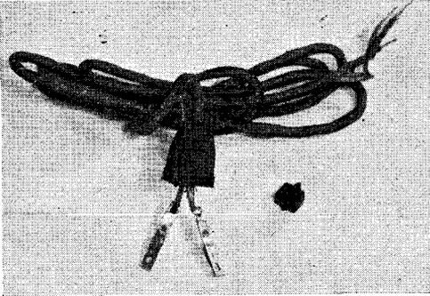
Yanking on a line cord often causes a break in the resistor wire. To avoid this, grasp the plug when removing it
