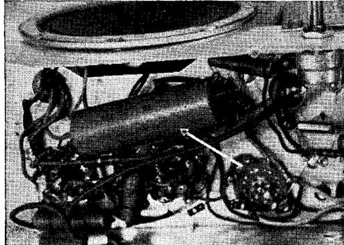
**NOISY TUNING IN THE LATEST RADIOS** may be caused by filings between plates of the oscillator tuning condenser. These may be burned out by connecting the secondary of a 700-volt power transformer across the condenser, as shown above and in the diagram. Be sure to disconnect the house current and the grid connection to the oscillator unit.
