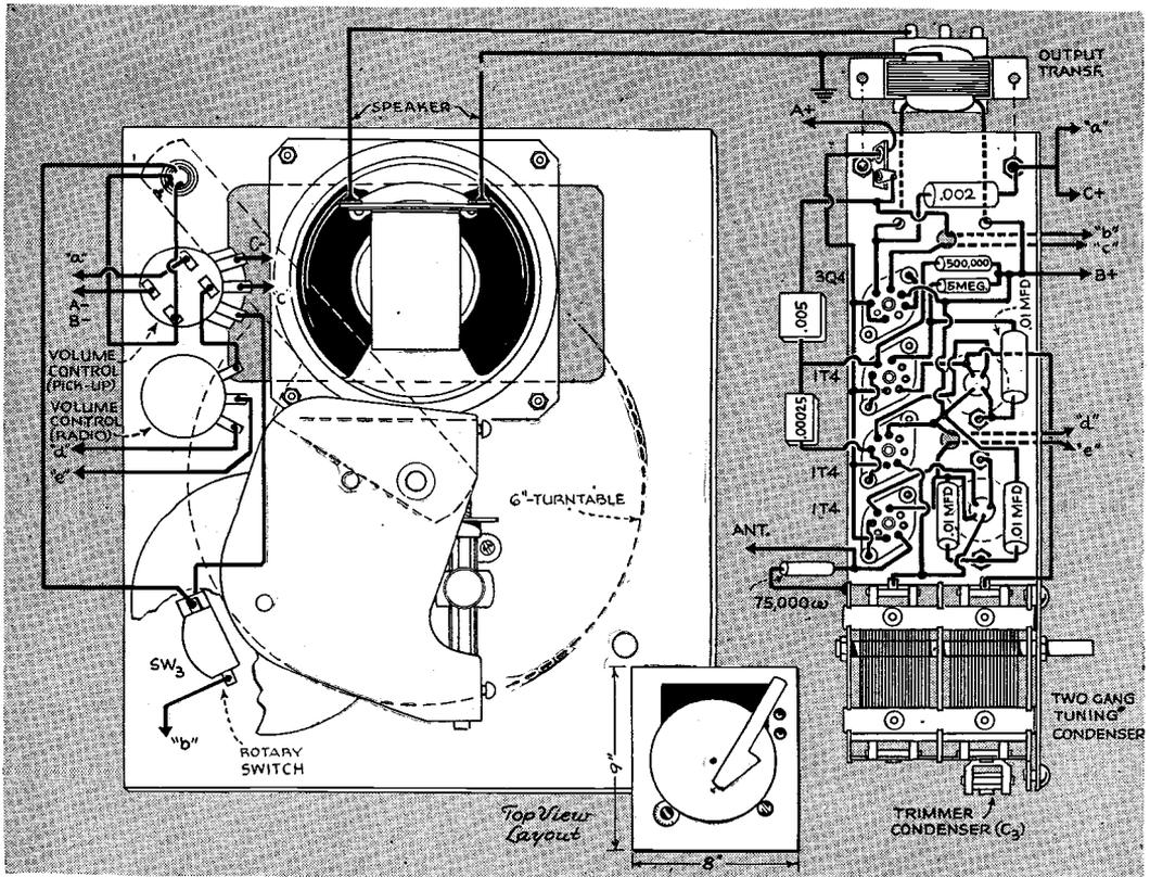
tween grid and ground. The antenna is connected directly to the grid of the first 1T4, and may be any length from 12' to 28'. No ground is necessary.
