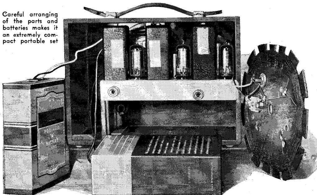
with cellulose cement and two  $\frac{1}{4}$ " round-head wood screws. These screws serve mainly to hold the pieces together while the cement dries thoroughly. All holes should be countersunk so the screw heads can be covered with wood putty. As a finish the case can be given two coats of clear lacquer with a sanding before and after the first, and a final rubbing down with pumice and rottenstone after the second, followed with wax.
