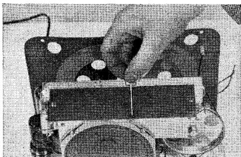
If the pointer is not calibrated properly with the frequency marks on the dial, it is an easy matter to move it to the correct position. Once it is set properly for one station, it will be correct for all
