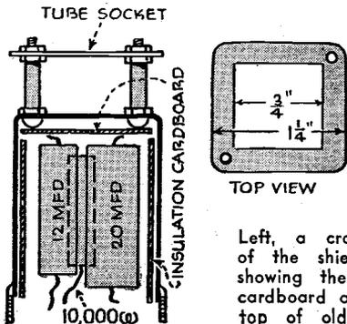
Left, a cross section of the shielding box, showing the insulation cardboard and, above, top of old coil can
