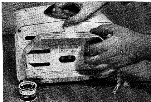
**5** Adhesive tape or glued paper holds the loop to the back cover of the radio cabinet or suspends it from the top of the back opening. The antenna is light enough to need no other support
