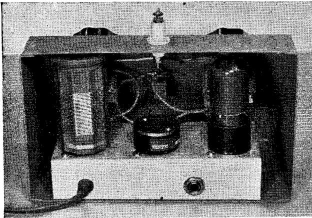
FOR the amateurs specially authorized by the Government to use transmitters for specified emergencies, a complete sending and receiving station is detailed on these pages. Inexpensive and compact, as well as easy to build, the efficient short-wave receiver and "punchy" little transmitter will provide an excellent stand-by station in case of trouble in regular equipment.
