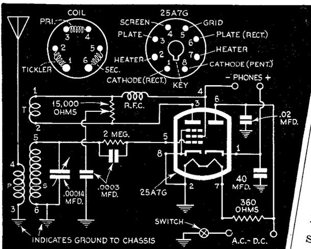
All connections are clearly shown in the diagram. Note particularly the negative phone connection to pentode-tube screen, and absence of a ground
