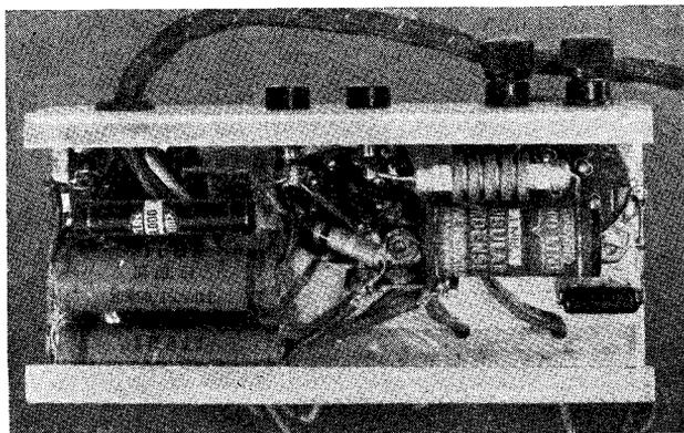
Amateur-band tuning is done with the coil (right) on the receiver chassis. The tubes are 6J7 and 25Z6. Above the two electrolytic condensers, at left in the bottom view, is the wire-wound resistor. The RF choke is shown at right
