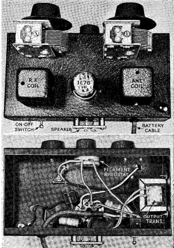
These views of the top and underside of the chassis will serve as a guide in placing the various parts. Below, the set in operation. Note the batteries and separate speaker unit
