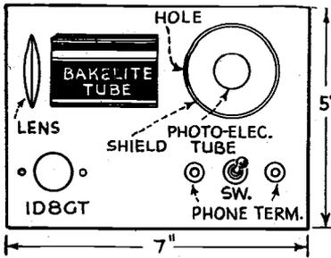
a 1.4-volt filament is used. To operate the receiver, two 45-volt "B" batteries and a 1½-volt "A" battery are needed.
