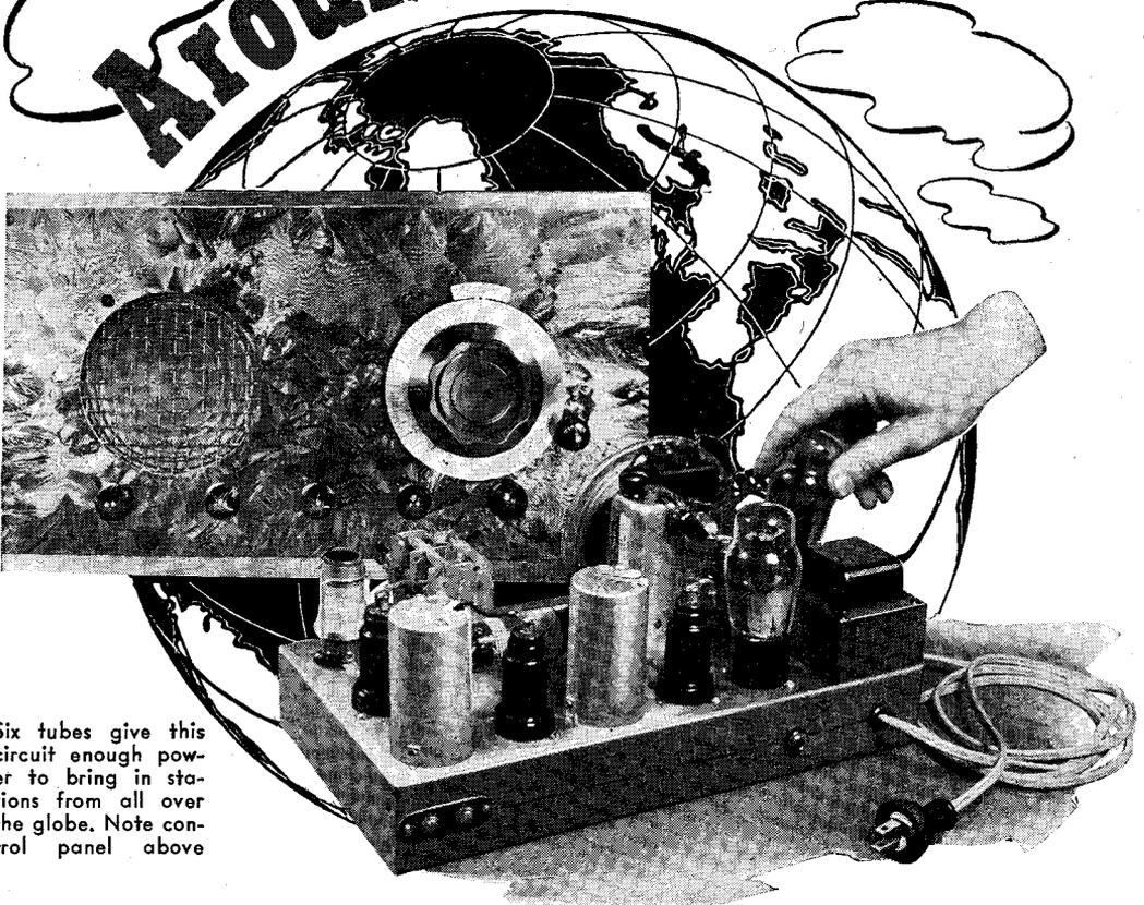
Six tubes give this circuit enough power to bring in stations from all over the globe. Note control panel above
