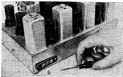
**WHEN TUNING-STAGE ALIGNMENT**, especially at the upper end of the dial, is not possible with a receiver using a loop antenna, reception may be improved in some cases by connecting a fixed condenser (.002 to .02 mfd.) across the loop antenna and ground, or by shorting the two.
