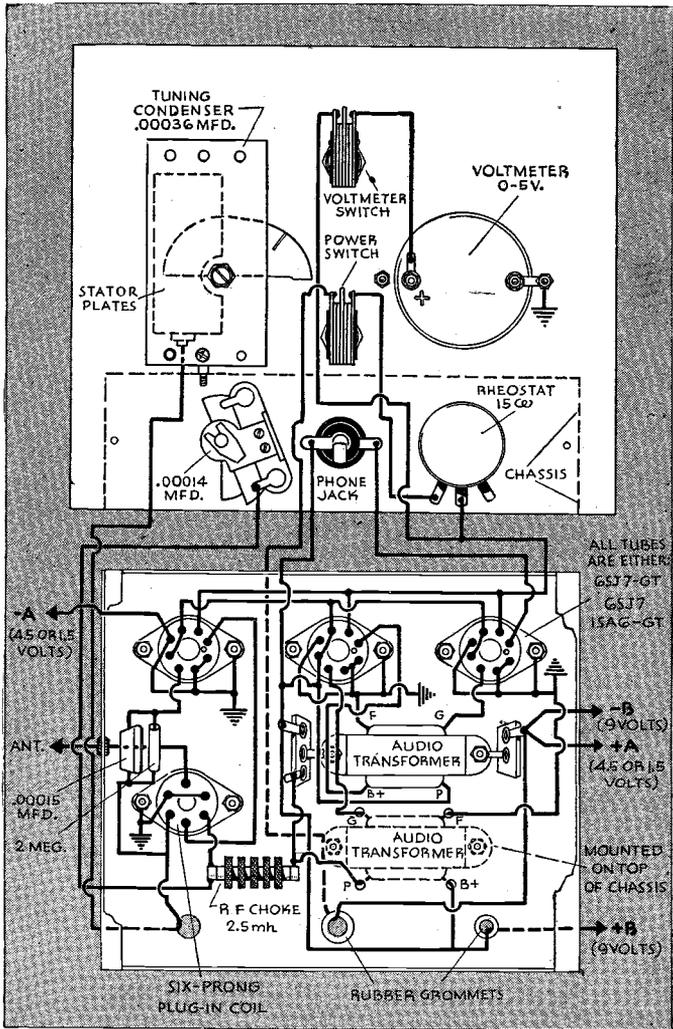
Pictorial diagram of the compact, portable emergency receiver. This shows in detail the placing of the parts both on the chassis and on the front panel. In making the connections, solder should be used
