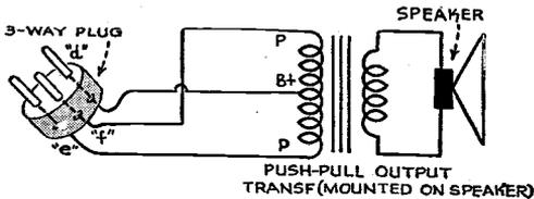
input stage transformer-coupled to a pentode push-pull output stage. When the amplifier is connected to the tuner, remove the triode tube (HY123) and join the grid and plate terminals of the socket as shown.
