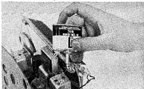
A squeaky slide-rule dial is remedied easily by a little oil on the wheels over which the dial cord runs. Oil very lightly with a light lubricant, being careful not to get any oil on the cord itself
