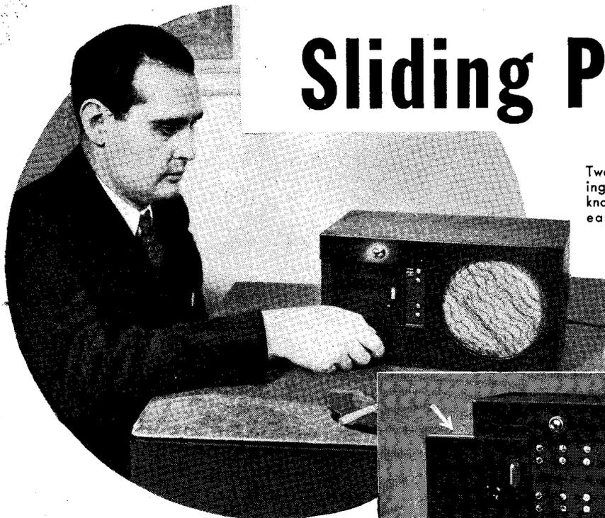
Two controls — a sliding panel and a volume knob — operate this easily built receiver
