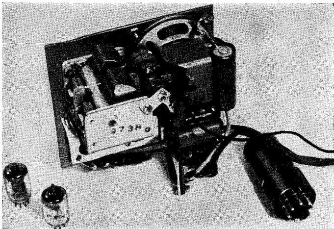
Back view of receiver, wired but with the tubes removed. The RF coil, mounted on the metal panel by means of a  $\frac{3}{4}$ " angle bracket, is shown just next to the 50,000-ohm variable resistor. The 9002 midget high-mu triode tube and 9003 pentode are at left
