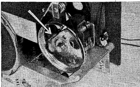
In some friction-drive dials, the cord is kept taut by a spring behind the dial plate as shown above. To tighten the cord, it is necessary only to remove the spring and make another knot in the drive cord
