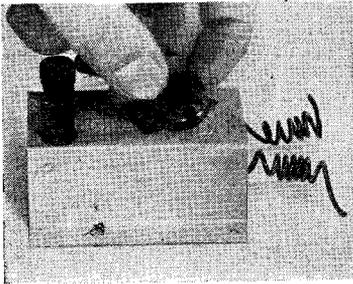
SHOULD an old-type electrodynamic speaker lack a "hum-bucking" winding on the voice coil, connect a 30-ohm, 10-watt, center-tapped potentiometer across the power transformer's 2.5-volt or 6.3-volt heater winding in series with the voice-coil winding. A short, soldered wire serves as a center tap.
