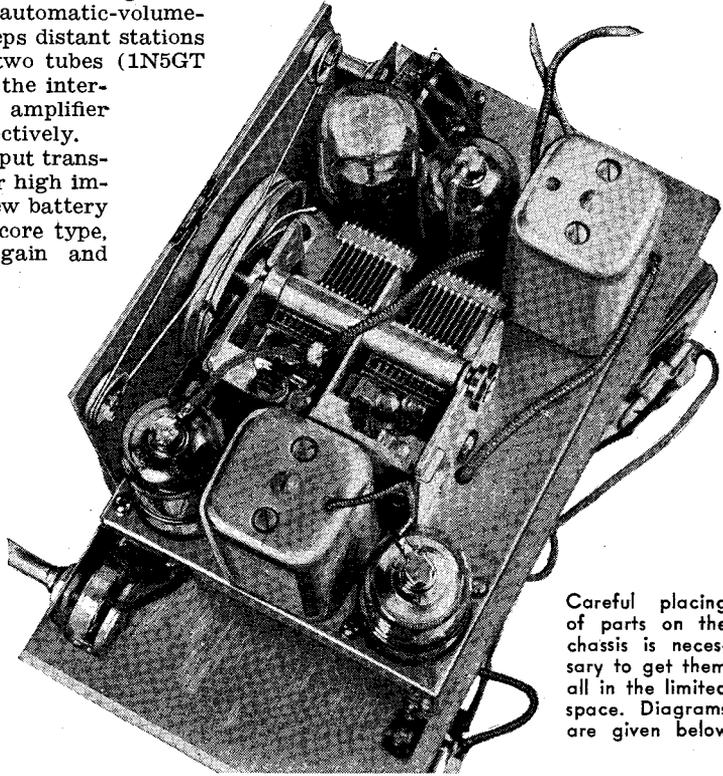
Careful placing of parts on the chassis is necessary to get them all in the limited space. Diagrams are given below
