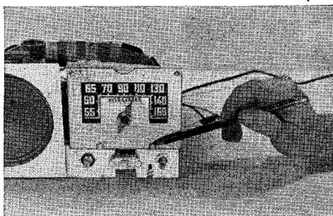
To get at a spring behind the dial plate as shown in the photograph above, it is necessary to take off the plate. To do this, loosen the two hex nuts indicated by the pencil in this illustration
