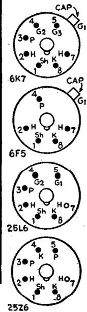
All connections for the A.C.-D.C. radio are given in this circuit diagram, while the sketches of the tube bases at right show how the tubes should be wired
