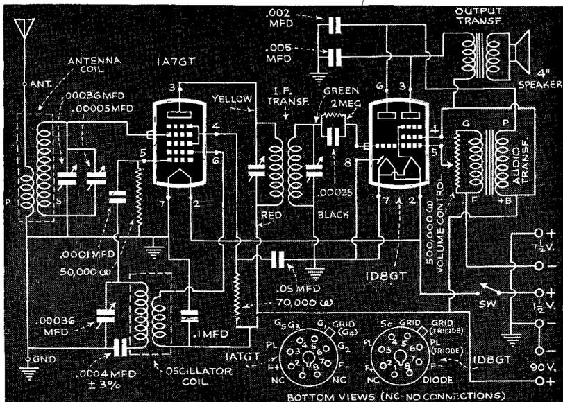
I. F. transformer can with a screw driver, until the signal is at its loudest. Then tune to a weaker station (near 1,500 kc.) and give it a final adjustment.
