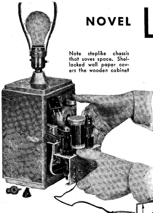
COMBINING a reading light and a broadcast receiver, this Chinese lamp radio will form a useful addition to a living room, a bedroom, or a den. It is easy to assemble, and the use of a modern dual-purpose tube makes the necessary parts few in number and inexpensive.
