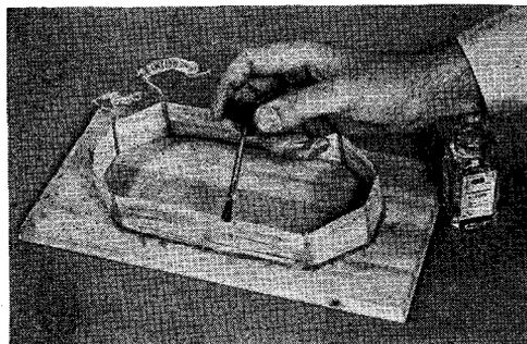
**3** At the sides, carefully drive in two more nails to stretch the windings; then apply with a brush a special liquid dope solution carried by radio stores. This sticks the windings together
