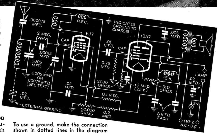
cuit are mounted on "steps" on the aluminum chassis which should be cut and bent to shape according to the diagram. The combination lamp base and radio cabinet is made of pine and is detailed in the drawings. Round the edges of the cabinet with a file and sandpaper before adding the wall paper, and you will avoid any homemade appearance in your finished job.
