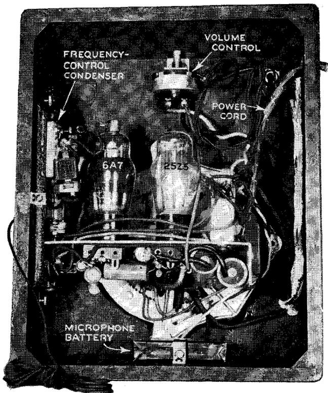
**I**NEXPENSIVE and easy to build, this "wireless" record player may be used with any alternating-current radio receiver without making any actual connections to the receiver circuit. In addition, when you plug in a microphone and flip a switch, the record player becomes a public-address system that will allow you to do your own program announcing through the radio's loudspeaker. In use, the device is simply plugged into a convenient electric outlet.
