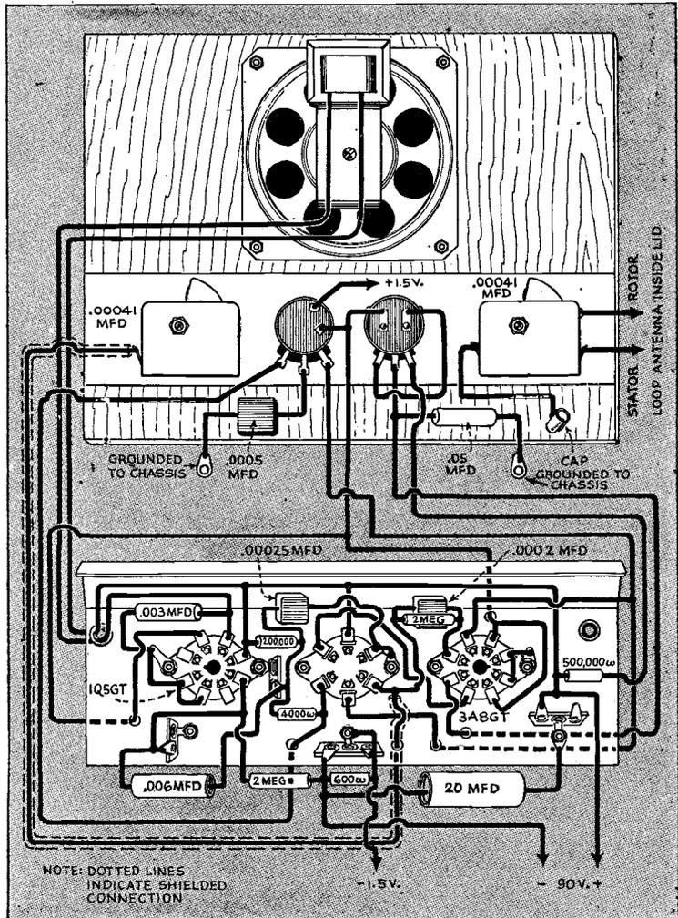
Complete wiring details for the circuit are given in this picture diagram
