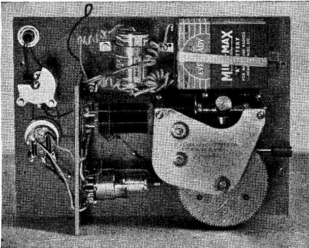
Underside of the phonograph's Masonite baseboard, showing transmitter, batteries, and turntable motor
