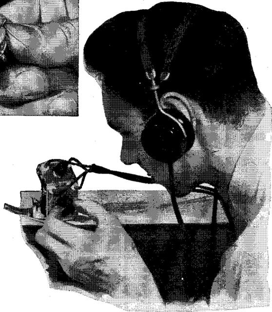
SO SMALL it fits in the palm of your hand, this little radio receiver makes use of one of the midget, acorn-type tubes. Powered by batteries, it provides good earphone reception on the broadcast band.
