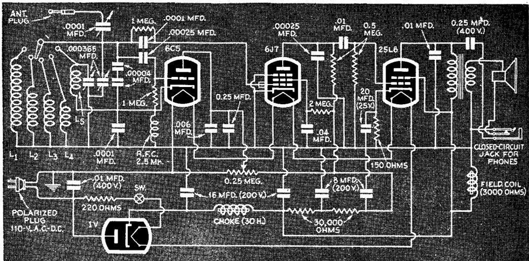
Two novel features of the hook-up are the polarized power plug, and the use of a separate tube for regeneration
