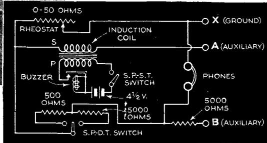
**P**ROVIDING a quick and easy means for measuring small resistances and testing grounds, the unit illustrated forms a handy piece of equipment for the radio experimenter and service man.
