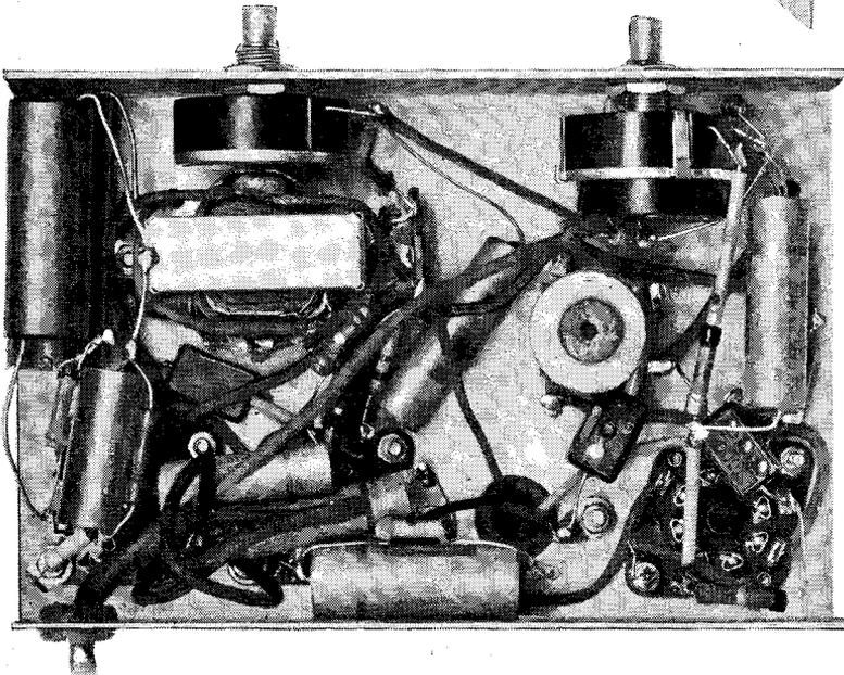
Top view of the chassis, above, will help you arrange the various parts. The chassis measures only  $6\frac{1}{2}$ " long by  $4\frac{1}{4}$ " in depth
