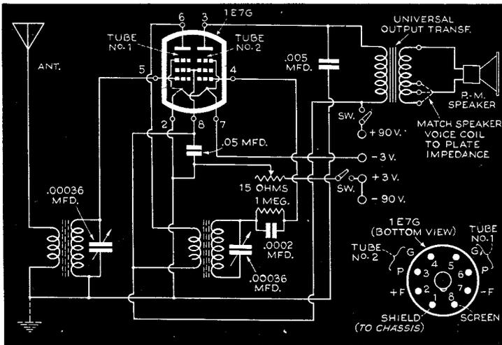
With only one tube, the circuit wiring is easy, even for a beginner.
