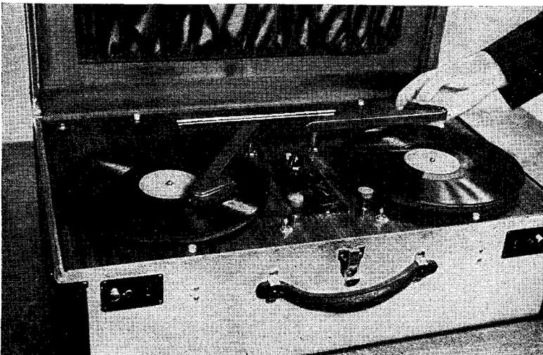
Close-up of the motor panel showing the two turntables and pick-up arms, and the tone and fader controls. The switches next to the turntables operate the phone motors. While one unit plays music, the other may provide the incidental sounds
