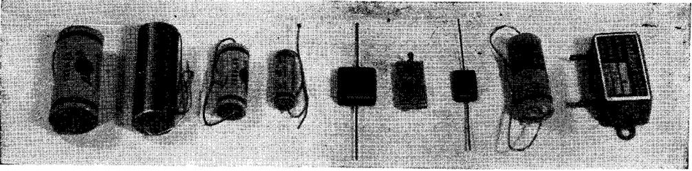
**FIXED CONDENSERS.** Nine types commonly used, left to right: .5-mfd. paper condenser; 8-mfd. midget electrolytic condenser; two (.05 and .02-mfd.) small paper condensers; three mica condensers (.002, .00075 and .0001-mfd.); a 50-volt, 25-mfd. electrolytic condenser; and a 1-mfd. paper condenser in a steel shell
