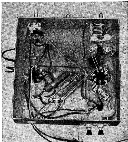
sistor. However, the filaments of the 1E7-G draw 2 volts at .24 amperes so that it is necessary to insert an 8-ohm semivariable resistor in series with the filament prong (No. 7) of the tube and the chassis.
