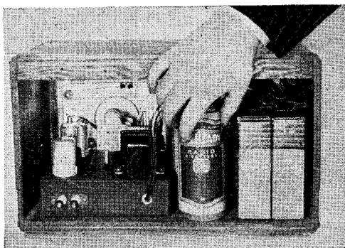
This is a back view of the cabinet shown above at right. The 2" by 7" by 7" chassis is on the left, and the "A" and "B" batteries are seen at the right
