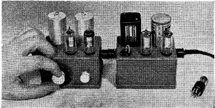
The tuner is a radio-frequency stage using a pentode r.f. amplifier coupled to a detector stage using a tube of the same type. Coupling is accomplished by means of an iron-core r.f. coil
