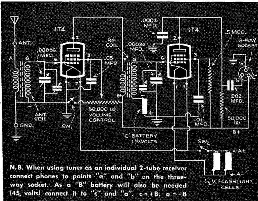
N.B. When using tuner as individual 2-tube receiver connect phones to points "a" and "b" on the three-way socket. As a "B" battery will also be needed (45 volts) connect it to "c" and "a". c = +B, a = -B
