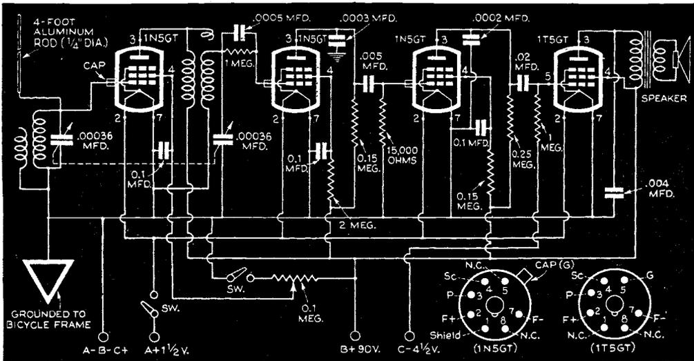
These circuit and tube-socket diagrams should be followed to the letter in constructing the set
