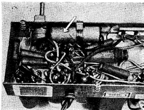
**SQUEALING AND WHISTLING** that make it impossible to tune in a station clearly on a small A.C.-D.C. receiver may mean failure of one or both of the filter condensers shown in the photograph above and the diagram below. The noise is usually accompanied by a noticeable loss in volume. If defective, the condensers must be replaced.
