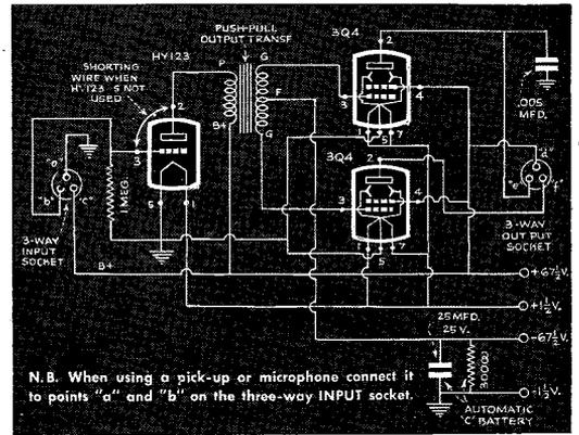
N.B. When using a pick-up or microphone connect it to points "a" and "b" on the three-way INPUT socket.
