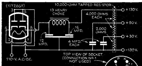
Parts needed for the unit can be itemized from the diagram. Note that the circuit is not grounded
