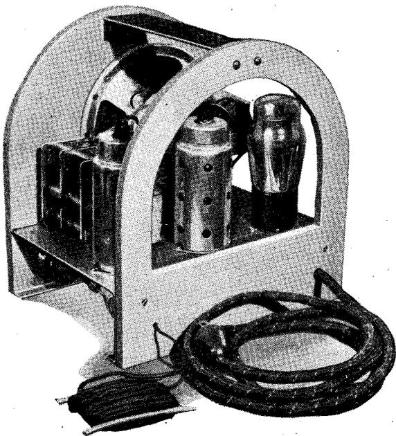
No outside ground connection is needed with the receiver. Only the short flexible antenna wire, at the left, is necessary to get excellent reception
