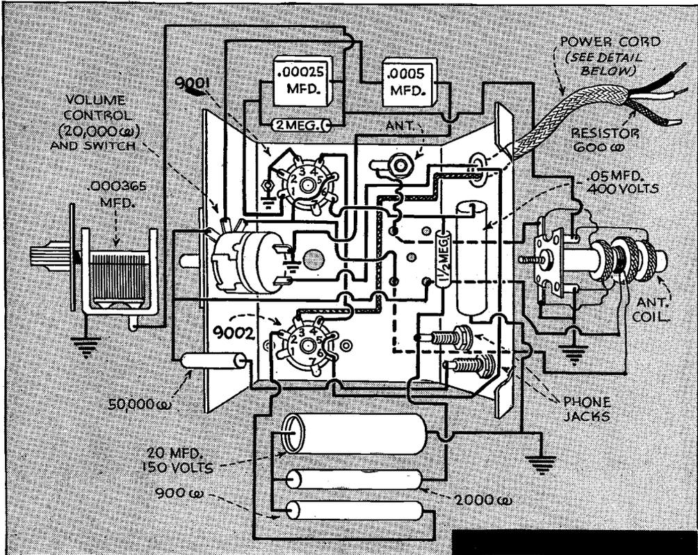
Arrangement of the parts is detailed in the pictorial diagram above. Note that the tickler-coil winding is placed between the antenna-coil and the first of two secondary-coil windings
