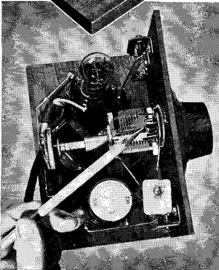
Follow this rear view of the set when placing the parts. Below, the crystal detector with cap removed
