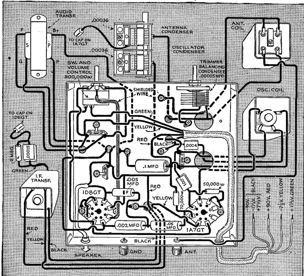
As shown in this pictorial diagram, the 1A7GT pentagrid tube is used as the first detector and oscillator, with the two-gang tuning condenser
