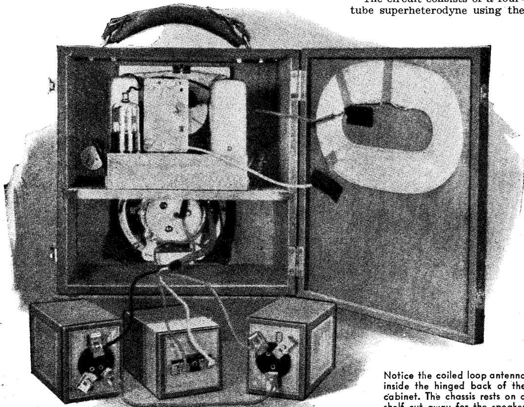
Notice the coiled loop antenna inside the hinged back of the cabinet. The chassis rests on a shelf cut away for the speaker frame. Under the shelf go the batteries for the four-tube set
