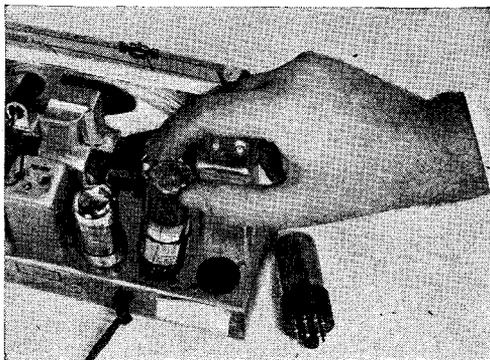
**INCREASED HEATER VOLTAGE** may be necessary if the rectifier tube burns out quickly on an A.C.-D.C. radio having a new high-voltage heater tube and no line-cord resistor. Try replacing the 35Z5-GT/G rectifier tube with a 45-volt rectifier, such as a 42Z5-GT/G, to increase the heater voltage to 120 volts.
