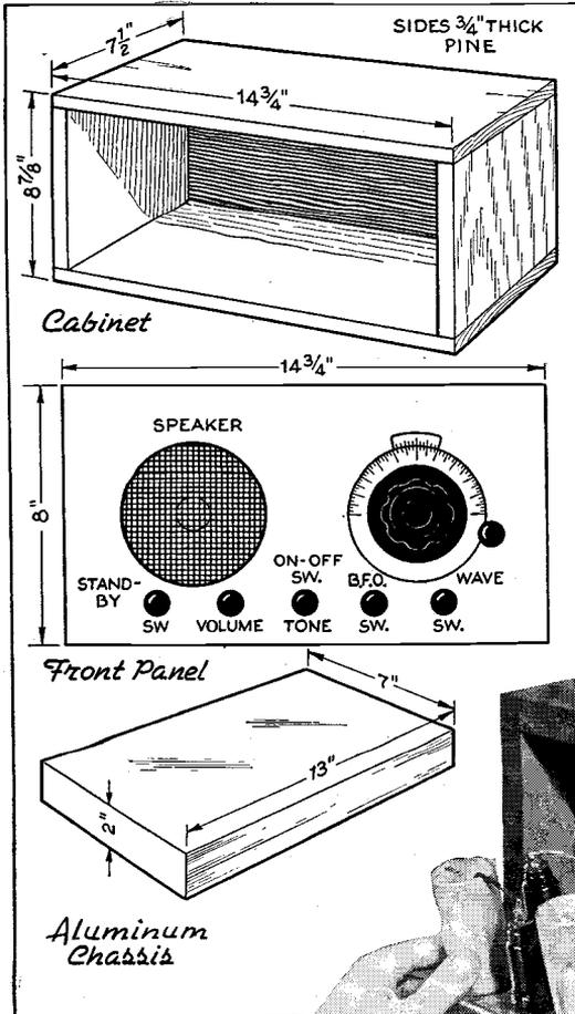
Cabinet, panel, and chassis dimensions and arrangement of controls should be followed closely
