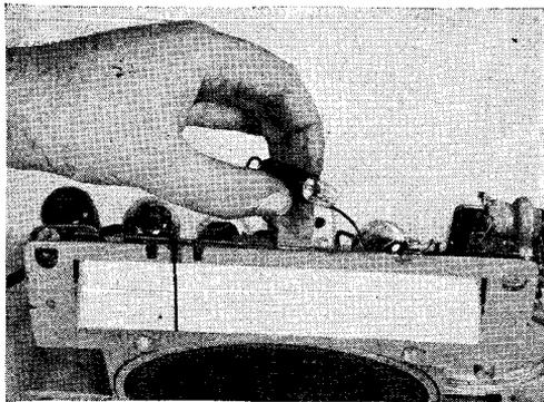
**CHANGING PILOT LIGHTS** is a simple operation in servicing a small A.C.-D.C. receiver, but be sure that you disconnect the radio at the wall socket—don't just turn off the switch. A serious short can occur if the pilot-light bracket and holder drop on the tuning condenser or chassis.
