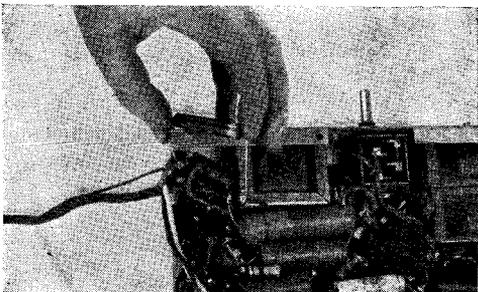
**FADE-OUT** experienced on many old sets is due to a fixed carbon resistor that has become crystallized. It usually can be recognized by a coating on its surface. If not, try connecting a 50,000-ohm, 2-watt resistor across each carbon resistor in the B+ circuit. If playing resumes, replace with one of correct value
