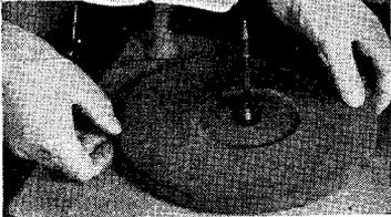
WHEN the hum occurs in the speaker only when the phonograph is being used, ground the pick-up arm and motor frame to the radio chassis, both leads from the pick-up being grounded with braided shield covering. If the hum persists, a 1/16" metal plate, 8" to 12" in diameter, will act as a magnetic shield if screwed to the motor board between the motor and turntable.
