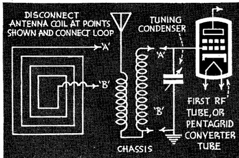
**6** To use the loop, disconnect the old antenna coil, as shown. A few turns of the loop may be removed one at a time if needed to balance the trimmer condenser on the ganged tuning condensers
