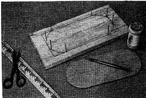
**1** Cut a cardboard template about three fourths the size of the back radio cover or opening, lay the template on a board, and around it drive eight 2" nails or pegs. The one here is 4" by 9"
