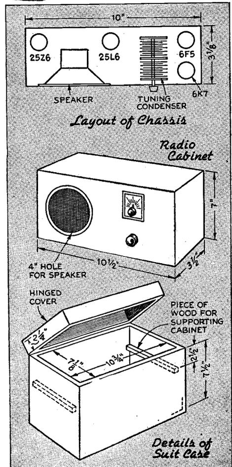
Measuring just over 5" square and less than 3" thick, this receiver and its 2" speaker cone equal the performance of much larger sets. The tiny cabinet is made of wood bound in genuine cowhide
