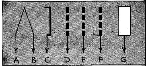
Shorts may be tested between plate and suppressor, G and F above; suppressor and either screen grid, E, or control grid, D; screen and control grid, E and D; control grid and cathode, D and C; and control grid and filament, D and A
