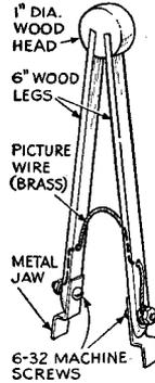
WORK CAN BE SPEEDED UP in servicing old radios with this gadget made from wooden photo tongs, such as is used on wet prints. Switch on the receiver and begin shorting the different fixed resistors. When the defective one is shorted, reception improves.
