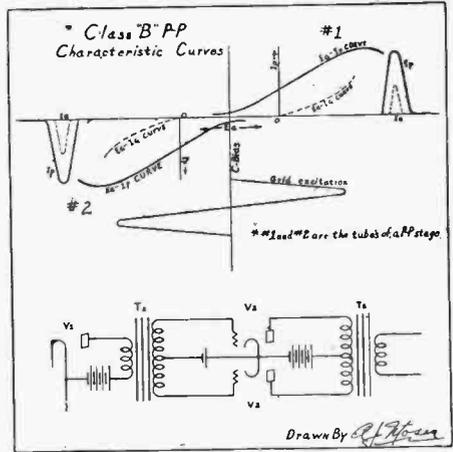
grids are excited, as shown below, a pulse of plate current flows for alternate half cycles in the plate circuit of each tube. Since these pulses of plate current of each tube do not flow during the same half cycle each current will set up a strong D. C. field necessitating the use of a large core for T<sup>2</sup> in order to minimize the possibility of core saturation.
