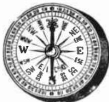
Each instrument is warranted to be accurate. Its needle will always point NORTH, and it therefore is invaluable for orientation purposes. It is extremely sensitive. The magnetic action of an electric street car a block away will deviate the needle. The metal casing is of polished brass.
