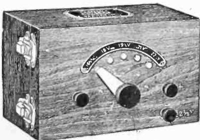
With a sealed-in B Battery there is no possibility of replacing a defective cell. If a loose connection or short circuit develops in one cell only, the whole Battery must be discarded, even though the remaining 14 cells are in perfect condition.
