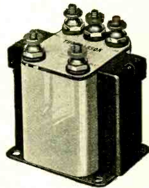
Thordarson Power Amplifying Transformers. Give best results when preceded by two stages using 3 1/2:1 Thordarson A.F. Transformers. May also be used as 4 1/2:1 audio freq. transformers by disregarding center taps, or as a coupling transformer for loud speakers. Unconditionally guaranteed. Per pair. . . . $13
