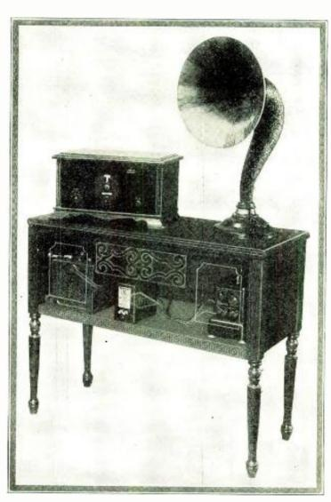
Photo A. The Lodge "N" Circuit Receiver is herewith shown as it appears when installed in a cabinet in conjunction with a table housing the necessary accessories for the proper operation of the receiver
