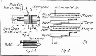
fibre about one inch in diameter. this form is wound about 5 oz. of No. 31 B. & S. enameled magnet wires to have a resistance of 118 ohms; paraffined paper is wound on between every layer of wire to improve the insulation. layers of wire are kept about 1/8" shorter or both sides than the waxed paper.
