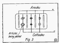
Below is given a table of the usual potentials employed for various kinds of electro-plating. The voltage should be specially adjusted for each case to give the most suitable current, and depends upon the size of the plating tank, the area of the anodes, the strength of the solution, and several other things, and most platers determine the best po-
