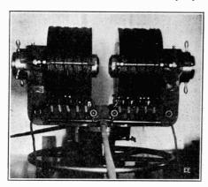
A 40 Kilowatt experimental electro-magnet with water cooled coils.
