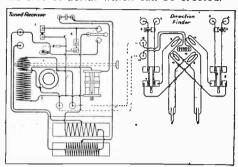
plane of the aerial is at right angles to the direction from which the signals are coming it receives no impulses. In intermediate positions the current induced in the aerial due to the Hertzian waves varies as the cosine of the angle between the plane of the aerial loop and the direction of the
