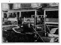
A radio outfit installed on a touring car.
