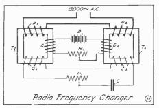
Arrangement of static transformer circuits for producing triple frequency multiplication.
