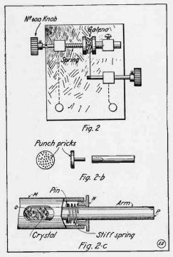
importance than the lightness of the contact. For this purpose a short piece of 36 or 38 guage copper or phosphor bronze, gold, etc., wire should be fast-ened at one end, and the other allowed to rest by its own weight on the galena.
