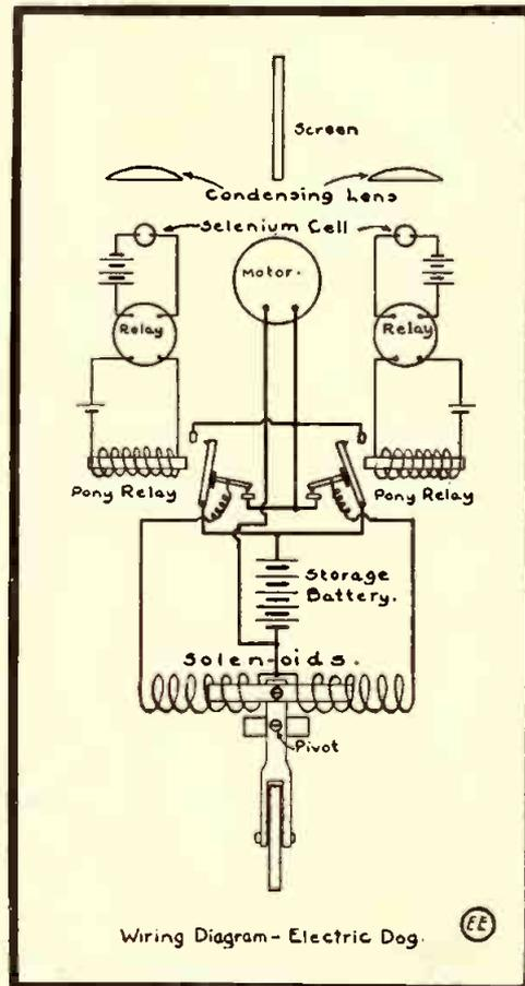
Diagram of Circuits Used in Electrically Controlled "Dog" Utilizing a Beam of Light and Two Selenium Cells.
