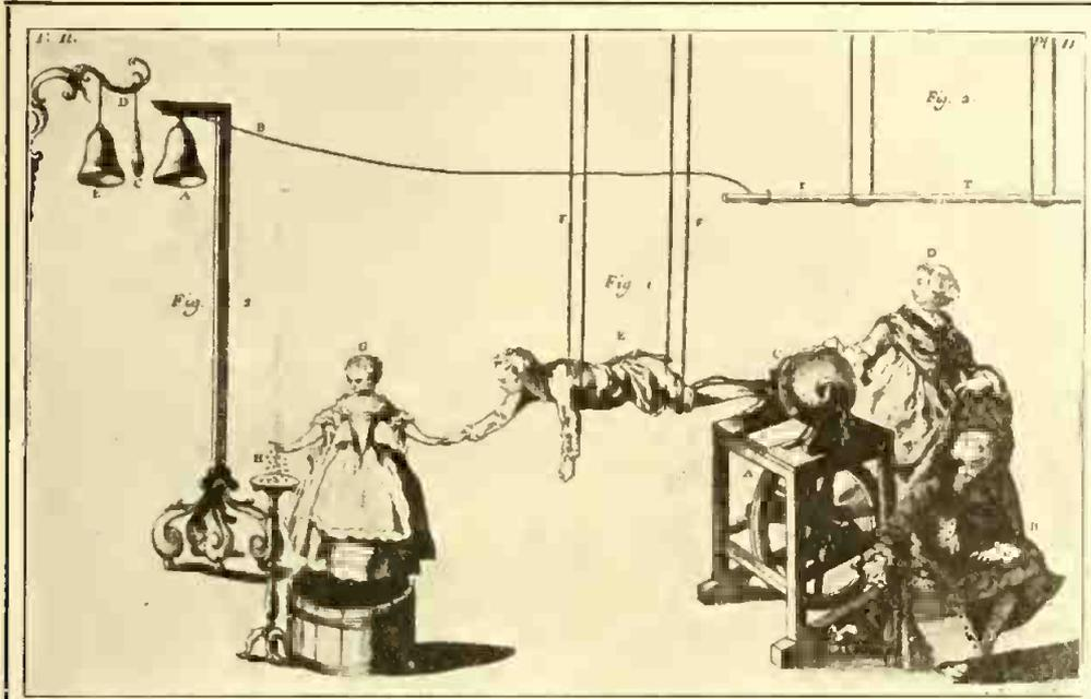
Fig. 2. Experiments with the Early Static Electric Generators Were Mostly Carried Out With a "Human" Prime Conductor as Here Shown.
