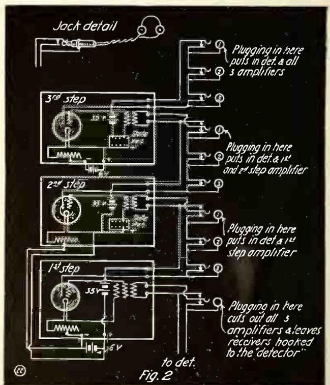
Fig. 2. Diagram of 3 Audion "Amplifier" Bulbs and 'Phone Jack Circuits.
