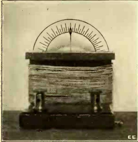
Photo of Complete Galvanometer. (Four Posts Being Used; Only Two Shown.)
