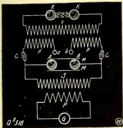
Imitating a Static Machine Spark with High Frequency Coils.
