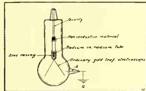
Fig. 7. Radium Will Run This Clock 2,500 Years. The Nearest Approach to Perpetual Motion.
