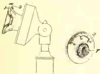
as to methods of quickly attaching and detaching same from telephone transmitters and receivers. Spring clips 9 and 12 enable the user to perform the attachment quickly. The transmitter shield 1 also carries a perforated disc 7, etc.
