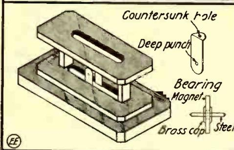
Assembly and Details of Sensitive Galvanometer.
