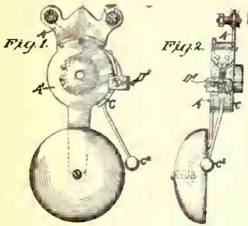
patentee arranges his bell very simply with a single magnet coil and the iron checks A and A' of the magnet bobbin attract the vibrating iron armature C, carrying the gong striker C'. The usual vibrator contact screw D is placed outside of the bell, but the general design is indeed rugged and simplified.
