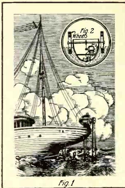
Attaching Small Battery Motors to Model Boats.
