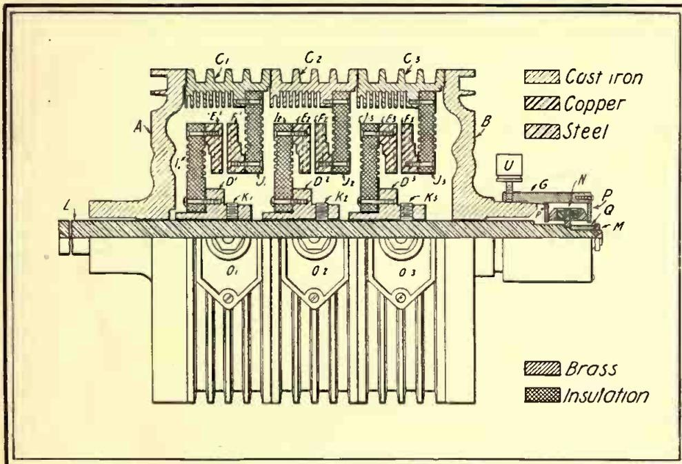
The Highly Efficient Rotary-Quenched Spark Gap (Hy-Tone) Produces 500 Cycle Tone Spark From 60 Cycles A. C. Etc.
