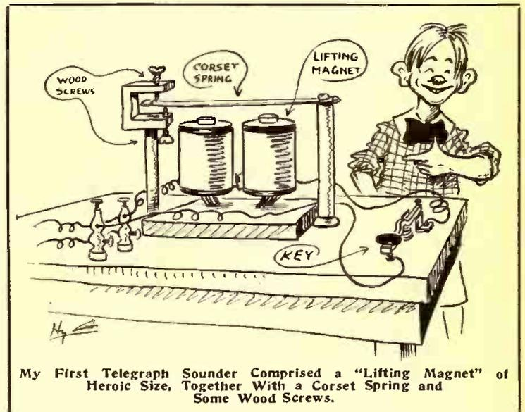
My First Telegraph Sounder Comprised a "Lifting Magnet" of Heroic Size, Together With a Corset Spring and Some Wood Screws.
