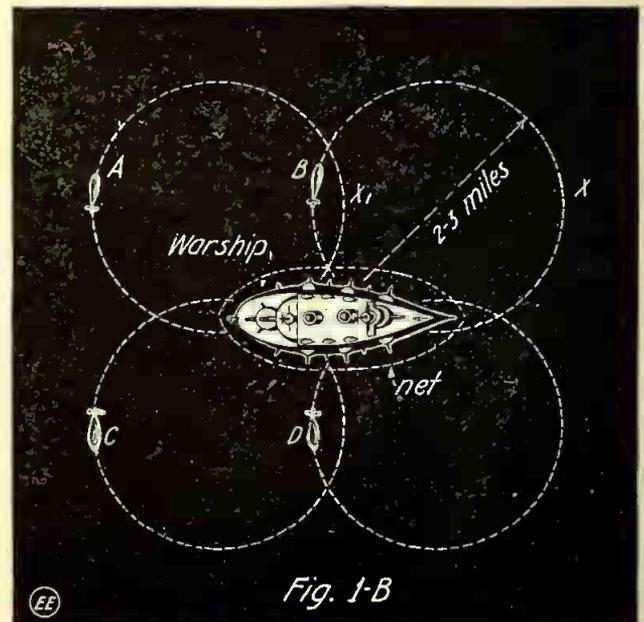
Fig. 1B. Scheme for Protecting "Dreadnaught" from Submarine with Several Radio Directive (Scouting) Torpedoes.
