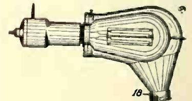
easily understood by examining the drawing. The inventor provides a metallic shell divided hemispherically, so as to be placed over an incandescent lamp by means of a suitable holder, as described. The egg to be inspected, is placed in the opening 18.
