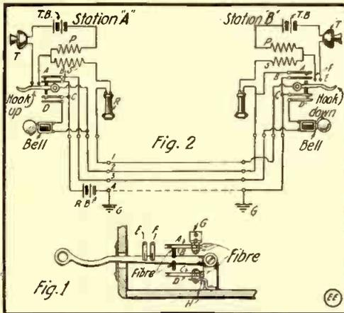
Automatic Bell Ringing Circuits for Battery Telephones.
