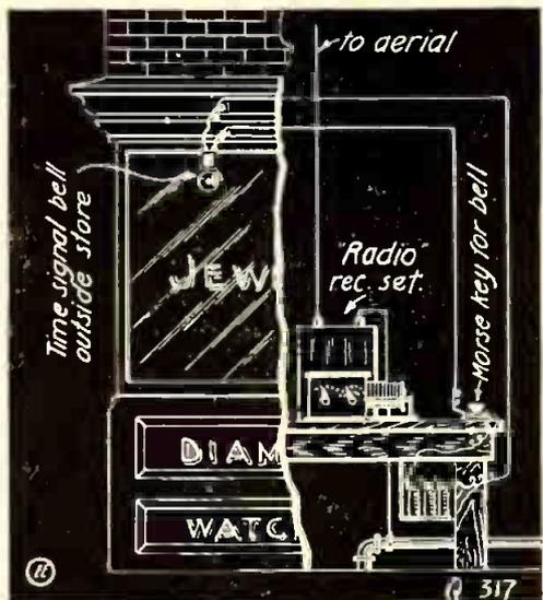
Electric Bell Signal for Radio Time Signals.
