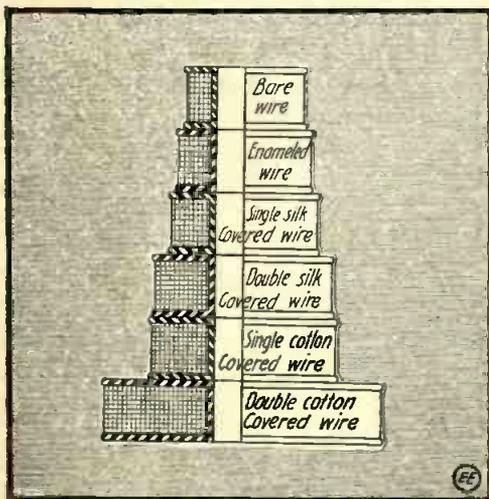
Showing Relative Volume of Various Kinds of Insulated Magnet Wire. Note Small Space Occupied by the Enameled Wire.
