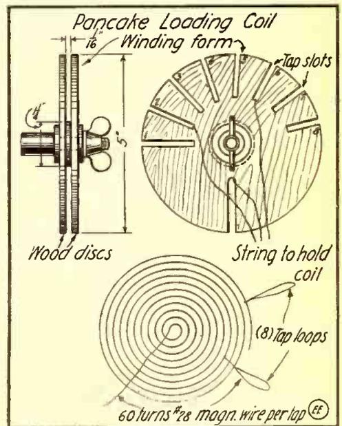
Details of Loading Coil for Loose Coupler Shown in Supplement.
