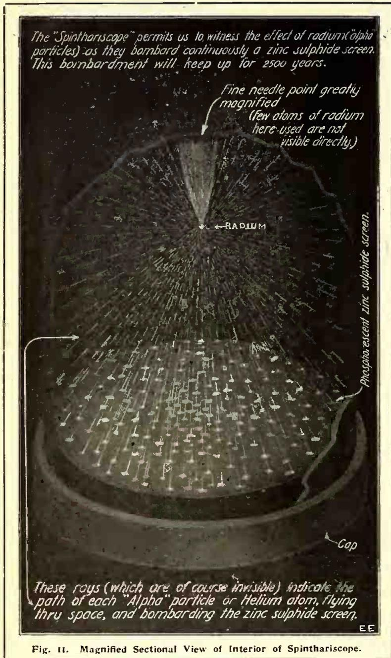
Fig. 11. Magnified Sectional View of Interior of Spintharoscope.
