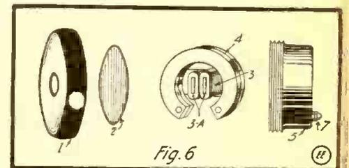
Fig. 6. Details of the "Watch-Case" Telephone Receiver.
