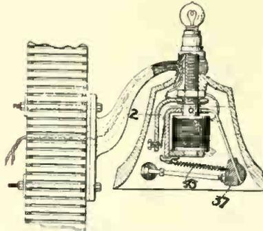
lamp is provided as well as special compact form of electro-magnetically operated bell. A single magnet coil attracts an iron armature 2 and this raises the striking hammer 37 in the bell. A spiral spring 43 helps to return the striking hammer.
