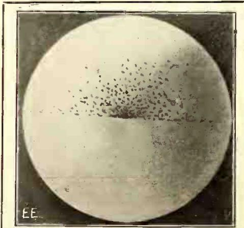
Fig. 10. View Through Eye-Piece of Actual Spintharoscope.
