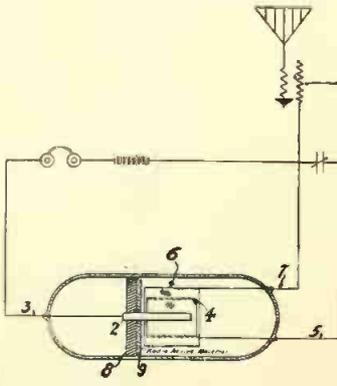
An electronic valve detector for wireless telegraphy, intended to utilize the electron radiations from some radio-active material, such as pitch-blende, etc. As drawing shows, the wireless tuning circuits are hooked up by means of wires, 3, 5,
