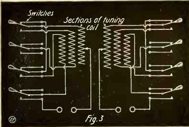
Fig. 3. Special Hook-Up of Loose-Coupler Windings to Prevent "Dead-Ends."
