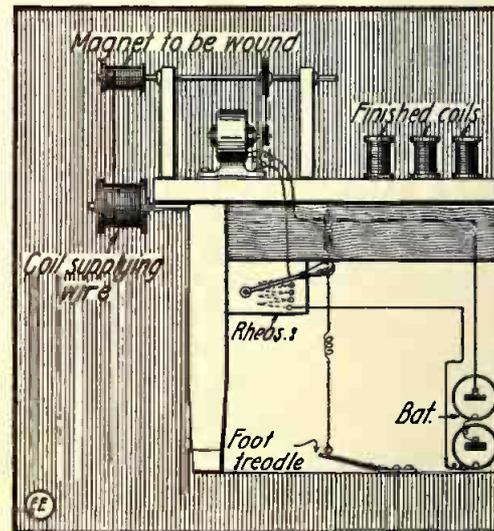
Simply Made Electric Winding Machine for Experimenters.
