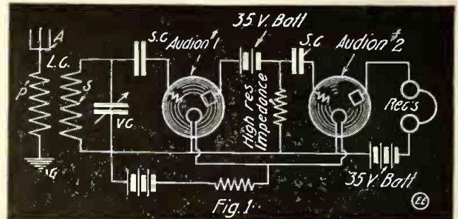
Fig. 1. Double Audion "Detector" Hook-Up.
