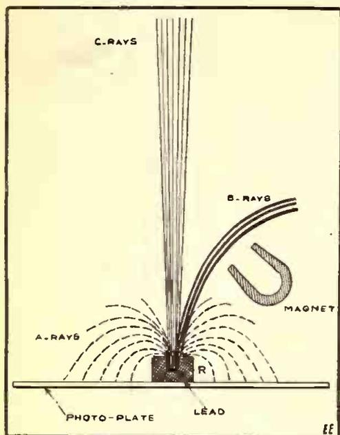
Fig. 1. Showing Effect of Magnet on the "Alpha" and "Beta" Rays.
