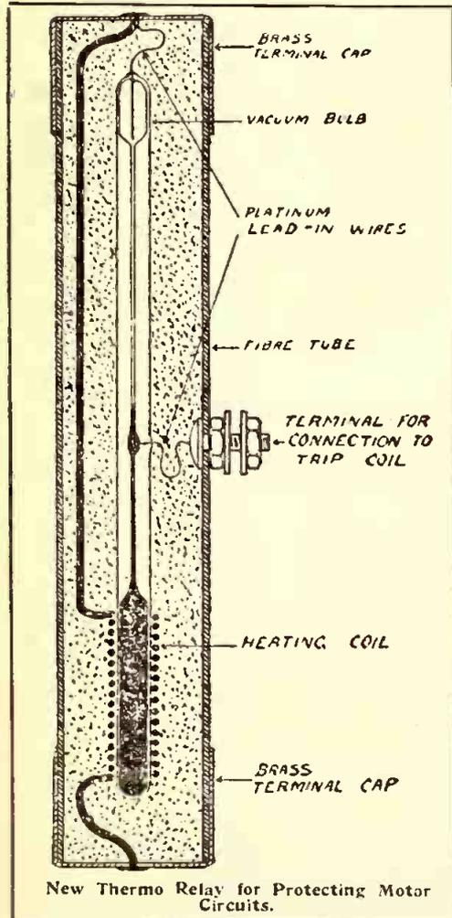
New Thermo Relay for Protecting Motor Circuits.
