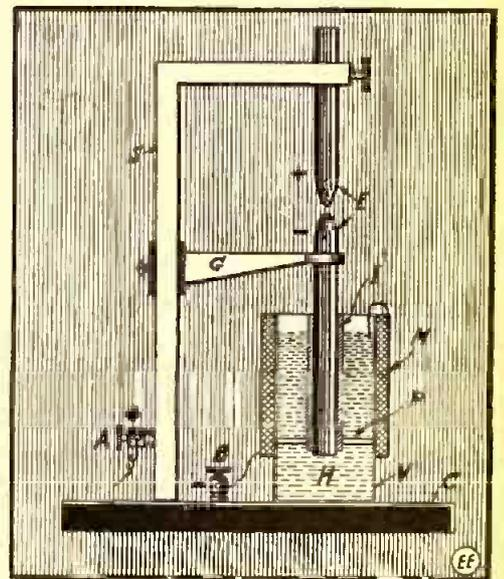
Construction of Simple Automatic Feed Arc Lamp.
