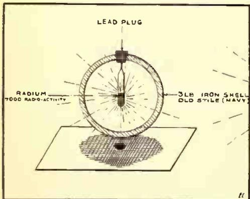
Fig. 4. Lead is Opaque to Radium Rays. The Lead Plug in an Iron Cannon Ball Shows a Black Spot on Photograph as Perceived.
