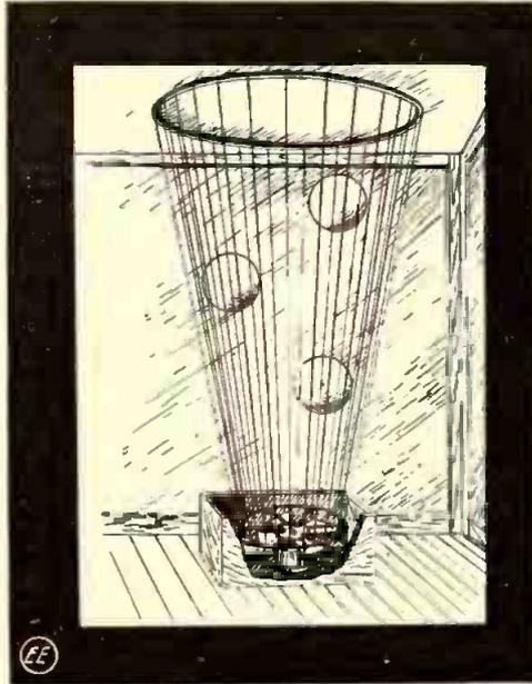
Effective Show-Window Attraction—Fan Blows Balloons Upward Continuously.
