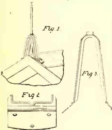
Simplified design for lightning rod points and particularly in rigid bracket supports for same, such as used on pitch-roofed houses. The device is seen in the illustration and the bracket is made from a specially grooved stamping to give maximum strength.
