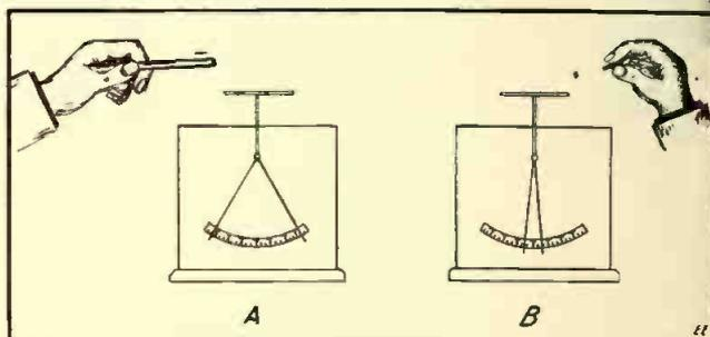
Fig. 2. Demonstrating How if Radium Is Brought Near a Charged Electroscope (A) That It Will Be Discharged (B) Owing to Electronic Rays Shot Off by the Radium.
