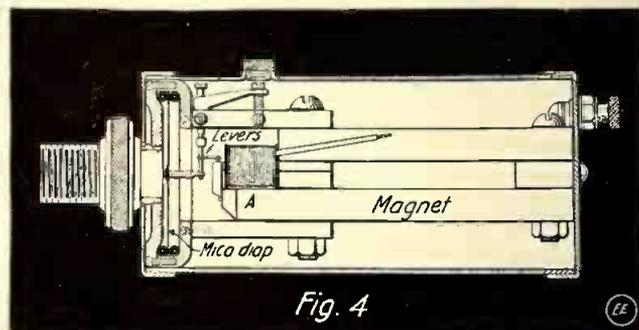
Fig. 4. Reproducer Construction Details.
