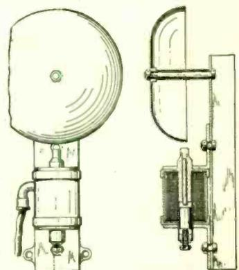
designed with an overhanging skirt on the head of the striker, so that no water can possibly enter the armature chamber or that of the coil.
