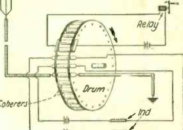
vided with switching attachments. First the coherer is connected to aerial and ground and after it is impregnated with an etheric wave current, it is the recipient of an inductive discharge current from the battery and inductance coil shown.
