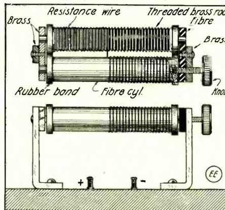
A Finely Adjustable Rheostat in which the Wire Is Wound On or Off a Threaded Metal Cylinder from a Fiber One.
