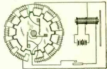
producing various tones of any desired frequency. A rotor, or plurality of rotors, having projecting teeth is used and these are surrounded by toothed stators having coils wound on them.
