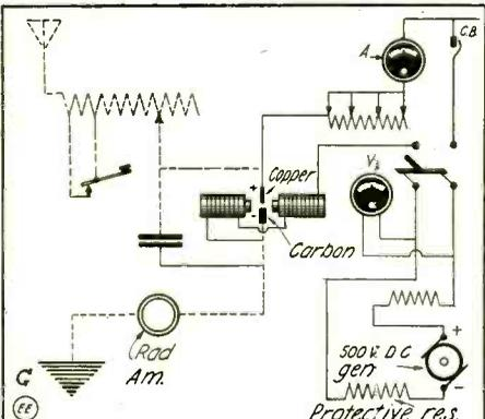
Fig. 7. How the 100 K. W. Poulsen Type Arc Transmitter at Arlington is Connected.
