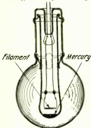
which is considerably above atmospheric pressure, allowing the carbon filament to be worked at high current density. Mercury vapor is desirable for these lamps and is carried in a small cup as indicated. The gas filling may include some nitrogen or argon.
