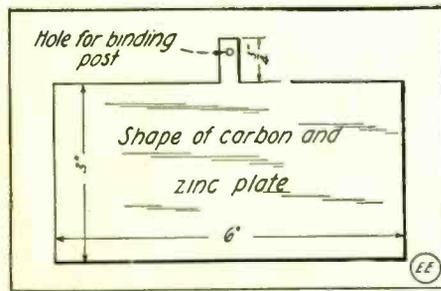
Showing Shape of Zinc and Carbon Plates Used in "Switchless" Battery Lamp.
