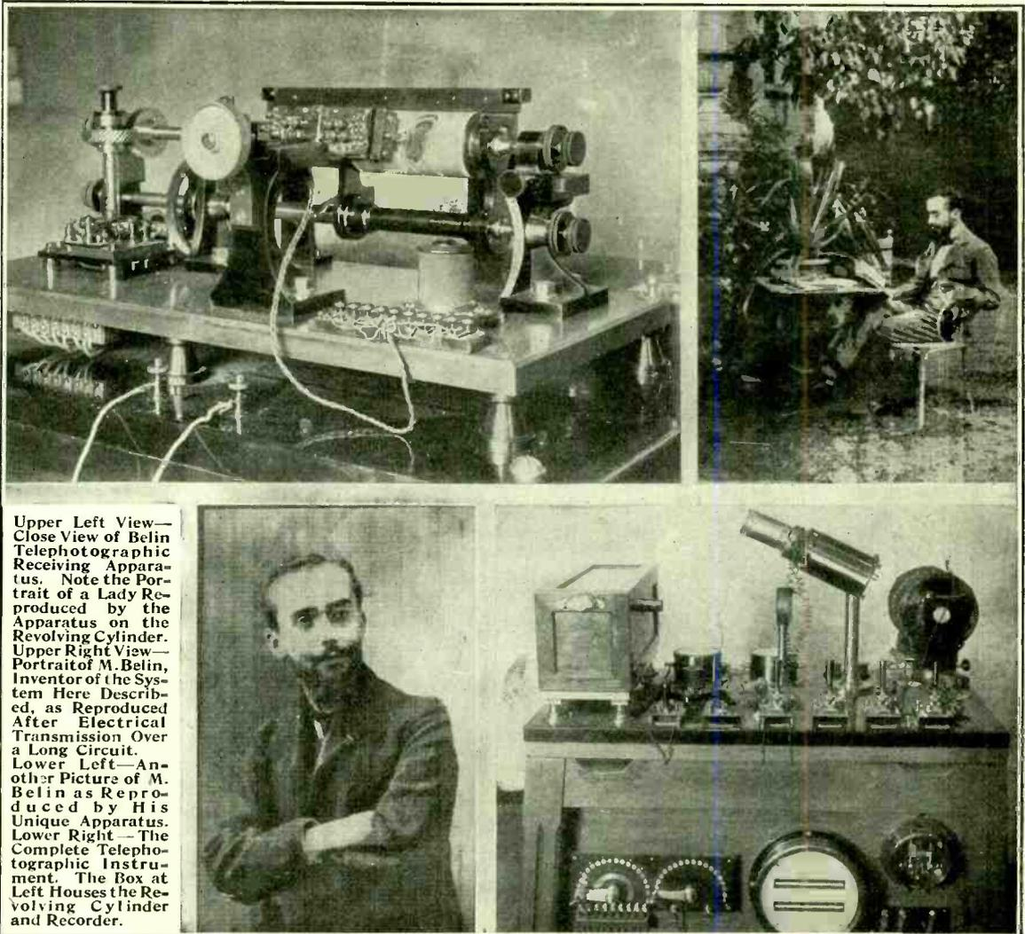
Upper Left View—Close View of Belin Telephotographic Receiving Apparatus. Note the Portrait of a Lady Reproduced by the Apparatus on the Revolving Cylinder. Upper Right View—Portrait of M. Belin, Inventor of the System Here Described, as Reproduced After Electrical Transmission Over a Long Circuit. Lower Left—Another Picture of M. Belin as Reproduced by His Unique Apparatus. Lower Right—The Complete Telephotographic Instrument. The Box at Left Houses the Revolving Cylinder and Recorder.
