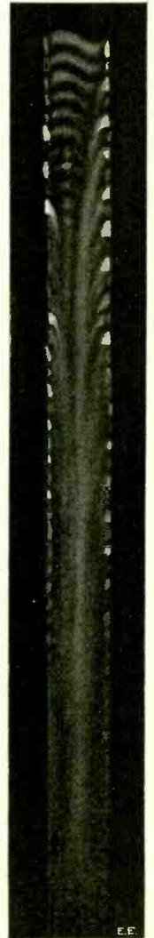
Fig. 3. Photograph of Spark Image Observable on Revolving Mirror Here Described, the Spark Occurring in Plain Gap.
