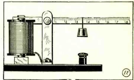
A Battery Gage that is Simplicity Itself. The Further Out the Weight is, the Stronger the Battery Excluding the Magnet.
