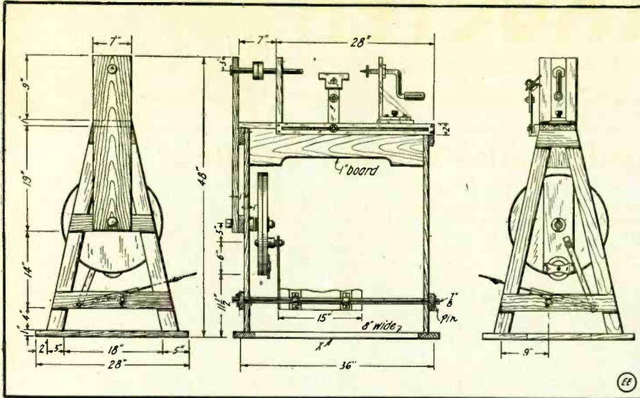
The Completed Lathe. It is Designed to Be Operated by Foot Power, but Can Be Readily Belted Up to a Motor or Engine. About 1/8 to 1/4 H. P. Will Drive It Nicely for Ordinary Work.
