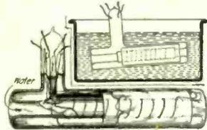
provided with an internal passage-way, as shown. Hence the device may be placed in a vessel containing water or other liquid, and a stream of water may be caused to flow thru as well as around the bulb. The tube contains the usual filament, grid and wing.
