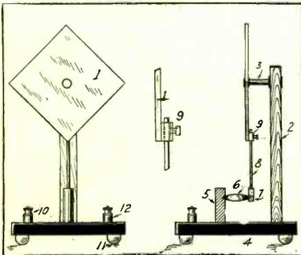
Experimental Microphone Capable of Being Made Extremely Sensitive. Utilizes a Sound Detecting Diaphragm Made of Wood.
