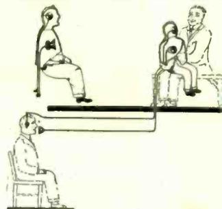
up telephone transmitters and receivers to a small dummy figure such as used by a ventriloquist on the stage. The operator speaks to the dummy and his words are carried by the microphone circuit in the dummy's head down to an assistant below the stage. The assistant can then (apparently) cause the dummy to speak by talking into the microphone in front of him, the speech being reproduced by the loud speaking telephone receiver in the breast of the dummy.
