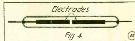
Oscilloscope Tube in Which Spark Must Take Place to Obtain Results Shown in Fig. 5.
