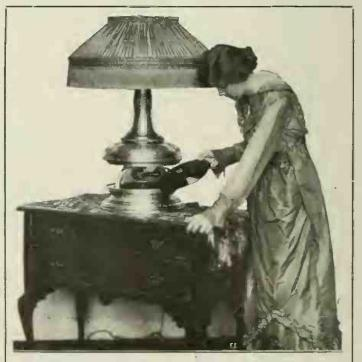
Behold! the Electric Table Lamp That Speaks and Sings— Thanks to a Phonograph Cleverly Concealed in the Base and Oriven by a Miniature Electric Motor.
