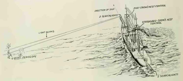
Fig 1. Keeping Very Powerful Searchlights Trained On the U-Boat Periscope, Makes It Impossible for Its Commander to Take the Attacked Ship's Bearings. The Searchlights Are Used in Broad Daylight. Now See Fig. 2.
