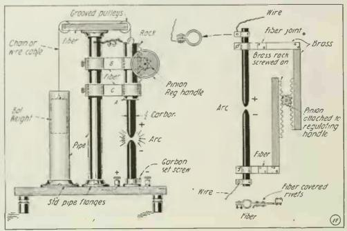
Fig. 2.—Hand Feed Types of Arc Lamp Which Lend Themselves Readily to the Constructional Skill of the Amateur Electrician.
