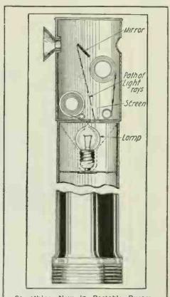
Something New In Portable Pyrometers. This Model, which May Be Held in the Hand. Compares the Luminous Valve of the Hot Body with That of an illuminated Tinted Film.
