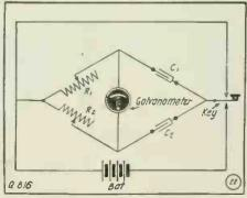
Showing How the Bridge Method is Applied for Measuring Condenser Capacities.
