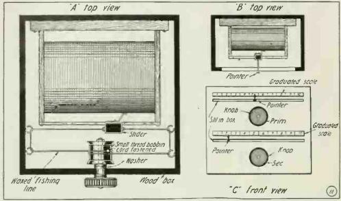
Now Is a Good Time in Which to Re-design Your Radio Apparatus. Here's a Fine Idea for Converting Your Old Tuning Coll Into a "Cabinet" Style Set. By Changing Around the Connections a Number of Effective Tuning Arrangements May Be Had.
