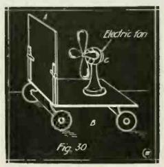
Illustrating "Action" and "Reactioh." With Board "A" Removed the Fan Propels the Wagon; With "A" in Place the Wagon Stands Still.
