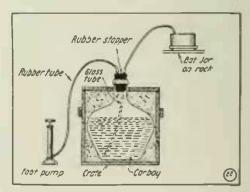
Method Whereby Battery Electrolyte Can Be Pumped by Comprest Air from Carboys Into Cells.
