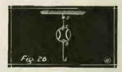
By Means of Thumb-Tacks, a Baseball Is Suspended as Shown. Pulling Suddenly on Thread at "A", it Breaks Between "A" and Pin "B": Pulling Slowly the Thread Parts Between "C" and "D".
