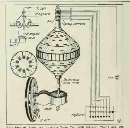
This Electric Spun and Variable Tune Top Will Interest Young and Old Alike. A Set of Keys Control Electric Circuits Actuating the Various Tone Reeds Within the Revolving Top.
