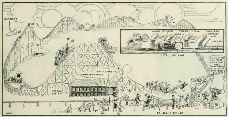
Here's Your Chance, "Electrical Bugs," to Become Internationally Famous. Design a Perpetual Motion Scenic Railway Like That Shown; the Descending Cars Pump Electrical Energy Back Into the Storage Battery; the Ascending Cars Are Helped Over the Peaks by Current from the Battery. For the Best 100 Words Explaining Why This Device Will or Will Not Keep Going For Years, Ignoring Wear and Tear, We Will Give a Year's Subscription to the "E. E."
