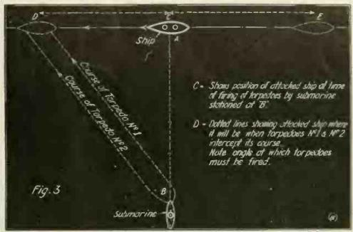
To Torpedo a Ship the Submarine Commander Must Know These 3 Things: 1st, Distance from A to B in Yards; 2nd, Speed of Ship, i.e., How Long It will Take to Travel from C to D; 3rd, Direction in Which Ship is Moving, i.e., Does it Travel from C to D or from C to E?
