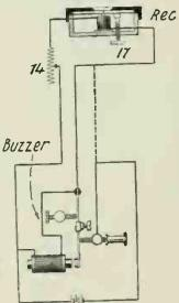
The apparatus in question consists of a telephone receiver connected with a circuit comprising a battery and a rapidly interrupted switch or contact, such as a buzzer.
