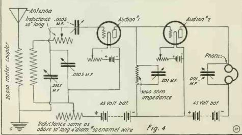
Detailed Circuit Diagram for Two-Audion Continuous Wave Radio Receptor Operating On the "Heterodyne" Principle.
