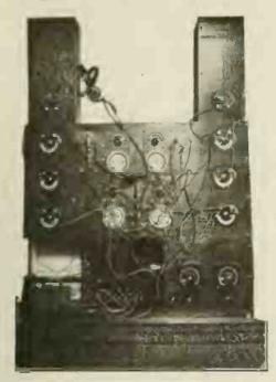
The Complete 20.000 Meter Audion Receptor for Undamped Waves, With Loading Inductances and Large Loose Coupler.
