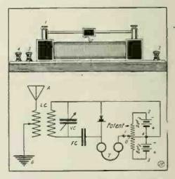
By Means of the Duplex Potentlometer Scheme Shown, It is Possible to Quickly Reverse the Battery Current Thru the Detector or Other Device.
