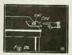
A Simple Example of "Inertia." If the Card Is Snapt by the Finger it Will Fly Off, the Coin Dropping Directly Underneath Its Previous Position.
