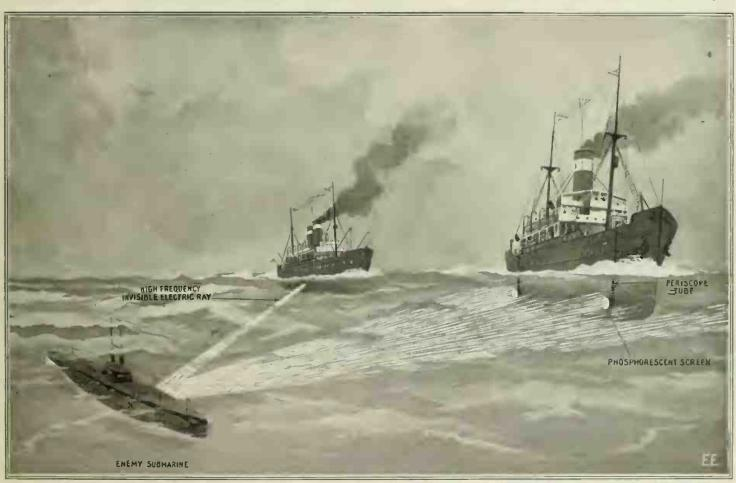
Nikola Tesia, the Famous Electric Inventor, Has Proposed Three Different Electrical Schemes for Locating Submerged Submarines. The Reflected Electric Ray Method is illustrated Above; the High-Frequency invisible Electric Ray, When Reflected by a Submarine Hull, Causes Phosphorescent Screens on Another or Even the Same Ship to Glow, Giving Warning That the U-boats Are Near.
