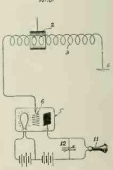
ductance coil is connected to the grid of vacuum bulb detector used in the manner shown, or a crystal detector may be used instead. It is seen that 'electrostatic coupling is thus employed and in tuning such a receiving set metal ring 2, is moved along coil 3, and also the degree of coupling may be varied by contracting or expanding ring 2.
