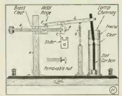
Fig. 1.—A Swinging Carbon Type of Arc Lamp for Amateurs.
