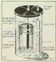
Finally the Gravity Cell Research Work Bolled Down to the Type Shown. The Copper Sulfate Oozed Out By Capillarity Thru Several Layers of Burlap Dipping in Both Solutions.
