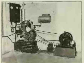
Complete Independent 400-Watt Electric Generating Which is Available for Supplying the Miniature City Shown Above with the Necessary Current.
