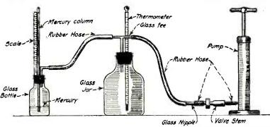
An Inexpensive Vacuum Pump Can Be Easily Made from a Single Cylinder Tire Pump, as Shown in the Accompanying Illustration. With Experimental Apparatus, Water Can Be Made to Boil at a Temperature of 1700 Degrees, Fahrenheit.
