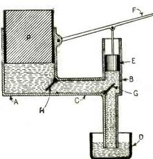
A Simplified Diagram Showing How a Hydraulic Press Operates Is Given Here. A Complete Description Is Given in the Text. If the Cross-Sectional Area of E Is 10 and That of P Is 100, the Piston P Will Move Only One-Tenth as Far as E.
