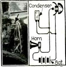
A Telephone Condenser Shunted Across the Horn Button Wires Saves Burning the Contacts.
