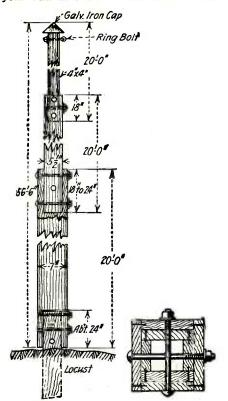
pole is made with 34 inch boards cut to the proper width. The top piece is solid, 4 inches by 4 inches tapered down to about 3 inches at the very peak. Each connecting section is bolted together with three wagon bolts.
