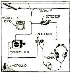
A Simple Crystal Detector Circuit Using a Variom-eter and a Variable Condenser for Tuning, 1s Given Above.
