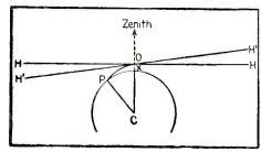
The Dip of the Sea Horizon: X Is the Height of the Observer, in Feet, Above Sea-Level. HH is the True Horizon of the Observer at O, Which Is at Right Angles to the Direction of the Plumb-Line. PO Is the Path of the Line of Sight to an Object, P, the Most Distant Point on the Earth's Surface Visible from O; the Line is Curved on Account of Refraction, Which Is Greatest at Sea-Level. The Observer at O Sees P in the Direction OH¹, Owing to the Effects of Refraction.
