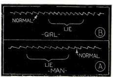
Actual Records Taken in the Editorial Offices to Determine the Possibilities of Detecting Lies by Meaus of a Sphygmomanometer and the Sphygmograph. A Rise in Blood Pressure of 6 to 8 Millimeters Was Quite Evident
