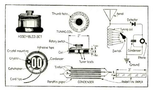
Diagram Above Shows Constructional Details and Wiring Diagram of Pocket Radiophone Receiving Set.
