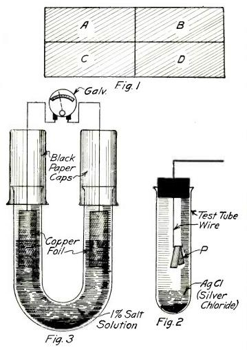
Fig. 1. A shallow Photo-Developing Tray Can Be Used to Show Photochemical Extinction. Fig. 2. Silver Chloride Blackens on Exposure to Light, the Blackening Being Approximately Proportional to the Intensity of the Light. Fig. 3. Using This Simple Cell, Light Produces a Chemical Reaction, and the Chemical Reaction Causes an Electric Current to Be Set Up.
