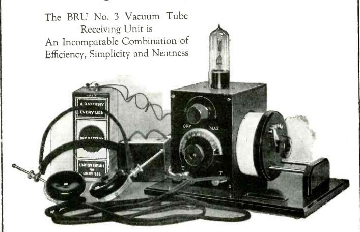
The BRU No. 3 Vacuum Tube Receiving Unit is designed to operate on ONE DRY CELL for filament current ("A" Battery).
