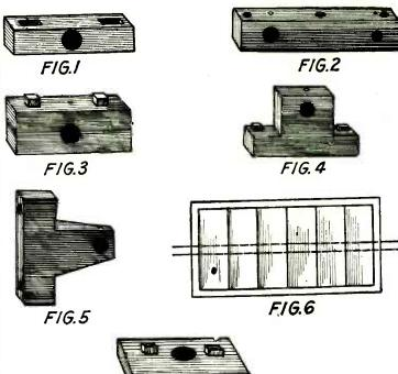
cept that Fig. 5 is intended for vertical work, where the shafts must be fastened to the wall. Fig. 7, which is suited to vertical work, can also be used for horizontal purposes.
