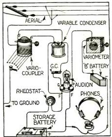
A Simple Form of Short Wave Regenerative Tuner Is Shown Hexewith, Employing a Single Variometer to Tune the Plate Circuit.
