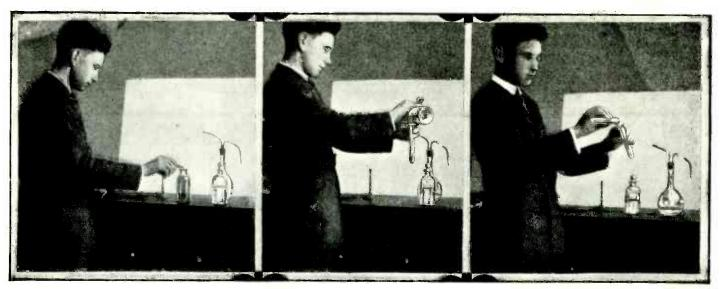
Left—Making the Starch Test for Iodine by Pouring the Iodine Solution into Very Thin Starch Paste and Obtaining a Blue Color. Center—Making the Brown Ring Test for a Nitrate. The Test Is Quite Sensitive and the Ring Clearly Defined. Right—Testing for Iron Salts. All of the Tests Here Shown Are Quite Simple.
