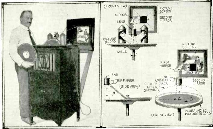
The Newest Movie-Phonograph Is Illustrated Above With Its Inventor, Mr. C. Francis Jenkins, of Washington, D. C. The Diagrams at the Right Show How the Reflected Light From Two Small Lamps Is Caused to Reflect the Image Up Through the Objective Lens or to the First Mirror, Thence on to a Second Mirror and From That on to the Screen, Which Is Placed in the Top of the Phonograph Cabinet Lid. No Celluloid Film Is Used, the Pictures Being Printed on Paper, Any Fire Hazard Thereby Being Obviated.
