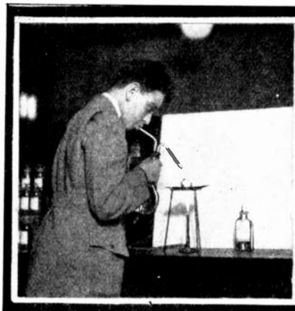
Slaking a sample of quicklime.
