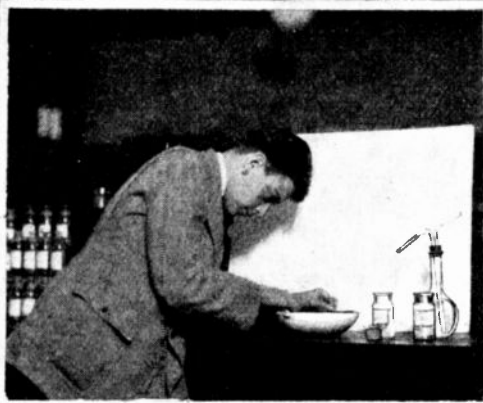
Testing soil with litmus paper, to determine whether it is acid or alkaline.
