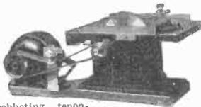
Does your ripping, mitring, grooving, rabbeting, tenoning, sanding, grinding and many other operations with surprising ease and accuracy. Top 10"x13" Saws 1 1/2" stock. Dadoes 5/8"x5/8". Machine built entirely of metal. Driven by 1/4 or 1/3 h. p. motor. Portable. Attaches to any light socket. Extremely accurate.
