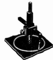
Especially designed for the Radio Constructor. Made of the finest material and equipped with the highest grade high steel cutting bits. It does three things at once. It drills its own pilot, cuts out plug and puts bead or scroll around the hole in one operation. Cuts holes 3/4 to 4 in. in diam. PRICE—No. 402.....\$3.00
