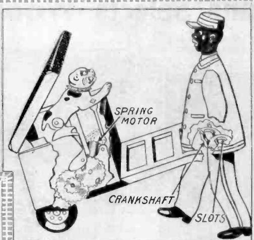
The photo and diagram at the left shows a mechanically operated porter pushing a trunk. As he moves along the floor, the cover of the trunk opens up and a dog seemingly growls at the porter, who hurries along with his burden. The mechanism is only applied to the wheels of the carrier, and yet one wonders at the remarkable way in which the porter walks along the floor. This is made possible through the ingenious crank movement to which the legs of the porter are fixed.
