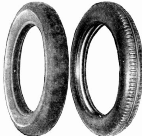
Two photos above show same tire before (left) being treated and after (right) new tread has been fused on to old tire. At a cost of about one-third the original price, tire is renewed and good for at least 75% of its original mileage.
