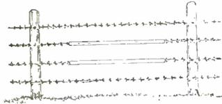
When it becomes necessary to negotiate a barbed wire fence, and one desires to avoid the expense of a gate, it is a good plan to adopt this hint.
