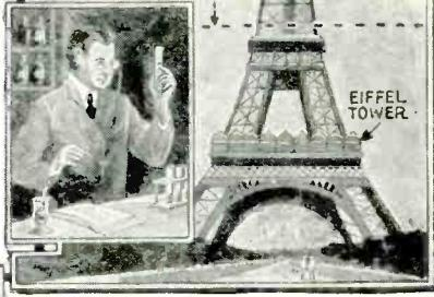
Using the various platforms of the Eiffel Tower as points for experimentation, officials of the Municipal Laboratory of Toxicology tested the odors of Paris, by exposing test tubes containing various chemicals effectual for the purpose, to the action of the atmosphere at various levels.
