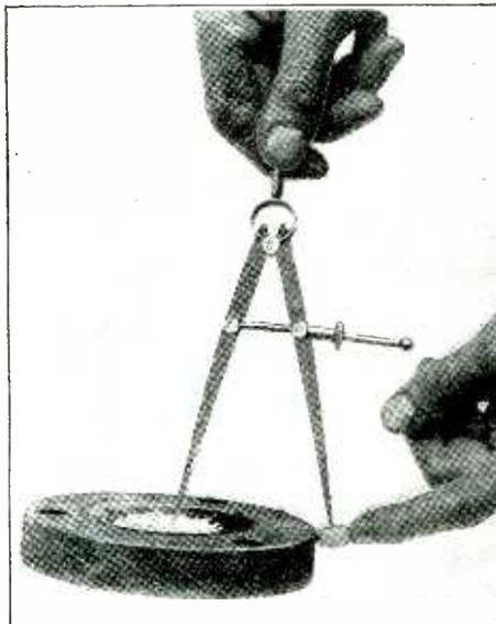
Large dividers can be made into good hermaphrodites as shown in the above photo. The end of an ordinary clothespin is stuck on one point and it gives the free point a better chance of hitting the same arc each time it is located at a different point for scribing.—Frank W. Bentley, Jr.
