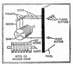
Buttons are used in the automatic arrangement shown above. One button is used for each station.
