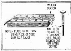
A guide block on which to place the two film ends to be spliced, is shown above.
