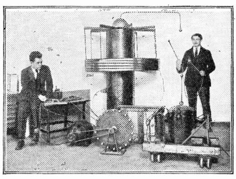
Above is a photograph of the completed Tesla coil, transformer, condenser, and rotary spark gap. The transformer may be seen placed upon the movable truck with the condenser just to the left.
