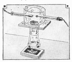
The manner in which the X-ray photographs are taken is illustrated above. The objects are placed in a holder above the sensitized plate.
