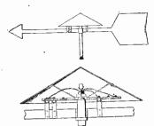
No. 1,670,488 issued to Hiram B. Whitcomb. With this device installed in a building the direction of the wind can be ascertained without viewing a weathervane, the direction being indicated by a small electric lamp on a dial inscribed with the points of the compass.
