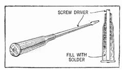
A simple and ornamental handle for small tools can be made from a brass cartridge. A wooden plug inserted in one end allows the shank of the tool to be inserted. Another way to hold the tool is to insert the shank and fill the opening with solder. The handle can be punched and polished if desired.—
