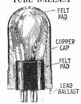
The tube ballast and the manner in which it is used is shown above. Felt pads prevent vibration of the device.
