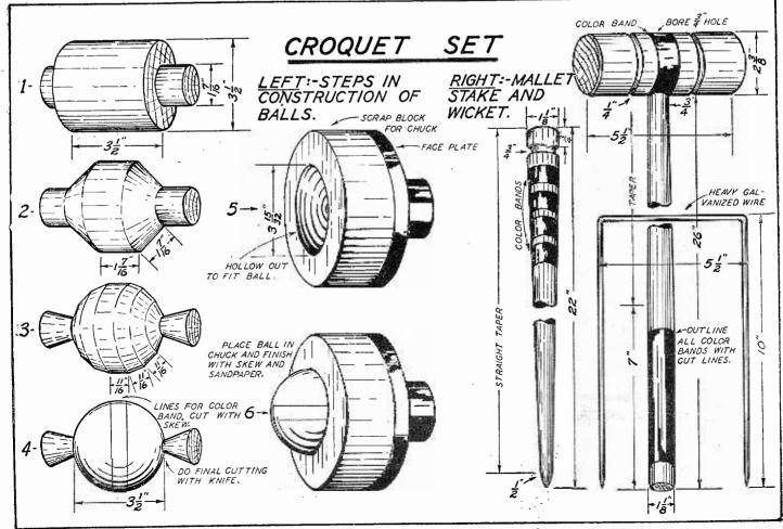
The above diagram illustrates the various steps which the amateur will take for making the mallets and constructing the balls. Observe that a in the construction of a croquet set. All of the dimensions are here given a set in the balls is made from a set ap block affixed to the face plate.
