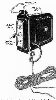
The loud speaker unit illustrated above can be used with almost any surface capable of vibrating.
