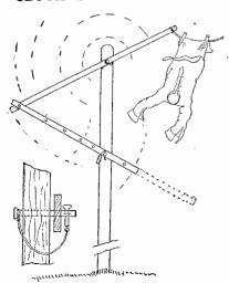
The ordinary clothesline is rather inconvenient in that it is often too high or too low for the particular article to be dried. However, by means of the simple device shown here it can easily be raised or lowered. A lever is cut from hard wood, pivoted as shown, with one end attached to a piece of strapiron. This allows the line to be raised or lowered.—S: Leonard Bastin.
