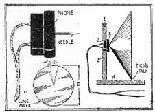
Details for the paper cone are also given. It should be about 10" in diameter. Sealing wax is melted and dropped into the apex of the cone. Next, the needle on the diaphragm is heated and pushed into the sealing wax. The cone is mounted upon a wooden stand. In the illustration 1 is a set screw, 2, hole for holding phone; 3, upright support; 4, baseboard. A thumb tack placed at the bottom of the cone assists in holding it in place.—Arnold Rankin.
