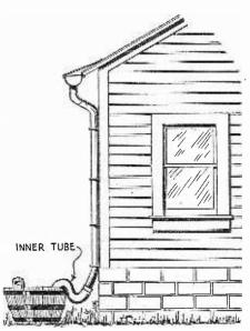
When it is inconvenient or impossible to use the present drain pipe, a piece of old inner tube can be utilized in the manner illustrated here. One end of the tube is simply slipped over the drain pipe and the other end is placed in a large tub.—C. N. Penington.
