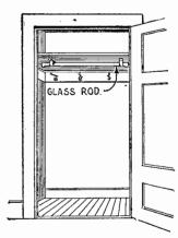
The capacity of a clothes closet can be doubled by installing a glass rod such as those used for towel racks. This rod is simply fastened to the closet shelf me an sof screws passing through the rod supports. this arrangement provides plenty of room so that the hangers can be placed at right angles to the walls of the closet.
