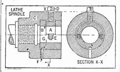
A lathe chuck for short round pieces of work can be made from cast iron fitted to the spindle of the lathe. A and B are the bushings, E coil springs, F pin, and G is a short keyway. Several size bushings can be made and used in a chuck of this kind.—F. N. Coakley.
