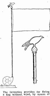
The invention provides for flying a flag without wind, by means of an artificial draft, and also provides illumination for the flag at night. C. A. Lapworth: No. 1,660,341.
