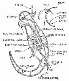
A sectional view of the parrot speaker is shown in the above illustration. Details of the door are also given.
