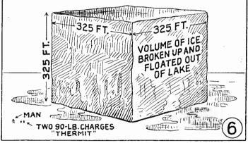
In a big ice jam at Ogdensburg, N. Y., two ninety-pound charges of thermit succeeded in breaking up a million tons of ice, which floated out of the lake.
