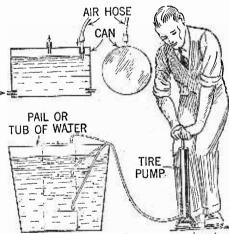
The above illustration shows an experiment which can be carried out to illustrate the principle of raising sunken ships with compressed air. A can fitted with check valves immersed in a pail of water has a hose connection with a tire pump. The can may be filled with air and will float.
