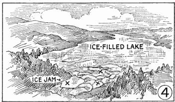
In many cases an ice jam occurs at the outlet of a lake, and the points marked X show where thermit charges may be placed to loosen the jam.
