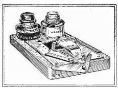
A manufactured type of 16 mm., film splicer and cutter is illustrated herewith.
