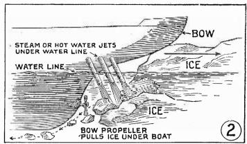
Bow propellers have been found useful on Canadian ice-breakers to move the broken ice sternward. In some cases steam and hot water jets are also employed.
