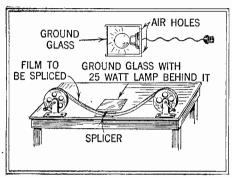
An electric bulb placed behind a ground glass screen proves useful in examining the film.
