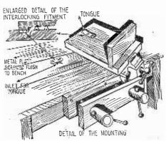
A small metal plate is next made flush with the bench top, as shown above. A metal tongue is fastened to the vise board and fits into a hole in the metal plate.—J. E. Lovett.
