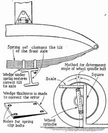
A car which gives unsatisfactory results due to wheel wobble can be readily fixed by using the above method. Small wedges gives the correct tilt to the front axle. The measure of the tilt is made with a square and a scale.
