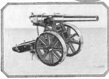
This neat and trim little model can be constructed quite easily by following all the instructions given on the blueprint on the accompanying page. In this model the gear used to elevate the gun was obtained from a mandolin. In the actual construction bevel gears are employed in the place of the rig here indicated.
