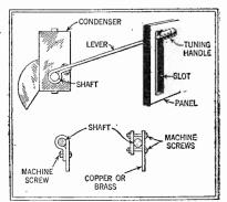
One of the simplest ways in which to obtain automatic tuning is illustrated above. The lever is set to the desired station indicated next to the slot.
