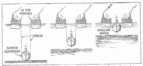
The above illustration shows the method pursued in raising the twenty-five one-thousand ton destroyers. The two halves of the submergible testing dock were fitted with ten ton winches. From these cables passed down to the sunken destroyer, which was raised and towed to shallow water.
