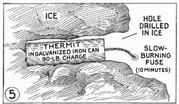
Above we see how a ninety-pound charge of thermit in its galvanized iron can is placed in a hole cut or drilled in an iceberg. Note the fuse.
