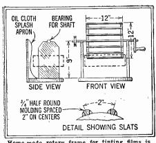
Home-made rotary frame for tinting films is shown above. A pan to hold a solution is shown in dotted line. Details are given at left.
