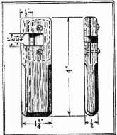
A knife for c u t t i n g t w i n e or string which can be carried in the pocket without danger is illustrated at the left. A safety razor blade is used for the cutting edge. A piece of hard wood is drilled and cut, as shown. The blade fits in a slot and
