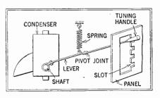
The illustration at the left shows a method which can be employed for tuning the set automatically. Only one lever is used for selecting stations, that is, on single dial sets. Multi-dial receivers will have the same number of levers as there are dials, the tuning lever simply replacing the dial.
