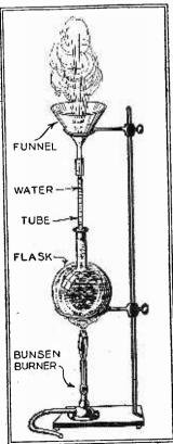
The above illustration shows how a small geyser can be made in the laboratory. The experiment can be carried out simply with the aid of a funnel, a flask and a piece of tubing.
