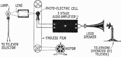
The above illustration shows how the Televox talks. Light rays pass through the film and strike a photo-electric cell.
