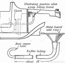
Wet clutches can be flushed and reciled casily by employing the method illustrated above. In flushing the clutch, it is desirable to use at least a quart of kerosene.
