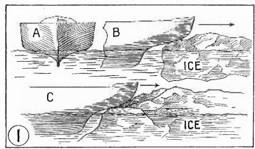
Boats used for "ice-breaking" are specially constructed; cross section shape preferred at A; B shows shape of bow, and C shows later stage.
