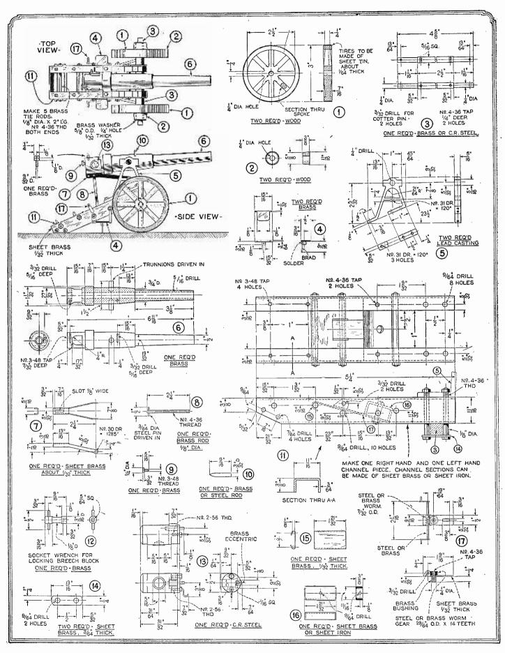
The above diagram gives the full details for the construction of the cannon which won the cup in the Model Contest for this month. Practically the
