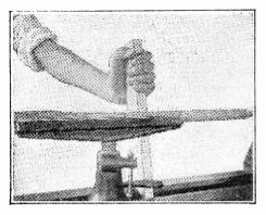
Get someone to help in turning the handle, by holding a wooden brace lightly against the work as it revolves.
