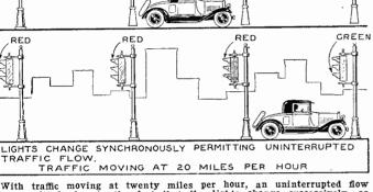
With traffic moving at twenty miles per hour, an uninterrupted flow is permitted, due to the fact that the lights change successively, as illustrated above.
