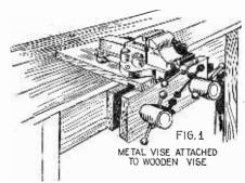
It frequently happens that the need for a metal vise arises and in order to conserve space it can be mounted on a wooden vise, as shown above in Fig. 1. The metal vise is first mounted on a piece of board. The screws which hold the vise to this board also pass through a board at right angles to the mounting board. The former is clamped between the wood vise, as shown.
