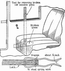
When a window of an automobile breaks, some pieces of the glass fall into the window aperture. A simple and serviceable tool for removing the glass from a car body is illustrated above. It consists of a lath, to which spring steel wire is attached with staples. The wire is pushed over the glass and will hold it tightly, permitting the fragment to be removed.
