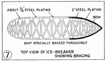
now ice-breaker ships are built, the bow being reenforced with two-inch armor steel. The inside of the hull is strongly cross-braced with steel girders.
