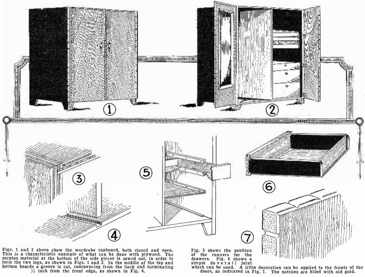
Figs. 1 and 2 above show the wardrobe cupboard, both closed and open. This is a characteristic example of what can be done with plywood. The surplus material at the bottom of the side pieces is sawed out, in order to form the two legs, as shown in Figs. 1 and 2. In the middle of the top and bottom boards a groove is cut, commencing from the back and terminating 1/2 inch from the front edge, as shown in Fig. 4.
