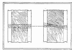
The straight film splice is shown at left; the stronger diagonal splice appears at the right.
