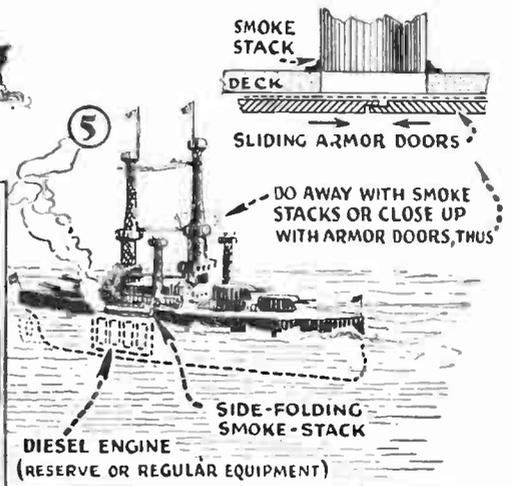
An aerial bomber flying low and with good luck could occasionally place a bomb in the smoke stack of a battleship with the result that the boilers and propelling mechanism would be completely destroyed. This is illustrated below and a suggestion for remedying the situation given above. With stacks closed, Diesel engines could be used.
