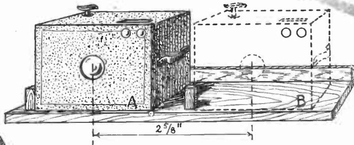
The diagram at the left shows how stereoscopic pictures may be taken with one camera.
