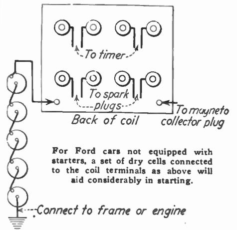
For Ford cars not equipped with starters, a set of dry cells connected to the coil terminals as above will aid considerably in starting.
