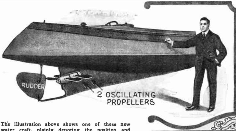
The illustration above shows one of these new water craft, plainly denoting the position and appearance of the two oscillating propellers which are capable of not only propelling the boat forward, but also of operating it in a reverse direction.
