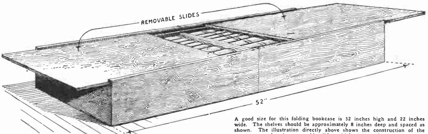
A good size for this folding bookcase is 52 inches high and 22 inches wide. The shelves should be approximately 8 inches deep and spaced as shown. The illustration directly above shows the construction of the grooves for the removable slides which protect the contents.
