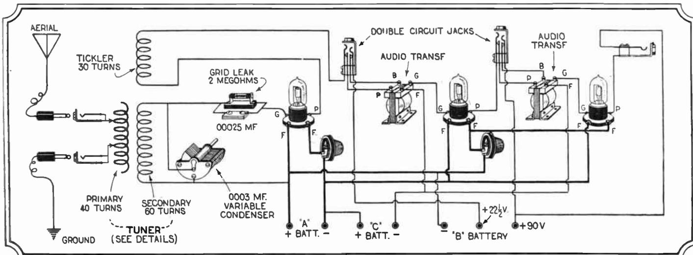
Five jacks, one each for the aerial and ground, detector and first and second stages of amplification afford very handy connection terminals. The antenna is a coil of bell wire 125 feet long which, when not in use, is placed in the
