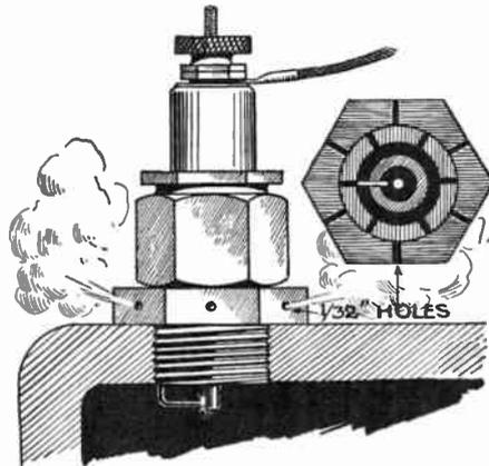
If holes are drilled in the shell of a spark plug as well as in a nut which fits the shank of the plug, carbon may be quickly removed from the porcelain by turning the nut so that the holes line up and running the engine for a few minutes. When in ordinary use the holes must be turned out of line. —M. Mather.
