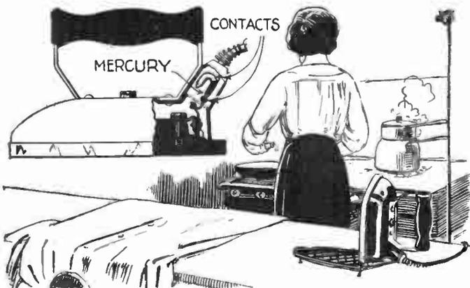
No. 1,511,382, issued to Dayton Ulrey and Daniel I. Mayne, covers several designs of fluid circuit breakers, the most basic of which is illustrated above. A conducting fluid, preferably mercury, completes the circuit when the electric iron is horizontal. The circuit is broken when the iron is tilted and so prevents overheating and waste of power.
