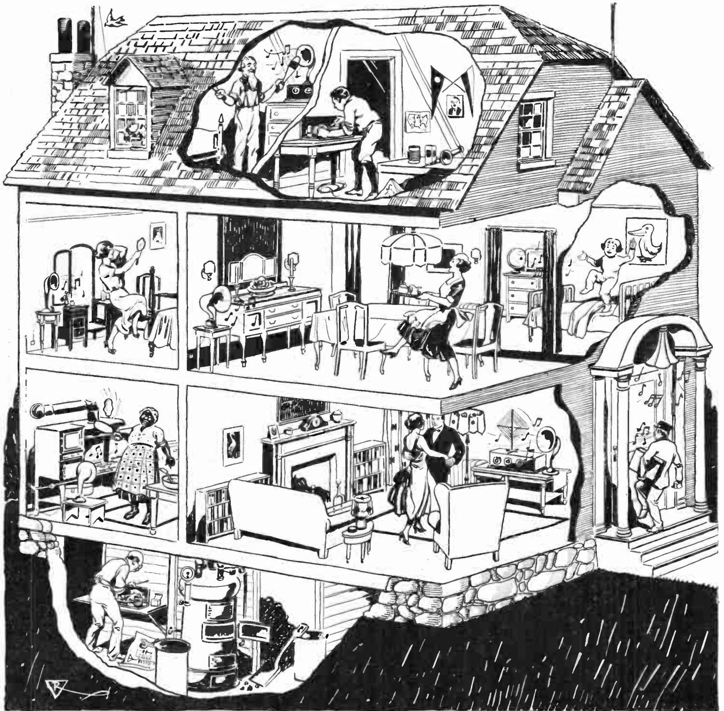
The loud speaker system installed in this house is quite easy to duplicate. A pair of wires run through all rooms where a loud speaker is wanted. The loud speaker is then plugged in at will by the use of a jack and plug system.
