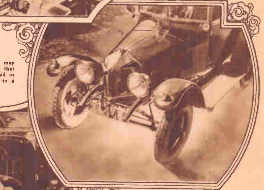
A new system of anti-glare motor car lighting has been devised by an English inventor, A. Kelway Ramber, and is said to be most effective. The device consists of five lenses placed under the body of the car through which the strong rays of a lamp are directed which light serves to illuminate the ground under and around the car, throwing it into relief.
