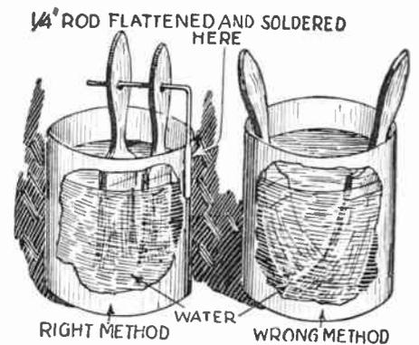
When paint brushes are left standing in water as at the right, the bristles are pressed out of shape. If, however, holes are drilled in the handles, the brushes may be protected by the water and the bristles kept straight by suspending from a rod as shown.—F. J. Wilhelm.
