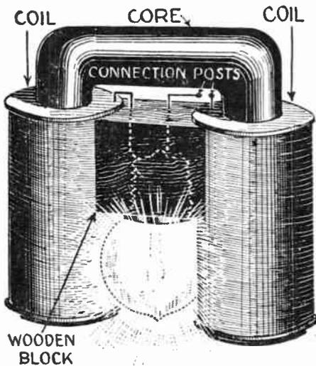
A handy trouble lamp for use around an automobile is made as shown above. The magnets will hold the lamp in any position, while the current is on and if the unit should become detached and fall, the magnets protect the lamp.
