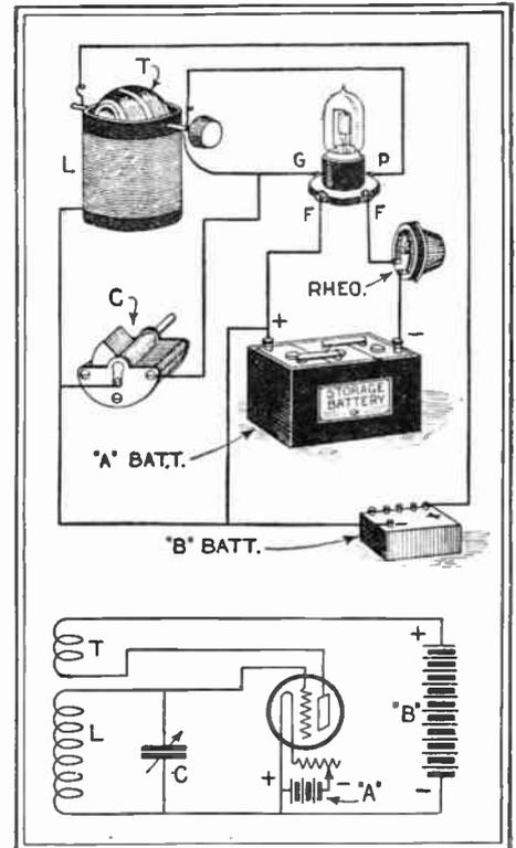
Herewith is shown a fundamental oscillatory circuit.
