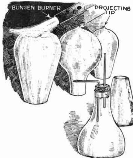
Handy flasks may be made from various types of electric light bulbs. The brass base is cut off and the edges of the glass rounded. If flame is then applied to the opposite end, the glass will be depressed so as to form a base.
