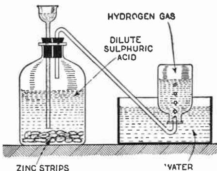
This shows a laboratory set up for the preparation of hydrogen gas.
