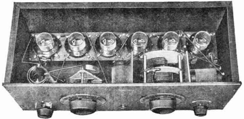
Note the interior of this well designed set. All parts are separated so as to eliminate to a greater extent the feed-back which would otherwise occur. The condenser to the right is a special type, and as can be seen, is well shielded. The audio frequency transformers are also shielded and placed under the tube rack toward the back of the cabinet. By the use of the best type of transformer, distortion in the audio circuit is eliminated.
