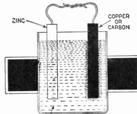
The simplest form of galvanic battery consists of a carbon or copper rod and a zinc plate immersed in dilute sulphuric acid.
