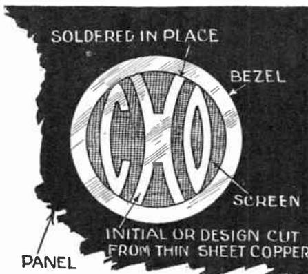
A design of the radio owner's initials cut from thin sheet copper and attached in the bezel in the receiving set, lends individuality to an otherwise common-place set.
