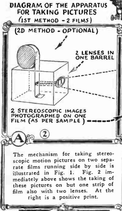
The mechanism for taking stereoscopic motion pictures on two separate films running side by side is illustrated in Fig. 1. Fig. 2 immediately above shows the taking of these pictures on but one strip of film also with two lenses. At the right is a positive print.
