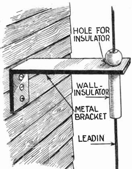
A handy stand-off insulator may be made by setting a wall insulator in the end of a metal bracket.
