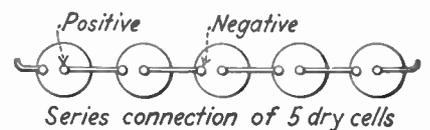
The correct connections for a series of five dry cells are illustrated above.
