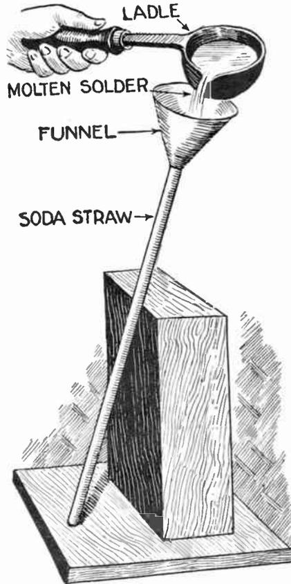
Usually after wiring up a set there is a considerable amount of solder left over. Melt the solder in a ladle and pour the molten solder into a soda fountain straw. By removing the straw after the solder has solidified or "set" a handy length will result.
