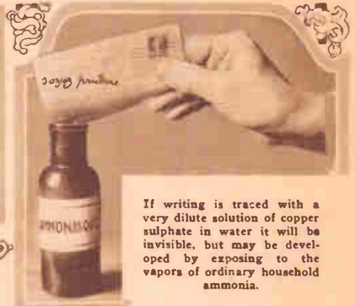
If writing is traced with a very dilute solution of copper sulphate in water it will be invisible, but may be developed by exposing to the vapors of ordinary household ammonia.
