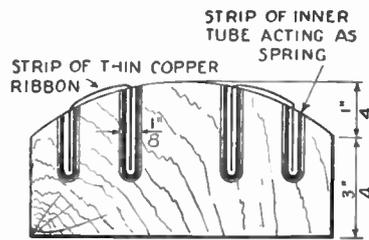
A miniature phone block which will accommodate 11 pair of phones, seven in series and four in parallel, is a very handy device which can easily be constructed upon the dimensions given in the diagram. A small block of wood is drilled and fitted with short lengths of thin copper strip. A piece of rubber tubing acts as a spring, effecting good contact. A fibre cover is screwed to the top, giving a pleasing appearance.
