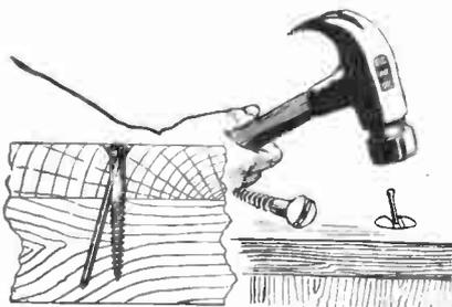
No. 1,518,119, issued to Warren C. Rees, covers the design of wood screw which is to be locked in position by means of a nail as illustrated above. It is impossible for a screw of this nature to loosen.
