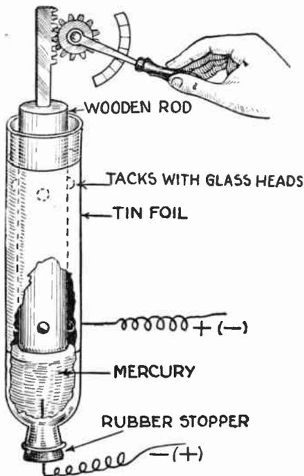
Take the bottom off a long, narrow bottle. Cork the bottle up tightly and force a stout copper wire through the cork. Coat the outside of the bottle with tin-foil. Pour mercury almost up to the height of the tin-foil. The device is operated by a handle which presses the plunger down and thereby raises the mercury in the bottle.
