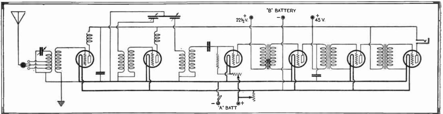
One might wonder at the above circuit diagram which shows two steps of radio frequency, detector and three steps of audio frequency amplification. In a few words, it was possible to add the third stage of audio because of the exceptionally good engineering design involved. Large by-pass condensers must of course, be employed in this circuit in order to readily by-pass the radio frequency currents.
