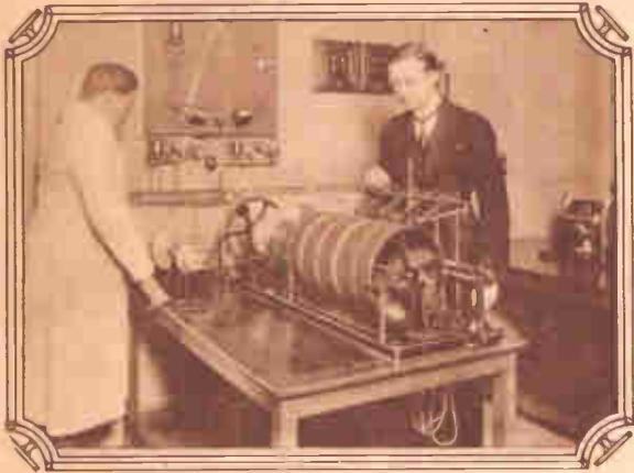
The photo directly above shows the chart room in which the registering apparatus for various tests is installed. Charts, curves or graphs are obtained for the many varieties of tests and observations to be made. A cylindrical recording device is being inspected.
