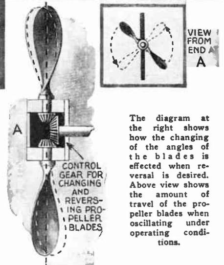
The diagram at the right shows how the changing of the angles of the blades is effected when reversal is desired. Above view shows the amount of travel of the propeller blades when oscillating under operating conditions.
