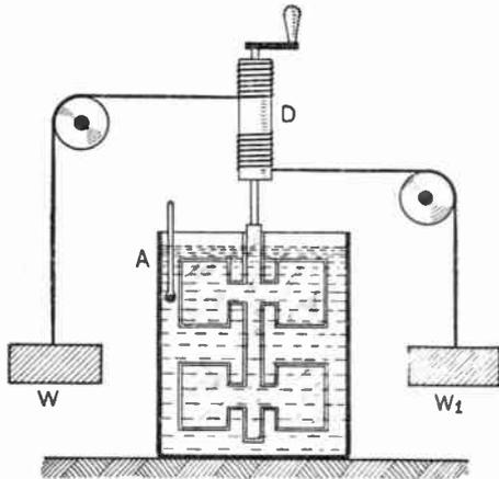
The simplest method for the determination of the mechanical equivalent of heat is shown above.
