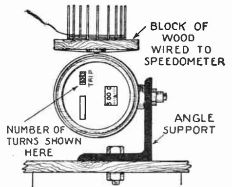
It is best to mount the recorder on the workbench in a convenient corner. Its simplicity is clearly indicated in the above drawing. Much faster work can be done with it than by merely counting.
