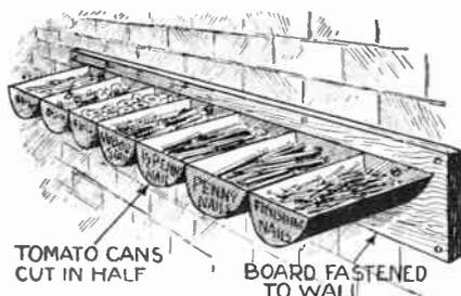
A rack for holding various small parts around the shop may be made from several tomato cans cut in half and mounted as shown above.
