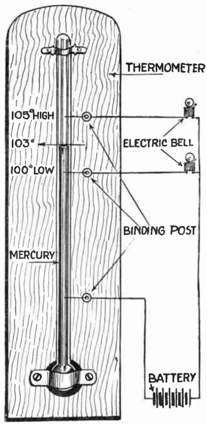
Heating alarms of the type illustrated above are by no means new and furthermore are not as efficient or as cheap to manufacture as thermostats. It is therefore not advisable to patent a device of this nature.
