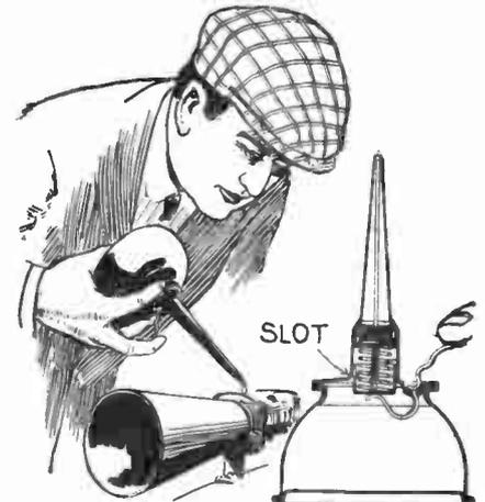
No. 1,520,829, issued to Gustave Lidseen, covers a type of oil can which cannot spill even though upset. Furthermore, a measuring device is incorporated which, if desired, allows only a certain amount of liquid to escape. Both the measuring and the sealing devices are actuated by a finger lever as indicated above.
