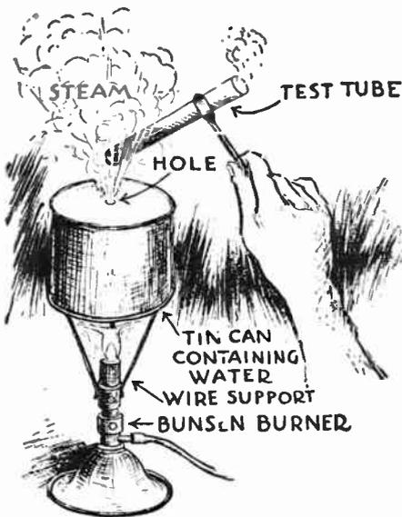
When materials in a test tube have to be carefully heated, the device illustrated above comes in very handy. A small tin can is fitted with a wire support and held above a Bunsen burner. Water is poured into the tin can and the cover, with a hole punched therein, placed in position. Heating the water soon evolves steam which in turn may be used to heat the test tube.
