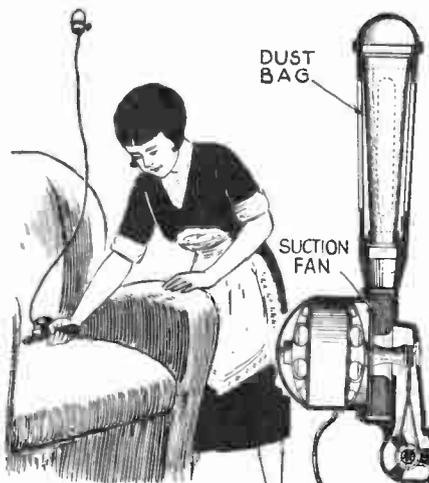
No. 1,596,231, issued to Frank W. Finkhausen, describes a novel type of portable vacuum cleaner which is entirely self-contained. Above at the right is shown a cross sectional view of this device. A small dust bag is incorporated in the handle. An electric motor operating from the house current turns a fan which in turn is belted to a small brush as shown.
