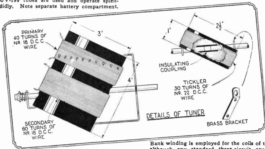
Bank winding is employed for the coils of the tuner, although any standard three-circuit coupler can be used.
