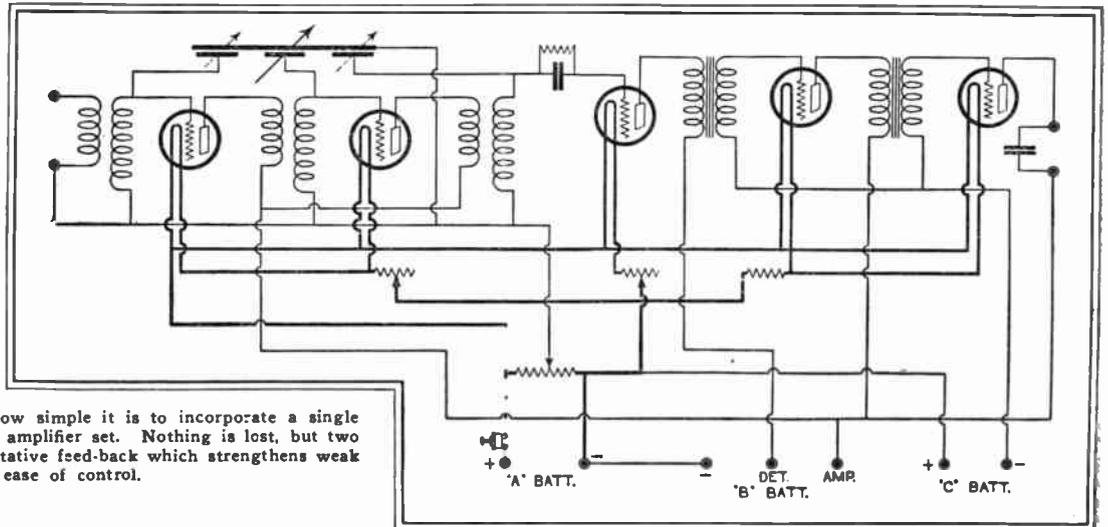
The diagram to the right shows how simple it is to incorporate a single tuning control in a radio frequency amplifier set. Nothing is lost, but two main advantages are gained—capacitive feed-back which strengthens weak signals and ease of control.
