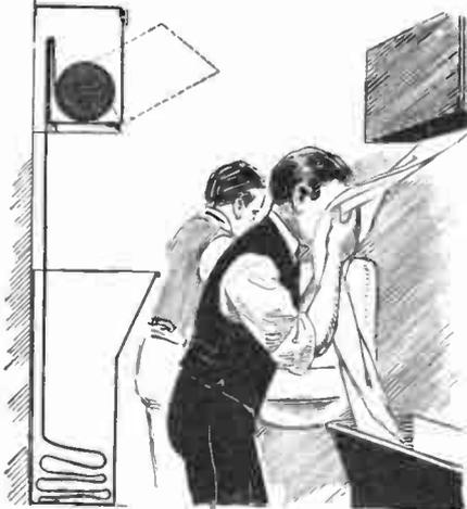
No. 1,514,400, issued to Frank M. Steiner, describes an improved type of towel holder for washrooms, wherein the same section of the toweling is used only once. A roll of absorbent cloth is kept in the hinged cabinet as illustrated above and when a clean section is desired, it is pulled down and the remainder allowed to collect as shown.
