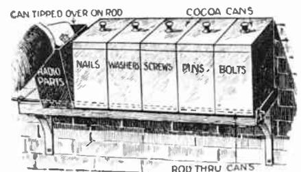
Another rack for various parts may be made of large cocoa cans placed on a shelf which does not extend quite to the edge of the can. A rod passed through them serves as a pivot.
