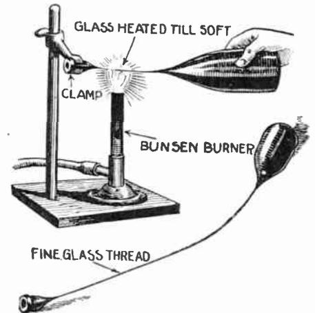
Fine glass threads are often required in various experiments. They may be quickly and easily made as illustrated above. Clamp the neck of a bottle in position and then heat the point shown. When the glass is softened, throw the bottle as far away as possible. A long fine glass thread will result.
