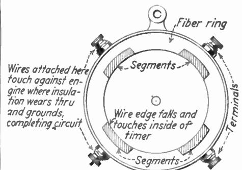
Other ignition troubles often occur at the commutator illustrated above. The wires connected to the terminal may become frayed and so short circuit to the commutator housing or the engine frame. Also the segment may become badly worn, whereupon a new timer should be installed.
