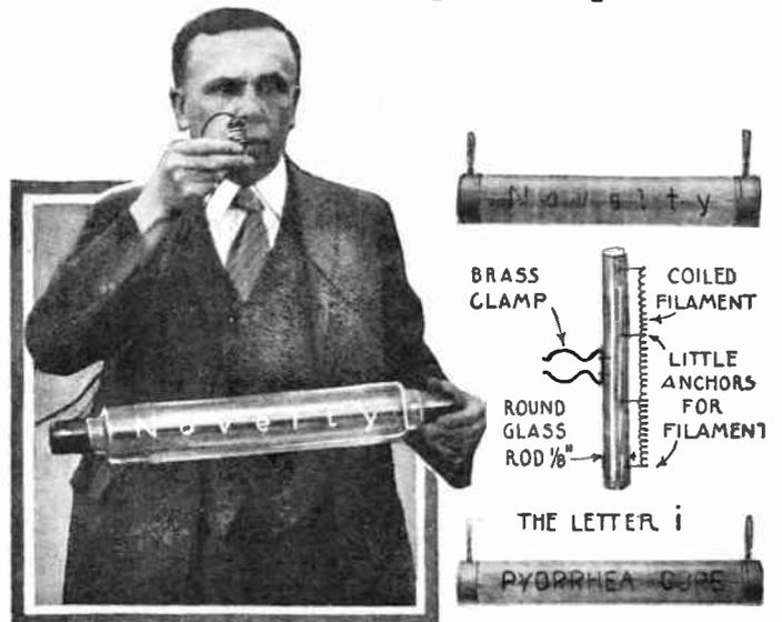
The novelty lamp illustrated above is the invention of Mr. H. Hartman. Upon a glass rod running from one end of the lamp to the other, a number of letters are clamped. These letters are of glass and contain little anchors which hold the filament. Three or four letters are connected in series and the groups then connected in parallel to the line wires. These are placed in the glass tube, which is then evacuated.
