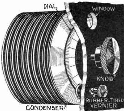
A novel effect is obtained when a dial is mounted in back of a panel. The dial numbers are viewed through a "window" drilled through the panel.
