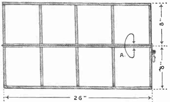
Above is shown a cross sectional view of this bookcase when folded for shipment. The removal slides indicated by A, amply protect the contents and prevent the books from becoming mixed up during moving.
