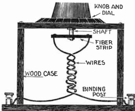
The device shown is an effective vernier condenser. Two wires, preferably twisted lamp-cord, are connected to binding posts on the base and are twisted together by a fibre strip mounted on the shaft of the dial. The wire should be about four to six inches long. By turning the knob, the wires are twisted together, thereby changing the capacity.
