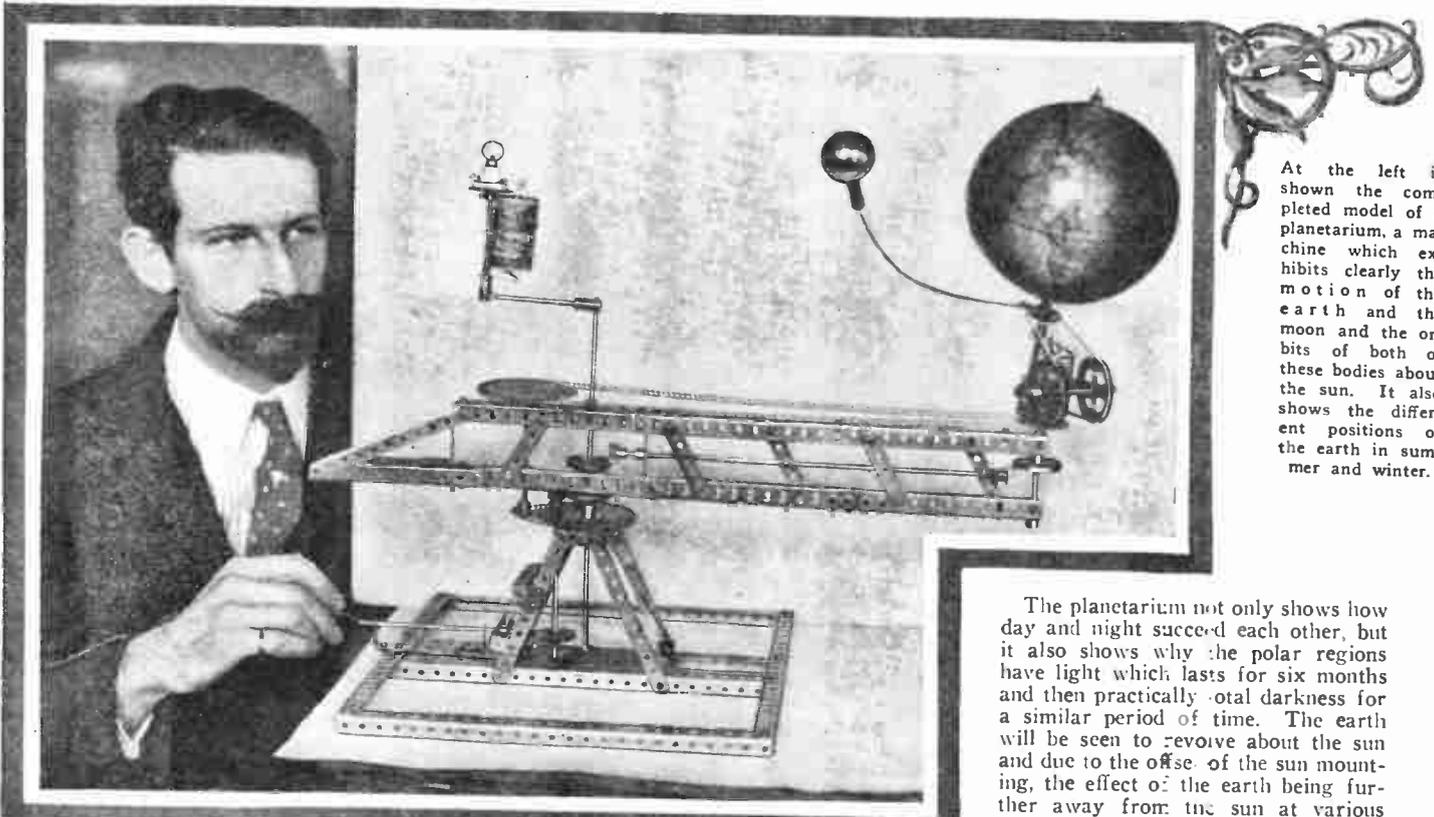
At the left is shown the completed model of a planetarium, a machine which exhibits clearly the motion of the earth and the moon and the orbits of both of these bodies about the sun. It also shows the different positions of the earth in summer and winter.
