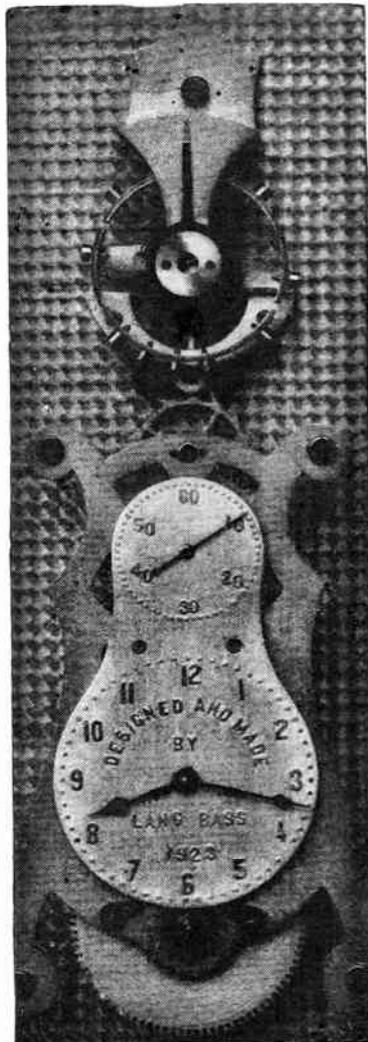
The clock here illustrated measures 8 1/2 inches high, and except for the main spring and hold jewels, was designed and constructed entirely by hand by the author. The hair spring is made of piano wire and the metals of the balance are fused together instead of being soft soldered. It loses less than 30 seconds during a week.
