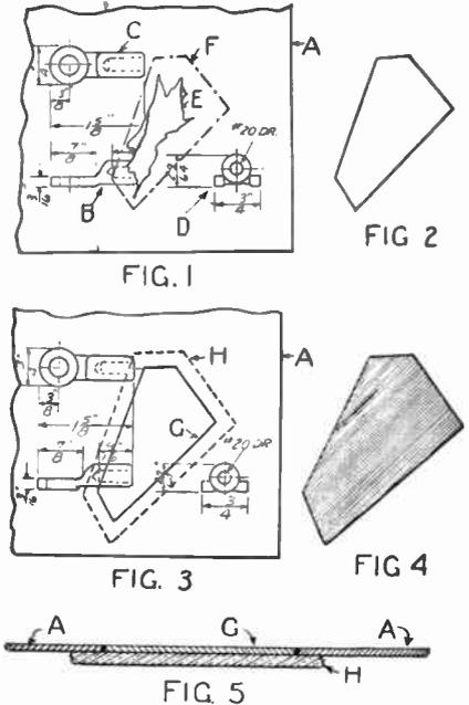
When a tracing is mutilated as shown in Fig. 1, it may be restored. The tear is at E. A second sheet of tracing paper is placed beneath the drawing and a section, F, is cut from both cloths, obtaining a strip from the new sheet which will fit into the removed portion of A. The new piece is placed and fastened with an overlapping strip and collodion. In Fig. 5, A is the original sheet, G the replacement, and H the binding strip. The removed portion is redrawn on the new piece.
