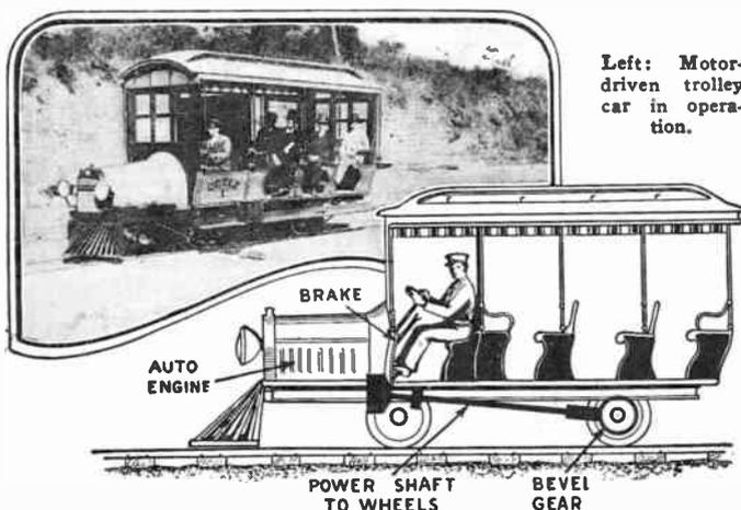
Left: Motor-driven trolley car in operation.
