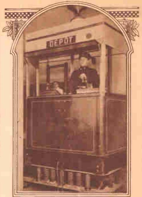
When a subject is to be examined for the position of a motorman on a trolley car, where quickness of thought and instant determination are an important factor, he is placed in a realistic reproduction of the front end of such a car as illustrated above. An observer seated directly to the rear records all movements and reactions.
