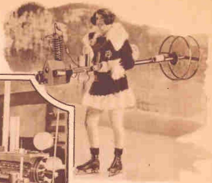
A version of the motopeller made popular by **SCIENCE AND INVENTION** recently appeared on the grand skating rink at St. Moritz. Photograph above shows Miss Zoe Hall handling the device. A  $1\frac{1}{2}$  horsepower motor of special design is said to drive the device over the ice at express speed. The propeller at the rear of the device is enclosed in a housing of metal screening so as to prevent injury in case of accident.
