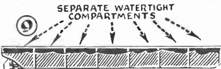
HOW SHIP HULL IS DIVIDED BY BULK-HEAD WALLS TO PREVENT FLOODING AND SINKING
