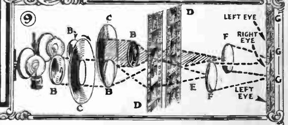
The diagram Fig. 9 illustrates how the images are made upon one single film to be used in the ordinary projection apparatus. When the intensity of light increases for the right eye, it decreases for the left eye.
