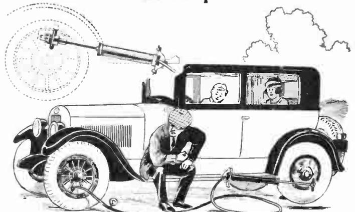
No. 1,520,249, issued to Elmer Kaufmann, provides protection for the type of tire pump clamps illustrated above. One end of the pump is secured on a swivel to the running board of the car, whereupon the handle is fastened by another swivel clamp to one of the rear wheels which is jacked up and turned by means of the motor.
