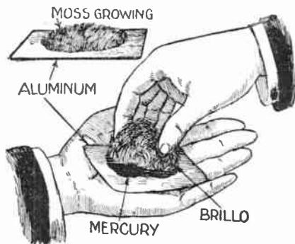
A pretty experiment involving the preparation of aluminum oxide may be performed as above. Place a few drops of mercury on a strip of aluminum and rub briskly with steel wool for a few seconds. A moss-like substance, aluminum oxide will "grow" on the aluminum.
