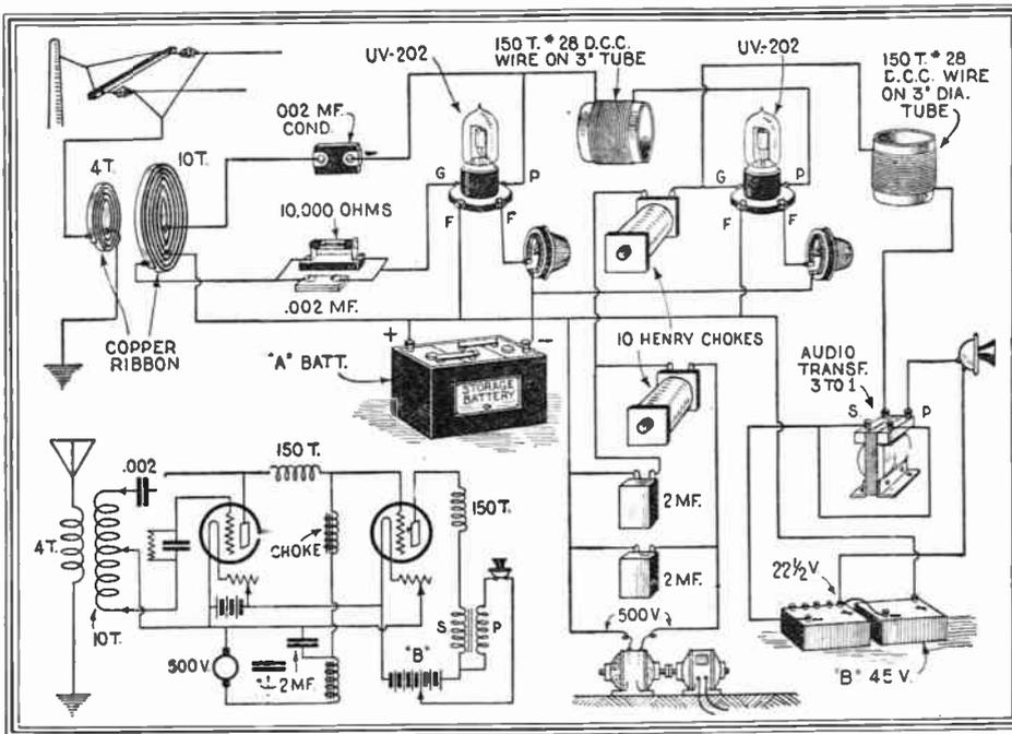
The low power broadcasting set shown above can be used to communicate with stations about 10 to 15 miles apart. The modulation system is of the best and latest design.
