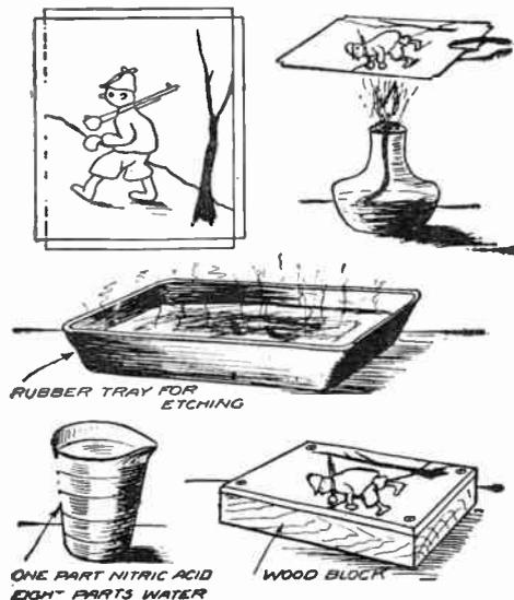
To make your own zinc cuts, draw the required picture on a sheet of zinc with printer's ink mixed with oil of wintergreen. Cover surface with powdered resin and fuse over flame. The sheet zinc is then etched in a bath of one part nitric acid to eight parts of water contained in a rubber tray. The zinc plate is then carefully washed and may be mounted on a wooden block ready for use in a press.
