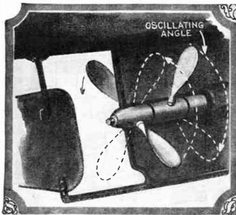
The movements of the two oscillating propellers when in action are indicated in the above diagram. In operation, the propellers are first at right angles to each other as shown in the solid lines, and then they proceed through 90 degrees to the dotted line position.
