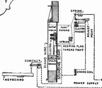
In this electric piano, the strings are vibrated by means of electro-magnets instead of hammers. A schematic diagram of the method is shown at the left. Pressing a key on the keyboard closes a circuit through an electro-magnet, which attracts the piano wire and sets the same in vibration. A second electro-magnet, equipped with an adjustment, breaks the circuit just after the key is pressed and so leaves the string free to vibrate.
