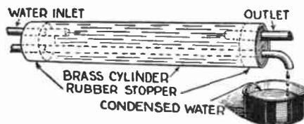
A chemical condenser may be quickly made from a few odds and ends as shown above. A brass cylinder, 3 glass tubes and 2 rubber stoppers are required. They are assembled as shown above and water lead into the inlet pipe whereupon it cools the continuous tube and flows out of the outlet.—William F. Pond.
