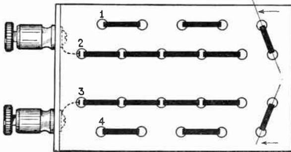
Between numbers two and three, five pair of phones can be connected in parallel. If desired, these phones can be connected in series, by simply plugging in the proper places. A 3/16ths inch drill is used to make all the necessary holes. The device will find a large use where many phones are used.
