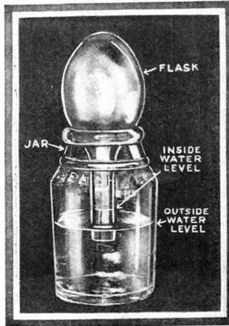
One of the simplest weather forecasters is the water barometer. A simple one may be made as shown above. A flask of any available size is inverted in a jar which is half full of water. It will be found that the water will rise or fall in the neck of the flask in accordance with atmospheric pressure. A rise indicates fair weather, while a fall means a change.
