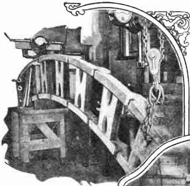
With the use of improved X-ray tubes and accessories thereto, it is now possible to detect flaws in the castings for big guns and their mountings, which otherwise would be invisible even under the most stringent inspection. X-ray tubes placed on one side of a casting and photographic plates on the other side reveal defects in the interior of the casting that could be found by no other means short of drilling.
