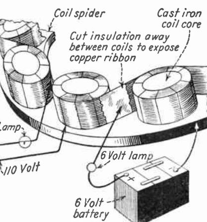
When testing magneto coils as above, if lamp lights, the coil is grounded. Replace with another one. Such trouble is indicated by consistent missing of the engine, not traceable to other causes.
