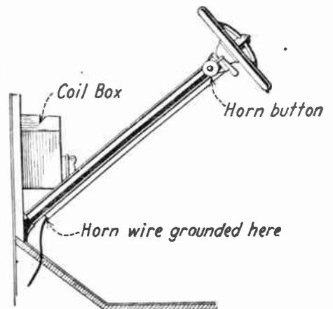
When Ford ignition troubles arise, they are often very difficult to locate. Short circuits occur frequently in unsuspected places. One of the most unusual places for a short circuit to occur, is illustrated above. The insulation on one of the horn wires may wear off at a point where it emerges from its protecting tube, whereupon a short circuit will occur and the engine stop.
