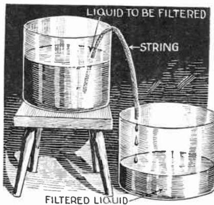
By wetting an ordinary cotton string, it may be used as a filter as shown above. The end from which the filtered liquid drips must be lower than the surface of the liquid to be filtered.
