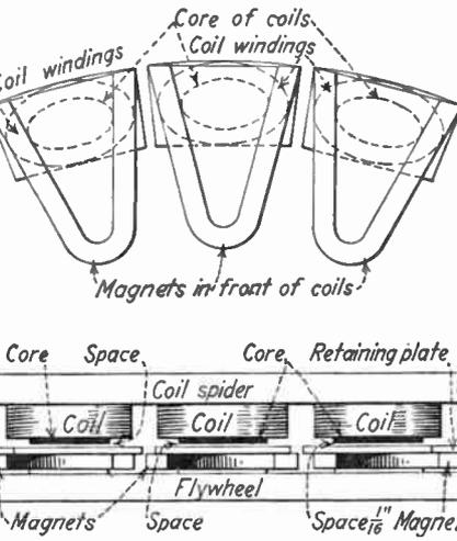
Above: Side and end views of the magneto magnets and winding.
