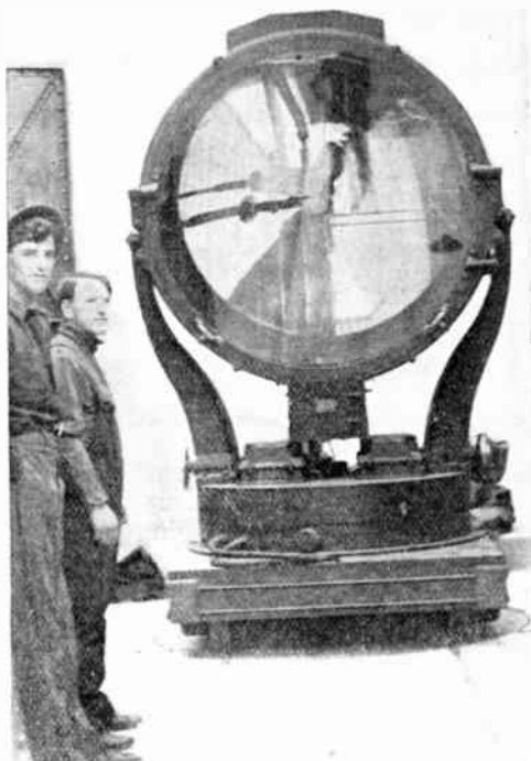
New type of sixty-inch searchlight, fifty of which are being installed at artillery posts on the Pacific Coast
