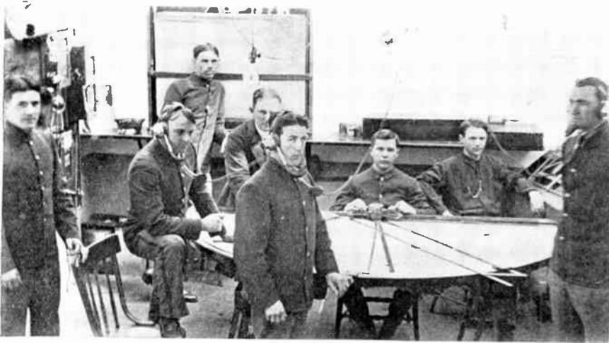
An artillery range-finding station showing plotting board, operated by soldiers in foreground
