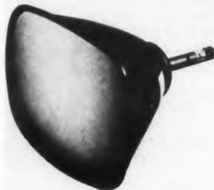
The face plate is of frosted neutral gray glass and relatively flat, to reduce ambient light reflections as well as reflections within the face plate itself, for better picture contrast.
