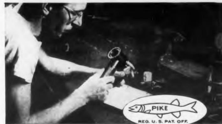
The inspection tool that *lights and magnifies*—FLASH-O-LENS—is in daily use at The B. F. Goodrich Company in making laboratory checks on the dispersion of pigments in milled rubber stocks.
