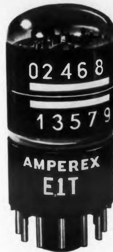
Fig. 1. The Type *E1T* Decade Counter Tube. A count is indicated by a rectangular luminous spot appearing next to one of the figures 0 to 9 on the circumference of the bulb.
