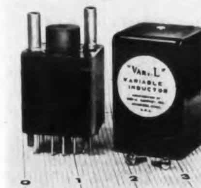
The Model PA-63 Variable Inductor is a manually-variable, high-frequency, saturable-core reactor, with improved stability obtained through use of a permanent-magnet bias. In many f-m and sweep applications
