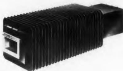
Type 311 High Power Load consists of a stainless steel jacket containing a lossy material which is compound tapered to maintain uniform power dissipation, as well as to achieve a low VSWR. Electrical characteristics include a frequency range of 1.15 to 1.25 kilomegacycles, a maximum VSWR of 1.08, a maximum average power of 1000w, and a maximum peak power of 1 megawatt.
