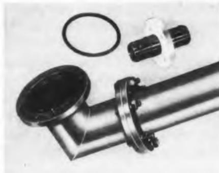
The Series 600 50 ohm V-H-F Teflon Coaxial Line manufactured in accordance with RTMA-134 standard incorporates RTMA anchor insulated connectors for better positioning of the inner conductors, as well as other features that provide better VSWR and attenuation characteristics than outmoded 51.5 ohm lines.
