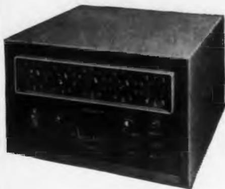
This Electronic Tachometer has been designed to measure rate, frequency, or speed by counting discrete pulses for an accurately timed interval (1sec). A clear, sharp, compact read-out is provided by the use of a cold cathode glow transfer tube.
