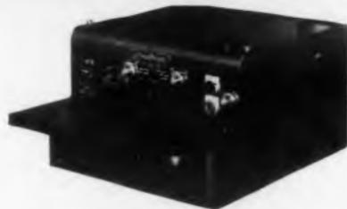
The versatile Analog Data Recorder provides visual or printed records of virtually any physical quantity converted into a corresponding voltage through various functionally operated sensing devices—thermocouples, photocells, tachometer generators, etc. Prints accurate numerical quantity in full figures on tape, tickets or cards.
