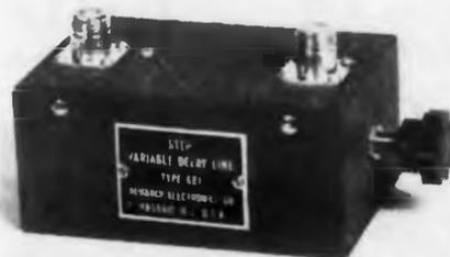
The Type 601 Step Variable Delay Line, consisting of 44 sections of lumped-parameter L-C networks, provides faithful reproduction of input signal pulses,
