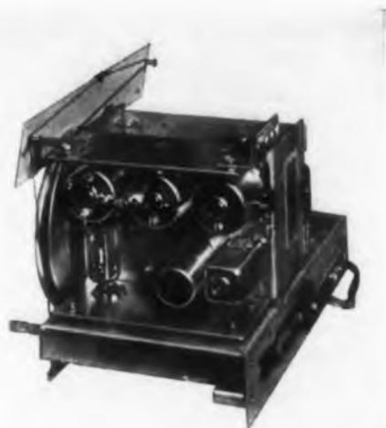
The "Cavi-Tuner"—a u-h-f tuner, has been designed as a component for TV sets to permit reception of u-h-f stations in addition to the present v-h-f channels.
