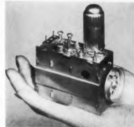
This Front-End Tuner Assembly for reception of u-h-f TV, will tune all channels from 14 through 83 in a continuous 180° sweep of the single tuning shaft. It may be used with any i-f strip capable of receiving its output frequencies
