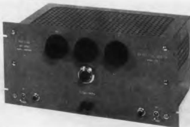
The Kay-Lab Model 123 Meter Calibrator produces a calibrated d-c voltage essentially independent of input line voltage and output load variations. It permits highly accurate and simple calibration of d-c meters. The circuit continuously compares the output voltage against an internal standard cell. The standard model affords absolute calibration to 0.1%, and the custom model calibration to 0.01%. Special models can be manufactured to meet any particular requirement.
