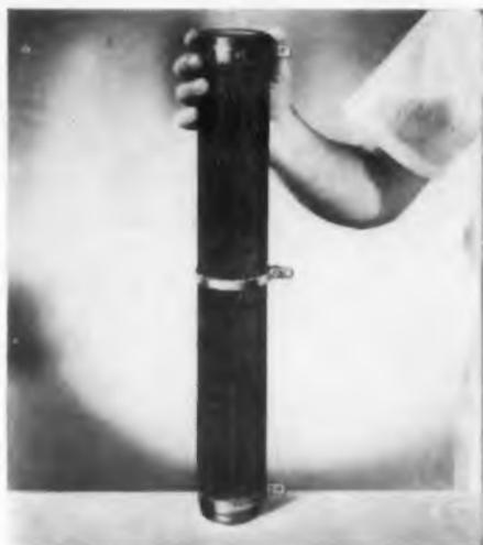
These resistors are available in ratings up to 2000w. They are wound with a specially designed resistance wire on high-temperature refractory cores, affording greater wattage dissipation in low resistance values. All connections are silver-soldered. Coating is
