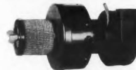
cooling tube seals. On the other end of the motor is mounted a centrifugal blower for cooling the main transmitting tube anode.
