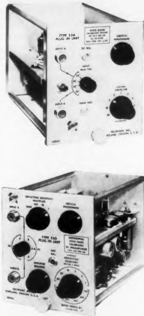
Fig. 1. Two of the plug-in preamplifiers which greatly increase the usefulness of the Type 535 Cathode-Ray Oscilloscope.
