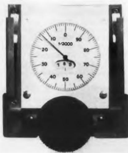
The "Multi-turn Microdual" Type 57-360 is designed for equipment requiring close angular setting, such as variable capacitors, inductances, wavemeters, and slide-wire potentiometers. It permits an unlimited number of 360° rotations. Up to 20 revolutions of the operating shaft are marked on the inset counting dial and the main dial shows 200 revolutions. The combination of the two dials permits positioning to 1 in 4000 divisions.
