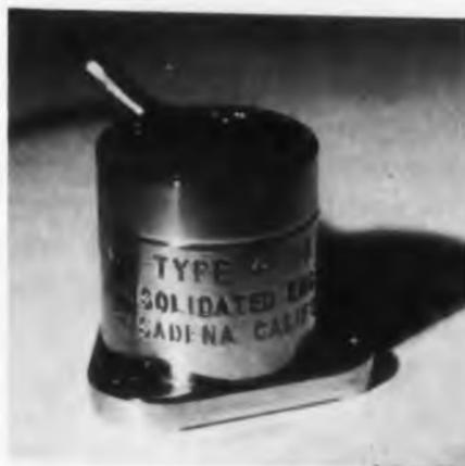
The Type 4-118 Miniature Vibration Pickup measures only 1" x 1" and weighs 1.3 oz. This compact unit is designed for operation at the elevated temperatures encountered in testing many aircraft components. It can operate continuously at 300°F or as high as 500°F for intermittent periods of up to 100 hours.
