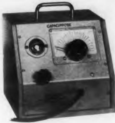
The Model C102 "Capaciprobe" consists of a stable r-f oscillator, a current conversion buffer, a parallel tuned circuit, and a variable sensitivity resonance detector. It enables the user to accurately and rapidly measure total capacitance at any
