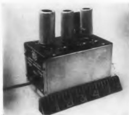
The Cascode Crystal Converter employs only three tubes and measures only 3" x 3" x 5". It is small enough to be mounted inside a communications receiver cabinet, and as many as five units can be
