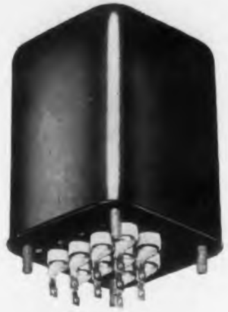
H-TYPE. Steel base cover is deep-seal soldered into case. Terminals hermetically sealed. Stud-mounted unit. Meets all MIL-T-27 specs.
