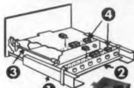
Arrange Alden Side Rails (1) and Alden Lock Frame (2) to suit your chassis. Alden Serve-A-Unit Locks (3) mount in your chassis to engage pre-punched holes in Alden Lock Frame (2) to pilot, draw in, lock or eject. Arrange Alden Back Connectors (4) in orderly row on Alden Lock Frame. Mount mating Alden Back Connectors on your Chassis.
