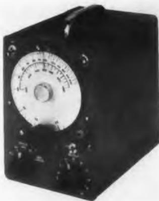
This Extended Range Audio Oscillator, the Model 411, makes measurements requiring a sine wave signal over the range from 20cy to 1Mc. A resistance-capacity tuned type oscillator and a cathode follower in the output system are employed to provide uniform response. Frequency accuracy is main-
