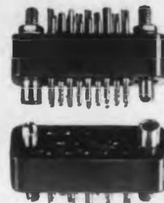
Except for the 8-contact unit, all connectors are interchangeable with similar equipment. Socket contacts are spring types which snap in and out easily without special tools. They require no "C" rings, and no undercutting is needed to seat a "C" ring on the solder-pot side. It is possible to insert insulating sleeving into insulator on the solder-pot side of both socket and pin contacts. Viking Electric, Dept. E1, 1061 Ingraham St., Los Angeles 17, Calif.
