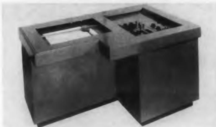
The "Electroplotter" plots from a variety of input data, such as analog or digital computers, punched card machines, or a manual keyboard. In the latter case, a high-speed 10-key keyboard with a numerical verifier provides for plotting rates of about 35 points per minute. Pen traversing speed is 18" min. Accuracy is  $\pm 0.1\%$ . The unit plots on any type paper up to 11" x 17"; larger sizes are available.
