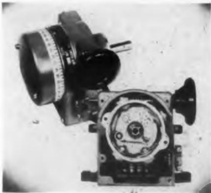
The "Rototimer" provides a simple, accurate means for angular position of a rotating shaft and the opening or closing of an electric circuit. It comprises a cam-operated spst switch that can be externally adjusted
