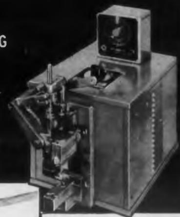
Design with production-wise Joyal equipment in mind to achieve easier production and increased efficiency. **BEFORE:** In making the contact arm shown, it was necessary to thread the wire into the hole, bend the wire, cut the wire, flux, bring part to soldering
