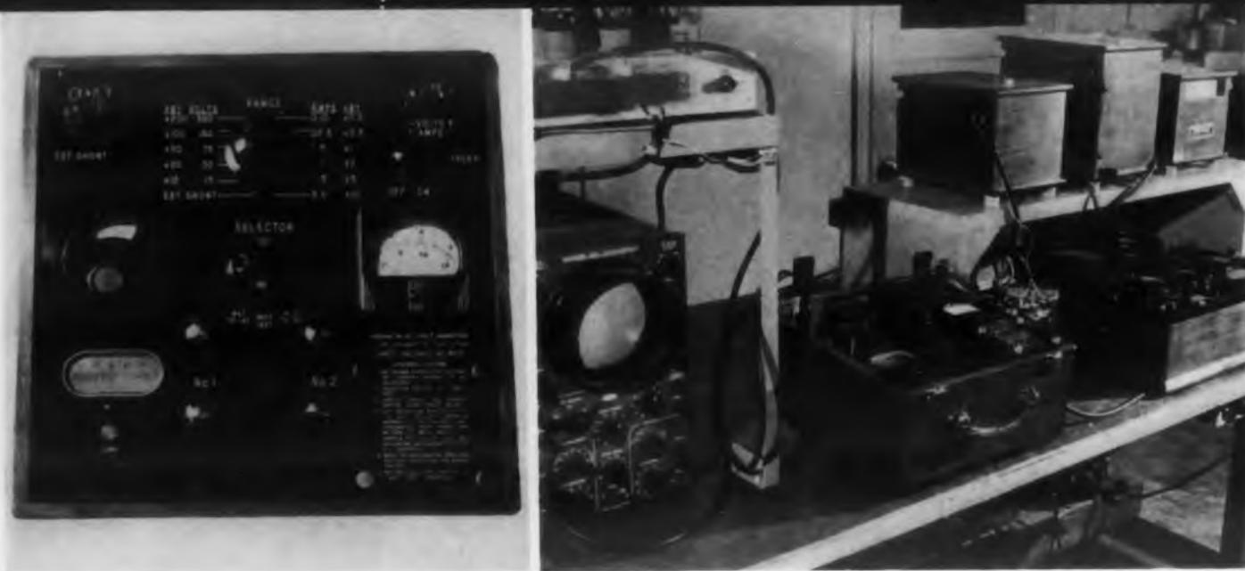
Fig. 1. Front panel of the Hermach-Englehard Transfer Volt-Ammeter is shown at the left, and a typical measuring setup appears at the right. The instrument is accurate to 0.05% over a 20cy to 20kc frequency range.
