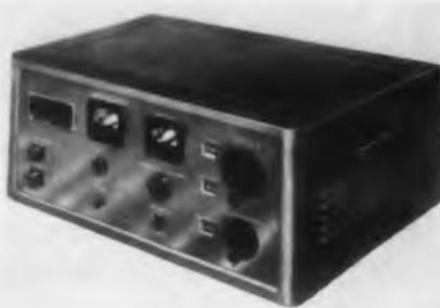
It is adaptable as a general purpose, low-power, portable transmitter.
