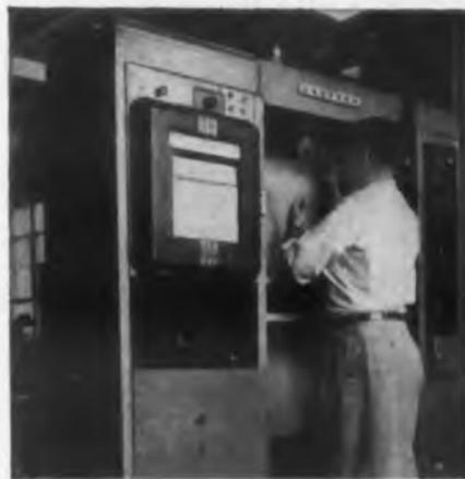
Sylvania employs the most critical test equipment to assure that physical characteristics are held within precise limits. Above is the Instron Tester which registers tensile strength, elongation and yield.
