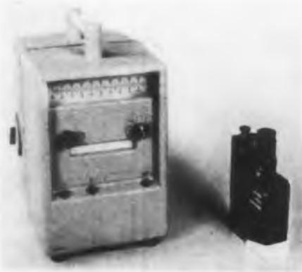
The Model 60A ruggedized galvanometer (right) and Model 61A display box (left) are designed for both field and laboratory use. The galvanometer suspension is totally immersed in liquid having a specific gravity equal to the mean density of the suspension. The resultant assembly is consequently impervious to linear acceleration and shock during operation.
