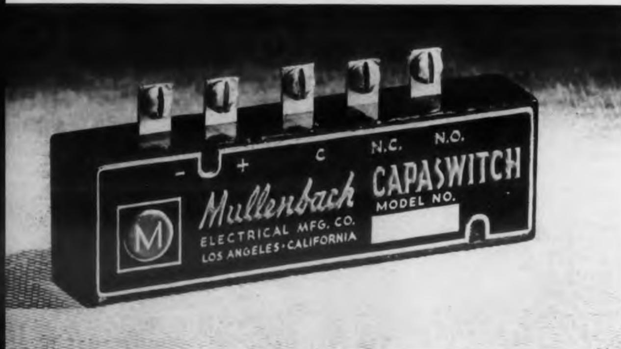
Fig. 1. The "Capaswitch" at the left is a sensitive nonmagnetic relay which operates by means of an electrostatic capacitive element. It requires very little power and responds to very short pulses.
