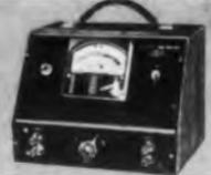
**No. 1060 VACUUM TUBE VOLTMETER.** A 50 megohm input impedance wide frequency range V.M. for use at audio and super-sonic frequencies.
