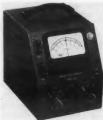
This special, expanded scale voltmeter is designed especially for measuring transformation ratios of transformers, synchros, and resolvers. It is equipped with separate inputs for primary and secondary voltages of 57.3v, 78v, 90v, 105v, and 115v. Primary or secondary
