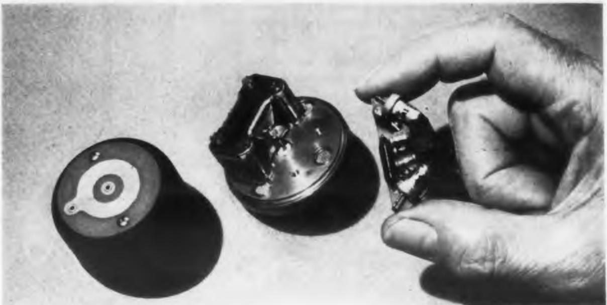
Fig. 1 (above). A disassembled preamplifier unit showing its high gain transistor amplifier. It affords improved reception, yet saves weight.
