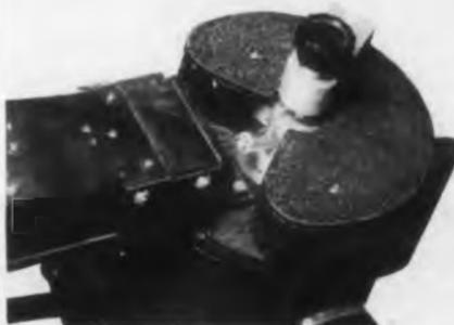
The Model C-7 High Frequency Vibration Exciter with its accessory equipment, Model P-70 Amplifier and F-34 Field Supply, is especially designed for testing sub-miniature electron tubes. It incorporates a means of rigidly clamping the tubes in the armature, and includes a flat top table to facilitate its use in the calibration of small vibration pickups and accelerometers.
