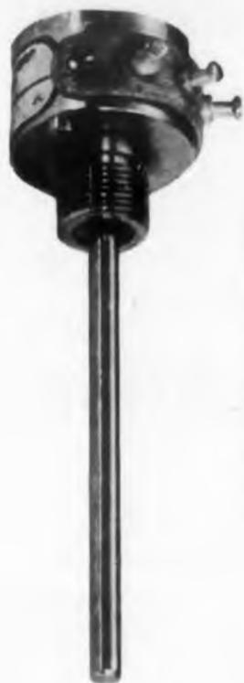
Fig. 2. The metallic film potentiometer which features small size, infinite resolution, satisfactory operation at temperatures from -55°C to +225°C, and high wattage dissipation. It can be used for military as well as industrial applications.
