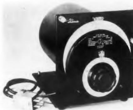
The Type 1211-A Unit Oscillator has a frequency span of 0.5Mc to 50Mc which is covered in two 10-to-1 logarithmic ranges. Frequency is read directly from a 6" dial, with a slow-motion-drive dial
