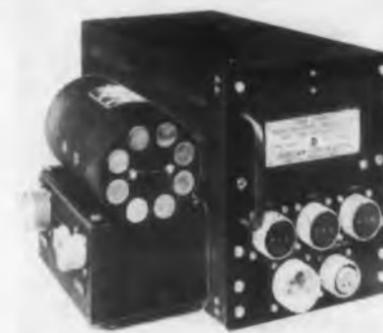
The Type VF-DD Test Instrument consists of a power supply and a three-channel demodulator unit. The power supply section is especially suited for exciting many types of transducers, such as gyros,
