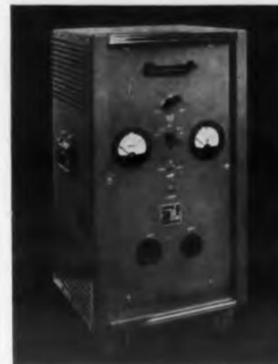
100 amps at 6 volts, 75 amps at 12 volts, 50 amps at 28 volts.
