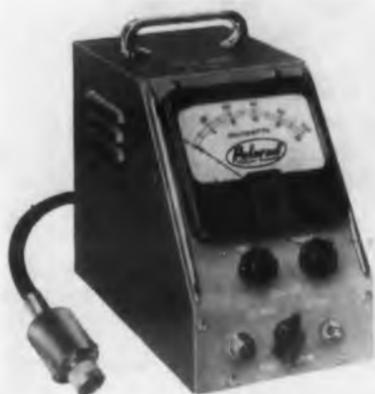
This power meter measures rms power over the frequency range of d-c through X-band without the use of frequency limited bolometer mounts. Completely self-contained, it uses a single power probe for all frequencies.
