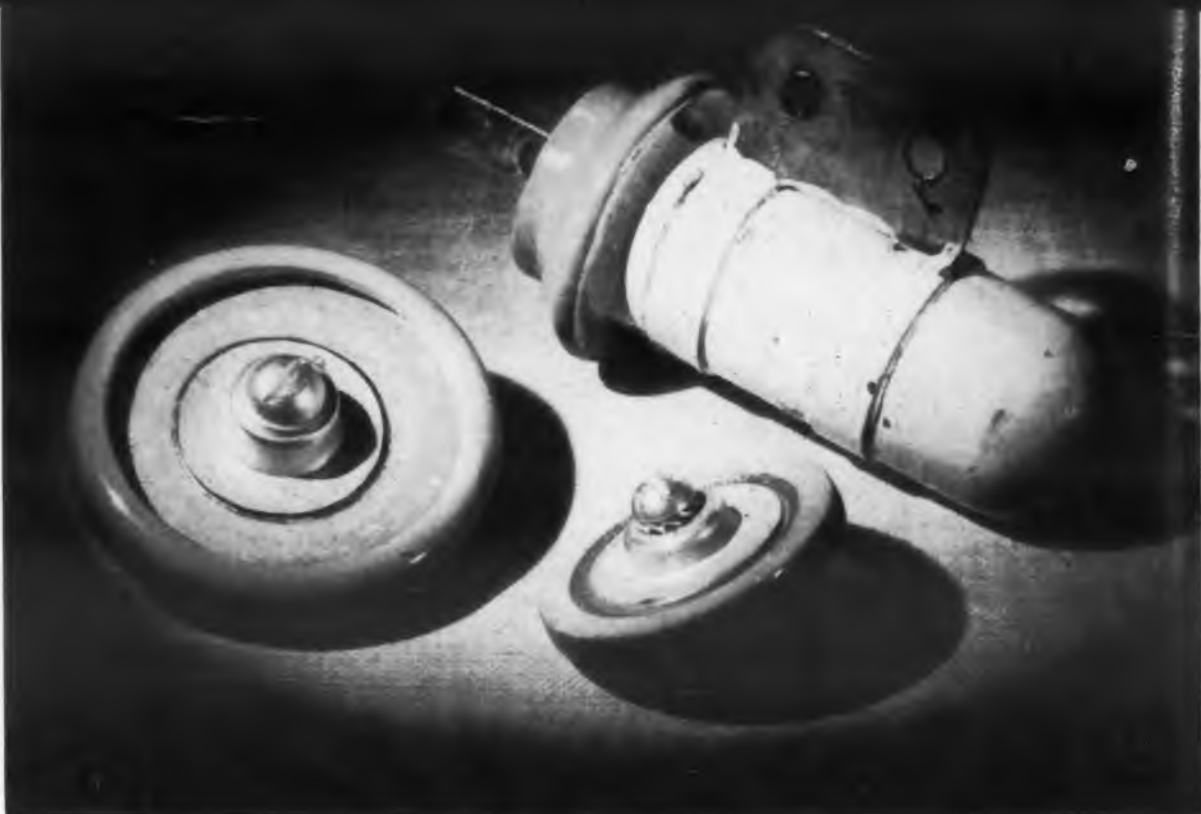
Fig. 1. These capacitors retain their properties to 1000Mc and above.
