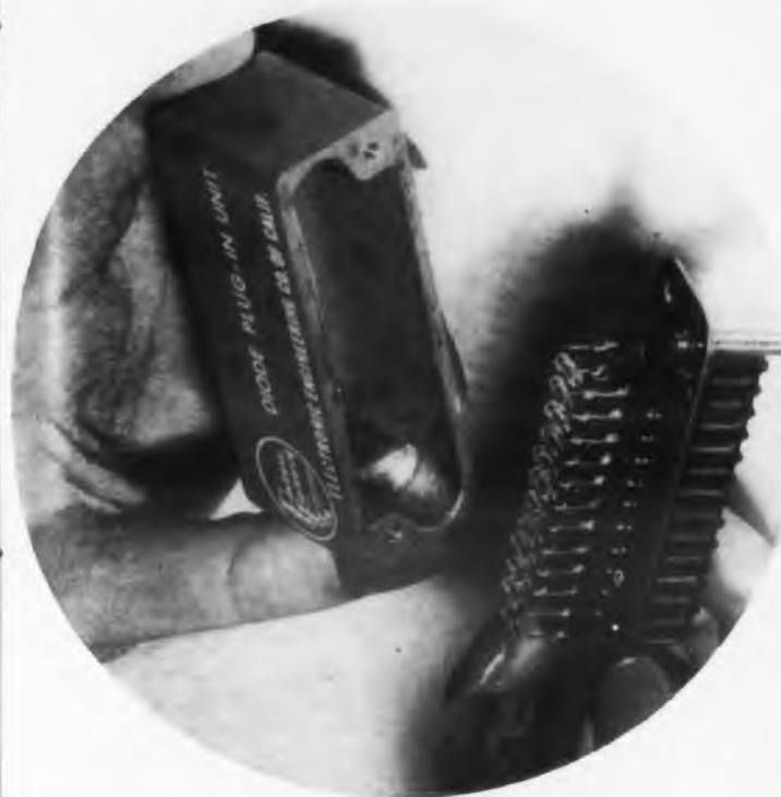
Fig. 3. By removing the two round head screws shown in Fig. 1, the components are quickly exposed for servicing. The cover is made of cast aluminum.
