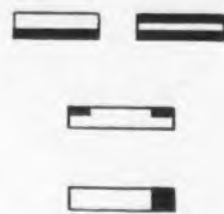
Fig. 1. Three forms in which clad metals are available: overlaid on one or both sides (top); inlay (middle); edge clad (bottom).
