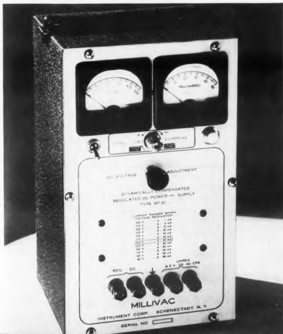
Fig. 1. The Series RP power supply. The load compensation control is centered just below the meters. The output characteristics of each model are printed on the panel, with rated values in a box.
