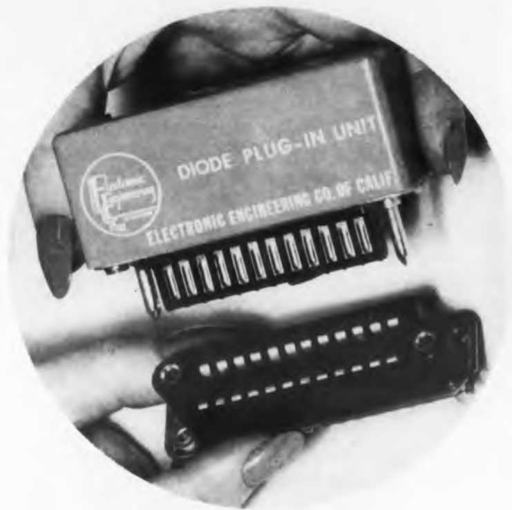
Fig. 2. The plug-in unit and its "Amphenol" base. The guide pins insure correct polarization.
