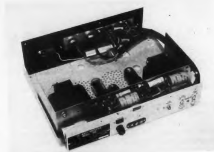
Fig. 6. Notice the separate pre-amplifier sub-chassis in the Horizon 10.
