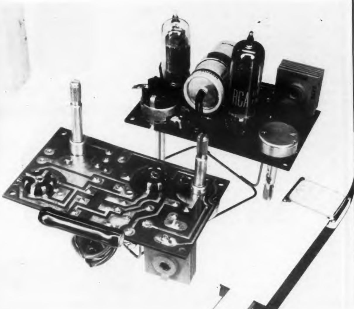
Fig. 1. Bottom and top views of the printed-wired amplifier.
