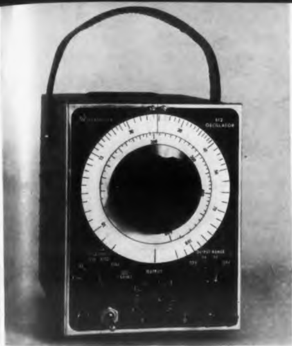
Fig. 3. The portable Model 512 Oscillator. The concentric frequency scale is 14" long.
