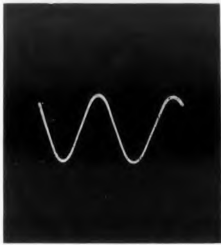
Fig. 1. A cathode-ray-oscilloscope photo of the 1cy output waveform.
