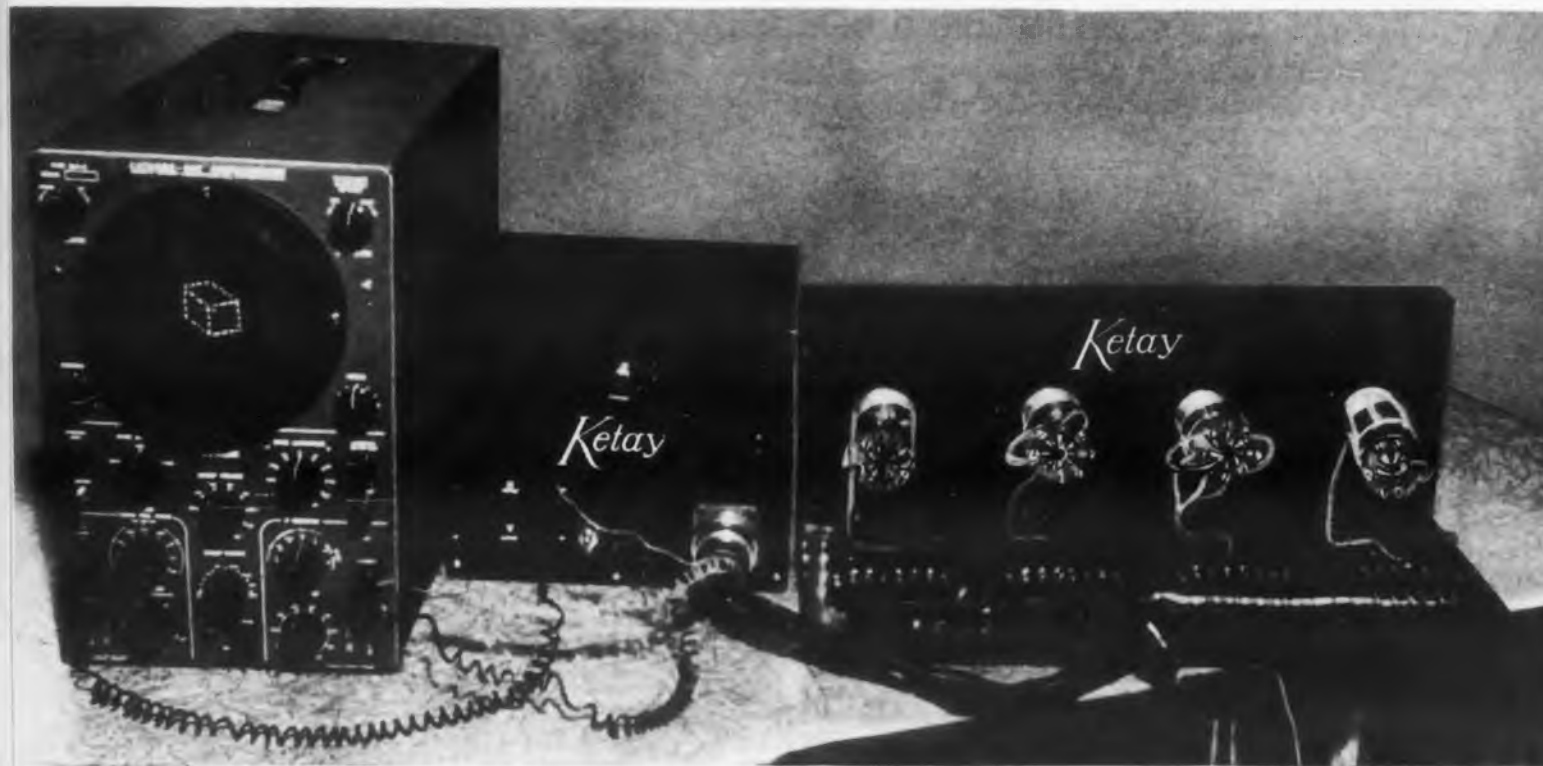
Fig. 1. The complete equipment required for a three-dimensional display includes an oscilloscope (left), a power supply for the resolvers, and the four-resolver assembly. A display is shown on the oscilloscope screen.
