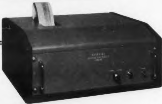
Model 1452 prints 6 digits (8 or 10 on special order) on standard adding machine tape. Is only 19" wide x 10 1/2" high x 14" deep, weighs 60 lbs. Price, $750.00 f.o.b. factory.
