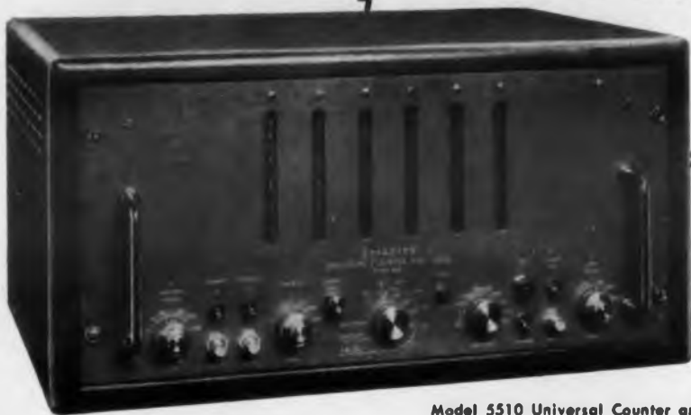
Model 5510 Universal Counter and Timer offers direct-reading digital display of count, frequency or microsecond time interval. Time bases from 1 mc. to 1 cps; gate times from .00001 to 10 sec. Accuracy \pm 1 count, \pm crystal stability (1 part in 10^6 ). Price $1,100.00 f.o.b. factory.
