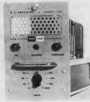
The Model 110 is a chopper - stabilized broadband d-c amplifier with longtime drift (40 hours) of  $\pm 2\mu\text{v}$ . Equivalent input noise is less than  $5\mu\text{v}$  peak-to-peak for 3cy bandwidth, less than  $5\mu\text{v}$  rms for 750cy band, and less than  $12\mu\text{v}$  rms for 50ke bandwidth. Variable gains of 0, 20, 30, 50, 70, 200, 300, 700, and 1000, accurate to 1%, are provided. Bandwidth is flat within 3db from d-c to 30ke.
