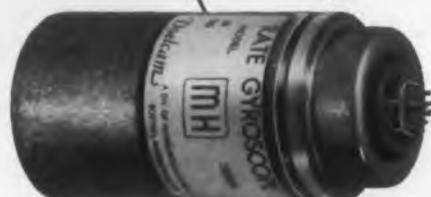
**Rate Measuring Gyroscopes, Type JR** for tactical weapon systems requiring less than one minute warmup. Incorporate damping compensator for constant damping ratio without heater. Linear output signal proportional to input rate within 0.25%. Withstand 50G shock, 15G vibration up to 2000 cps. Angular Momentum — 10<sup>6</sup> gm.-cm.<sup>2</sup>/sec. Size 3¾" long x 2.0" diameter. Write for Bulletin JG10
