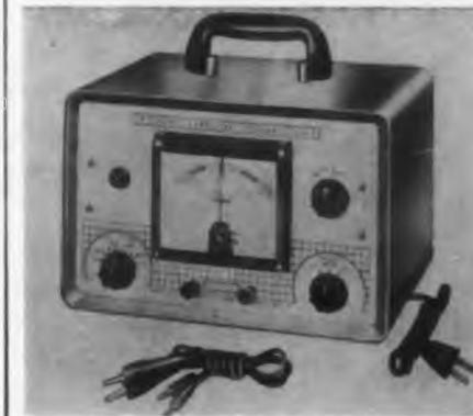
The In-Circuit Capacitor Leakage Tester, Model 383, shows the presence or absence of leakage in virtually all paper, mica, or ceramic capacitors while connected in the circuit, eliminating disconnecting and resoldering.
