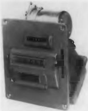
This panel-mounting electrical impulse counter is presettable in seconds for any number to 100,000. On reaching predetermination a dpdt process control switch is thrown and the counter resets automatically by motor and is ready for the next cycle. It is also resettable by signal (pushbutton, etc.), or manually by lever. It may be
