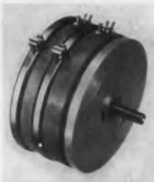
A special clamp band provides an unrestricted tapping area, allowing up to 33 taps, and presents a simplified means of phasing units in a ganged assembly without disassembling the units. The potentiometer is gangable in assemblies of up to 6 cup units on a single shaft. It has a diameter of 3-1/8" max and a cup width of 0.984". Potentiometer Div., Fairchild Controls Corp., Dept. ED, Robbins Lane, Syosset, L. I., N. Y.
