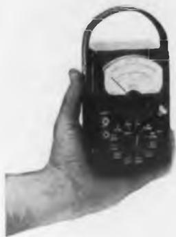
Now! Voltage measurements to 1 MC with  $\pm 5\%$  accuracy, no ac power supply. Temperature stable 0 to 120° F. Transistorized, rugged printed circuitry. Battery powered, weighs 32 oz. \$250.00.
