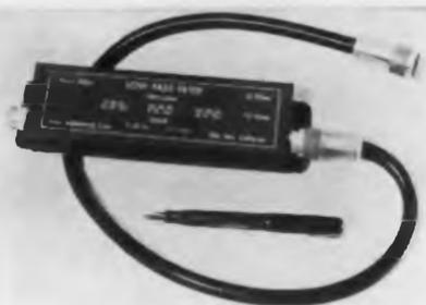
The Low Pass Filter Unit No. 8314 has wide application for use between the transmitter and antenna to attenuate spurious r-f output. It is particularly use-
