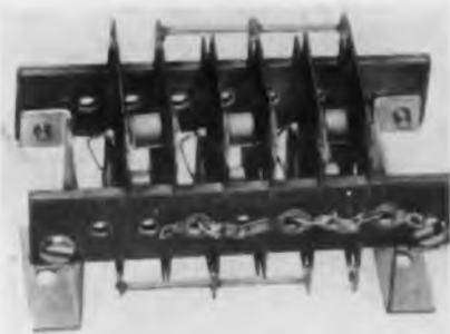
These germanium rectifier power stacks are smaller than previous designs by about one-third, as a result of improved convection and cooling. Despite this smaller size, a special base
