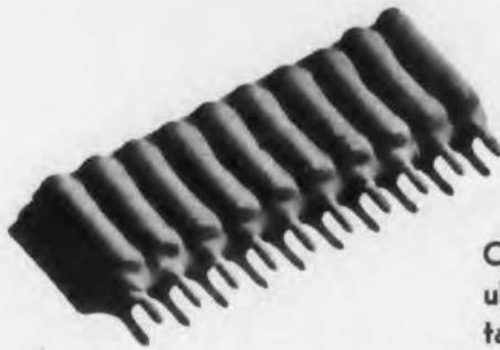
One form of the modular sub-circuits containing 10 components.
