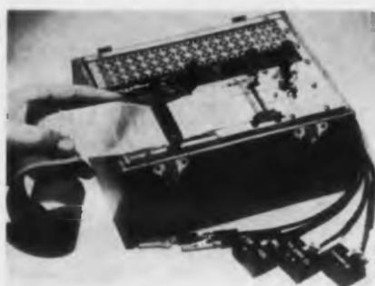
"Record-a-meters" are compact, rugged, light-weight, direct-writing oscillographs used in place of, or in conjunction with, meter-type test equipment to secure a continuous recording of any measurable phenomenon within the frequency and sensitivity limits of the instrument.
