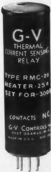
G-V Sensing Relays operate contacts when current or voltage to their heaters exceeds or drops below the operating point.
