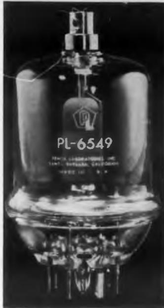
Here is Penta's new PL-6549 beam pentode, a compact power package which is daily finding new applications where reliability, high efficiency at low and medium voltages, low driving power, and excellent linearity are required.
