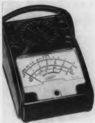
This instrument is available in two models, Industrial Model 455 and Audio Model 456, and features a new technique to eliminate accidental burn-outs. The instrument disconnects itself and raises a reset button on the case if a dangerous overload is applied.
