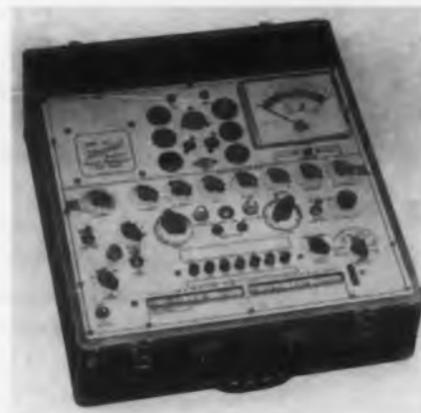
The Model 750 permits quick and accurate evaluation of any tube normally encountered in all phases of electronic work, including the latest military ruggedized types, TV, or hearing aid receivers. It also tests germanium diodes
