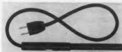
The magnetic erasing pencil, Type 8905, is most practical for erasing limited small areas when it is necessary to erase a syllable or part of a word. It operates on 115v 60cy at 10w, and comes complete with press-to-operate switch and 6' of cord. Dimensions are similar to a king-size fountain pen.
