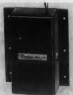
This small, lightweight, transistorized, d-c transformer is completely static and has no bearings or brushes. It handles an input of 24 to 30v d-c, and will produce any d-c output. Occupying only 10 cu in, the unit is well suited for miniaturization applications. The shape of the unit is squared and is suitable for stacking. Weight is only 11 oz. Efficiency is 85%.
