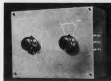
A series of custom-built Variable Delay Lines is available for use as laboratory test equipment to facilitate the design and development of advanced computer and radar systems, or for use as components. The lines come completely enclosed in dust-proof cases with coarse and fine controls. Delays are proportional to the angular position of the respective control shaft. Delay time, impedance, and bandwidth are designed to meet individual specifications.
