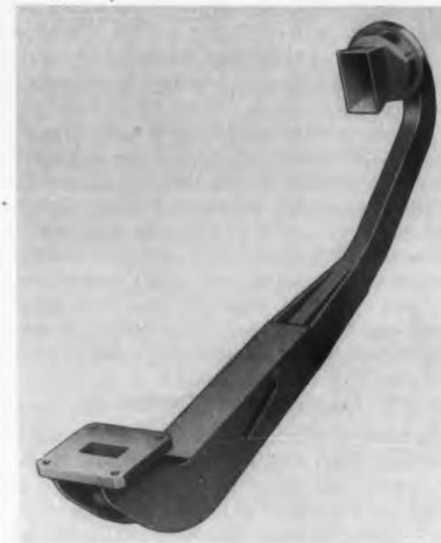
Waveguide in this feed horn is bent in both planes, and twisted 90°, from one length of seamless extruded magnesium tube. Electrical function is not impaired by structural weldments.
