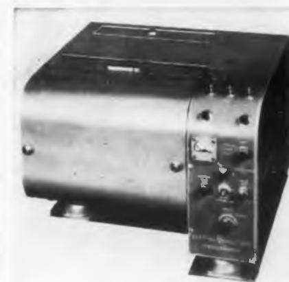
The PM-20 is a general-purpose oscillograph for static or dynamic testing of all types of industrial or aircraft equipment and is available in d-c and a-c models. It will record up to 71 individual variables on one oscillogram when combined with suitable transducers and amplifiers for the measurement of pressure, vibration, strain, flow, etc. This makes it possible for users to record simultaneously the many variable factors encountered in dynamic testing of machinery.
