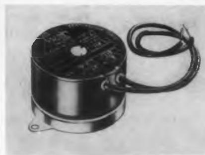
The Type 113 is an inexpensive synchronous timing motor. Torque rating is 30 in-oz at 1rpm. Right, left, or oscillating shaft rotation is available. The motor runs equally
