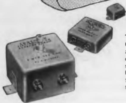
These SEC Polystyrene Capacitors have an accuracy in the order of 0.1% or better and longtime stability in the order of 0.03%. Natvar Styroflex film is used as the dielectric.
