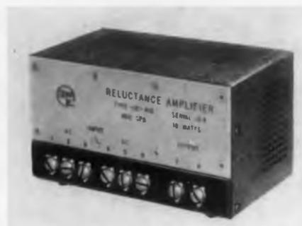
This small, lightweight, reluctance-type servo amplifier, Model 1121, accepts two a-c inputs and one d-c input in any combination. With instantaneous response (time lag is negligible compared to 1 cy of supply frequency) it produces proportional and reversible power output for most 115v 400cy servo motors rated at 18w or less. Operating directly from the power line, total power consumption is low for small input signals, and less than half plate dissipation is required at no load.
