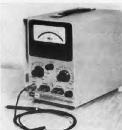
The Model 203 D-C Microvolt-meter-Ammeter is capable of making accurate measurements of voltages as small as  $10\mu\text{v}$  and currents as small as  $1\mu\text{amp}$ . Fifteen voltage ranges cover from  $100\mu\text{v}$  to 1000v (full scale). Ten current ranges from  $100\mu\text{amp}$  to 100ma (full scale) are provided. The small signal to be measured is amplified by a chopper amplifier, rectified, and applied to a precise microammeter.
