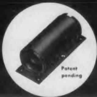
IERC "Hard Mounts" permit operation of electron tubes at full rating at ambients up to 175°C without exceeding maximum bulb temperature. Resonance-free up to 2000 cps, "Hard Mounts" withstand highest shock and vibration in any equipment—give best cooling, failure-protection.
