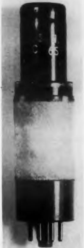
These plug-in circuits stand 4½" off the chassis, including tube.
