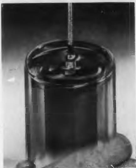
The 5049 Series Hermetically Sealed Receptacles are designed to mate with 50 ohm screw-type Microdot coaxial cable plugs. Hermetic seals are obtained by a glass head section in the dielectric and by soft soldering each receptacle to the panel.
