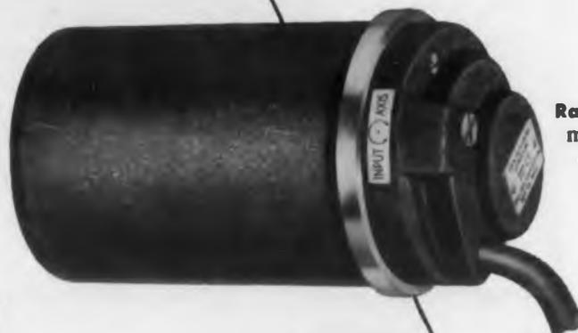
**Rate Measuring Gyroscopes, Type K** for guided missile control and homing systems and flight evaluation of military aircraft. These models measure absolute angular rates where high accuracy and superior dynamic response are essential. Linear output signal proportional to input rate within 0.25% of full scale. Withstand 100G shock in any plane and 15G vibration up to 2000 cps. Weight—3½ lbs. Size—5¾" long x 3.20" diameter. Write for Bulletin KG10
