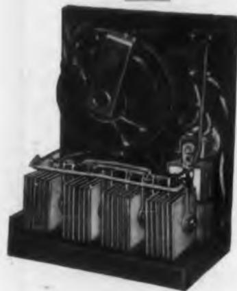
One of General Radio's Variac Motor Speed Controls showing a typical application of Radio Receptor Selenium Rectifiers. Six RRco. units are employed here.
