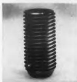
Compare UNBRAKO-recommended tightening torques with those of ordinary socket set screws and you readily see why you can set an UNBRAKO and then forget it. The reasons are simple. UNBRAKOs have deeper sockets, which give you better purchase with the wrench; rounded socket corners, which eliminate the sharp corners
