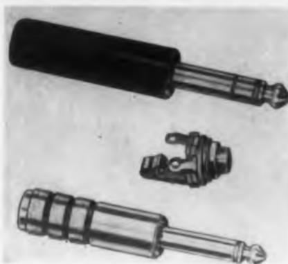
A line of "Hand-D" phone plugs and jacks has been introduced by this firm. The plugs are reduced in size, sturdy in construction, and contain a one-piece solid brass nickel-plated rod pressed into the tip terminal
