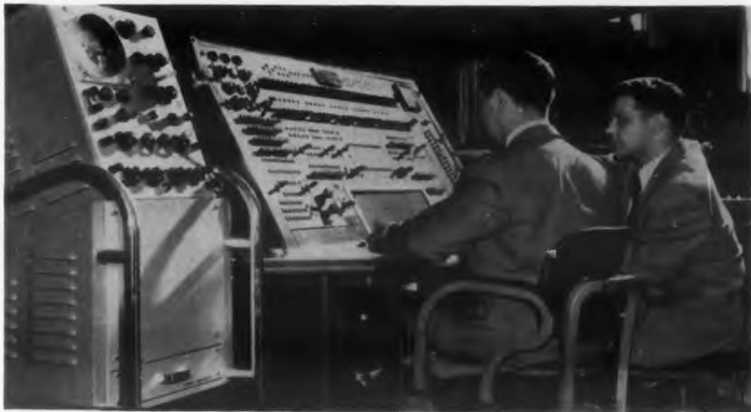
This electronic panel controls operations involved in obtaining a massive calculation from the "Univac" central computer at the new data processing center of Sylvania Electric Products, Inc. at Camillus, N.Y.
