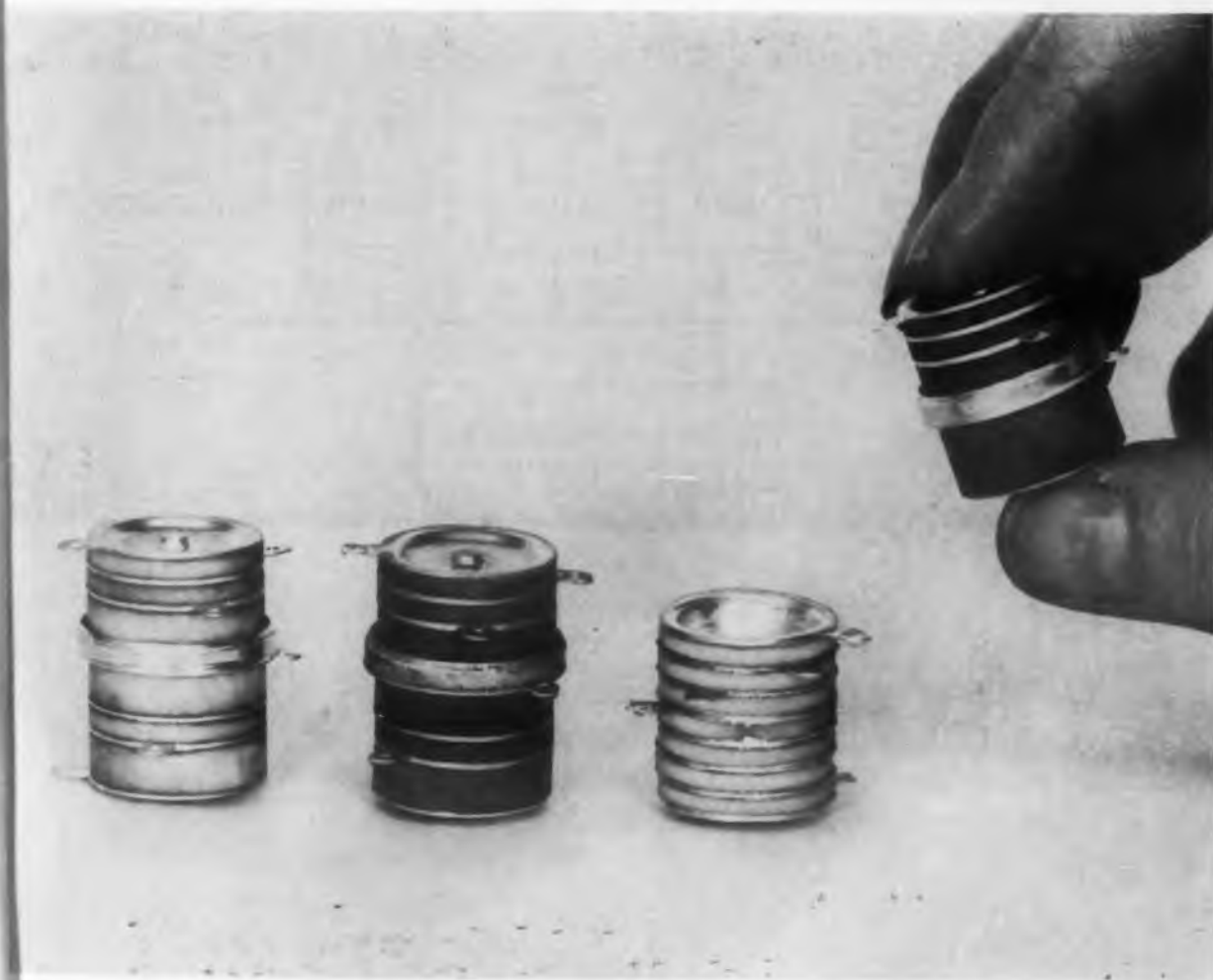
Four ceramic tubes adaptable for environments found in aircraft and missile applications.
