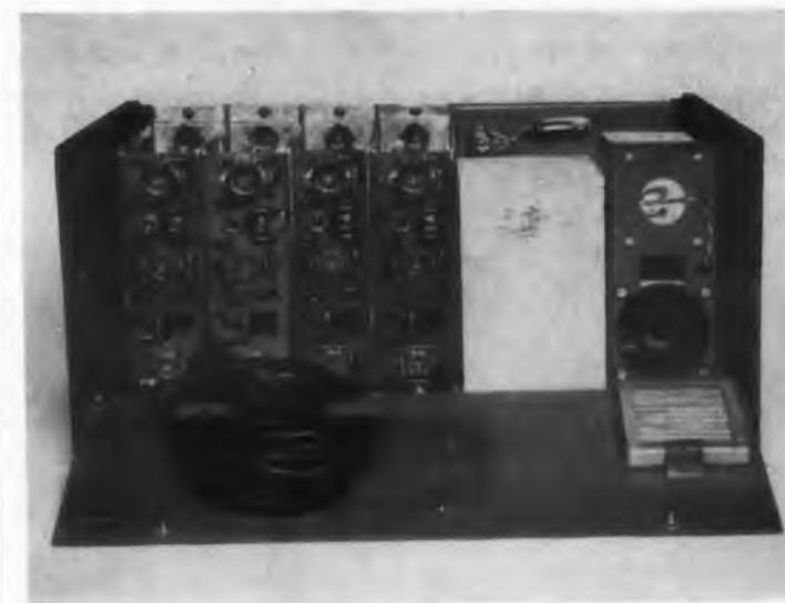
Fig. 3 Rear view of the unit showing 4 amplifier cells and fan with filter (lower right).
