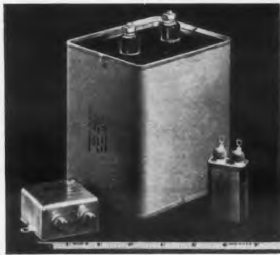
MIL-C-25A CAPACITORS —for filter, by-pass, and blocking in military equipment. Ratings: .05 to 15 uf at 100 to 12,500 v. d-c in case styles CP50, CP60, CP70 series. Temp. range: -55C to +85C, and -55C to +125C. Write for GEC-810.
