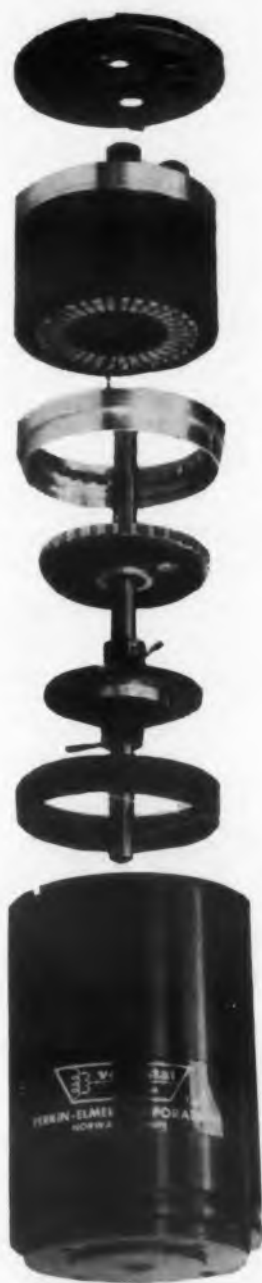
Fig. C. Exploded view of the Vernistat showing construction of the gear mechanism.
