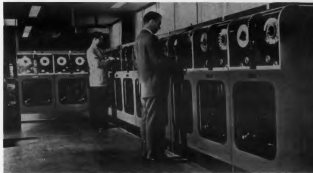
Each of these units carries magnetic tape to and from the computer. In effect, they "read" instructional information and transmit it to the "Univac". After the computer digests the information and solves the problem, the Univacs "write" this new information back on to the magnetic tape and carry it along to the printer.
