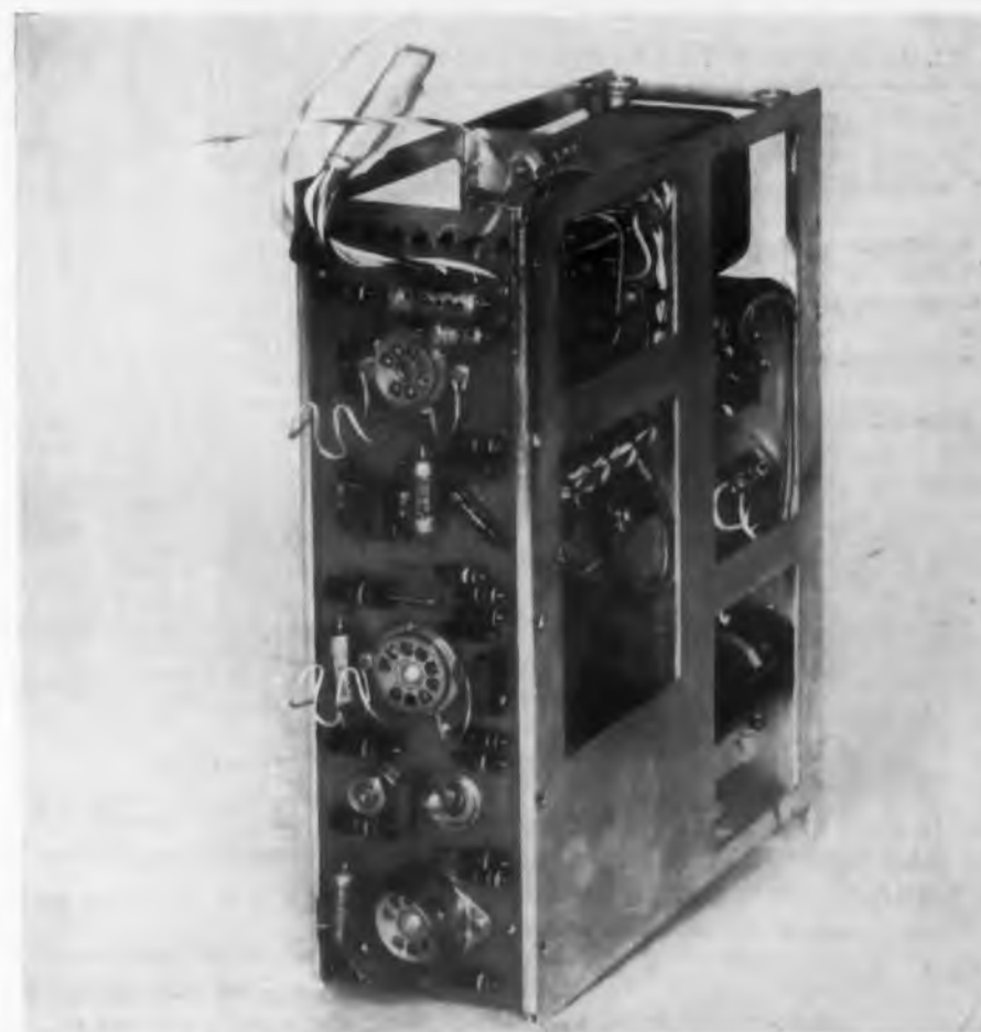
Fig. 2 Cellular type construction permits easy removal for servicing.
