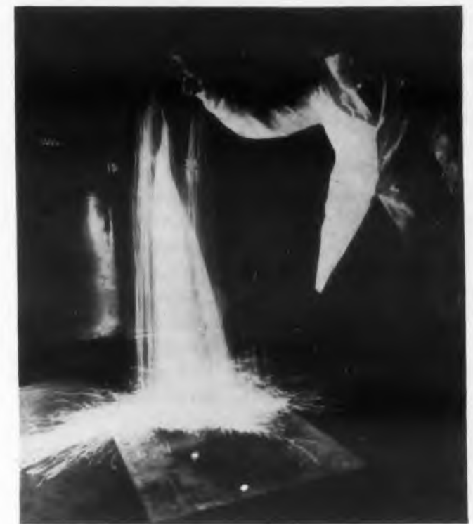
Highly purified manganese-bismuth catches fire spon- taneously on exposure to air and must be processed in an inert atmosphere of helium.
