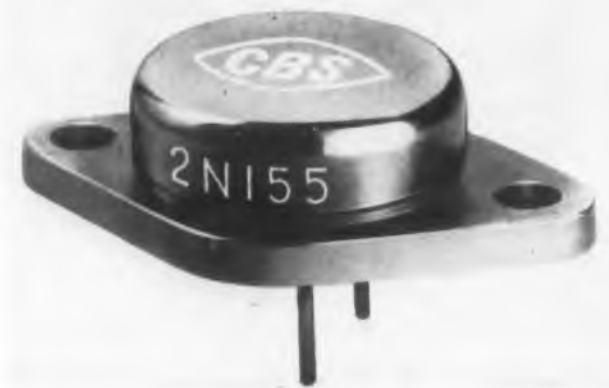
Fig. 3. Power transistor with collector attached electrically and mechanically to case for good heat transfer.
