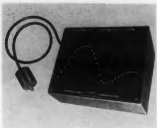
Fig. B. Front panel of the printed-circuit switch provides a visual representation of the output. Each vertical slider connects one of the 31 poles to one of the 100 auto-transformer taps. Panel is 6 x 7-1/2 in.
