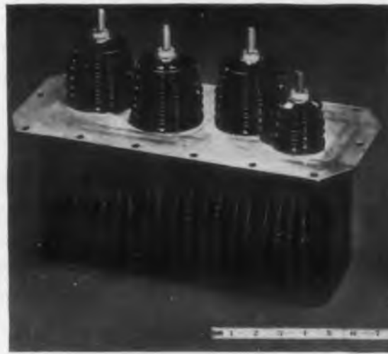
CAPACITOR PULSE FORMING NETWORKS —for missiles and radar equipment. Capacitance tolerance: \pm 7\% (at +25C). Temperature range: -55C to +125C. Write for GEA-4996.
