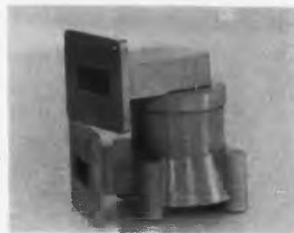
Capable of operating at 600 kw peak power for short intervals, the rotary joint will operate at 350 kw during extended use. Impact and vibration tests per MIL-T-17113 show unimpaired mechanical operation and no internal damage.
