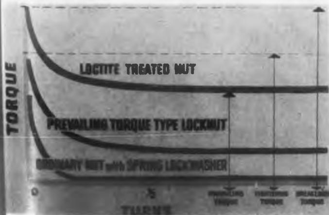
Torque comparisons of loctite, locknut, and spring lockwasher
