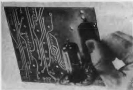
This new angle socket has been designed for use in electrical and electronic units in conjunction with printed circuits. The socket provides for the
