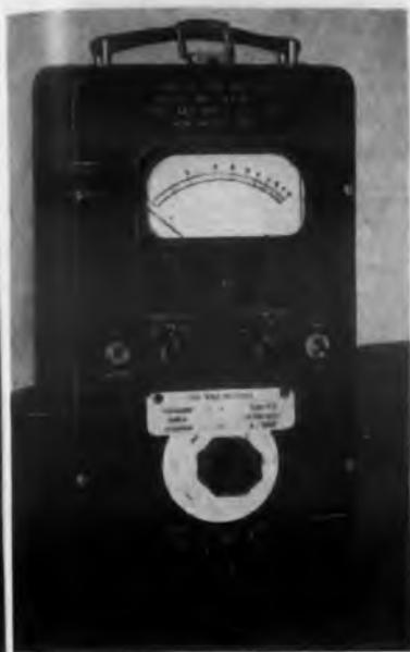
This improved Model M6 vibration meter teams up with an MB Vibration Pickup to give you the facts on vibration. It measures voltage generated by pickup... directly in terms of amplitude, velocity or acceleration of the vibratory motions.
