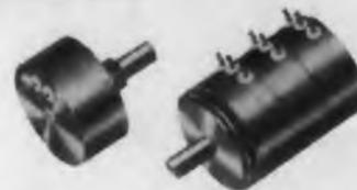
Precision 1 1/4" dia. single-turn potentiometer. Standard Resistance Range—10 $\Omega$  to 30 K $\Omega$   $\pm 3.0\%$ . Standard linearity  $\pm 0.5\%$ . May be ganged—2 to 15 sections. Up to 14 extra taps per section.
