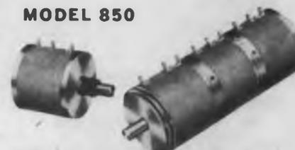
Precision 1 1/4" dia. 3-turn potentiometer. Standard Resistance Range—20 $\Omega$  to 120 K $\Omega$   $\pm 3.0\%$ . Standard linearity  $\pm 0.3\%$ . May be ganged—2 to 3 sections. Up to 18 extra taps per section.
