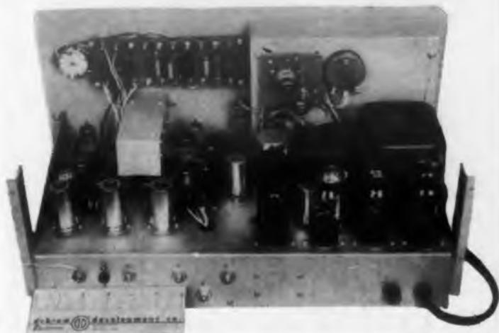
The circuit also incorporates a phase inverting amplifier, phase network driving amplifiers, a phase shifting network, cathode followers and output amplifiers. Printed circuits and miniature components are employed which result in a small packaged unit.
