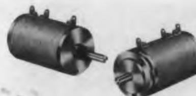
Precision 7/8" dia. miniature 10-turn potentiometer. Standard Resistance Range—25 $\Omega$  to 120 K $\Omega$   $\pm 3.0\%$ . Standard linearity  $\pm 0.3\%$ . Up to 38 extra taps per section.
