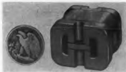
The Model 24 Torque Motor features fast response and high output force. It weighs only 11-1/2 oz and has an output conservatively rated at 8 lb of force for 3 w of input power. Designed to drive hydraulic servovalves or similar mechanisms, it may be operated by electronic, magnetic, or even transistor amplifiers.
