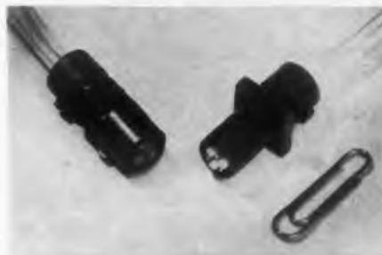
These miniature, high altitude, high temperature connectors are capable of operation at any altitude and temperature up
