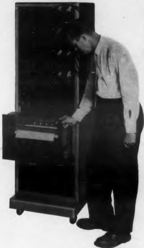
Rack-mounted Dynograph assembly. The amplifiers are at the left, the input couplers to the right. The stylus control panel is below, and just above the slide-out recorder.
