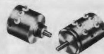
Precision 7/8" dia. miniature single-turn potentiometer. Standard Resistance Range—10 $\Omega$  to 20 K $\Omega$   $\pm 3.0\%$ . Standard linearity  $\pm 0.5\%$ . May be ganged—2 to 6 sections. Up to 9 extra taps per section.
