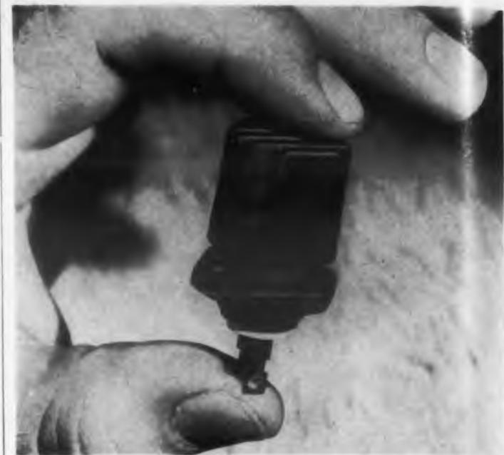
**H**IGH power in miniature size and single hole chassis mounting make this new wire wound resistor significantly interesting. More rapid heat dissipation is afforded by a finned surface on the die cast aluminum housing, together with the location of the resistor hot spot in close proximity with the chassis.
