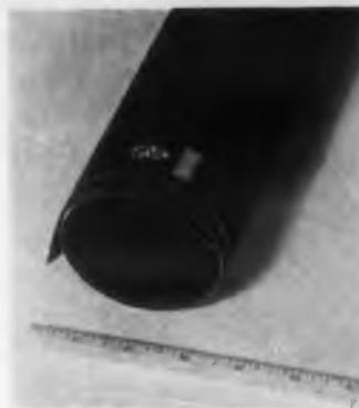
Grade FM is a low cost glass-mat polyester plastic insulation available in flexible form suitable for bending around corners or wrapping in cylindrical forms. It is heavy enough to give substantial mechanical support, flexible enough (in 1/32 in. thickness) to bend to a 3 in. diam without loss in dielectric strength, and heat-resistant enough to withstand continuous exposure to Class B temperatures (130 C) without loss in dielectric strength.
