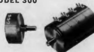
Precision 2" dia. single-turn potentiometer. Standard Resistance Range—20 $\Omega$  to 75 K $\Omega$   $\pm 3.0\%$ . Standard linearity  $\pm 0.3\%$ . May be ganged—2 to 15 sections. Up to 21 extra taps per section.
