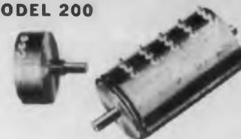
Precision 1 3/4" dia. single-turn potentiometer. Standard Resistance Range—5 $\Omega$  to 65 K $\Omega$   $\pm 3.0\%$ . Standard linearity  $\pm 0.3\%$ . May be ganged—2 to 15 sections. Up to 21 extra taps per section.
