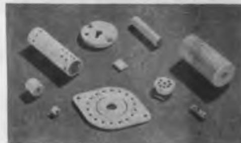
The new treatment consists simply of a dip in Dow Corning 200 Fluid followed by a short baking cycle, contrasted to the costly individual air-brushing and high temperature kiln-firing required for a glazed surface. The silicone treatment gives equivalent or better moisture resistance and surface resistivity for all but the highest frequency applications.
