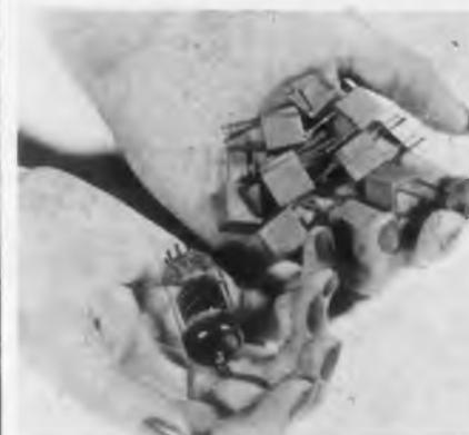
Ferristors, developed to replace vacuum tubes in electronic equipment are now available as independent standard products. They are reliable, lightweight, low power components,
