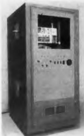
The Model PC 40 Pulse Modulator, when used with an appropriate high-voltage dc supply, provides up to 50 kv positive output pulses. Pulse width is continuously variable from 5-200  $\mu$ sec at repetition rates up to 1 kc. Both pulse width and repetition rate are controlled continuously by knobs located at ground level. Pulse rise and pulse fall times are
