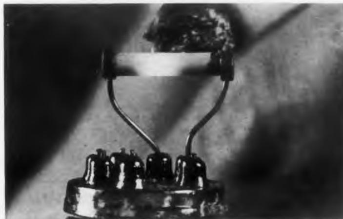
New resistors operate at heat level sufficient to light cigarette.
