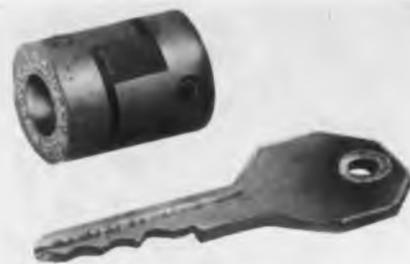
This miniature flexible coupling was developed especially for sub-fractional horsepower motors and other small units, such as used in coding devices, radar equipment, film and tape recorders, actuators, laboratory test equipment, aircraft components, etc. Rated at 1/20 hp at 1750 rpm, the full range is from 0.003 hp at 100 rpm to 0.103 hp at 3600 rpm. Dimensions are 5/8 in. OD x 3/4 in. overall length. Bore sizes are 1/8, 3/16, 1/4, and 5/8 in.
