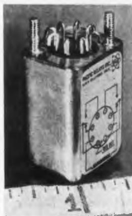
"CPL" Relays are for application where low and high temperatures are a major factor. Hermetically sealed or open, they are available in spdt or dpdt, in contact ratings to 5 amp resistive at 28 v dc, 115 v ac, or 3 amp inductive. Qualification test is to MIL 6106 A.
