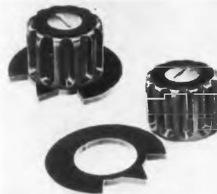
This military style knob, the type MK-2, is for 1/4 in. flatted shafts. It incorporates a positive locking collet which eliminates all possibility of inoperativeness due to loosening on the shaft. The collet snugly grips the shaft, evenly distributing locking pressure on all outside surfaces. It will not scratch or gouge the shaft surface. The collet is actuated by a slotted cap screw, made to fit screwdrivers.
