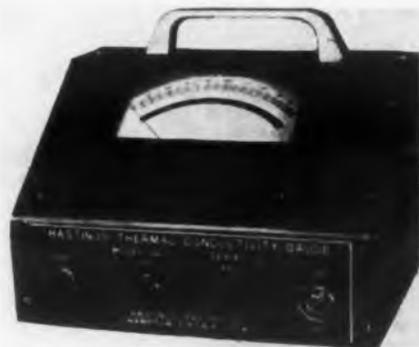
This thermal conductivity cell, used for determining the thermal conductivity of gases, is based on a patented compensated thermopile principle. It is designed to permit highly accurate measurements without the instability and temperature effects of older resistance type instruments.
