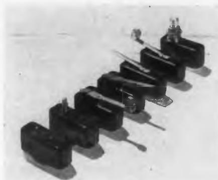
Licon (R) Type-10 series of limit switches offer movement differentials less than 0.0005 in., for use in operations requiring extreme sensitivity, and the exclusive "serpentine" snap action of the switches consistently gives more than 10,000,000 actuations in tests. The low stress design eliminates drift at the trip points.
