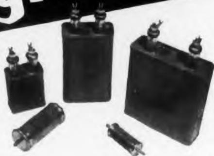
Capacitors designed and manufactured by Condenser Products Co., Division of New Haven Clock & Watch Co., are extensively used in calculators, computers, integrating circuits, electronic controls, sawtooth oscillators, and other equipment where stability and low dielectric loss are important.
