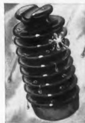
Furthermore, the film maintains high surface resistivity despite heavy contamination by air-borne fly ash, cement dust and earth particles. Its effectiveness appears to persist without maintenance for many years.
