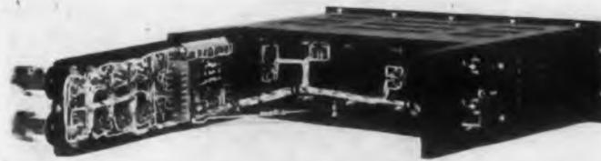
Rack model regulated dc power supplies offered by this firm feature germanium rectifiers and a panel height of only 7 in. Models rated at 800 ma are available for the ranges of 125-325 v and 325-525 v dc.
