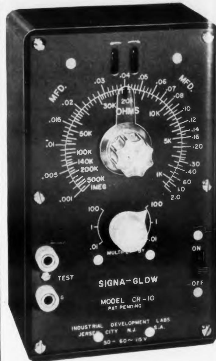
**M**ODEL CR-10 Signa-Glow is intended for use where measurement of capacitance and resistance must be made rapidly with moderate accuracy. The bridge, based on the Wheatstone Bridge principle, covers the ranges of 10  $\mu$ f to 200  $\mu$ f, and 5 ohms to 50 megohms.
