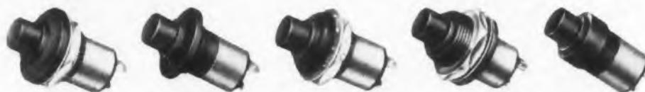
Designed to MIL-S-6743 drawing MS25089, these rugged, fully moisture-proofed snap action switches take a full 50 G shock and wide-amplitude vibrations up to 55 cps without contact transfer.
