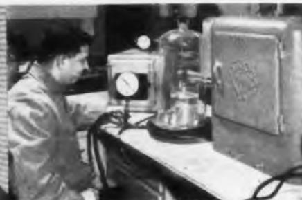
Seal tests under extremes of cold, heat, and vibration.
