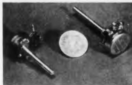
The Series 44 Miniaturized Control has many applications in transistorized assemblies such as hearing aids, pocket radios, portable radios, TV sets, portable test equipment, and printed circuits. It measures only 21/32 in. diam x 5/16 in. deep. It is rated at 0.2 w at 40 C.
