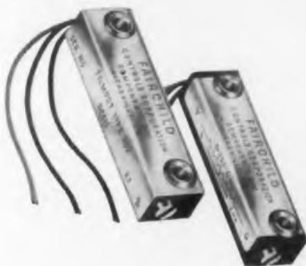
Fairchild FilmPot® trimmers are high quality potentiometers offering operating characteristics of infinite resolution, precision adjustment, and stability of performance over a temperature range from -55 to +175°C. The Nobl-Ohm® metallic film resistance elements are evaporated continuous films of precious metal alloys.
