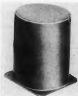
These coils employ special laminated Hipermalloy structures to provide extremely high Q and stability for low frequency (10-400 cps) applications. Laboratory adjusted to 2% accuracy at 1 v 60 cps, stability is such that inductance change is less than 1% for a 10 times
