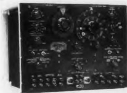
The Type 1391-A Pulse, Sweep, and Time-Delay Generator is a pulse source and measuring device designed to meet the diverse requirements of
