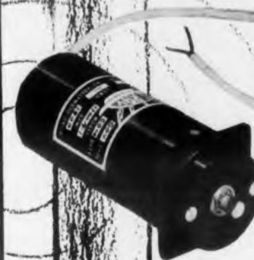
Measuring only 2.805" from mounting flange, El Ray's new 1700-9-1 series is a miracle in functional compactness. It features a governor controlled planetary gear train with integral filter. Now in production for important missile applications, this compact unit is highly effective in timing elements for telemetering, commutator switching and kindred functions.
