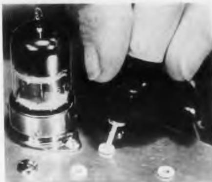
These color-coded "Press-Fit" miniature contact sockets to take the popular 0.080 in. test probes have been added to this firm's line, making sockets available for three different probe sizes: 0.040, 0.050, and 0.080 in. The Teflon bushing or insulator body measures only 0.185 in. diam with 0.218 in. diam front face, permitting spacing as close as 1/4 in. between centers.
