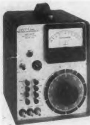
The Model 605 Resistance Bridge provides a means for rapidly and easily checking resistances to an accuracy of  $\pm 0.15\% + 0.05\%$  full scale. Seven ranges from 100 ohms to 100 megohms full scale are selectable by front panel pushbutton switches. The lowest measurable resistance is 5 ohms.
