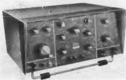
The Model BCT 300 Transistor Curve Tracer is for designing transistor circuits; comparing, matching, selecting transistors; detecting anomalies; studying effects of temperature, age, normal usage, and over-loading; and for detecting failures and cause. The unit is flexible and permits testing on all types in forward or reverse direction; it plots the entire family of curves on a standard laboratory dc oscilloscope.
