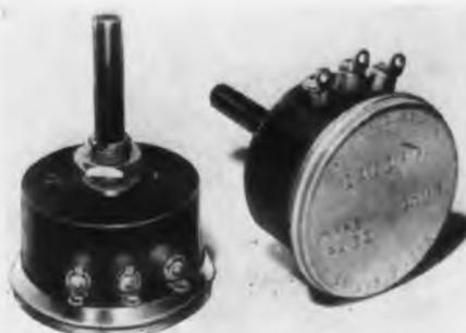
The DP-12 Potentiometer is designed to withstand environmental vibration, shock, and ultra-high altitude. It surpasses JAN-R-19 specifications calling out Type RA-30 potentiometer requirements. It is completely hermetically sealed. Difficulty in dissipating heat from a totally enclosed resistance is overcome by close fitting of the resistance element with the die cast aluminum case. Heat is rapidly transferred to the outside of the case, providing rapid heat radiation.
