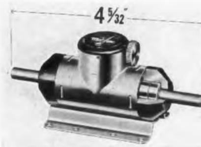
This adjustable ratio speed changer has anodized aluminum end bells with two pressed-fit ball bearings for each shaft, resulting in high concentricity and extremely smooth operation. Metal construction gives high resistance to impact and vibration. Increased stability over a wide temperature range is obtained because of close correspondence of coefficients.
