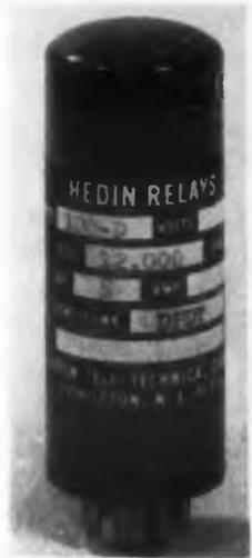
Incorporating a complete wiping action with sensitivity as low as 5 mw per contact, the Type 100-D Relay has an operating life rated well into the millions. It is designed for dc applications. The wiping action also has the advantage of eliminating bounce and chatter at normal operating voltage.
