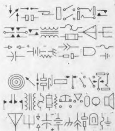
Electrical Symbol Template, for Leroy lettering and symbol-drawing equipment, that conforms to the new and revised Graphical Symbols prepared by the American Standards Association, meets military specifications. The new
