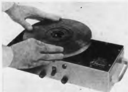
Two light-weight degaussers, the "5000" and the "2400", are offered for telemetry and sound recording. The standard-sized "5000" Eraser
