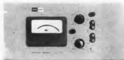
The Model 203R is a rack-mountable unit. It permits accurate current measurements from 10  $\mu$ amp to 100 ma and voltage measurements from 10  $\mu$ v to 1000 v, with an input impedance of 100 megohms and an output impedance of 2 ohms. The impedance accuracy is  $\pm 1.5$  per cent. The unit may also be used as a low drift dc amplifier with 80 db gain.
