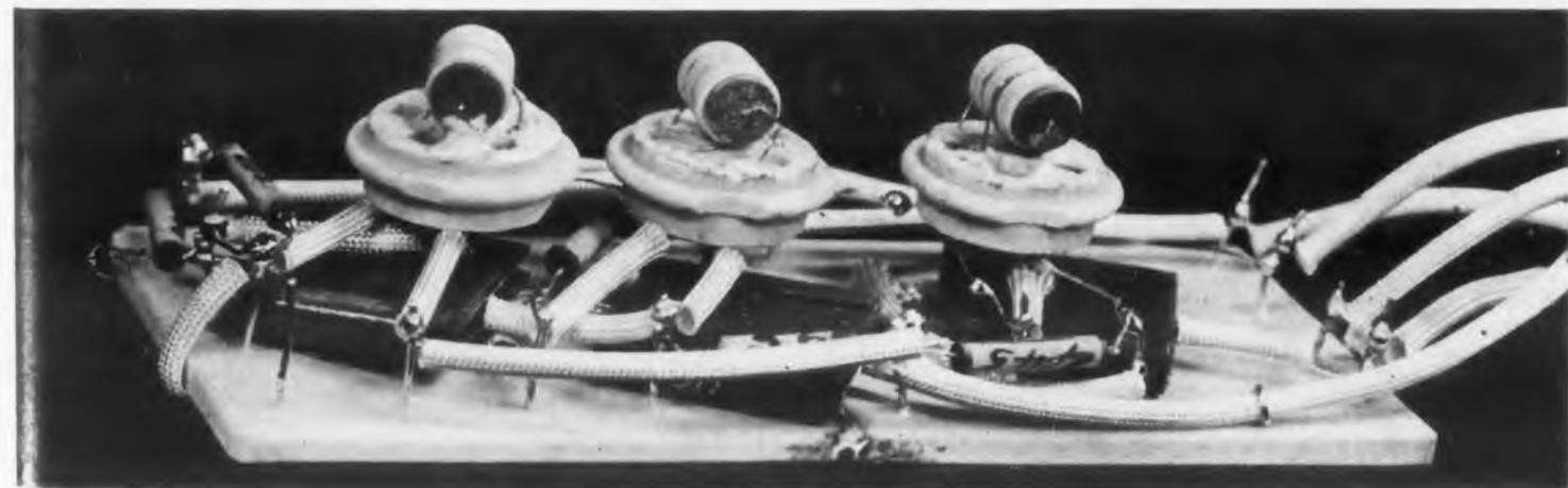
Shown here is a complete 3 stage circuit using all high-temperature components. The pancakes are tubes.
