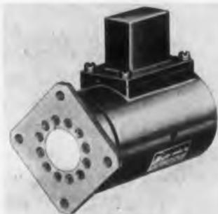
A Faraday rotation type ferrite isolator for airborne microwave applications, the Model W 152-2A weighs only 6 oz. It will handle 100 kw of peak power and give 25 db of isolation with an insertion loss of less than 0.25 over a 200-300 Mc bandwidth in the 8-12 kmc band. This new unit is one of a family of isolators available for the microwave, radar, and communication fields.
