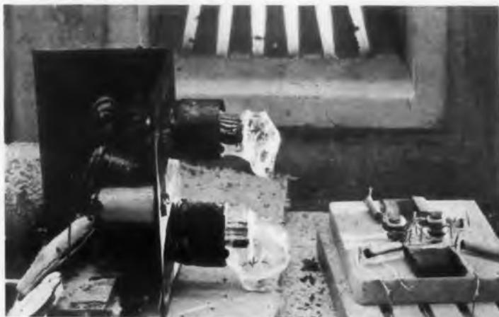
After 800 C oven treatment ordinary electronic components melt. New ceramic devices are intact.
