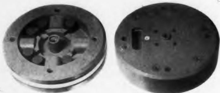
Fig. 4. Potting Mold—Two Halves
