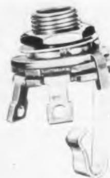
Currently supplied in three models, No. 334 (Jan Type JJ-034) is a 2 conductor open circuit jack, No. 389 (Jan Type JJ-089) provides a 2 conductor closed circuit, No. 333 (Jan Type JJ-033) is a 3 conductor open circuit type. All have heavy brass nickel plated frames and fit any standard mating plug.
