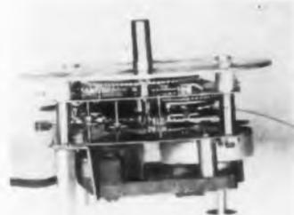
Highly accurate, the duplex time component runs electrically or mechanically and does not stop upon power failures. It consists of an accurate synchronous electric time unit combined
