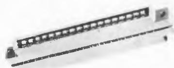
A new connector developed for pressurized printed circuits, has 15 coded contacts mounted in Or-
