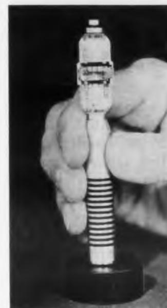
This small, accurate hardness gauge, can be used in measuring hardness of materials such as rubber and plastics. This gauge, called Rex Model A, indicates hardness in Durometer units that comply with A.S.T.M. specifications for rubber hardness.
