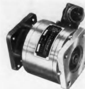
The wave shape is sinusoidal and frequencies to 240 cycles per revolution are available with this system. The output voltage is approximately 1 volt rms at 100 rpm.
