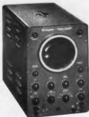
The Knight-Kit scope is designed for general purpose high frequency applications. Included among its features are a sweep range from 15 to 150,000 cps in 4 ranges; vertical response is down only 3 db at 700 kc (1000 cycle reference); high vertical sensitivity, 25 rms mv/in.; 1-v peak-to-peak, square
