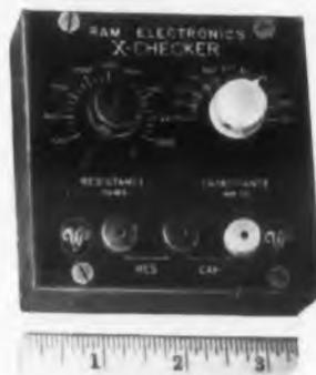
The X-Checker is a substitution box with a continuously variable resistor and capacitor which may be inserted alone or in series combination in an electronic circuit. The resistance range is from 0 to 2500 ohms. The capacitance range is
