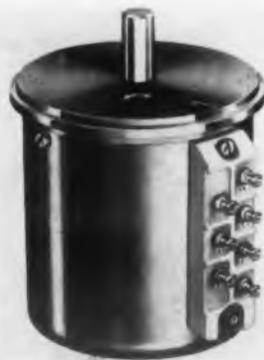
A 10-turn, 1-13/16 in. diameter unit for servo or 3-hole pilot mounting, this precision potentiometer has a choice of two windings; air-core winding with a range of total resistance from 200 to 5000 ohms; copper-mandrel winding from 5000 to 200,000 ohms.
