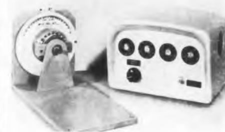
This dynamometer features a system of torque indication which is independent of speed, rotor bearing friction and external sources of me-
