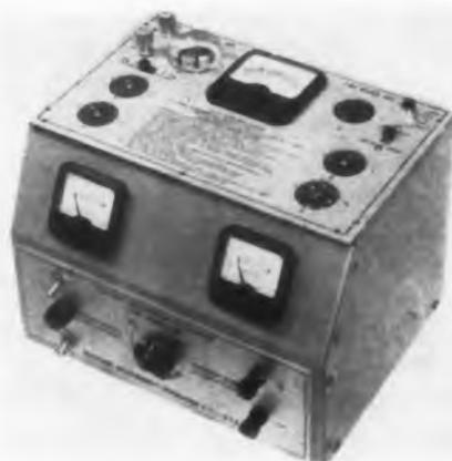
A combination battery eliminator and vibrator checker, EMC Model 905-6A, can supply 6 v at 10 amp or 12 v at 6 amp continuously. The output voltage is continuously variable from 0 to
