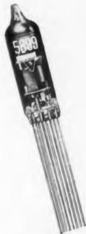
By providing a more realistic tube vibration test which can be adapted to large-scale production techniques, the "white noise" vibration test is contributing to greater tube reliability.
