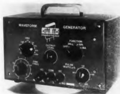
The first of a line of fully-transistorized, battery-powered test equipment, the Model 500 waveform generator provides clipped-sawtooth and
