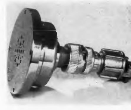
In the Type 4-340 dynamic pressure pickup, dynamic pressure applied to the diaphragm of a sealed, liquid-filled cell causes an infinitesimal amount of polar liquid
