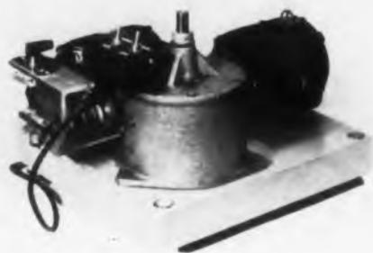
This 9 speed direct - shaft drive is designed for better recording equipment. Using two specially developed synchronous continuous duty motors, one worm gear and synthetic notched belts, the drive provides smooth, positive speeds of 16-2/3 - 33-1/3 - 45 - 66-2/3 - 78.26 - 90 - 156.52 rpm plus two additional speeds useful in lab work.
