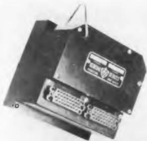
No force or phase adjustments are required in these switches which provide constant force brushes, and precision phasing. Available with one to three poles, up to 60 shorting or 30 non-shortening channels per pole, with 6, 12, or 28 v dc motor, shielded rf filter, spur gear reduction, and speed governor. Plugs are recessed and mounted into housing.
