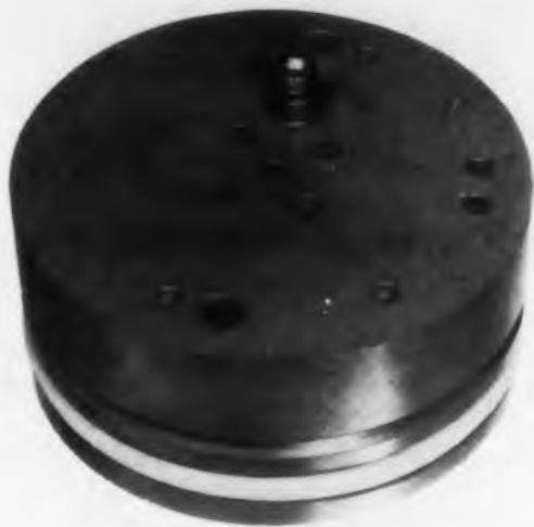
Fig. 3. Potting Mold Assembled
