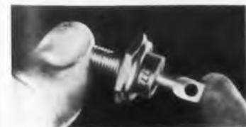
The silicon power rectifiers, type CK777, has a peak inverse rating of 325 v and an average current rating of 5 amp at 125 C. Maximum reverse
