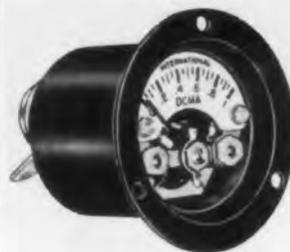
A new 1 in. round panel meter for flush mounting provides long scale arc in small panel space. The Model 104 employs a miniaturized D'Arsonval type movement, and accuracy is held to  $\pm 3$  per cent of full scale deflection for dc instruments and  $\pm 5$  per cent for ac instruments.
