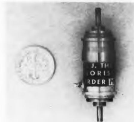
These miniature electromagnetic clutches have one input gear hub normally clutched to the output shaft while the opposite end input hub is free turning. When energized the
