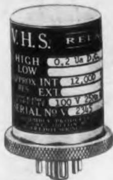
The Model 266 VHS relay has been modified for operation under shock and vibration and ambient temperatures of  $-55$  to  $150$  F. Sensitivities from  $0.2 \mu\text{amp}$  to  $10$  amp, or  $0.1$  mv to  $500$  v—with external multipliers even higher ranges of volts or amperes can be furnished.
