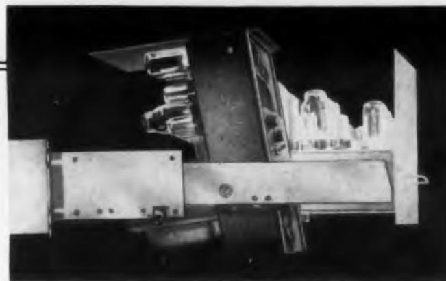
The Grant 3400 Thinslide requires only 19/64" space per side—installs readily in standard racks and cabinets. Allows instant access to chassis measuring from 10" to 16" deep. Tilts through 100° for under-chassis servicing. Positive lock in "out" position. Lock has finger-tip release for instant return or removal of chassis. Eight hardened steel rollers carry the rated load of 100 lbs. smoothly and easily—durability insures frictionless rolling for thousands of cycles of use.
