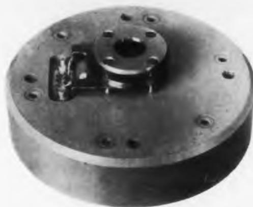
Fig. 5. Microsyn Mounted on Upper Half of Potting Mold
