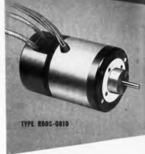
Holtzer-Cabot's Type 0810 has been used widely in gun fire control, radar navigation and radio tuning. Versatile and efficient, it features immediate response to minimum input signal. The armature is designed for continuous excitation from a 24 to 29 volt D.C. source through a 28 ohm series resistor. The field has two 10,000 ohm sections: one for CW and the other for CCW rotation. Full rated motor output is obtained by 6 ma. differential.
