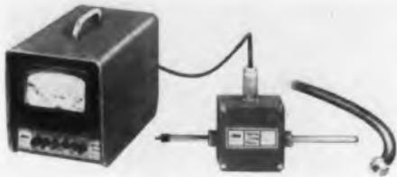
The MF-2 speed-feed meter measures and indicates linear rates of travel and rpm in a
