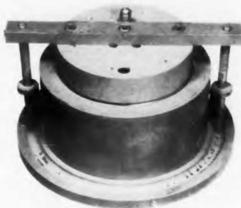
Fig. 6. Assembled Mold Preparatory to Potting
