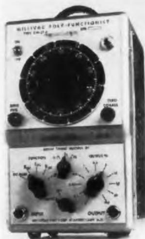
This new combined shunt box and Wheatstone bridge facilitates electrical measurements in chemistry and physics. The CM-21A Poly-Functionist uses a 10 Kohm 10 turn Helipot control alternatively as a calibrated shunt for the measurement and recording of dc currents or as the measuring arm of an ac or dc Wheatstone bridge. When used as
