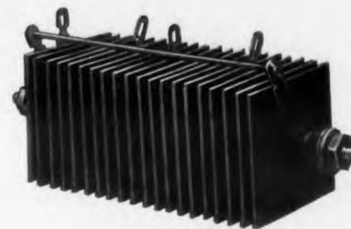
Guiding the 120 electric clutches that act as automated fingers in a new rug tufting machine is a Warner control panel whose key components are six Radio Receptor rectifiers. These fingers "feel" the rug pattern on a revolving roll, send information to the control station from which actuating impulses are relayed to clutches controlling yarn feed.
