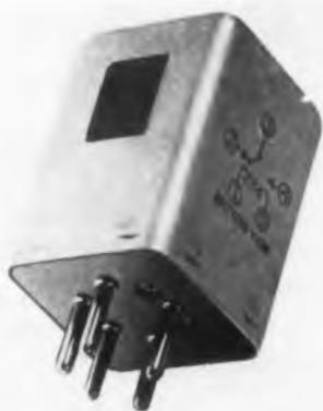
A new photoelectric control utilizes a broad area cadmium sulfide photocell and a relay, which are mounted on a 5-pin plug-in base and housed in a dust can measuring 1-1/2 in. square x 2-1/4 in. high.
