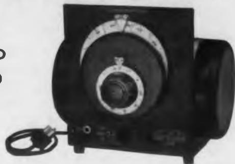
Delivers 200 mw into 50-ohm load . . . direct-reading to  $\pm 1\%$  with precision slow-motion drive . . . warm-up frequency drift 0.1% . . . sine, square-wave pulse or frequency-variation modulation can be applied . . . for general-purpose laboratory use with power and shielding adequate for driving bridges, slotted lines and other impedance-measuring equipment.
