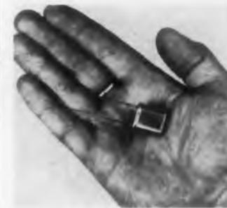
A snap-acting, disc-type thermostat for applications where maximum shock and vibration resistance are required, feature a disc thermal element, fine silver electrical contacts, and a complete hermetically sealed assembly.
