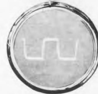
Photos show single transient pulses, 20 microseconds wide with a one microsecond rise time, showing writing capabilities of one million inches per second. These photos were taken in full daylight without a hood.
