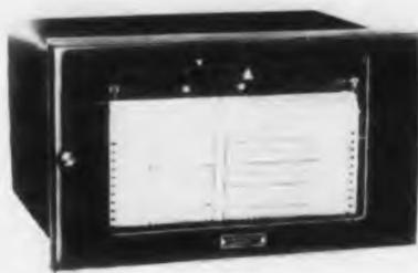
A two pen, 11 in. recording potentiometer designed for laboratory and field applications features a 3 speed selsyn motor chart drive which provides 1, 2, or 5 in. chart travel for 100 turns of the selsyn, or synchronous motor chart drives to provide standard chart speeds.
