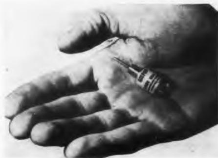
Only 1/2 in. x 1/2 in. in size, specifications of Acepots include: resistance range from 10 ohms to 250 K standard; weight 1/4 oz; power 2 w for 60 C rise; extremely high resolution; ambient temperature -55 C to 150 C; case is one-piece precision machined aluminum; available in standard threaded bushing, servo or flush mountings, and ganged units.
