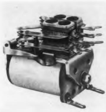
This miniature, telephone type multi-contact relay is suited for aircraft, computers, and data processing equipment. The Type 9 relay measures 1-5/32 in. long by 23/32 in. wide. It is available as a hermetically sealed unit,
