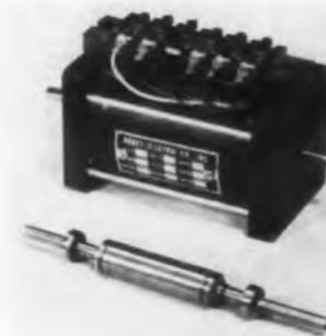
This new power servo has a high torque to inertia ratio and is capable of delivering 20 w output. The stall torque is min. 32 oz in. The torque to inertia ratio is 50,000, the weight only 4 lbs. The motor can be stalled continuously. The control phase can be wound for single phase or centertapped for push-pull operation. Full rotor without slots results in smooth operation. 10, 20 and 30 w servo motors are also available.
