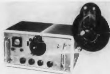
The Wide Range Type 504 heterodyne frequency meter is equipped with an interpolation dial which avoids ambiguity. Visual presentation is facilitated by a two inch CRT, and headphones can be used to determine zero beat. The instrument measures frequencies from 100 to over 10,000 mc. It can also be used as a calibration instrument because it generates frequencies from 500 mc to over 10,000 mc.
