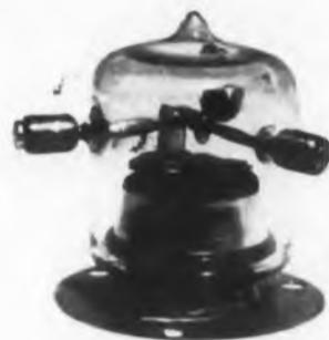
The Type JGF-RE2 single pole double throw vacuum relay is designed for antenna transfer switching applications in high altitude aircraft. It is a Type RE2 vacuum transfer relay that has been welded into a rugged gas-filled steel housing so that it can be
