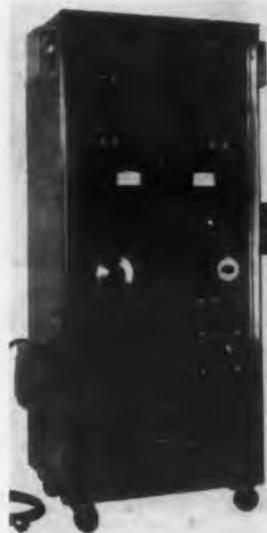
The Model No. 233 soft-tube pulse modulator provides a continuously adjustable range of pulse widths from 0.75 to 3.0  $\mu$ secs while using a thyratron as the switch. Output pulses up to a peak of 25 kv at 22 amps peak current are produced, and a maximum duty cycle of 0.003 makes available 1650 w of maximum average power. Included among the features of this equipment are a built-in oscillator for internally controlling the
