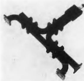
This Ku band divider was designed to operate over the frequency range of 16 to 17 Kmc. It presents a maximum input mismatch of 1.2 and a maximum insertion loss of less than 1/2 db. The unit
