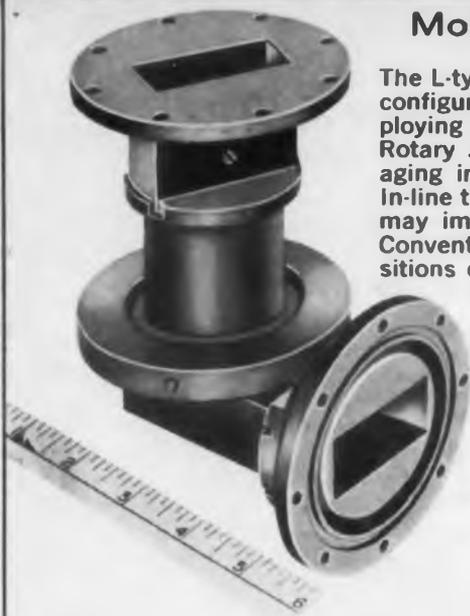
The L-type Rotary Joint illustrated is one of three configurations available for use at C-band employing Canoga designed transitions. The L-type Rotary Joint was designed for convenient packaging in radar systems and antenna pedestals. In-line transitions on both ends of the rotary joint may improve packaging in certain applications. Conventional rotary joints with right angle transitions on both ends are also available.
