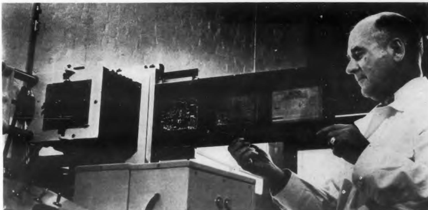
This projector is used for blowing up 105 mm negatives onto blueprint-size sheets of photopaper for exact reproductions of original engineering drawings.
