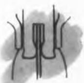
**New whisker mounting**—The use of a crimp hold rather than impulse weld to mount the whisker eliminates the possibility in production of overheating the tungsten whisker. Thus, the conductive properties remain undisturbed, assuring more reliable performance over longer life.
