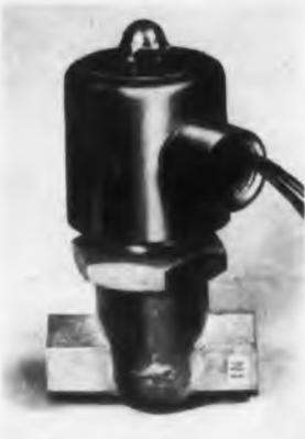
This solenoid valve for air pressures up to 100 psi, the Electroflo, may be secured with a full 3/8 in. or 3/4 in. orifice. Continuous duty solenoids are available from 6 v dc to 440 v ac. The overall length of the 3/8 in. valve is 2-17/32 in.; the 3/4 in. valve, 3-3/4 in. The inlet center to top dimension of the 3/8 in. valve is 4-3/8 in.; the 3/4 in.
