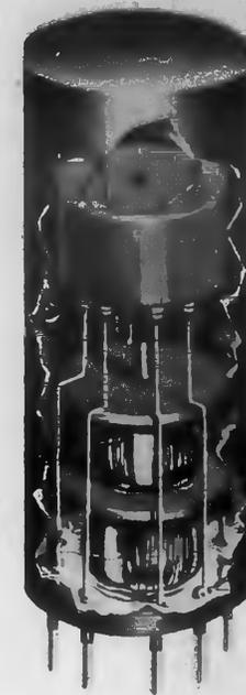
Designed for reliable operation at speeds up to 500 kc with maximum digit repetition rate above a megacycle, the Datakor DK107 is a high-speed magnetic shift register unit using two-cores-per-bit. All components including the two cores and four gold-bonded germanium diodes are mounted on a miniature tube base and encapsulated in epoxy.
