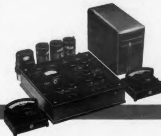
*The Weston Standard Cell Comparator Model 1000, made by Weston Electrical Instrument Corp.,\* Newark, N. J., with associated milliameters, dry cells, main galvanometer, and auxiliary standard cell.*
