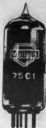
A new 75 v stabilizer tube, the 75C1, has been developed for application where low voltage stabilizers are normally employed. Mechanically strong, it combines zirconium electrodes and the sputtered envelope technique. A special uranium oxide coating ensures that the maximum striking voltage is 110 v in both daylight and darkness. The 75C1 has a current range of 2 to 60 ma with a regulation of only 9 v and a variation of burning voltage of less than 1 per cent per 1000 hours.
