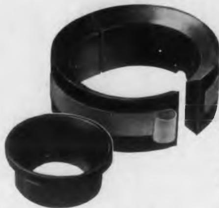
This ferrite "full-round" deflection yoke core for use in TV picture tube assemblies is pressed as a ring of perfectly uniform section and circularity. It is then "cracked" into two halves for
