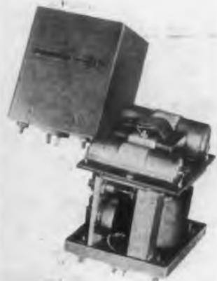
Four all semiconductor dc-dc converters are available with inputs of 12 and 28 v dc and filtered dc outputs of 325 v at both 100 and 200 ma. These supplies are hermetically packaged in cans 3-1/16 x 3-3/16 x 2-5/8 in. and are designed for efficient, reliable operation. The units can be operated in ambi-
