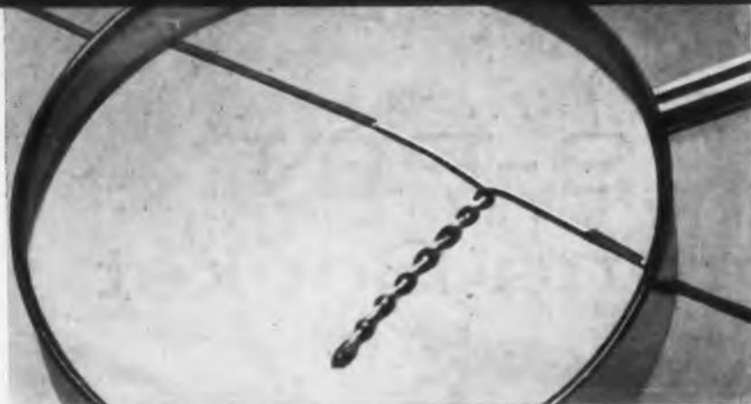
**1. STRONG JOINTS**—as strong as the same joints made in bare copper wire—are produced. Here in laboratory test, joint holds under high stress.
