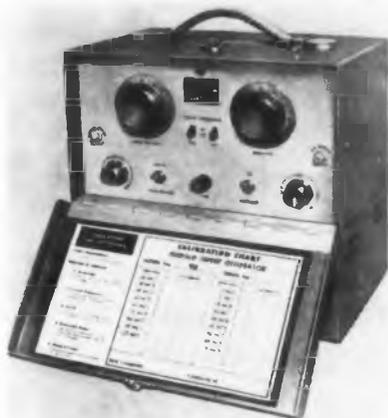
Two portable wide-band Sweep Generators, designed to cover the frequency spectrum from 22 mc to 216 mc, contain an all-electronic sweep circuit, of the saturable reactor type, with a sweep range of approximately 5 to 1. The rf output of
