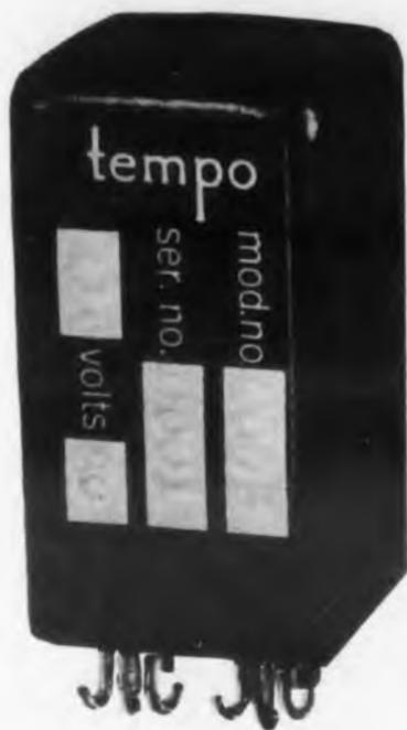
Both ac and dc models are available in a wide range of voltages and frequencies. The relay itself has dpdt contact arrangement, and contacts will handle a 2 amp resistive load. Power consumption is only 0.5 w.
