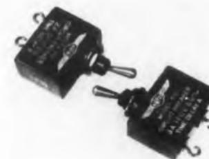
These miniature magnetic circuit breakers withstand 10 g at 55 to 1000 cps. The trip level is 135 per cent of rated load current. Units are available for interrupting 50 dc volts at currents from 0.05 to 10 amp and for interrupting 120 rms volts, 60 or 400 cps., at current from 1.0 to 10 amp. The toggle bushing of this breaker is the same as on conventional On-Off switches, enabling it to replace switches on electronic equipment.
