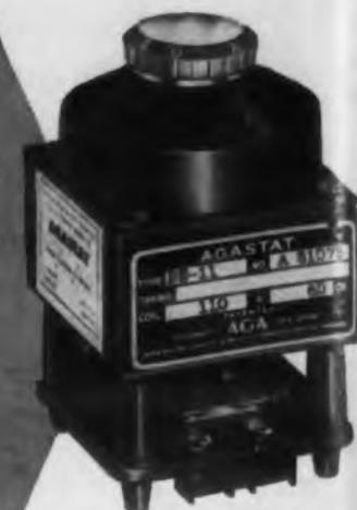
Frequent time adjustments are no problem with the dial head available on AGASTAT time/delay/relays. They provide a complete range of adjustment with 1 revolution of the dial. Dial markings permit easy calibration for accurate adjustment. And you can spot each of the 4 timing ranges quickly because they are color coded: blue from 30 seconds to 15 minutes; red from 10 seconds to 2 minutes; yellow from 0.1 to 10 seconds; white from 0.1 to 3 seconds.
