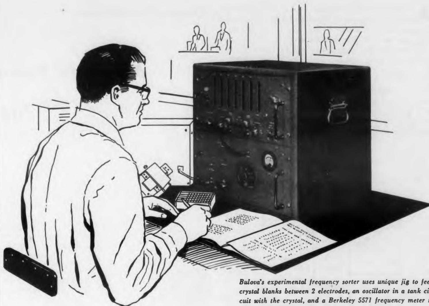
Bulova's experimental frequency sorter uses unique jig to feed crystal blanks between 2 electrodes, an oscillator in a tank circuit with the crystal, and a Berkeley 5571 frequency meter to give precise digital reading of frequency.
