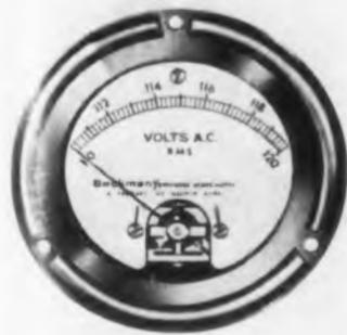
These expanded scale voltmeters embody a design which expands the useful portion of the conventional scale and eliminates the rest. The expansion is accomplished by means of a stable non-linear bridge, which is in balance at
