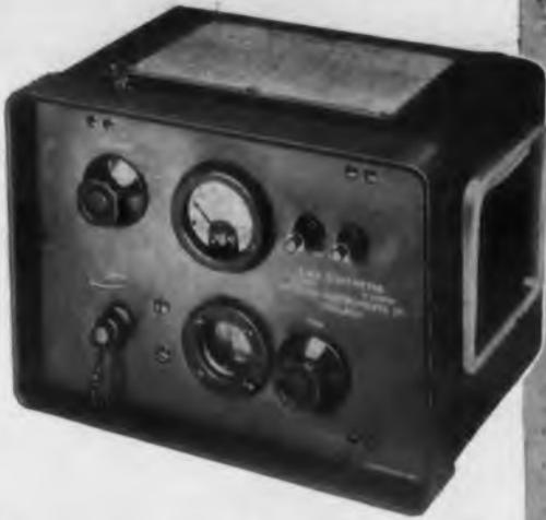
Model 1059 is the latest example of Marconi engineering skill and craftsmanship. Wide frequency coverage is obtained by use of a cavity oscillating in a hybrid mode, from TEM to  $TM_{010}$ . Tuning is by 2½" lens-viewed, sealed micrometer driving a non-contact plunger in the cavity.
