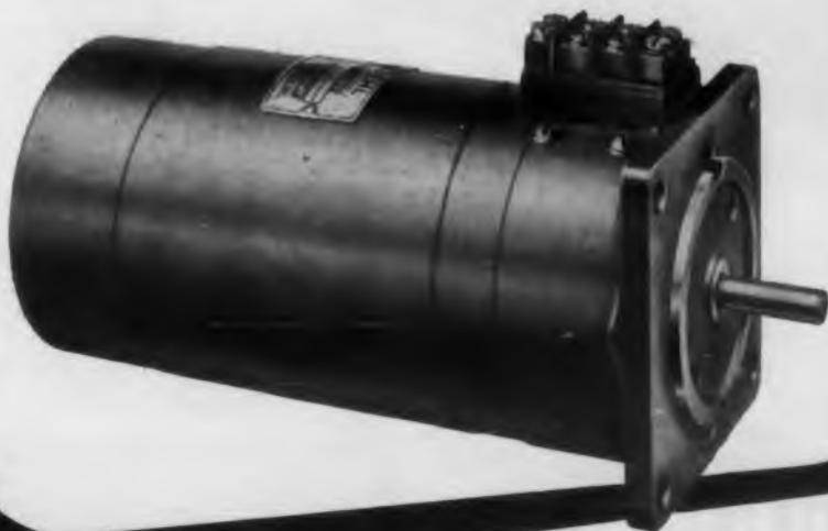
Linearity of this tachometer is within 0.02% expressed as a percentage of the output voltage at any speed from near zero to 4000 rpm. Unique design features maintain ripple voltages between 100 rpm and 4000 rpm at less than 0.04% of the output voltage and the magnitude of the ripple voltage decreases appreciably at speeds below 100 rpm.
