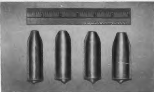
Single crystals of silicon, grown at Clevite Transistor Products Metallurgical Laboratory, demonstrate the unusual uniformity made possible by Clevite's crystal pulling technique.
