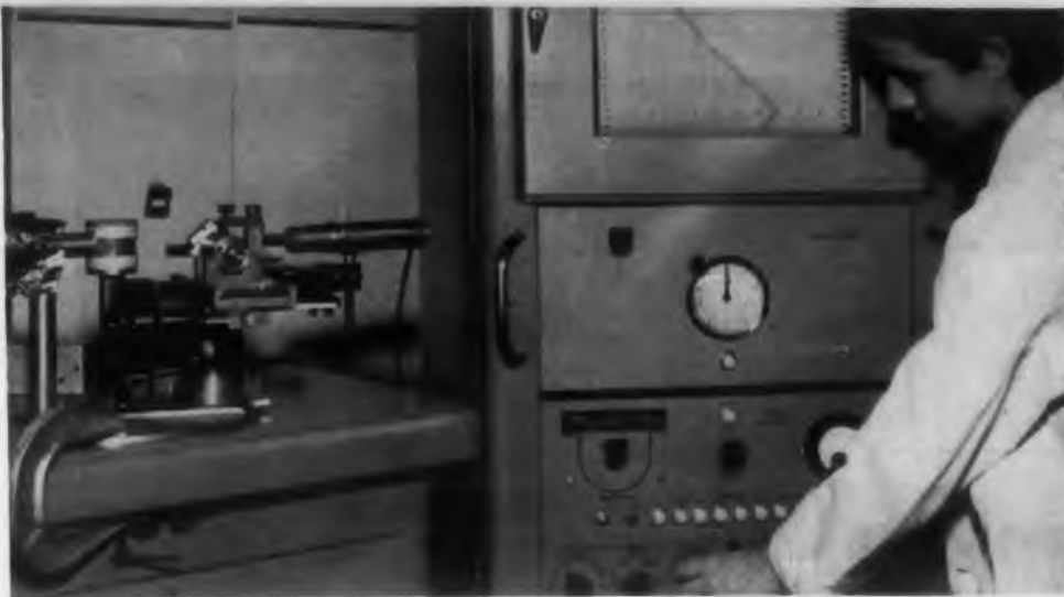
Crystal structures are double-checked in Clevite's Materials and Metallurgy Laboratory by X-Ray and Double Crystal Spectrometer to match crystal quality to specific application requirements.
