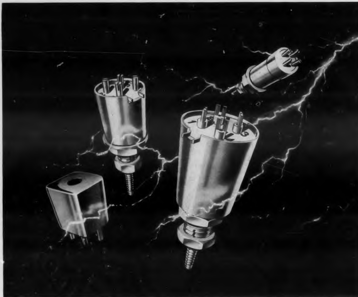
These shielded coil forms offer the utmost in reliability due to their unique design and construction. Dimensions when mounted, including terminals, are: LS-9, \frac{1}{16} " diameter x \frac{1}{2} " high; LS-10, \frac{5}{8} " x \frac{1}{16} "; LS-11, \frac{1}{16} " x \frac{1}{32} ". Each form mounts by a single stud. The LS-12 is a square type for printed circuits and measures \frac{1}{2} " x \frac{1}{2} " x \frac{1}{2} ". Single layer or pie-type windings to your specifications.
