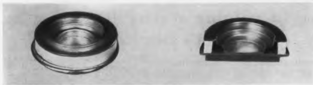
ACTUAL SIZE OF G-E germanium and silicon rectifier cell, hermetically sealed in ceramic housing, is shown in side view (left) and cutaway (right).
