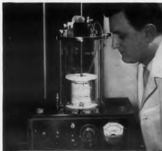
Continuous vertical crystal puller, developed by Clevite engineers, has tremendously improved the crystal-growing art. It is just one indication of the solid-state knowledge and volume production set up that keeps Clevite in the forefront of semiconductor developments.
