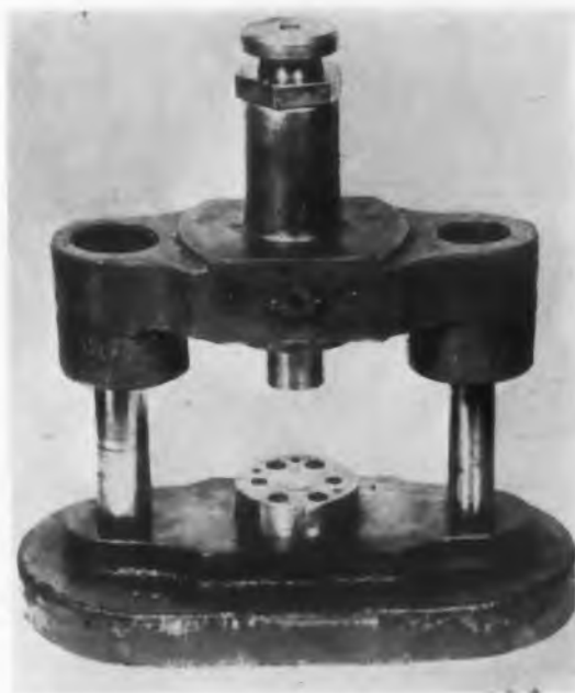
Fig. 3. Dies use carbide inserts pressed into a steel ring as shown. High accuracy results.
