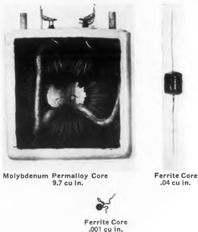
Fig. 1. Evolution of inductors. (upper left) Early molybdenum permalloy toroid; (upper right) currently available subminiature ferrite coil; (lower) micro-miniature ferrite coil now in the laboratory.
