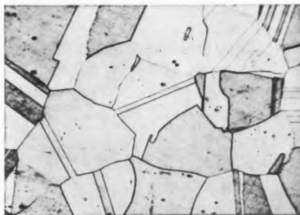
Vacuum melted NICHROME V, annealed. Note that reduced inclusions result in much larger grain size for the same annealing treatment.
