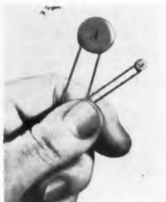
Centralab's "ultra-kap" and a conventional disc capacitor of the same rating.
