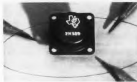
Diffused Junction Transistor Dissipates 15 W at 100 C
