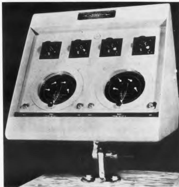
Fig. 1. Reduction in size of the Raydist Position Indicator is made possible primarily by use of watch-making techniques. Old Indicator is shown for comparison. Detailed requirements of micro-miniaturized computer-indicator are given in the text.
