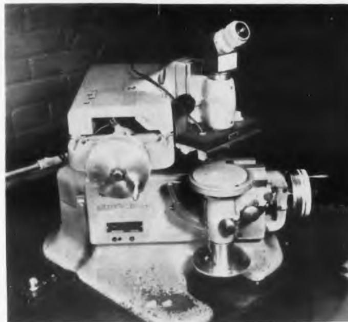
Fig. 5. This machine has its own built-in microscopic inspection device for close, accurate tolerances.
