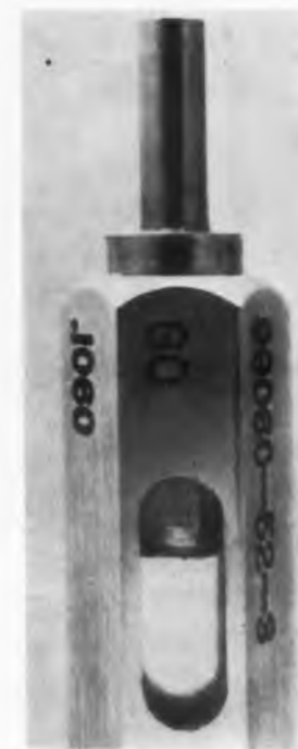
Fig. 6. Special "go-no-go" plug gage developed by Hamilton to assure close tolerances in holes.
