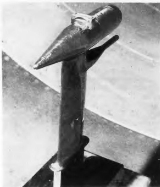
Air temperature sensing device as mounted on an aircraft.
