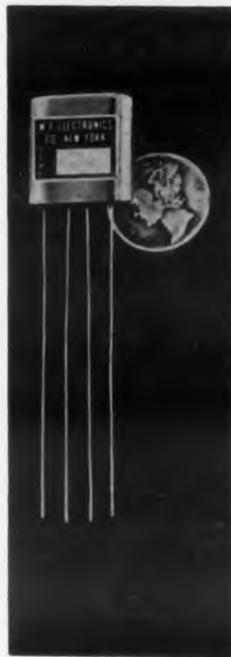
This 400 cycle multivibrator is one of a line of miniaturized circuit assemblies which will fit in less than one fifth of a cubic. M F Electronics Co., N. Y. features stability and reliability over a temperature range from -25 to +50 C. The circuits are encapsulated in epoxy resin in a drawn nickel-silver can. In the photo, Q1 and Q2 are Raytheon PNP transistors; R1 , R4 , C1 , and C2 are Glenco products, R2 and R3 are Allen-Bradley resistors and C3 is made by Ohmite.
