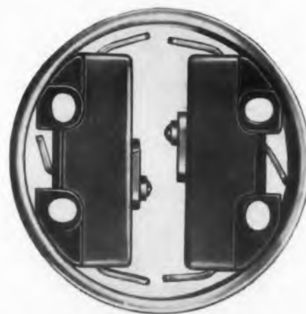
Two precision switches in a 1 in. diam case.
