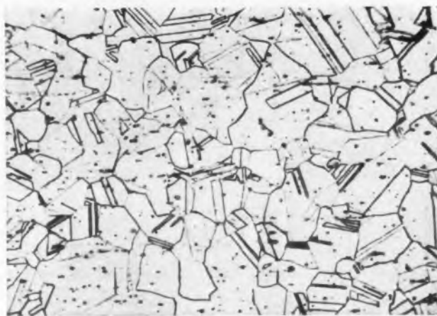
Polished and etched sample of Air Melted NICHROME* V in annealed condition.
