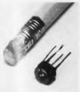
Fig. 1. A single stage transistor amplifier no larger than a pencil eraser.
