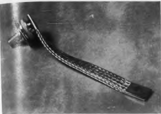
Fig. 1. This silicon rectifier cell is capable of carrying 140 average amp in a 40 C ambient, with 1,000 linear ft per min cooling air and mounted on a 6 x 6 x 1/4 in. copper plate. Standard stud mounting insures tight fit to cooling plate, using conventional nut. Power take-off is heavy braid for low resistance path.
