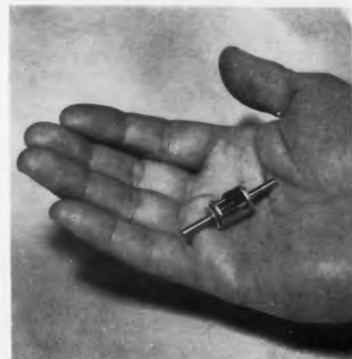
Mechanical differential (above), developed by the Pitometer Log Corp., is believed to be the smallest in existence. Overall diam. is 1/8 in. Weight is approximately 10 grams including typical end gears. Breakaway torque: 0.01 oz-in. (08. gm-cm). Unit employs sub-miniature ball bearings.
